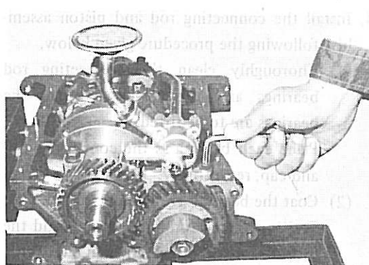
Fig. 3-75 Installing Oil Pump
