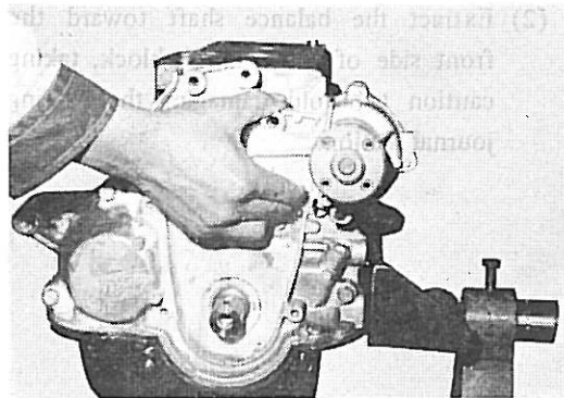
Fig. 3-47 Removing Water Pump
