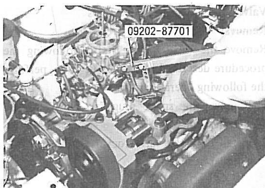
Fig. 3-120 Removing Valve Spring Retainer Locks
