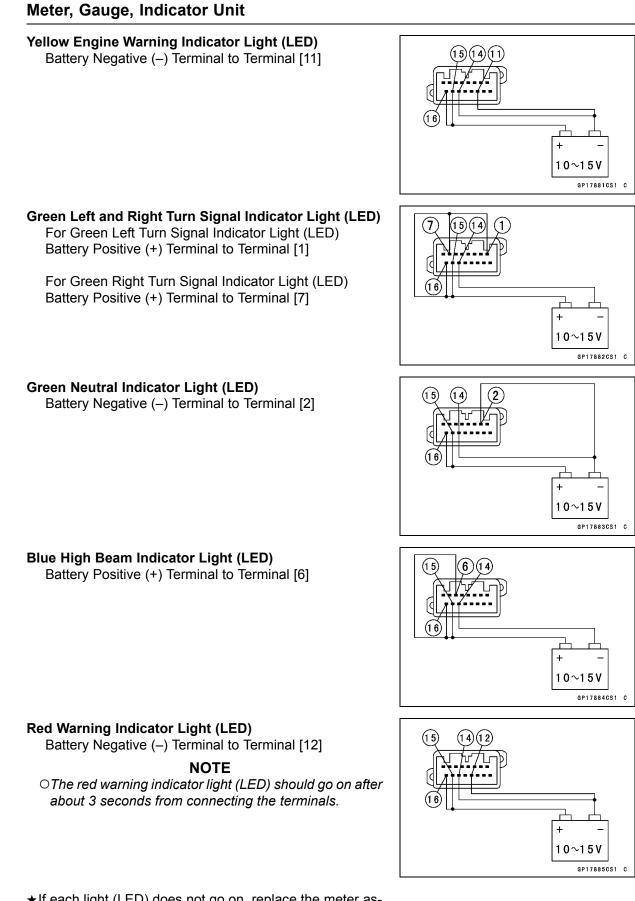
★ If each light (LED) does not go on, replace the meter assembly.
