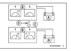
Battery [A] Battery Charger [B] Standard Value [C] Current starts to flow [D]
