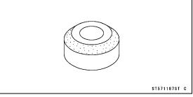
Valve Seat Cutter, 55° -  $\phi$ 35: 57001-1247
