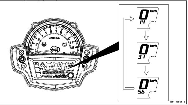
Olf there is no problem or when the repair has been done, the yellow engine warning indicator light (LED) goes off and service code is not displayed.
