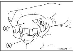
• Tighten the bleed valve, and install the rubber cap.
