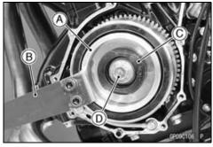
Using the flywheel puller assembly [A], remove the alternator rotor from the crankshaft.
