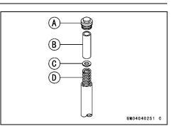
• Compress [A] the fork [B] upside down to draw out the oil into the suitable container [C].
