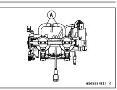
• Connect a vacuum gauge (special tool) and hoses [A] to the fittings on the throttle body.
