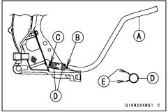
OApply molybdenum disulfide oil solution to the edge of the oil pipe [E].
