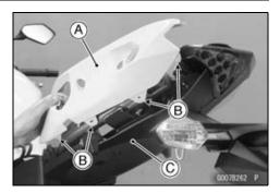
OInstall the center seat cover [A] so that the projections [B] fit into the slots [C].
