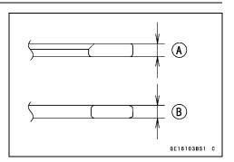
★ If any of the measurements is less than the service limit on either of the rings, replace all the rings.
