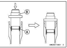
Install the needle bearings [A], ball bearing [B] and oil seals [C] as shown. Circlip [D] 42.5 mm (1.67 in.) [E] 24 mm (0.94 in.) [F] 41.5 mm (1.63 in.) [G] 5.5 mm (0.22 in.) [H]
