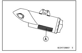
Muffler with Hole [A] for Oxygen Sensor [B]
