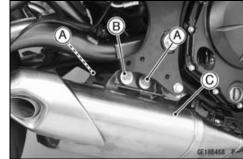
Remove: Muffler Body Mounting Bolts [A] Muffler Body Mounting Nut [B]
