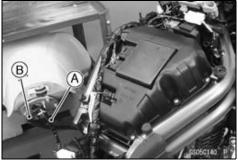
★If any one vacuum is not within the specification, turn in the bypass screws until it seats fully but not tightly.
