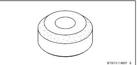
Valve Seat Cutter, 32° -  $\phi$ 30: 57001-1120
