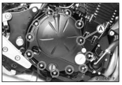
• Turn the release lever [A] counterclockwise, and remove the clutch cover [B]. About 90° [C]
