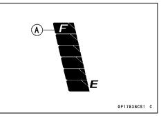
Check that the number of segments [A] matches the resistance value of the variable rheostat.
