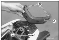
OInstall the grab rails and tighten the bolts.
