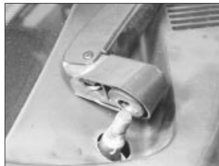
15.5 Removing the wiper arm from the spindle
