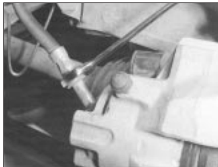
3.3 Loosening the flexible brake hose at the caliper
