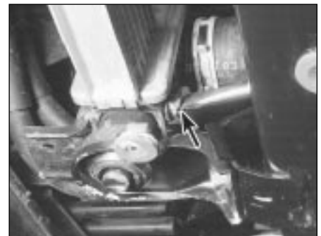
28.3B . . . to unscrew the radiator drain plug (arrowed) and empty the cooling system. Try to protect yourself from coolant splashing into your eyes or onto your skin, catching as much of it as possible in the drain tray
