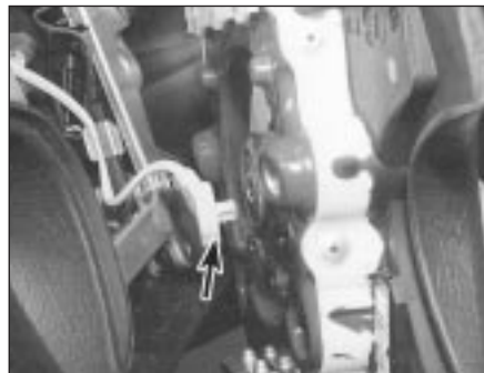
28.4 Disconnecting the air bag wiring multi-plug (arrowed)
