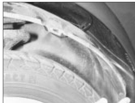
34.4 Removing a front wheel arch liner
