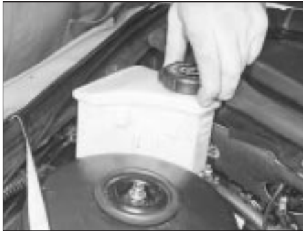
4.36A Unclip and lift power steering fluid reservoir - take care not to spill fluid . . .
