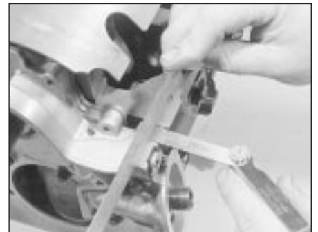
16.13 Check the oil pump is positioned correctly
