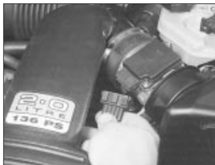
4.40 Unplugging the air mass meter's electrical connector . . .
