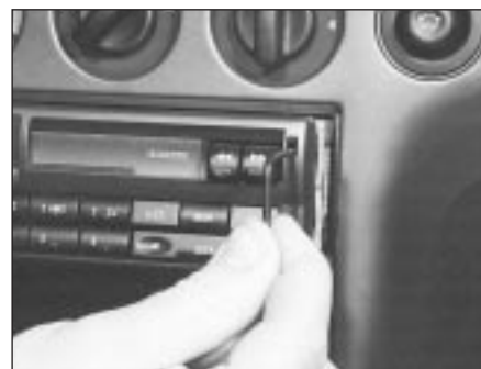
23.6 Using the special U-shaped rods to remove the radio
