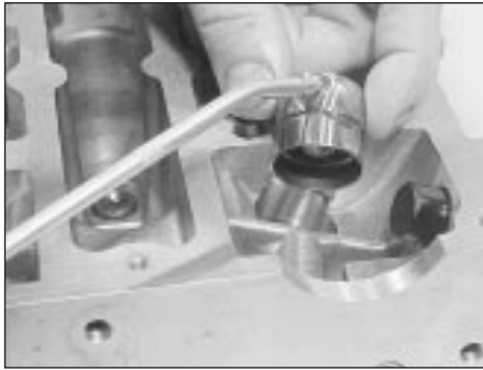
13.17 Oil liberally when refitting hydraulic tappets
