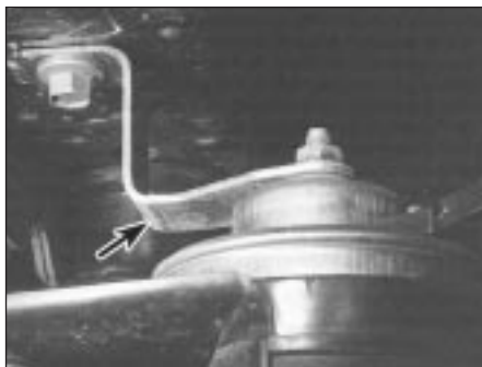
14.4 Horn and mounting bracket (arrowed)
