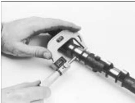
13.12 Measure each journal diameter with a micrometer - if any journal measures less than the specified limit, renew the camshaft
