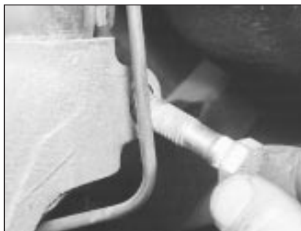
11.10B . . . and remove the knuckle-to-strut clamp bolt
