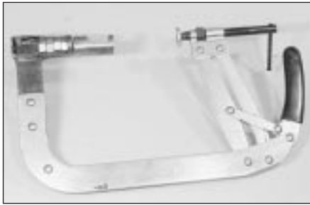
6.3A Standard valve spring compressor modified as shown . . .
