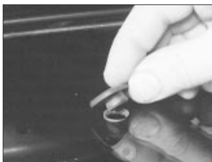
22.12B . . . and prise out the rubber grommet
