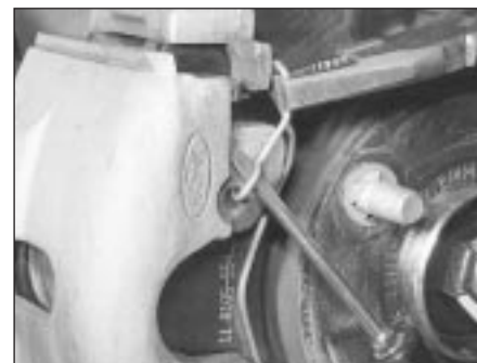
2.3A Prise the retaining clip from the caliper. Hold it with a pair of pliers, to avoid personal injury. On models fitted with pad wear sensors, it will be necessary to disconnect the wiring
