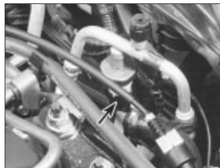
12.33 Unplug pressure-regulating switch electrical connector (arrowed)
