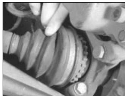
20.2 Check the driveshaft gaiters by hand for cracks and/or leaking grease
