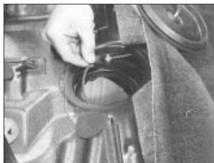
9.7B Fuel pump/fuel gauge sender unit's sealing ring must be renewed whenever it is disturbed
