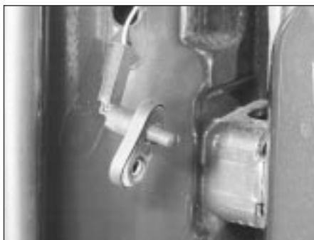
4.57B . . . and pull out the courtesy light switch
