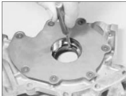
20.2 Driving out crankshaft right-hand oil seal
