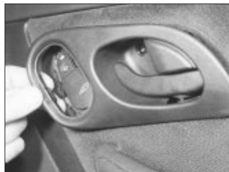
11.2C . . . and withdraw the bezel from the inner door handle
