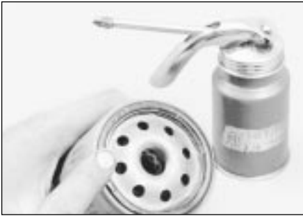
15.10 Lubricate the filter's sealing ring with clean engine oil before installing the filter on the engine
