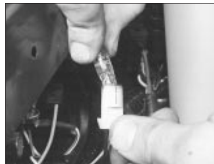
5.10 Pulling the wedge-type bulb from the bulbholder
