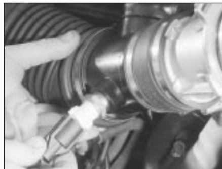
4.7 Unplugging intake air temperature sensor's electrical connector
