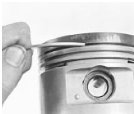
12.4B . . . or a section of a broken ring, if available
