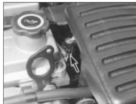
6.15 Location (arrowed) of coolant temperature sensor
