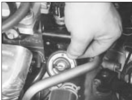
4.14 Ensure thermostat is refitted as shown
