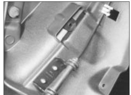
28.6A Detach the rear seat release cable
