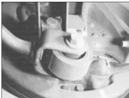
11.8A Tie-bar mounting bolt on knuckle
