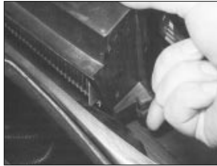
27.5A . . . release clips to lift out pollen filter housing . . .
