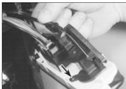
10.8 Unhooking operating cable from temperature control - note retaining screw (arrowed)
