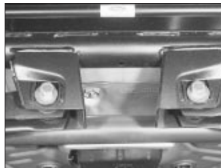
22.3 Bolts securing the rear lower arms to the crossmember - note the eccentric spacers
