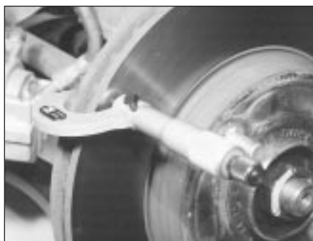
4.4A Using a micrometer to measure the thickness of the front brake disc
