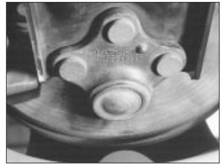
8.0 Original riveted front suspension lower arm balljoint
