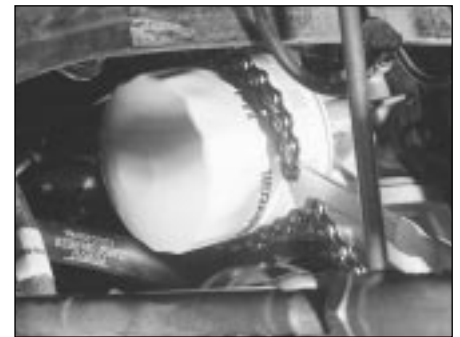
15.9 Since the oil filter is usually on very tight, you'll need a special wrench for removal. DO NOT use the wrench to tighten the new filter. Pack rag under the filter before removal to minimise the mess
