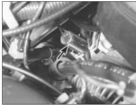
5.10 Charcoal canister-purge solenoid valve (arrowed) is clipped to bulkhead behind engine
