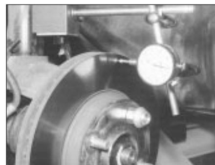
4.5 Measuring the disc run-out with a dial gauge
