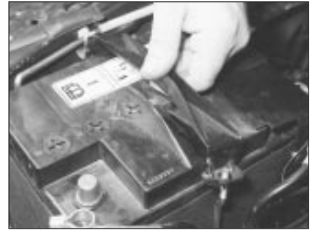
2.2B . . . and withdraw hold-down clamp to release battery
