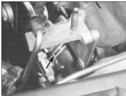
8.8 Power steering system pump should be removed to reach water pump hose union (arrowed)
