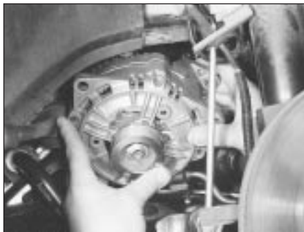
12.6 Alternator must be withdrawn through right-hand front wheel arch
