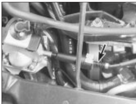
6.11 Location of TCS throttle actuator-to-throttle housing cable adjuster (arrowed)
