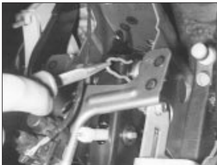
12.3 Removing the hairpin clip from the right-hand end of the brake pedal pivot shaft
