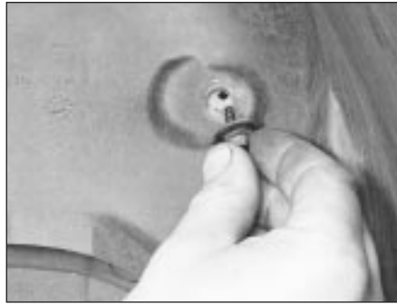
34.3 Removing a wheel arch liner retaining screw
