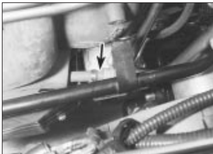
6.15 Unbolt exhaust manifold heat shield, and unscrew sleeve nut (arrowed) securing EGR pipe to exhaust manifold . . .
