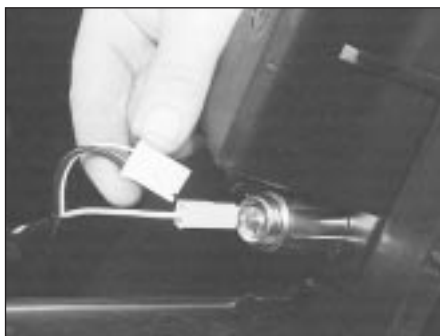
30.8 Disconnecting the cigar lighter wiring
