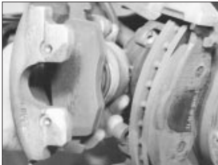
2.3E Withdraw the caliper from the disc, and support it on an axle stand to avoid straining the hydraulic hose. The outer pad will normally remain in position against the disc, but the inner pad will stay attached to the piston in the caliper
