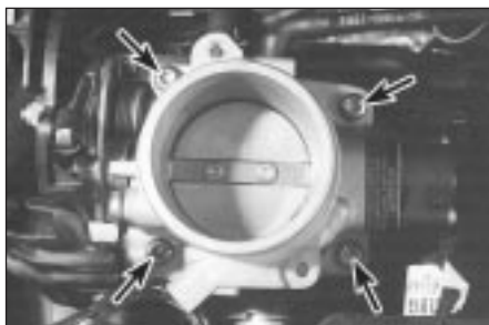
16.8 Undo screws (arrowed) to remove throttle housing
