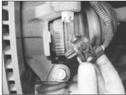
21.4 Unscrew the mounting bolt and remove the ABS sensor
