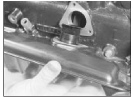
11.1C . . . unbolt crankcase ventilation system oil separator . . .
