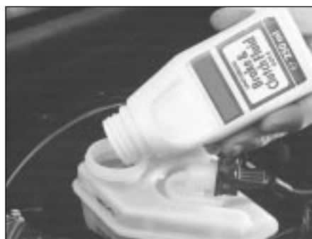
3.22 Topping-up the brake fluid reservoir
