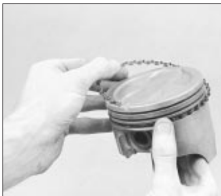
16.7B DO NOT use a piston ring installation tool when installing the oil ring side rails
