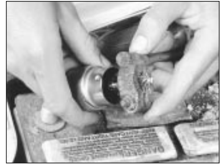
9.7A When cleaning the lead clamps, all corrosion must be removed - the inside of the clamp is tapered to match the terminal, so don't remove too much material
