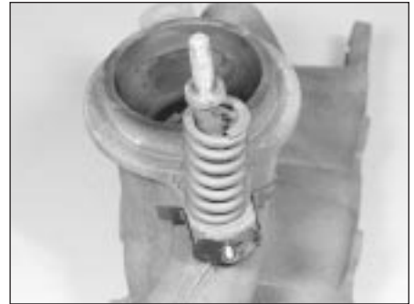
7.13A Showing exhaust downpipe-to-manifold securing bolts - note coil spring, and shoulder on bolt
