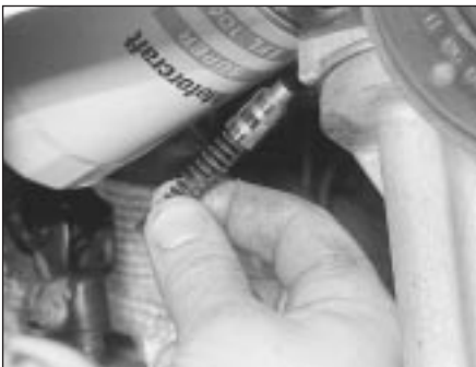
16.9B . . . to withdraw oil pressure relief valve spring and plunger
