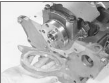
20.15 Use new gasket when refitting left-hand oil seal carrier
