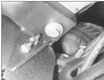
26.7B Rear suspension crossmember front mounting bolt
