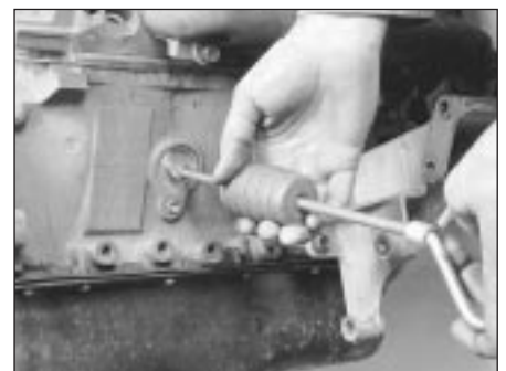
11.4 The core plugs should be removed with a puller - if they're driven into the block, they may be impossible to retrieve
