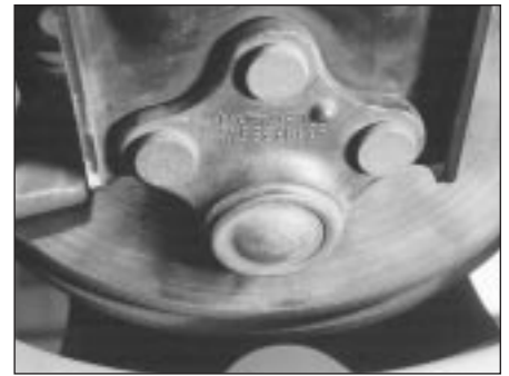
8.0 Original riveted front suspension lower arm balljoint
