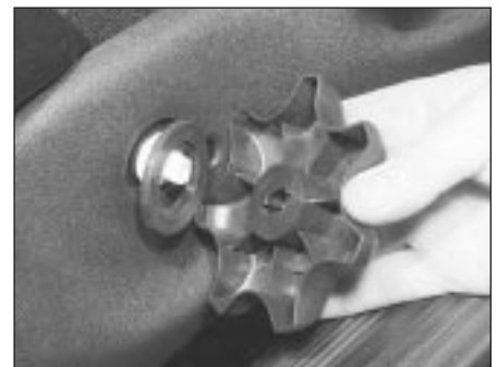
28.5A Remove the recline adjustment knob ...
