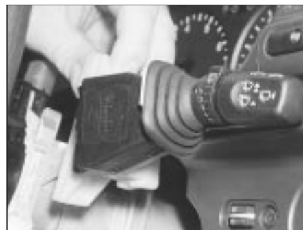
4.8B . . . and remove the windscreen wiper multi-function switch
