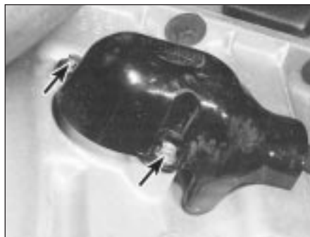
18.3 Remove screws (arrowed) to remove oil level sensor cover . . .
