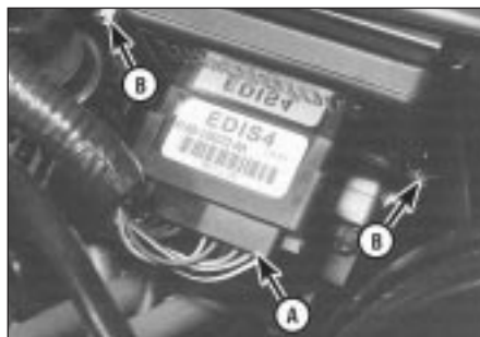
7.3 Separate ignition module is fitted to automatic transmission models only - note electrical connector (A) and retaining screws (B)
