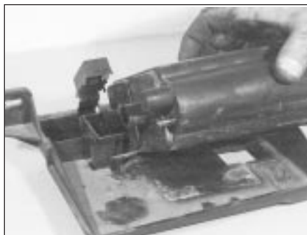
5.18 Release clip and drive out pin to separate canister from mounting bracket
