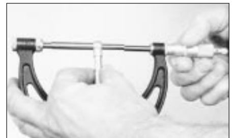
11.14C The gauge is then measured with a micrometer to determine the bore size
