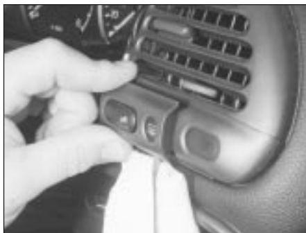
4.49 Prising out the heated rear window switch
