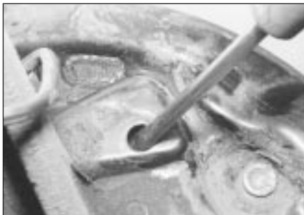
5.2A Releasing the automatic adjuster mechanism with a screwdriver inserted through the small hole in the backplate
