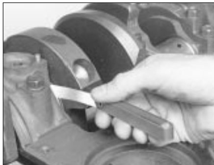
10.3 Checking crankshaft endfloat with a feeler gauge
