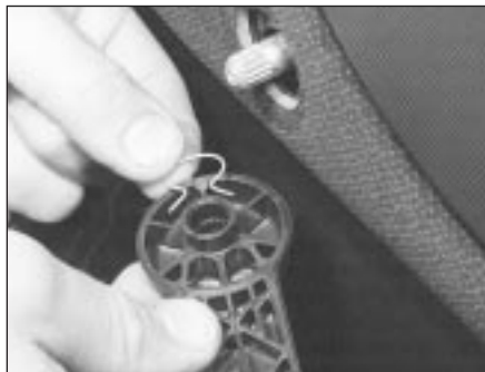
11.7C Recover the spring clip from the window regulator handle
