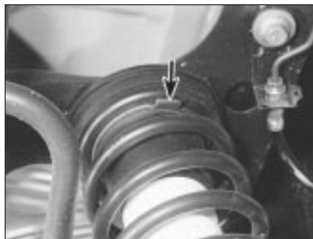
21.9 Correct location of the coil spring in the upper seat (arrowed)
