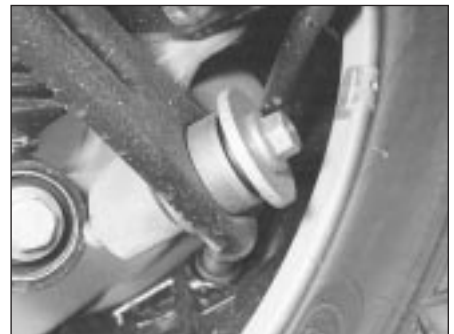
21.6 Front lower arm-to-knuckle mounting bolt
