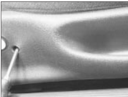
28.5B ... unscrew the trim retaining screws ...
