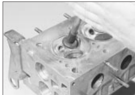
7.15 Grinding-in a valve seat - do not grind in the valves any more than absolutely necessary, or their seats will be prematurely sunk into the cylinder head
