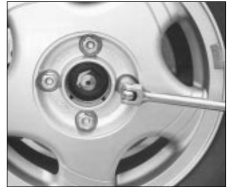
Slacken roadwheel nuts in diagonal sequence
