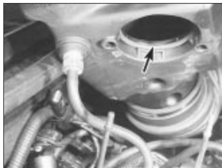
4.10B . . . and the sealing O-ring (arrowed) in the chamber's mouth
