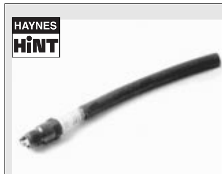
To avoid the possibility of cross-threading a spark plug, fit a short piece of rubber hose over the end of the plug. The flexible hose acts as a universal joint, to help align the plug with the plug hole. Should the plug begin to cross-thread, the hose will slip on the spark plug, preventing thread damage.
