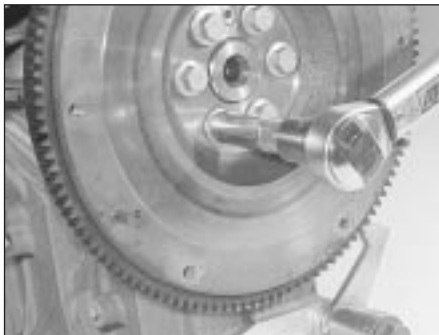
21.11 Note method used to lock flywheel/driveplate while (new) bolts are tightened
