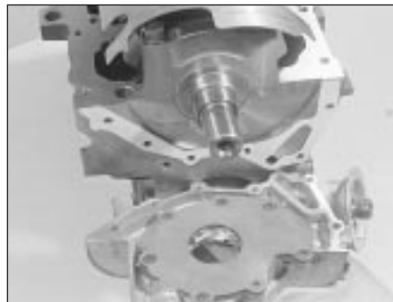
16.12 Use new gasket when refitting oil pump
