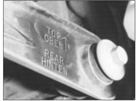
14.11 "TOP" marking on the rear lower arm
