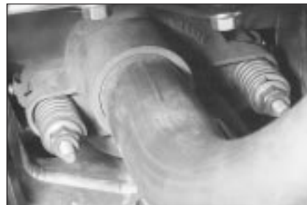
17.5 Tighten exhaust system front downpipe-to-manifold nuts as described - do not overtighten them
