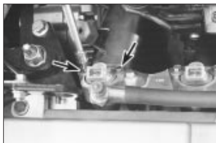
16.12A Fuel injectors can be unbolted (arrowed) . . .
