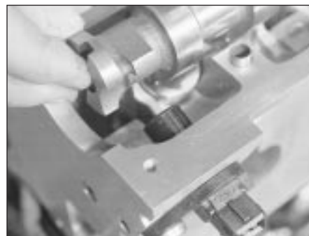
13.5B Inlet camshaft has lobe for camshaft position sensor
