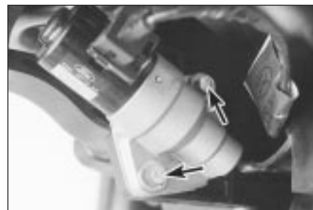
16.40 Unscrew bolts (arrowed) to remove idle speed control valve
