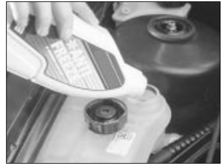
3.13 Remove the cap to add coolant only when the engine is cold - top-up to the "MAX" level line using the specified coolant mixture
