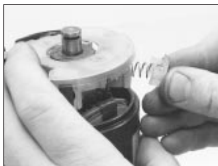
17.2D . . . then unclip the brush holders and springs . . .
