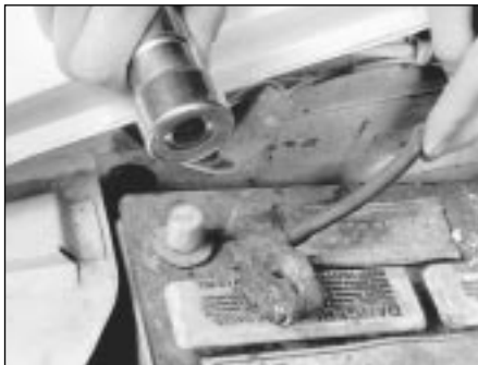
9.7B Regardless of the method used to clean the terminals, a clean, shiny surface should result
