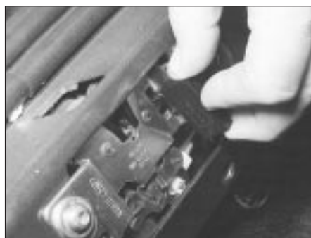
22.14 Removing the door-ajar sensor from the lock
