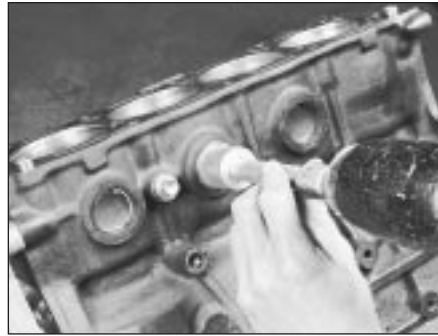
11.9 A large socket on an extension can be used to drive the new core plugs into their bores
