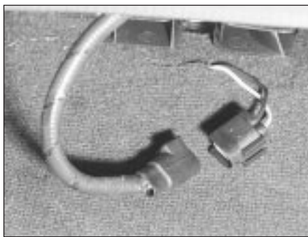
27.4 Disconnecting an electric seat multi-plug
