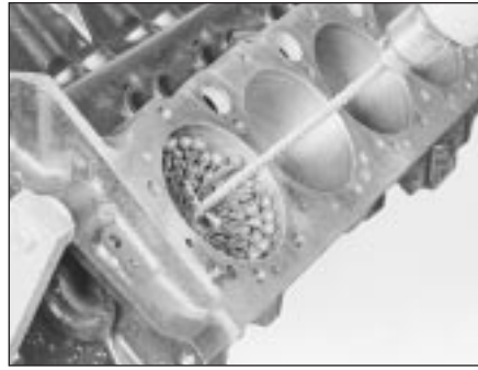
11.23A A "bottle-brush" hone will produce better results if you have never honed cylinders before
