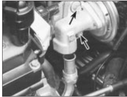
6.9B . . . unscrew EGR pipe sleeve nut and remove bolts (arrowed) to release valve from inlet manifold
