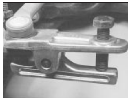
35.4 Using a balljoint separator tool to release the track rod end balljoint
