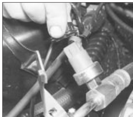
4.9A Unplug the power steering pressure switch electrical connector . . .
