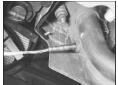
4.62 Oxygen sensor is screwed into exhaust system front downpipe . . .
