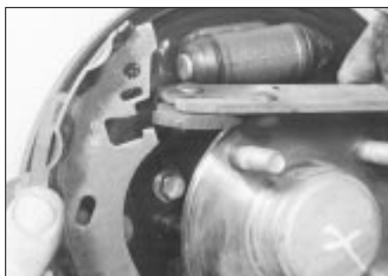
6.2I . . . and withdraw the leading shoe from the backplate
