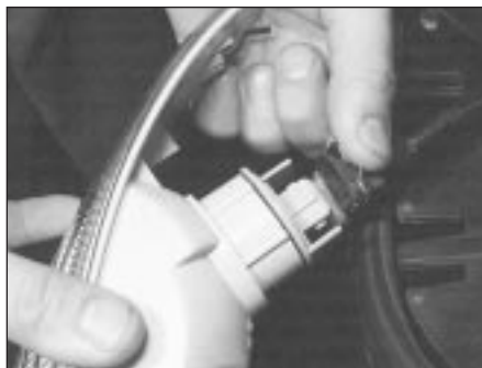
7.12 Disconnecting the wiring plug from the indicator bulbholder
