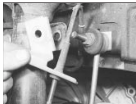
6.2B . . . and disconnect the anti-roll bar link and (on ABS models) the sensor wiring support bracket
