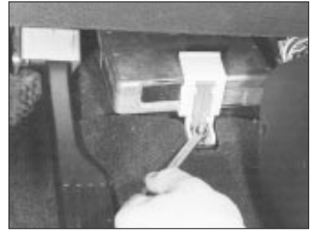
4.37 Unscrew retaining bolt and withdraw ECU's mounting bracket . . .
