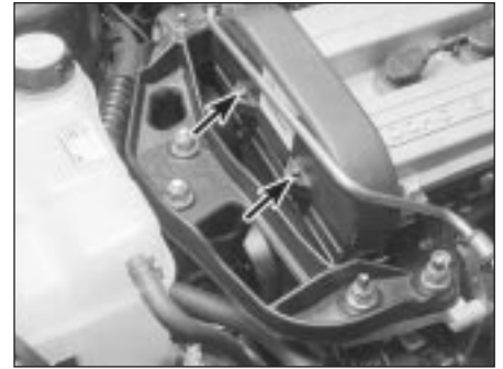
9.1 Remove bolts (arrowed) to release timing belt upper cover
