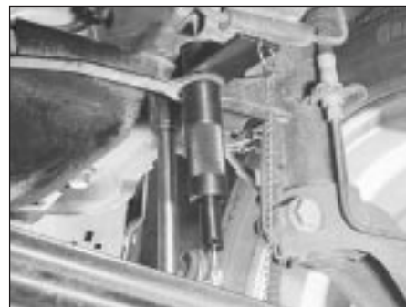
5.22 ... ensure aligned crossmember does not move - Ford tools used here - while mounting bolts are tightened
