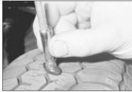
4.2B A tyre tread depth indicator should be used to monitor tyre wear - they are available at accessory shops and service stations, and cost very little
