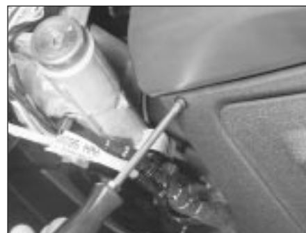
29.23A Unscrew the mounting screws from the upper corners . . .
