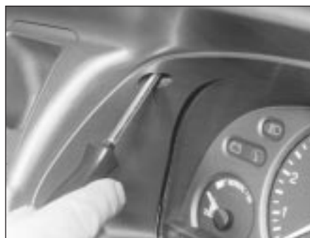
10.8A With the blanking covers removed, unscrew the concealed screws . . .
