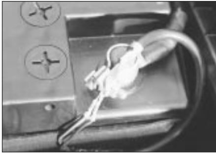
1.2 Always disconnect battery - negative (earth) lead first - to prevent the possibility of short-circuits
