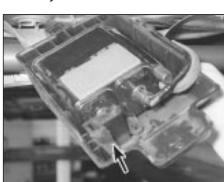
5.29 Charcoal canister assembly - Estate models - showing plastic cover (arrowed) and pin securing canister to mounting bracket
