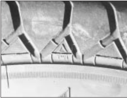
4.2A The TWI mark on the side of the tyre shows the position of the tread wear indicator bands
