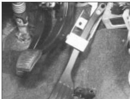
7.2 Removing the accelerator pedal assembly
