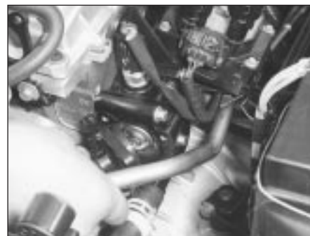
4.5 Unbolt water outlet to withdraw thermostat
