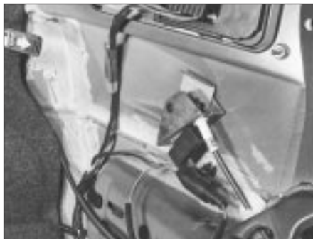
22.6 Tailgate lock barrel and bracket
