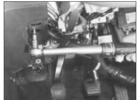
28.13 Tightening the steering column mounting bolts
