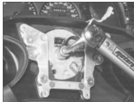
27.9 Tightening the steering wheel retaining bolt
