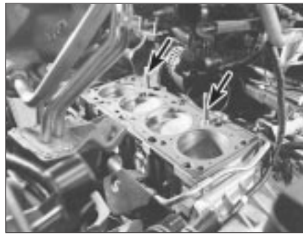
14.30 Refitting cylinder head - note fabricated guide studs (arrowed)
