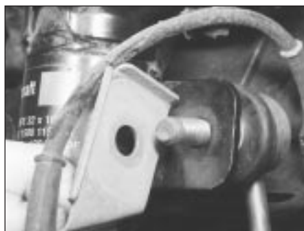
4.7 Removing the anti-roll bar link and ABS sensor wiring bracket
