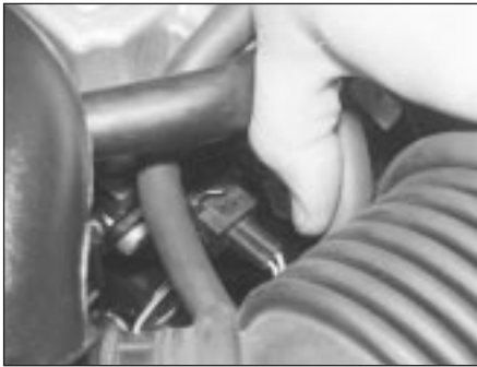
4.45 Camshaft position sensor is located at left-hand rear end of cylinder head
