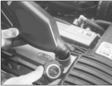
3.6 The yellow/black oil filler cap is screwed into the cylinder head cover. Always make sure the area around the opening is clean before unscrewing the cap, to prevent dirt from contaminating the engine
