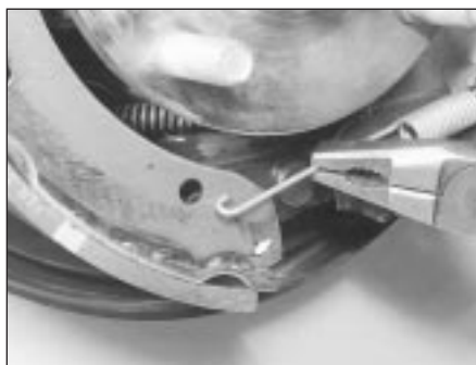
6.2F Unhook the lower return spring from the shoes, noting the location holes
