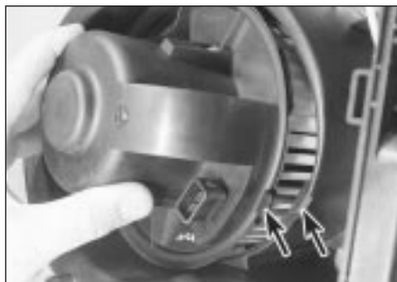
9.6 Ensure blower motor retaining lug (arrowed) engages securely in heater unit on reassembly
