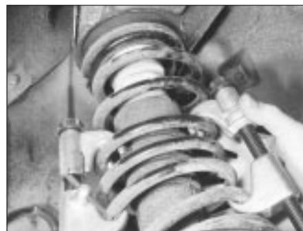
11.14 Removing the rear suspension strut
