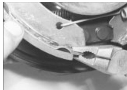
6.2D Pull the bottom end of the leading (front) brake shoe from the bottom anchor (use pliers or an adjustable spanner over the edge of the shoe to lever it away)
