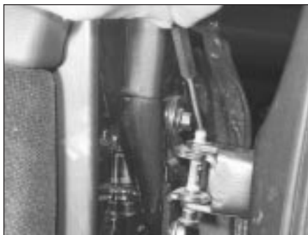
15.5A ... then drive out the hinge pins ...
