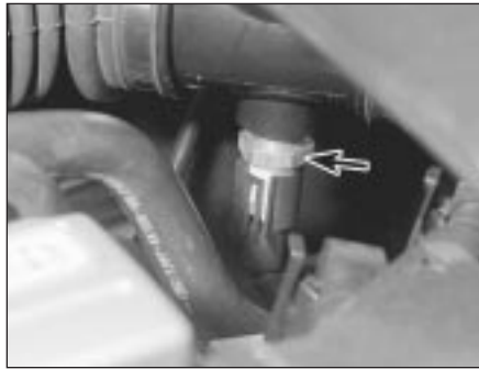
4.49 Intake air temperature sensor (arrowed) is screwed into underside of air intake resonator
