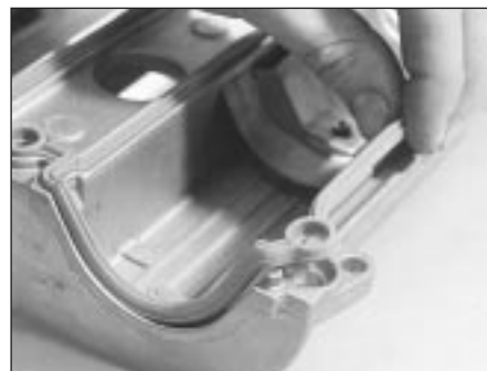
5.8 Ensure gasket is located correctly in cover groove
