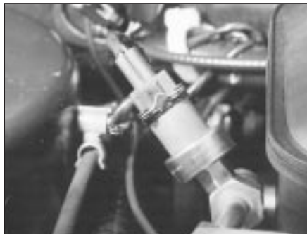
4.56 Power steering pressure switch is screwed into pipe at right-hand rear end of engine
