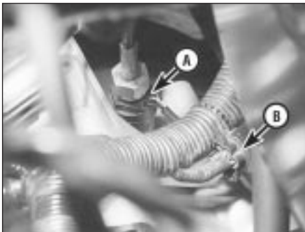
4.55 Vehicle speed sensor "A", with its electrical connector "B"
