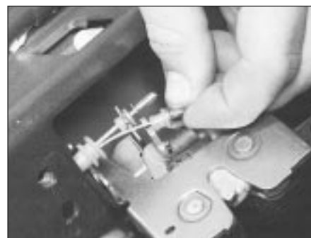
22.16 Disconnecting the cables from the lock
