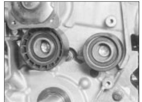
11.13 Tighten timing belt guide pulley bolts to specified torque settings on refitting
