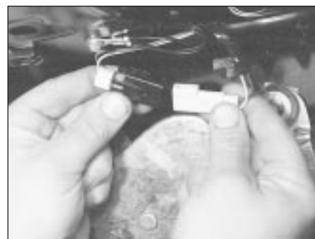
17.4 Disconnecting the tailgate wiper motor multi-plug
