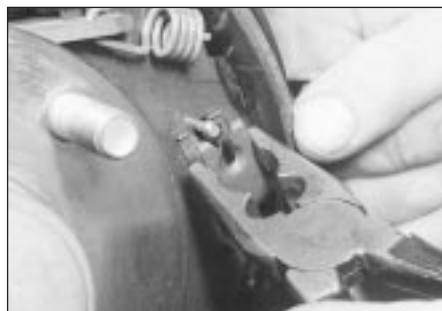
6.2B Remove the two shoe hold-down springs, using a pair of pliers to depress the upper ends so that they can be withdrawn downwards off the pins
