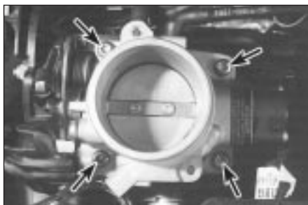
16.8 Undo screws (arrowed) to remove throttle housing
