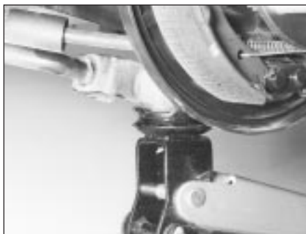
11.10A Support the knuckle on a trolley jack . . .
