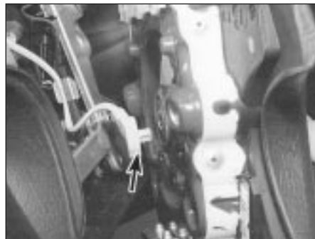
28.4 Disconnecting the air bag wiring multi-plug (arrowed)
