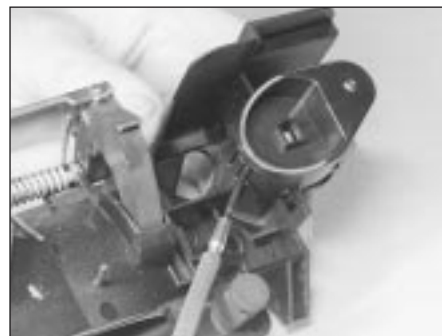
14.24 Prise out the barrel retaining tab . . .
