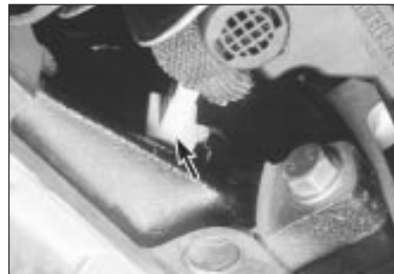
9.4 Location of crankshaft speed/position sensor - connector arrowed - in front of cylinder block/crankcase
