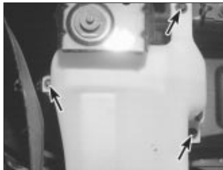
22.2 Washer reservoir mounting bolts (arrowed)
