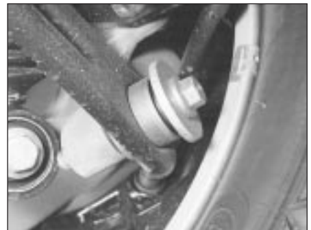
21.6 Front lower arm-to-knuckle mounting bolt
