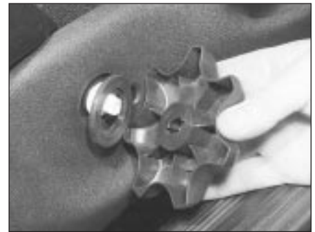
28.5A Remove the recline adjustment knob ...
