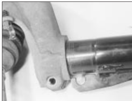
4.12B Releasing the knuckle from the strut
