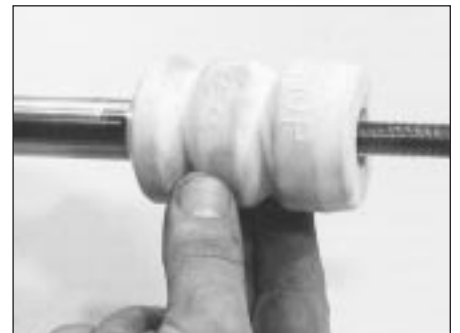
5.5D Removing the bump stop
