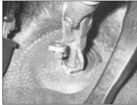
28.6B . . . and swivel the clamp plate around
