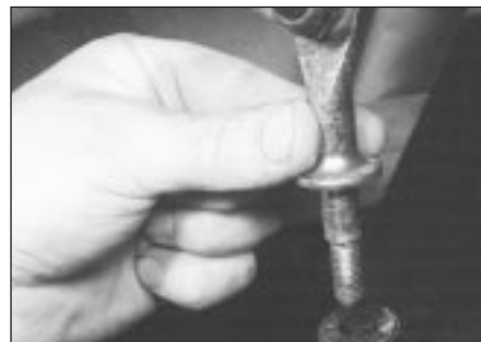
13.2C . . . and remove the anti-roll bar link from the lower arm
