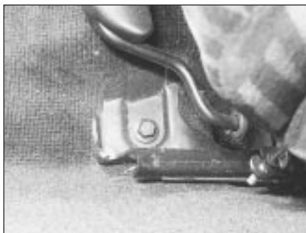
27.5 Front seat front mounting bolt
