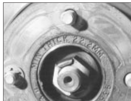
4.4B Disc minimum thickness marking
