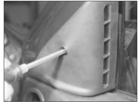
11.5A Remove the plastic cap and the screw . . .
