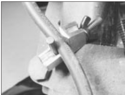
3.2 Brake hose clamp fitted to the front flexible brake hose
