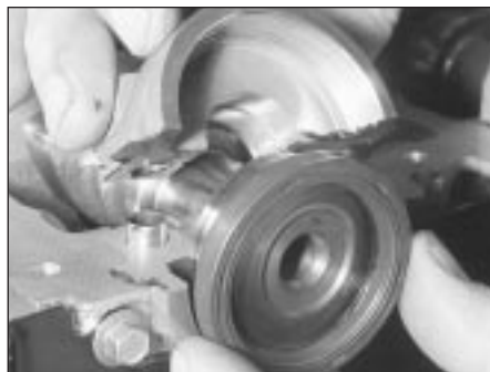
12.6 Alternatively, seal can be inserted when camshaft bearing cap is unbolted
