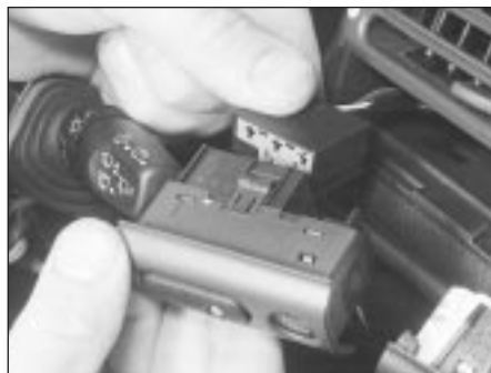
4.50 Disconnecting the multi-plug from the heated rear window switch
