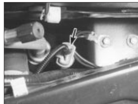
12.23 Unplug pressure-cycling switch electrical connector (arrowed)
