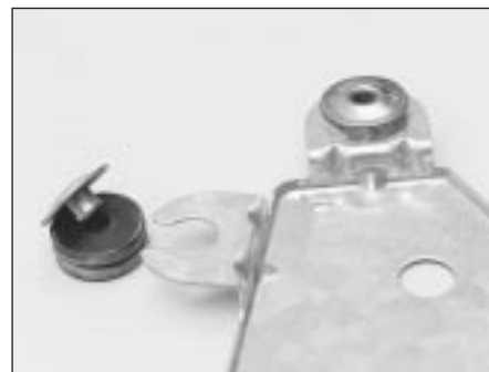
17.7B A mounting rubber removed from the mounting plate
