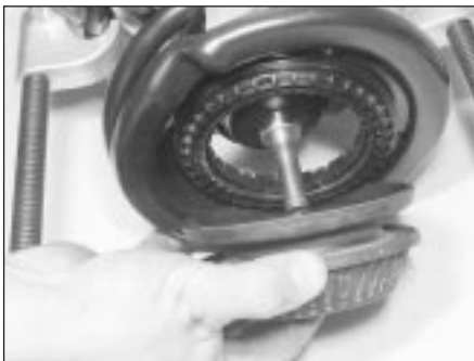
5.5B Removing the top mounting from the strut
