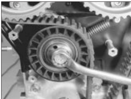
10.22 Slacken tensioner bolt to give initial belt tension
