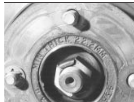
4.4B Disc minimum thickness marking
