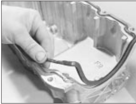
15.17 Ensure gasket is located correctly in sump groove
