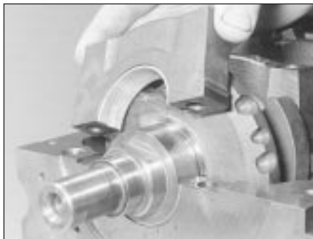
17.7 Refit the main bearing caps and tighten the bolts as specified
