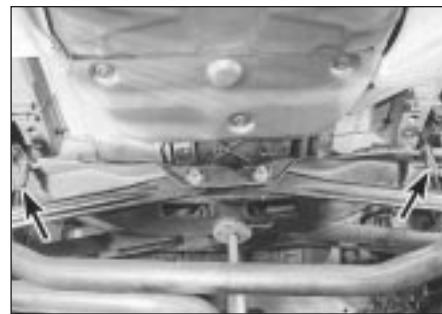
5.21 Refitting rear suspension crossmember with Ford service tools (arrowed) in place to align it with underbody ...
