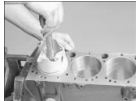
16.2 When checking piston ring end gap, the ring must be square in the cylinder bore (this is done by pushing the ring down with the top of a piston, as shown)
