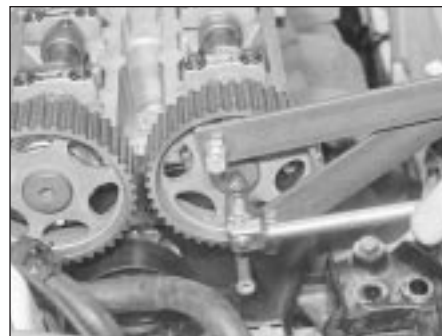
13.3 Using forked holding tool while camshaft toothed pulley bolt is slackened
