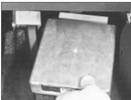
4.38 . . . then lift ECU to disengage it, and withdraw it
