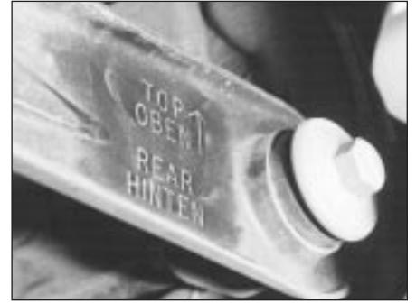
14.11 "TOP" marking on the rear lower arm
