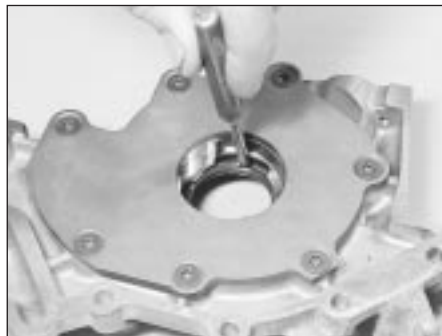
20.2 Driving out crankshaft right-hand oil seal
