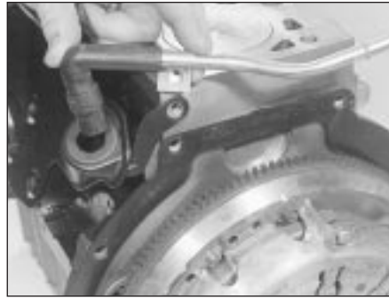
11.1B . . . crankcase breather pipe and PCV valve . . .
