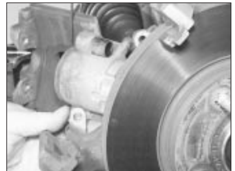
3.6 Removing the caliper carrier bracket
