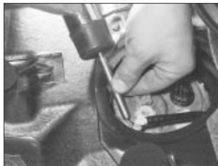
9.6 Fuel pump/fuel gauge sender unit's retaining ring can be released using ordinary tools as shown. Correct service tool will probably be required on refitting
