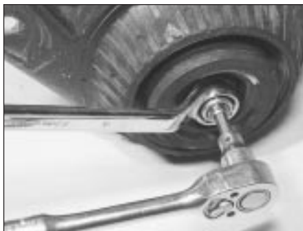
12.1A Rear strut dismantling - unscrew the upper mounting nut . . .
