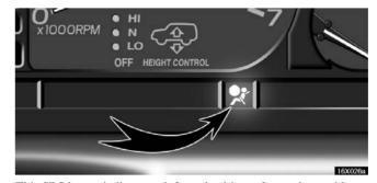
This SRS has an indicator to inform the driver of operating problems. If either of the following conditions occurs, this indicates a malfunction of the airbags and/or seat belt pretensioners. Even if the seat belt pretensioners should fail, the seat belts will operate conventionally. Contact your Lexus dealer as soon as possible to service the vehicle.
