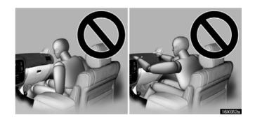
• Do not sit on the edge of the seat or lean over the dashboard when the vehicle is in use. The airbags inflate with considerable speed and force; you may be killed or seriously injured. Sit up straight and well back in the seat, and always use your seat belt.
