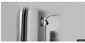
The power outlets are designed for power supply for car accessories.
