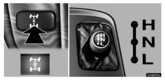
Use the four-wheel drive control lever and center differential lock button to select the following transfer and center differential modes.
