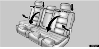
1. Lower the head restraints to the lowest position, unlock the seatback by pulling the lever on the side of the seatback and fold it down.
