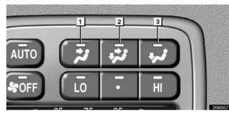
The outlets from which air is delivered can be selected manually by pressing in the appropriate air flow control button. The function of each button is as follows:
