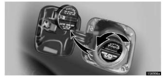
2. To remove the fuel tank cap, turn the cap slowly counterclockwise, then pause slightly before removing it. The removed cap can be stored on the back side of the fuel filler door.
