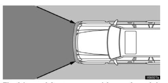
The driver and front passenger airbags and seat belt pretensioners are designed to activate in response to a severe frontal impact within the shaded area between the arrows in the illustration.
