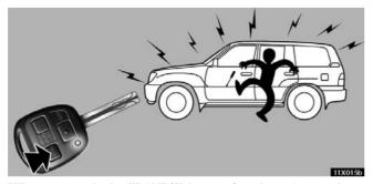
When you push the "PANIC" button for about 1 second, an alarm sounds to deter any person trying to break into or damage your vehicle.
