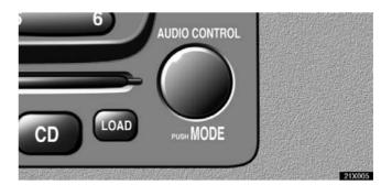
Each time you push the "AUDIO CONTROL" knob, the display changes as in the following. To adjust the tone and balance, turn the knob.
