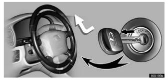
When the ignition key is removed, the steering column moves forward away from the driver and also tilts up for easy exit and entry.
