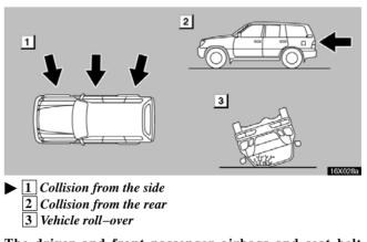
The driver and front passenger airbags and seat belt pretensioners are not designed to inflate or activate if the vehicle is subjected to a rear impact, if it rolls over, or if it is involved in a low-speed frontal collision.
