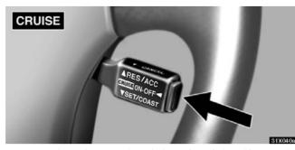
To operate the cruise control, push the main switch. This turns the system on. The indicator light in the instrument cluster shows that you can now set your desired cruising speed. Another push on the switch will turn the system completely off.
