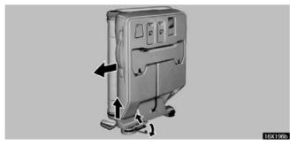
4. Remove the lever cover and pull the lock release lever. Lift up the rear side of the seat and pull the whole seat backward.
