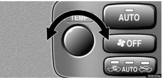
2. Turn the "TEMP" knob until the desired temperature is
