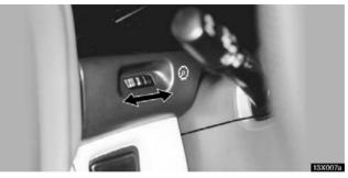
To adjust the brightness of the instrument panel lights, turn the dial.
