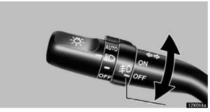
To turn on the fog lights, turn the switch to the "ON" position. The fog lights come on only when the headlights are on low beam.
