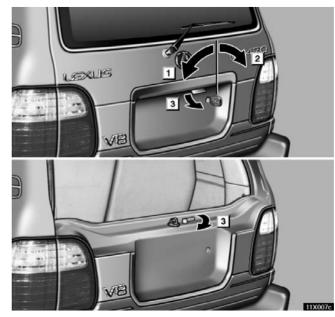
► Opening from outside 1 Unlock 2 Lock 3 Open All the doors lock and unlock simultaneously with the back door.
