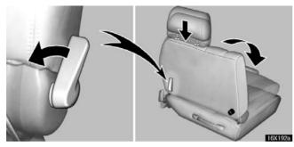
1. Lower the head restraint to the lowest position. Pull the reclining lever up and fold down the seatback.
