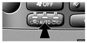
Each time you push the air intake control button, the mode changes in order from the RECIRCULATED AIR mode to AUTOMATIC mode to OUTSIDE AIR mode, then back to the RECIRCULATED AIR mode. Each indicator light shows which mode is now selected.
