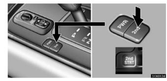
In the "2nd STRT" (second start) mode, the transmission system shifts up from second gear. Use this mode when starting your vehicle in sand, mud, ice or snow.
