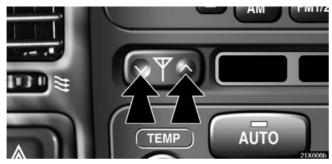
To adjust the height of the antenna manually, push the switch.
