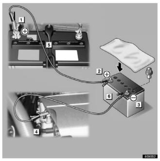
► 5 Discharged battery 6 Booster battery JUMP STARTING PROCEDURE
