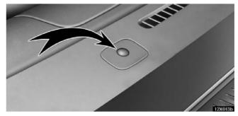
The automatic light control sensor is on top of the passenger's side instrument panel.
