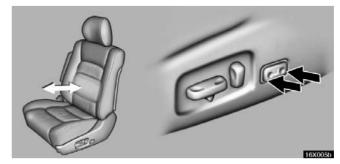
Push the control switch on either side.
