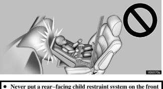
Never put a rear-facing child restraint system on the front seat because the force of the rapid inflation of the front passenger airbag can cause death or serious injury to the child.
