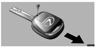
1. Remove the screw, and then the cover while pushing it in the arrow direction.
