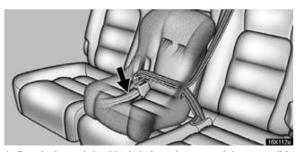
1. Run the lap and shoulder belt through or around the convertible seat following the instructions provided by its manufacturer and inserting the tab into the buckle taking care not to twist the belt. Keep the lap portion of the belt tight.
