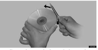
A new disc may have rough edges on its inner and outer perimeter. Remove the rough edges by pressing the side of a ball-point pen or pencil against the inner and outer edges of the disc as shown.
