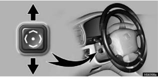
To adjust the tilt of the steering wheel, push the control switch upward or downward to set it to the desired position.
