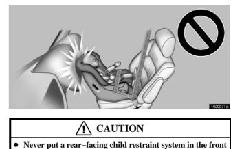
Never put a rear-facing child restraint system in the front seat because the force of the rapid inflation of the passenger airbag can cause death or serious injury to the child.
