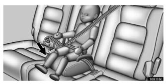
1. Sit the child on a booster seat. Run the lap and shoulder belt through or around the booster seat and child following the instructions provided by its manufacturer and insert the tab into the buckle.
