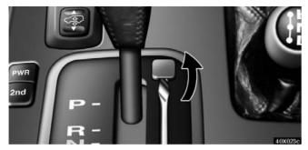
If you cannot shift the selector lever, use the shift lock override button as follows:
