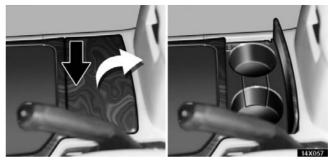
**To use the cup holder, push the cup holder lid.** You can use it as an accessory box by removing the separator inside.
