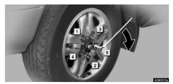
9. Lower the vehicle completely and tighten the wheel nuts.
