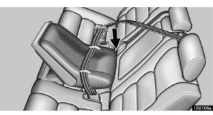
1. Run the lap and shoulder belt through or around the infant seat following the instructions provided by its manufacturer and inserting the tab into the buckle taking care not to twist the belt. Keep the lap portion of the belt tight.
