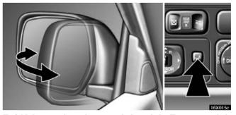
To fold the rear view mirrors, push the switch. To return to their original position, push the switch again.
