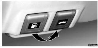
1. To open the fuel filler door, pull the lever under the instrument panel.
