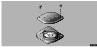
3. Remove the 2 screws to take out the lid of the module.
