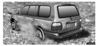
The rear differential lock system is provided for use only when wheel spinning occurs in a ditch or on a slippery or ragged surface.
