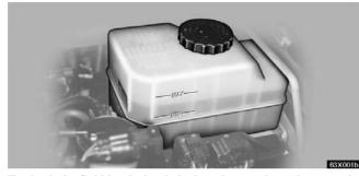
To check the fluid level, simply look at the see-through reservoir. The level should be between the "MAX" and "MIN" lines on the tank.
