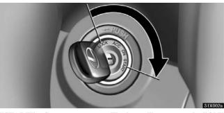
"START" – Starter motor on. The key will return to the "ON" position when released.
