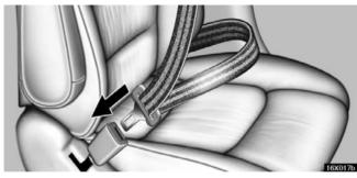
Adjust the seat as needed and sit up straight and well back in the seat. To fasten your belt, pull it out of the retractor and insert the tab into the buckle.
