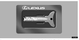
Since a transponder chip is not built in this flat key, you cannot start the engine with this key. Use this key to release the lock in case you accidentally lock your keys inside the vehicle.
