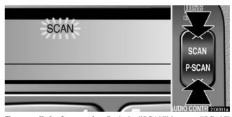
**To scan all the frequencies:** Push the "SCAN" button. "SCAN" appears on the display. The radio will find the next station up the band, stay there for a few seconds, and then scan again. To select a station, push the "SCAN" button a second time.
