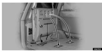
5. Remove the seat hook covers from the back of the seat cushion and install them onto the seat anchor brackets.
