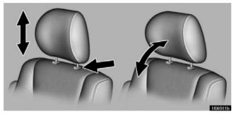
To raise the head restraint, pull it up. To lower it, press the lock release button and push the head restraint down. To move the head restraint forward or rearward, pull or push on the top.
