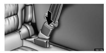
4. To remove the convertible seat, press the buckle–release button and allow the belt to retract completely. The belt will move freely again and be ready to work for an adult or older child passenger.
