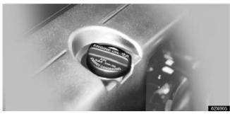
If the oil level is below or only slightly above the low line, add engine oil of the same type as already in the engine.
