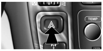
To turn on the emergency flashers, push the switch. To turn them off, push the switch again.
