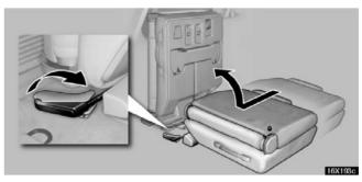
3. Slide the seat backward by pulling the lever and swing the whole seat sideways.
