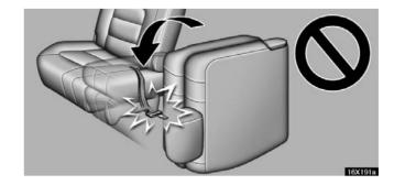
• Make sure to stow the third center seat belt in order not to cause damage on the seat belt by pinching it between the third seat inner leg and seat striker.
