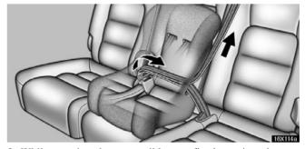
3. While pressing the convertible seat firmly against the seat cushion and seatback, let the shoulder belt retract as far as it will go to hold the convertible seat securely.
