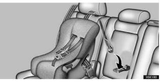
If your child restraint system requires the use of a top strap, latch the hook onto the anchor bracket and tighten the top strap.
