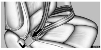
To release the belt, press the buckle release button and allow the belt to retract.
