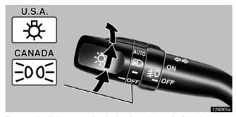
To turn the lights on, twist the knob on the end of the lever.
