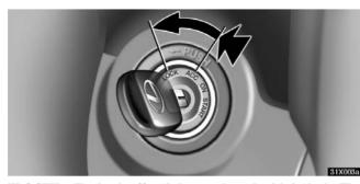
"LOCK" – Engine is off and the steering wheel is locked. The ignition key can be removed only at this position.
