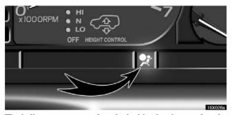
The indicator comes on when the ignition key is turned to the "ACC" or "ON" position. It goes off after about 6 seconds. This means the SRS is operating properly.
