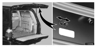
Whenever small children are in the vehicle, lock the back door so that it does not open from the inside. To do this, move the lever to the "LOCK" position as shown and then close the back door.
