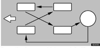
To equalize tire wear and help extend tire life, Lexus recommends that you rotate your tires approximately every 12000 km (7500 miles). However, the most appropriate timing for tire rotation may vary according to your driving habits and road surface conditions.
