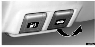
To open the hood, pull the hood lock release lever under the instrument panel. The hood will spring up slightly.
