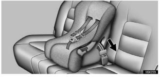
1. Run the center lap belt through or around the convertible seat following the instructions provided by its manufacturer and insert the tab into the buckle taking care not to twist the lap belt.
