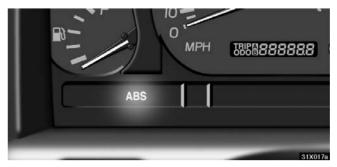
This light comes on when the ignition key is turned to the "ON" position. After about a few seconds, the light will go off.
