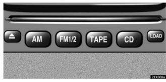
Push "AM", "FM1/2", "TAPE" or "CD" to turn on that mode. The selected mode turns on directly.
