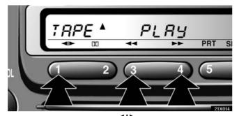
"Program" button: Push the " $\triangleleft i \triangleright$  " button to select the other side of a cassette tape. The display indicates which side is currently selected ( $\blacktriangle$  indicates top side,  $\blacktriangledown$  indicates bottom side).
