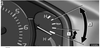
▶ 1 When the engine is warm 2 When the engine is cool
