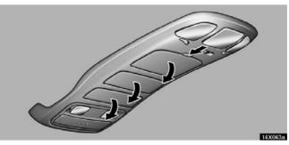
► Overhead console on the vehicle not equipped with moon roof
