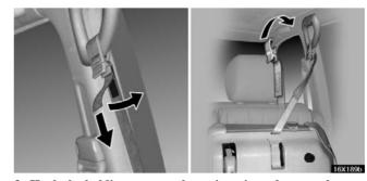
3. Hook the holding strap to the assist grip and secure the seat by pulling its free end.
