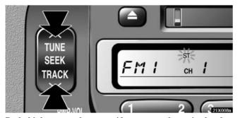
Push this button on the upper side to step up the station band or on the lower side to step down.
