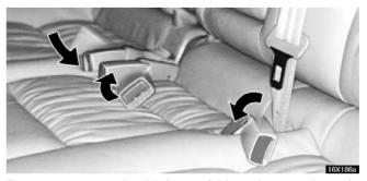
For easy access to the third seat, fold up the second seat in accordance with the following procedure.
