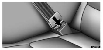
3. To remove the convertible seat, press the buckle–release button.
