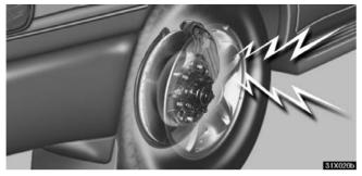
The brake pad wear limit indicators on your disc brakes give a warning noise when the brake pads are worn to the extent that replacement is required.
