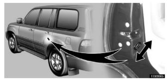
Whenever small children are in the vehicle, lock the rear door so that it does not open from the inside. To do this, move the lever to the "LOCK" position as shown on the label.
