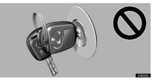
• When starting the engine, do not use the key with other transponder keys around (including keys of other vehicles) and do not press other key plates against the key grip. Otherwise the engine may not start, or may stop soon after it starts. If this happens, remove the key once and then insert it again after taking off other transponder keys (including keys of other vehicles) from the ring or while gripping or covering them with your hand to start the engine.
