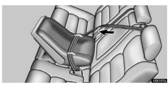
2. Fully extend the shoulder belt to put it in the lock mode. When the belt is then retracted even slightly, it cannot be extended.
