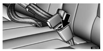
To release the belt, press the buckle release button.
