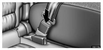
2. To remove the child restraint system, press the buckle–release button and allow the belt to retract.
