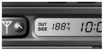
This display shows the outside temperature when the ignition switch is on.
