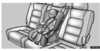
A convertible seat is used in forward-facing and rear-facing positions depending on the age and size of the child. When installing, follow the manufacturer's instructions about the appropriate age and size of the child as well as direction for installing of a child restraint system.
