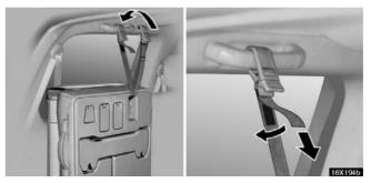
4. Hook the holding strap to the assist grip and secure the seat by pulling its free end.
