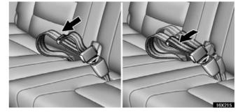
Remove excess length of the belt and adjust the belt position.
