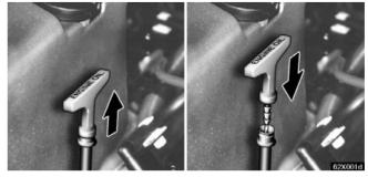
With the engine at operating temperature and turned off, check the oil level on the dipstick.
