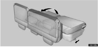
2. Pull the lever under the seat cushion and swing the whole seat forward.
