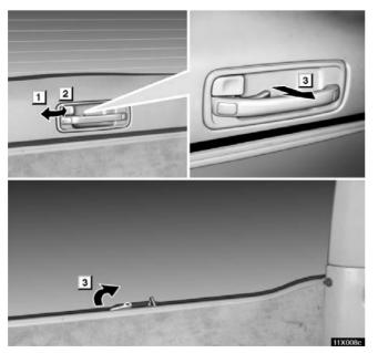
► Opening from inside 1 Unlock 2 Lock 3 Open The back door can be opened as shown.
