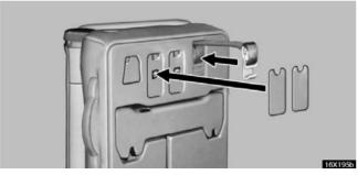
When returning the third seat to its original position, stow the holding strap and the seat hook covers into the holder facing the direction shown in the illustration.
