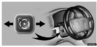
To adjust the steering column length, push the control switch forward or backward to set the steering wheel to the desired position.
