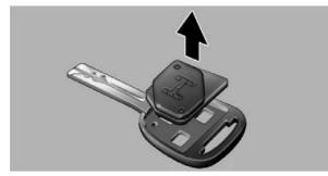
2. Remove the module from the key frame.
