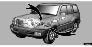
Three–way catalytic converters are emission control devices installed in the exhaust system.
