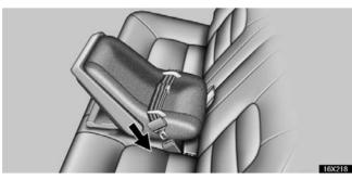
1. Run the center lap belt through or around the infant seat following the instructions provided by its manufacturer and insert the tab into the buckle taking care not to twist the lap belt.
