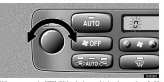
When you turn the "TEMP" knob, the sensitivity changes from "+3" down to "-3". If you do not operate any button for a few seconds or if you push the button other than the air intake control button and temperature control knob, the previous display returns.
