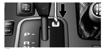
**2** Insert your finger, the screwdriver or equivalent into the hole to push down the shift lock override button. You can shift the selector lever while pushing the button.
