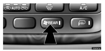
To turn on the rear air conditioning when you sit on the front seat, push this switch. The rear air conditioning operates in the automatic mode. To adjust the air flow and setting temperature, follow the steps in accordance with "Rear air conditioning controls" on page 143.
