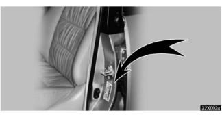
The vehicle identification number (VIN) is also on the Certification Label.
