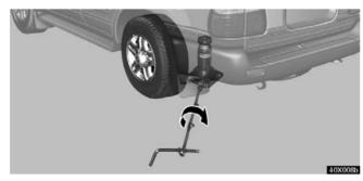
6. After making sure no one is in the vehicle, raise it high enough so that the spare tire can be installed.
