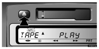
When you insert a cassette tape, the exposed tape should be to the right.
