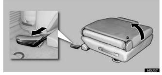
2. Pull the inner-lock lever and lift the whole seat.
