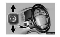
To tilt the steering wheel up or down to the desired angle, push the control switch in the required direction and release the button when the steering wheel reaches the desired angle.
