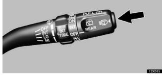
To spray fluid on the headlights, push the switch with the headlights on.
