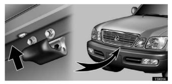
Insert your fingers under the hood, push up the auxiliary catch lever and lift the hood.
