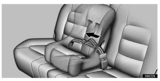
2. While pressing the convertible seat firmly against the seat cushion and seatback, tighten the lap belt by pulling its free end to hold the convertible seat securely.
