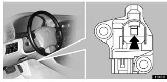
The fuel pump shut–off system activates when the impact detection sensor located in the footwell of the driver's seat detects an impact larger than specified.
