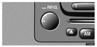
Push this knob to turn the audio system on and off. Turn this knob to adjust the volume.
