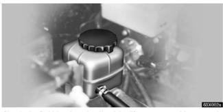
Check the fluid level on the dipstick. If necessary, add automatic transmission fluid DEXRON  $^{\textcircled{B}}$  II or III.
