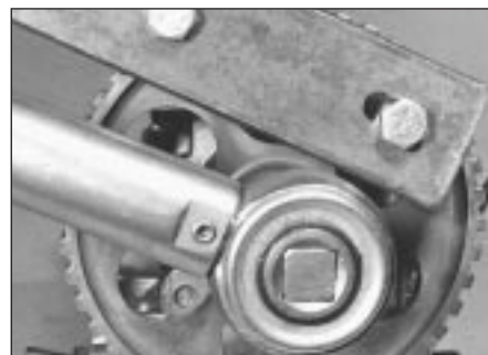
35.5 Method of tightening camshaft sprocket bolt
