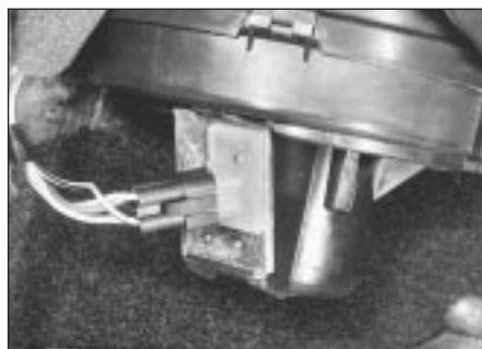
9.3 Blower unit and wiring connection
