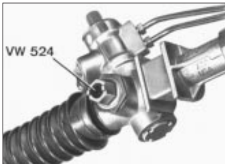
16.8 Power steering gear adjustment – use VW tool
