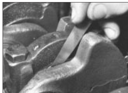
15.3 Checking crankshaft endfloat at No. 3 main bearing
