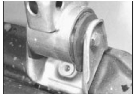
5.26a Undo front mounting through-bolt
