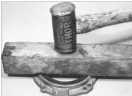
14.16 Installing new crankshaft rear oil seal
