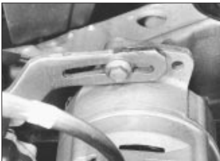
13.4a Alternator drivebelt tensioner link - 1.3 litre
