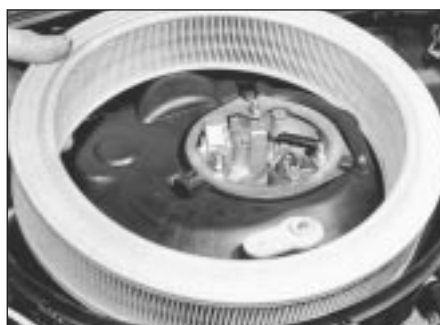
32.2 . . . and remove the element - 1.3 litre, carburettor
