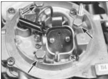
13.8 Carburettor securing bolts (arrowed) - Pierburg/Solex 2E3
