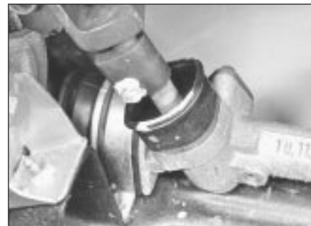
17.6 Steering gear pinion-to-lower column joint
