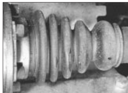
24.2 Inspect condition of each CV joint boot
