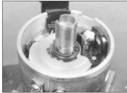
7.7 Hall sender unit, retaining ring and washers
