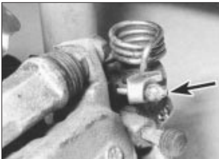
2.15 Release handbrake cable (arrowed) from caliper
