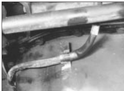
15.1 Alternator wire clip on sump
