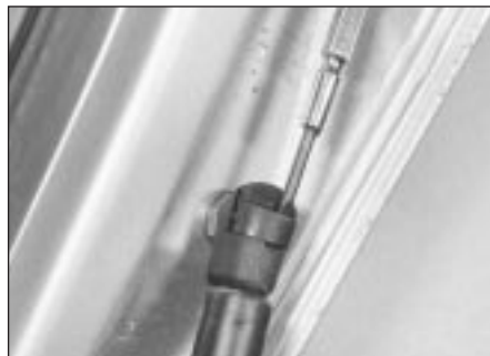
9.2a Releasing tailgate strut balljoint clip
