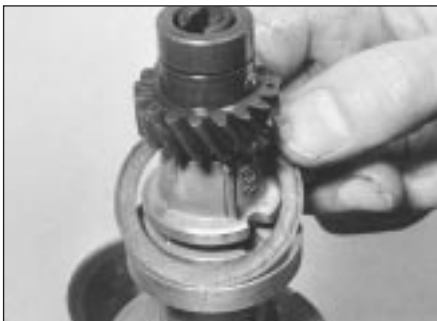
6.6b The gasket must be removed
