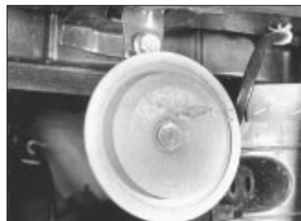
24.1a Single horn location behind front grille
