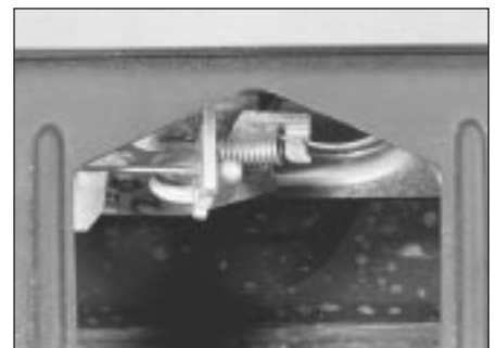
7.4 Bonnet release cable-to-lock attachment
