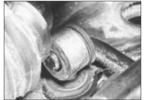
4.5 Anti-roll bar location in eye bolt
