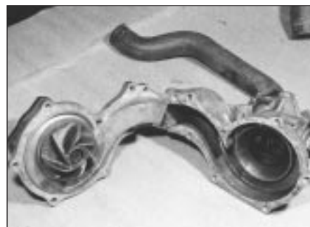
6.17 Two halves of coolant pump - 1.6 and 1.8 litre
