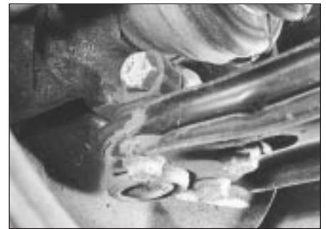
7.3 Track control arm balljoint and clamp bolt
