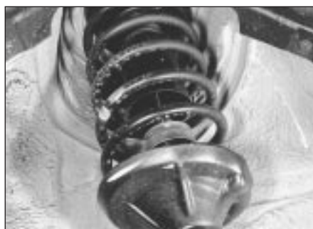
29.4 Check shock absorbers for leakage
