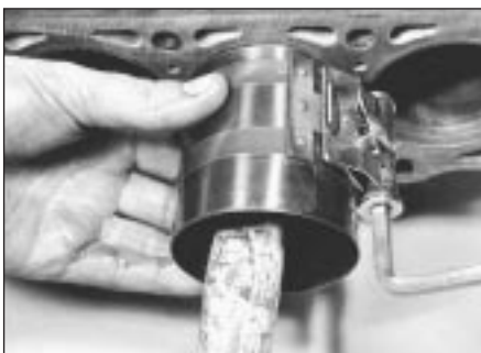
30.4 Using a piston ring compressor
