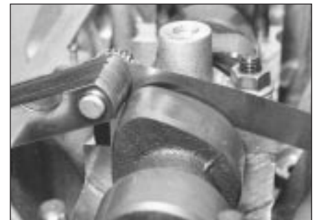
8.6 Measuring camshaft endfloat
