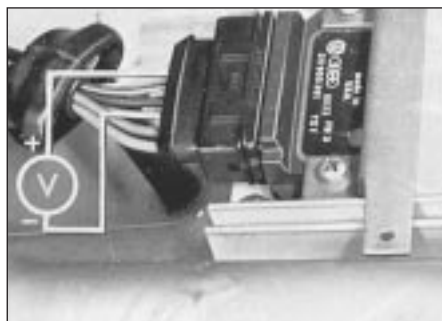
5.4 Voltmeter connection when testing Hall sender
