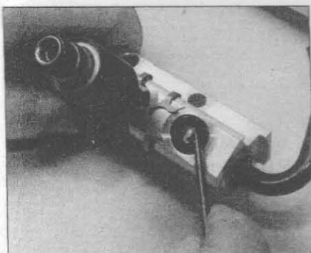
13.35a Remove the injector seal from the fuel rail. The injector seals that are positioned in the fuel rail are black - the seals that go into the manifold are brown (conventional style injectors)
