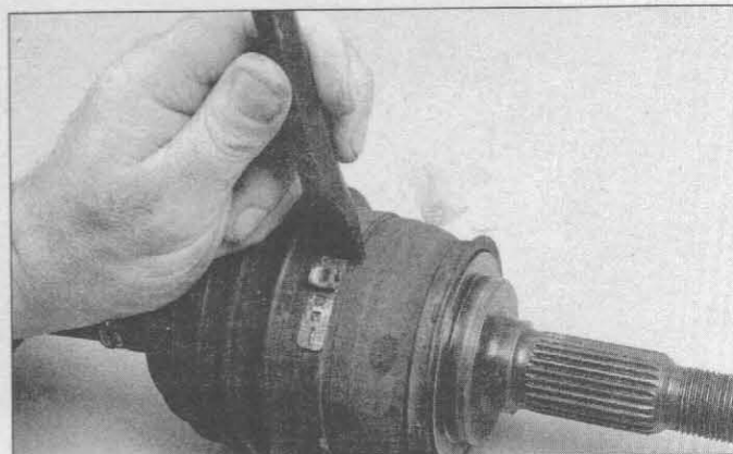
11.4a Cut off the band retaining the boot to the shaft, then slide the boot toward the center of the shaft
