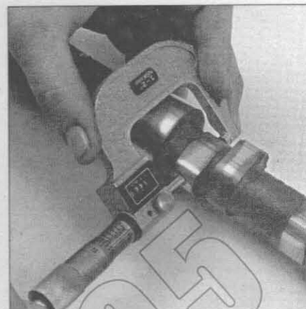
13.9 Measure the lobe heights on each camshaft - if any lobe height is less than the specified allowable minimum, replace that camshaft
