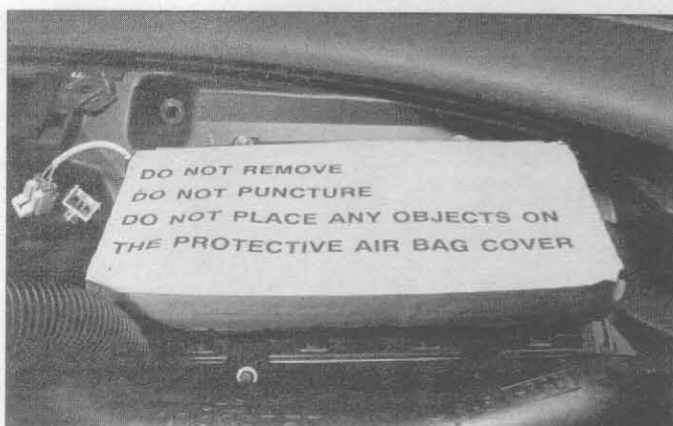
25.2 The passenger's side airbag is located on top of the dash, right above the glovebox (instrument panel trim pad removed); notice that the big yellow connector, known as the Connector Position Assurance (CPA) connector, has been unplugged to ensure that the passenger's airbag isn't accidentally deployed while you're working in that area
