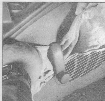
15.5b If you don't have a window regulator handle removal tool, work a clean shop rag up between the handle and the door trim panel from underneath as shown and pull up on the rag to pop the handle retaining clip loose, then remove the handle
