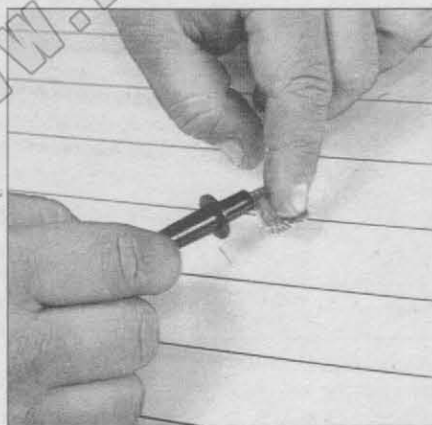
13.4 When measuring the voltage at the rear window defogger grid, wrap a piece of aluminum foil around the positive probe of the voltmeter and press the foil against the wire with your finger
