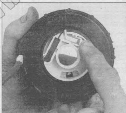
25.16 To center the SIR coil, hold it with its underside facing up, depress the spring lock and rotate the hub in the direction of the arrow on the coil assembly until it stops
