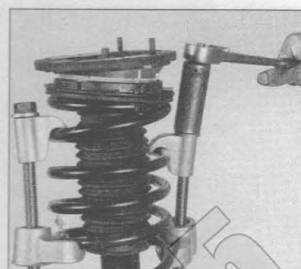
4.4 Following the tool manufacturer's instructions, install the spring compressor on the spring and compress it sufficiently to relieve all pressure from the upper spring seat
