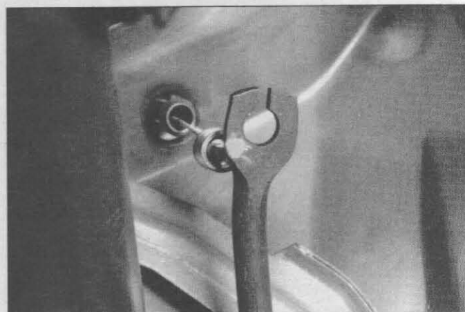
10.2 Slide the accelerator cable through the slot in the pedal arm
