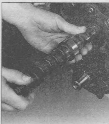
13.15 Support the camshaft near the block to avoid damaging the bearings
