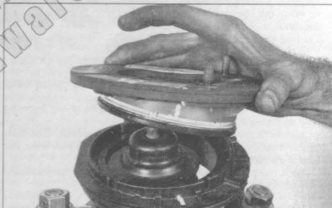
4.6b ... and the strut mount; inspect the bearing in the mount for smooth operation and the rubber portion of the mount for cracking and general deterioration, if the bearing doesn't turn smoothly, or if there's any separation of the rubber, replace the mount
