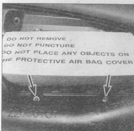
24.8c To detach the upper right part of the instrument panel, remove these two screws (arrows)
