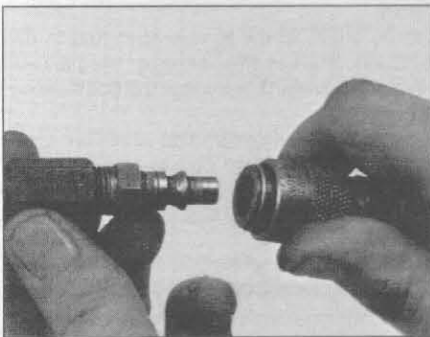
10.5 This is what the air hose adapter that threads into the spark plug hole looks like - they're commonly available from auto parts stores
