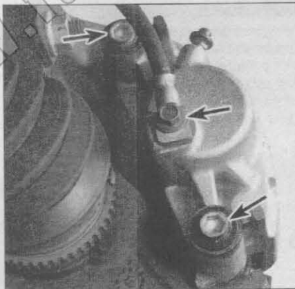
3.4b To detach the front caliper from the steering knuckle, remove these two bolts (upper and lower arrows); don't remove the banjo bolt (center arrow) for the brake hose unless you intend to overhaul the caliper
