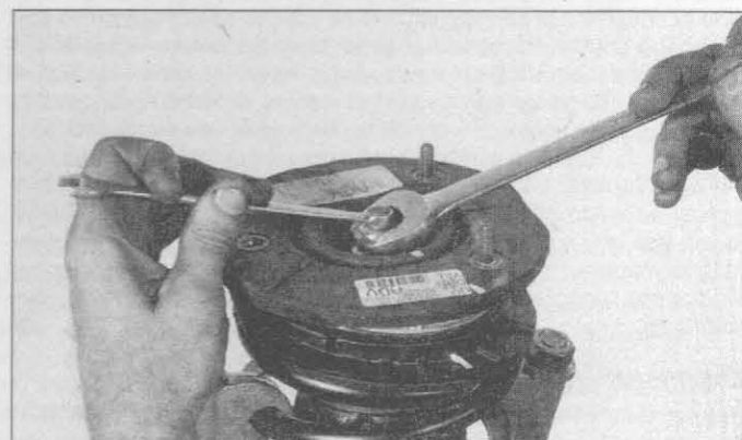
4.16 Hold the damper shaft from turning, then tighten the nut securely (unless you have a special socket with a "window" in it for the back-up wrench, you won't be able to torque the nut until the strut assembly is installed in the vehicle and the vehicle is on the ground)
