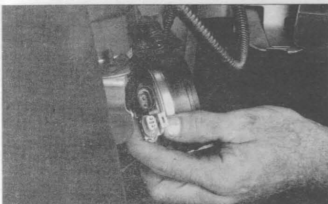
21.2 To test the horn, connect the horn to the battery with fused jumper wires; if the horn doesn't operate, replace it
