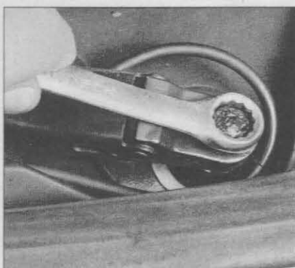
20.3 Gently pry off the trim cap and check the tightness of the wiper arm retaining nut
