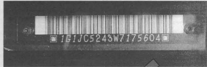
The Vehicle Identification Number (VIN) is stamped into a metal plate fastened to the dashboard on the driver's side - it's visible through the windshield
