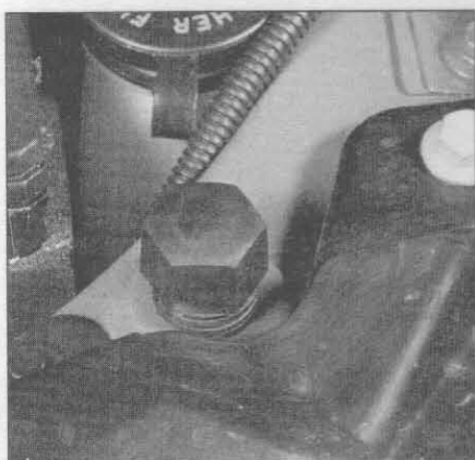
9.11 Screw the hood bumpers in or out to adjust the hood flush with the fenders (left bumper shown, right bumper identical)
