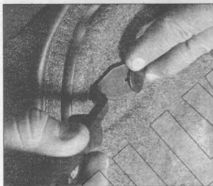
17.10a To gain access to the rear brake, taillight, turn signal and side marker light bulbs, release this push-in retainer and peel back the trunk liner ...
