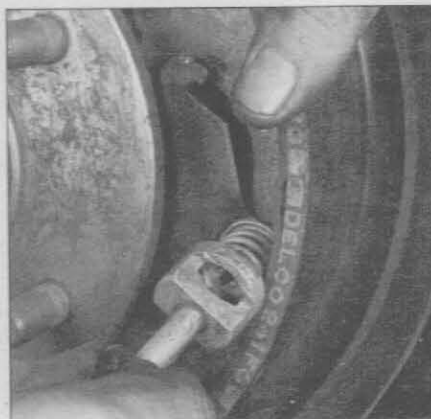
6.4c Remove the hold-down springs and pins by pushing the retainer in with and turning it 90-degrees - the tool shown here is available at most auto parts stores
