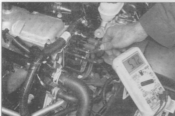
6.7a Check the secondary coil resistance across the towers on each coil pack (2.2L engine)
