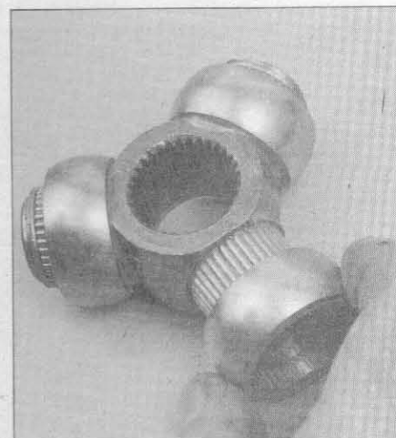
11.3k Clean all of the old grease out of the housing and spider assembly, then remove each bearing, one at time
