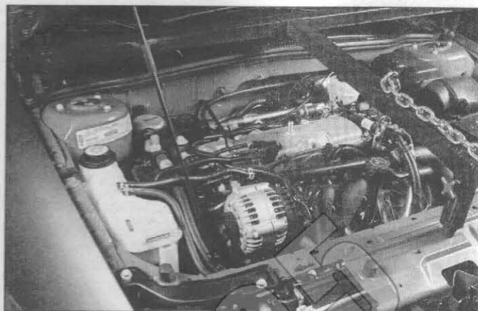
5.2 During transmission removal, support the engine with a support fixture designed for this purpose. They are often available from rental yards
