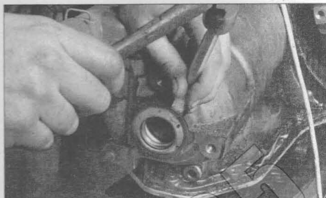
8.5 Dislodge metal-type driveaxle oil seals by working around the outer circumference with a chisel and hammer (transaxle removed for clarity)
