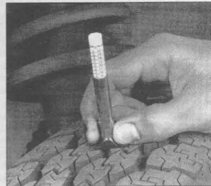
5.2 Use a tire tread depth gauge to monitor tire wear - they are available at auto parts stores and service stations and cost very little
