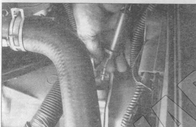
5.6 Pull up on the TV cable until the end of the cable is visible, then disengage it from the transaxle link
