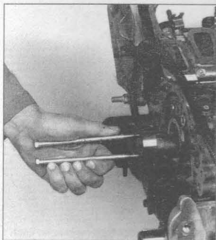
13.14 Thread long bolts into the sprocket bolt holes to use as a handle when removing and installing the camshaft
