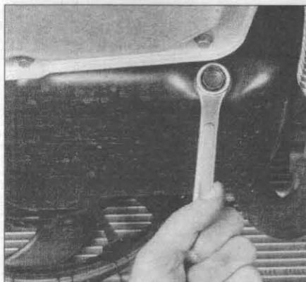
9.7 The engine oil drain plug is located at the rear of the oil pan - it is usually very tight, so use a box-end wrench to avoid rounding off the hex
