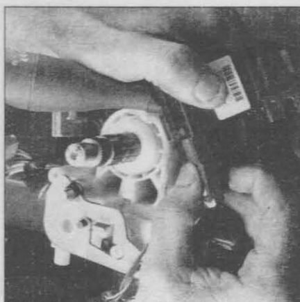
9.6 Detach the windshield wiper/washer switch from the steering column housing assembly and unplug the electrical connector
