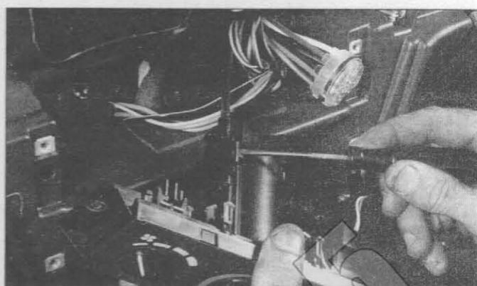
12.3f Use a small screwdriver to pry apart the clips that retain the air conditioner control cable (if equipped)
