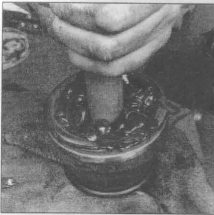
11.4q Apply grease through the splined hole, then insert a wooden dowel (with a diameter slightly less than that of the axle) through the splined hole and push down - the dowel will force the grease into the joint - repeat until the bearing is completely packed
