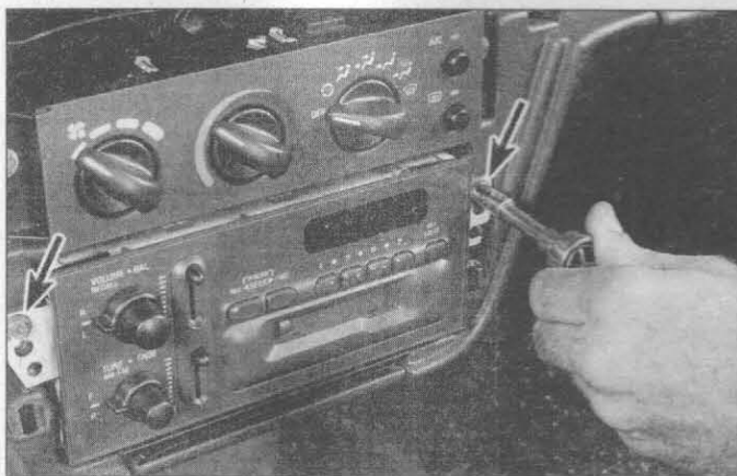
11.3 To detach the radio from the dash, remove these two screws (arrows)
