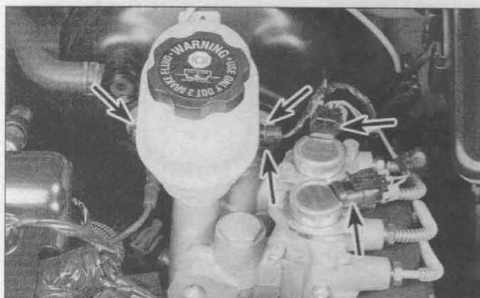
8.3 Unplug the electrical connectors for the fluid level warning switch (center arrow) and the ABS solenoids (two right arrows); to detach the master cylinder from the power brake booster, remove the two mounting nuts (upper arrows) (1995 through 1999)
