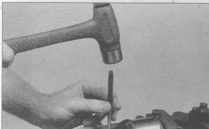
15.4a Use a center-punch or number stamping dies to mark the main bearing caps to ensure installation in their original locations on the block (make the punch marks near one of the bolt heads)
