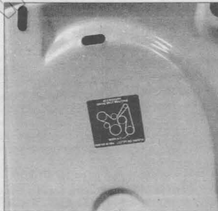
14.7 The serpentine drivebelt routing diagram is located on the radiator shroud (later model diagram shown)
