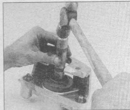
4.19 Use a hammer and seal driver to seat the boot in the caliper
