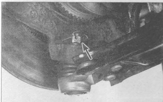
5.3 Remove the cotter pin and loosen - but don't remove - the nut (arrow) from the balljoint stud
