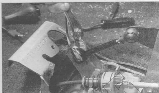
3.5b ... squeeze the locking tangs together, then disengage the cable from the bracket
