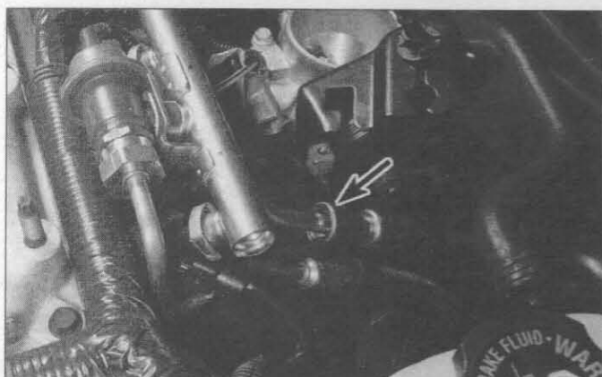
13.29 Use a special fuel line disconnect tool to detach the fuel feed line from the fuel rail
