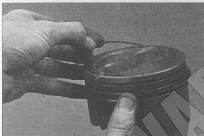
23.9a Installing the spacer/expander in the oil control ring groove
