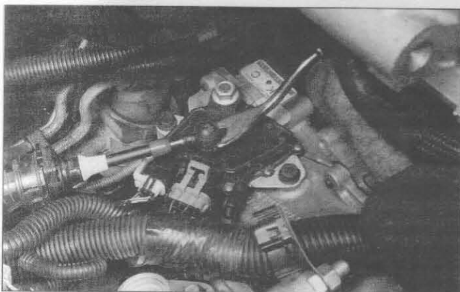
3.2 To disconnect the shift cable from the transaxle manual lever, pry it off the pin on the lever with a prying tool or screwdriver
