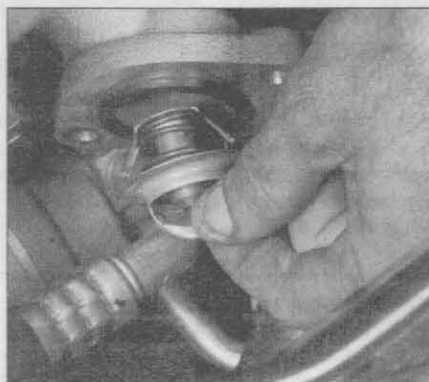
3.9 Note how it's installed, then remove the thermostat (the spring end points toward the engine)
