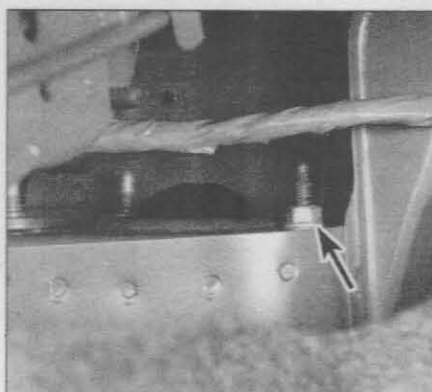
9.2 Remove this single nut (arrow) from the trunk space (the other two bolts, the threads of which are visible in this photo, are removed from underneath after the vehicle is raised)
