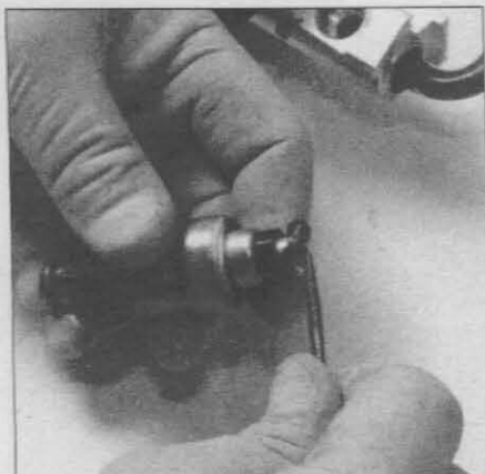
13.35b Carefully pry the seals off the injectors
