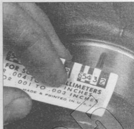
24.15 Measuring the width of the crushed Plastigage to determine the main bearing oil clearance (be sure to use the correct scale - standard and metric ones are included)
