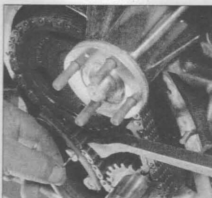
12.14 Press the tensioner in and insert an appropriate size drill bit through the hole to retain the tensioner in the retracted position
