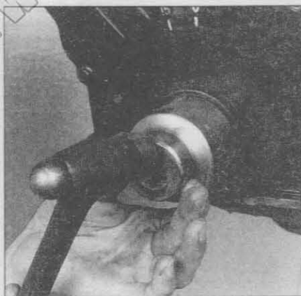
6.9 Install the new seal with a large socket or section of pipe
