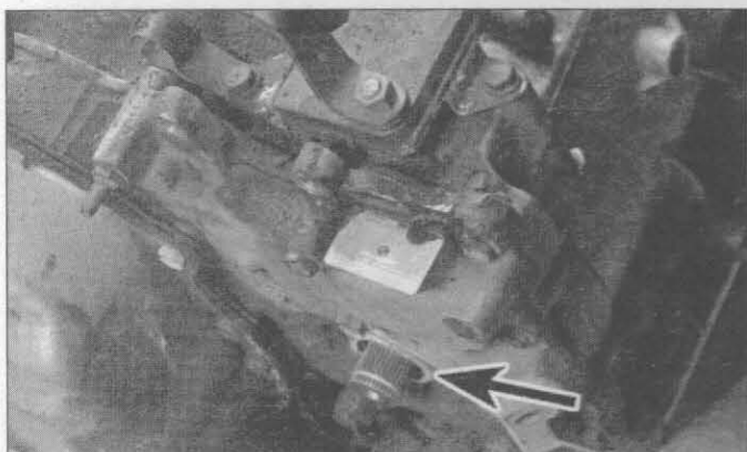
8.4 Rubber-type driveaxle oil seals (arrow) can be pried out of the transaxle housing with a screwdriver; be careful not to damage the splines of the axleshaft (transaxle removed for clarity)
