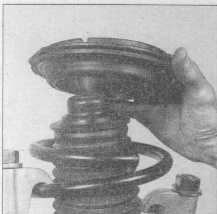
4.7 Remove the upper spring seat and insulator from the damper shaft; inspect the insulator for cracking and hardness and, if necessary, replace it
