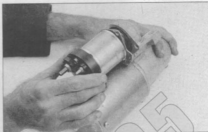
14.5 To remove the solenoid housing from the starter motor, remove the screws and turn it clockwise
