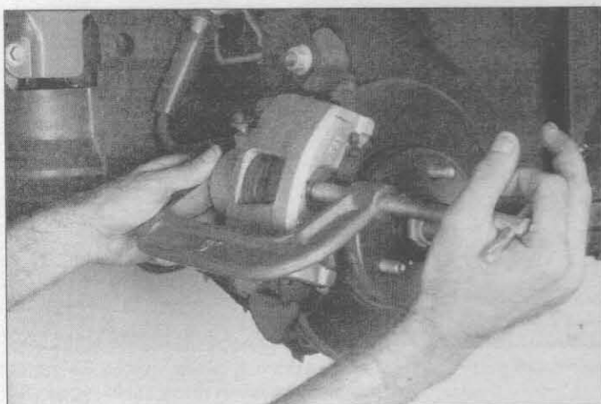
3.3 Depress the piston into the caliper with a large C-clamp
