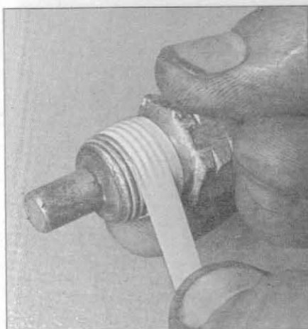
5.1 To prevent coolant leakage, be sure to wrap the temperature sensor threads with Teflon tape before installation
