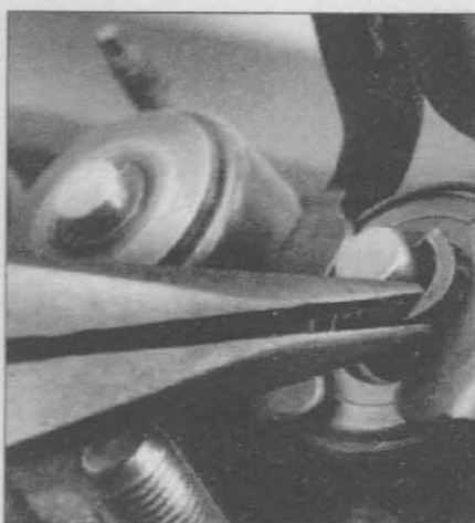
9.3 Use a valve spring compressor to compress the spring, then remove the keepers from the valve stem
