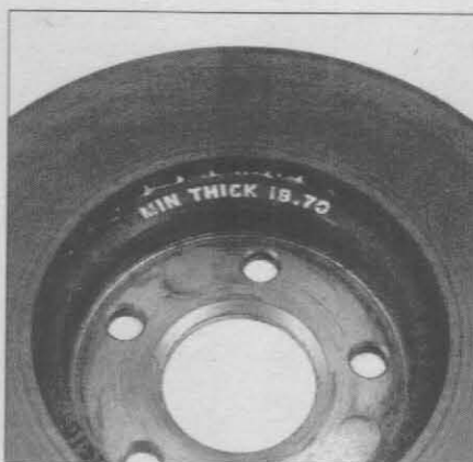
5.6a The minimum allowable thickness of the disc is cast into the hub area
