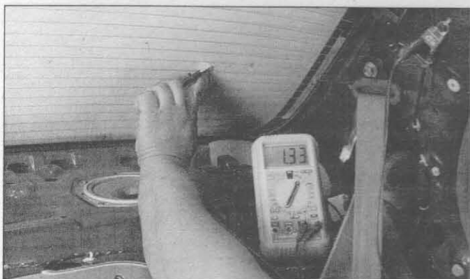
13.7 To find the break, place the voltmeter negative lead against the defogger ground terminal, place the voltmeter positive lead with the foil strip against the heating element at the positive terminal end and slide it toward the negative terminal end - the point at which the voltmeter reading changes abruptly is the point at which the element is broken
