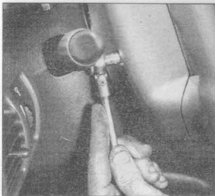
12.3 Remove the airbag module retaining screws (the other screw is in the same location on the other side of the steering column)
