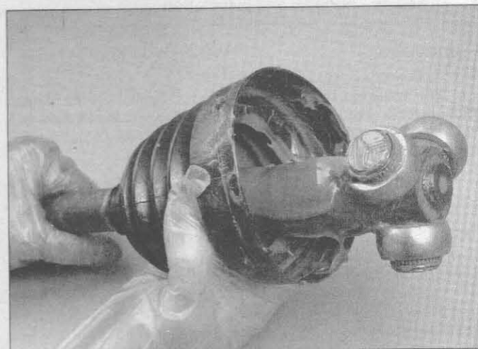
11.3d Slide the boot towards the center of the driveaxle
