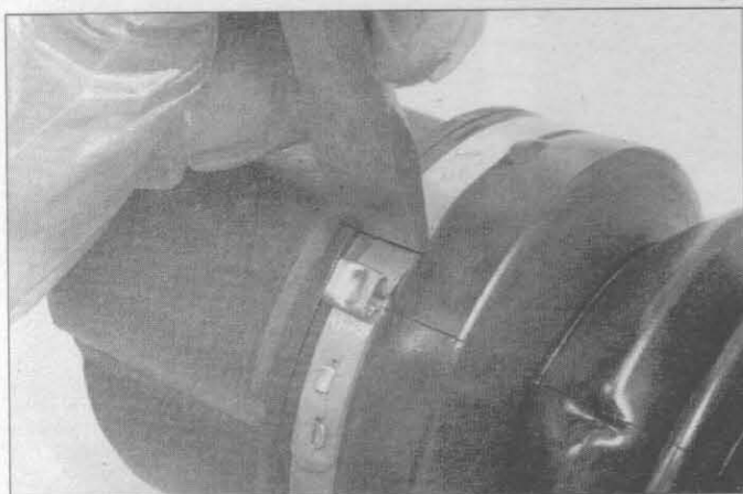
11.3a Cut off the boot seal retaining clamps, using wire cutters or a chisel and hammer
