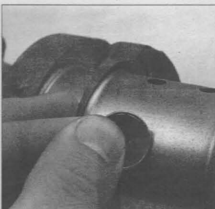
20.3 Rubbing a penny lengthwise on each journal will reveal its condition - if copper rubs off and is embedded in the crankshaft, the journals should be reground
