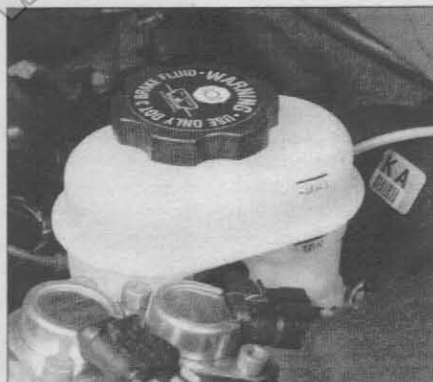
4.18 The fluid level inside the brake fluid reservoir can easily be checked by observing the level from the outside - fluid can be added to the reservoir after the cover is removed by prying up on the tabs
