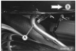
Prepare a rubber hose of the inside diameter 7.3 ~ 7.5 mm (0.29 ~ 0.30 in.) [e.g. Part No. 92191-1264] × L 100 mm (3.9 in.) and make a plug hose [A] with one end tied with a wire [B].
