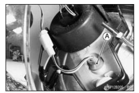
• Remove the wedge-base type bulb [A], pull the bulb straight out of the socket [B].
