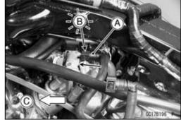
Push and pull [A] the fuel hose joint #2 [B] back and forth more than two times and make sure it is locked and doesn't come off. When the fuel hose joint #2 is correctly installed, it should slide on the delivery pipe about 5 mm (0.2 in.).
