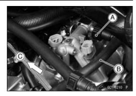
Unscrew the inlet manifold bolts [A].
