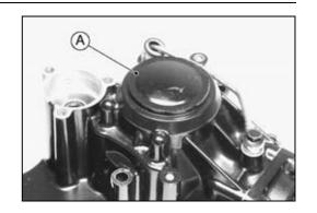
OPry open the drive gear nut [A] with a small chisel. OInstall:
