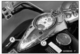
Disconnect the meter [A] and ignition switch [B] connectors.
