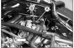
Push and pull [A] the fuel hose joint #2 [B] back and forth more than two times and make sure it is locked and doesn't come off. When the fuel hose joint #2 is correctly installed, it should slide on the delivery pipe about 5 mm (0.2 in.).
