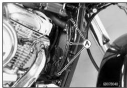
Remove: Radiator Fan Motor Connector [A] Radiator Hoses
