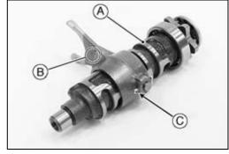
• Disassemble the shift drum assy as shown.
