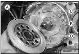
• Pull the needle bearing [A], sleeve [B], and thrust washer [C] off the drive shaft.
