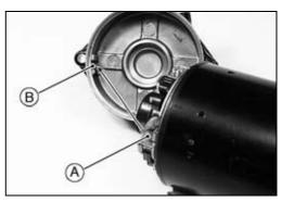
Apply a thin coat of grease to the oil seal [B] in the right end cover [A].
