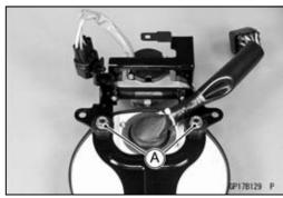
• Pull out the meter unit [A] from the pins [B] on the bracket.
