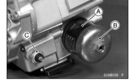
• Remove the right crankcase bolts.  $\phi$ 8 mm Bolts (5) [A] OBe sure to remove this bolt [B]
