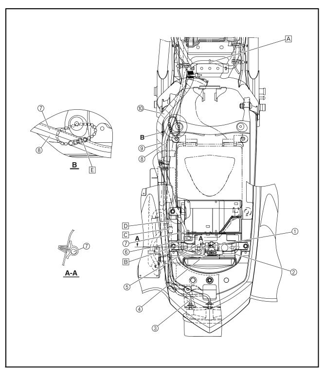
E Fasten the coolant reservoir hose and the cylinder head breather hose to the frame with the plastic beaded tie at its loosest position so that the hoses are not pinched.
