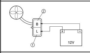
Does the radiator fan motor turn?
