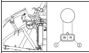
Measure the pickup coil resistance.
