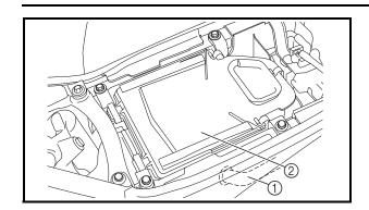
3. Disconnect the air filter case breather hose ①, and then remove the air filter case ② with the air intake duct.
