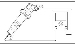
Measure the secondary coil resistance.
