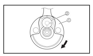
a. The crankshaft ① and the crankshaft pin ② oil passages must be properly interconnected with a tolerance of less than 1 mm (0.04 in).
