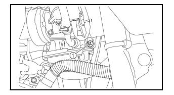
2. Loosen the clamp screw ①, and then disconnect the air intake duct.
