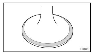
a. Apply a coarse lapping compound to the valve face.
