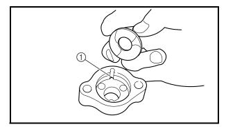
5. Mesh the bearing race tab ① with parking brake case slit.
