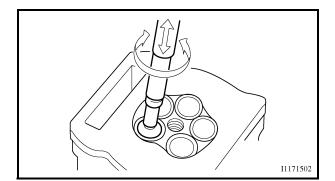
e. Apply a fine lapping compound to the valve face and repeat the above steps.
