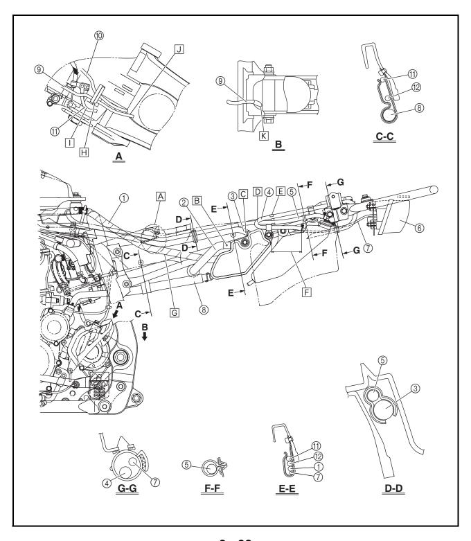
K Route the carburetor drain hose between the frame and connecting arm and let it hang freely under the vehicle.
