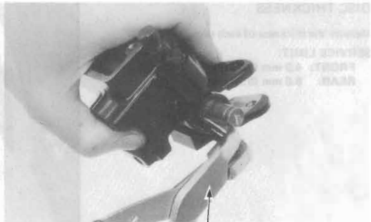
SNAP RING PLIERS or EQUIVALENT IN U.S.A. 07914-3230001
