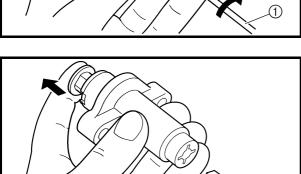
a. Lightly press the timing chain tensioner rod into the timing chain tensioner housing by hand.
