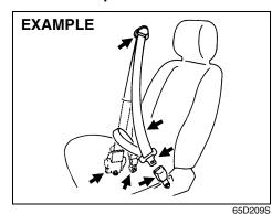
Periodically inspect the seat belts to make sure they work properly and are not damaged. Check the webbing, buckles, latch plates, retractors, anchorages and guide loops. Replace any seat belts which do not work properly or are damaged.
