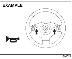
Press the horn pad on the steering wheel to sound the horn. The horn will sound with the ignition switch in any position.
