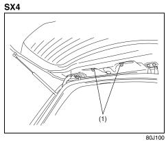
To remove a high-mounted stop light hous-ing the following procedure:
