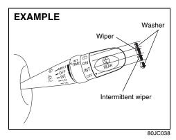
To turn the rear wiper on, twist the rear wiper switch on the end of the lever forward to the "ON" position. If your vehicle is equipped the "INT" position, the rear wiper operates intermittently when you twist the switch forward to the "INT" position. To turn the rear wiper off, twist the switch rearward to the "OFF" position.
