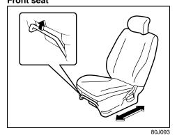
The adjustment lever for each front seat is located under the front of the seat. To adjust the seat position, pull up on the adjustment lever and slide the seat forward or rearward. After adjustment, try to move the seat forward and rearward to ensure that it is securely latched.
