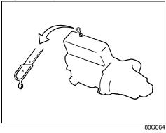
It is important to keep the engine oil at the correct level for proper lubrication of your vehicle's engine. Check the oil level with the vehicle on a level surface. The oil level indication may be inaccurate if the vehicle is on a slope. The oil level should be checked either before starting the engine or at least 5 minutes after stopping the engine.
