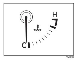
When the ignition switch is in the "ON" position, this gauge indicates the engine coolant temperature. Under normal driving conditions, the indicator should stay within the normal, acceptable temperature range between "H" and "C". If the indicator approaches "H", overheating is indicated. Follow the instructions for engine overheating in the "EMERGENCY SERVICE" section.
