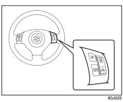
The cruise control system allows you to maintain a steady speed without keeping your foot on the accelerator pedal. The controls for operating the cruise control system are on the steering wheel. You can use the cruise control system at speeds of about 40 km/h (25 mph) or higher.
