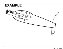
To turn the lights on or off, twist the knob on the end of the lever. There are three positions: in the "OFF" position all lights are off; in the middle position the front parking lights, taillights, license plate light, and instrument lights are on, but the headlights are off; in the third position the headlights come on in addition to the other lights.
