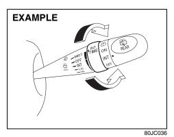
If the lever is equipped with the "INT TIME" control, turn the control forward or rearward to adjust the intermittent wiper operation to the desired interval.
