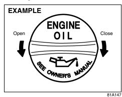
Remove the oil filler cap and pour oil slowly through the filler hole to bring the oil level to the upper limit on the dipstick. Be careful not to overfill. Too much oil is almost as bad as too little oil. After refilling, start the engine and allow it to idle for about a minute. Stop the engine, wait about 5 minutes and check the oil level again.
