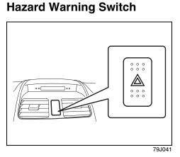
Push in the hazard warning switch to activate the hazard warning lights. All four turn signal lights and both turn signal indicators will flash simultaneously. To turn off the lights, push the switch again.
