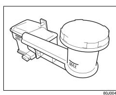
Check the clutch pedal for smooth operation and clutch fluid level from time to time. If clutch dragging is felt with the pedal fully depressed, have the clutch inspected by your SUZUKI dealer. If the clutch fluid level is near the "MIN" line, fill it up to the "MAX" line with DOT3 brake fluid.
