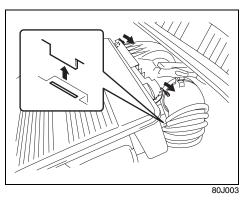
If the air cleaner is clogged with dust, there will be greater intake resistance, resulting in decreased power output and increased fuel consumption.
