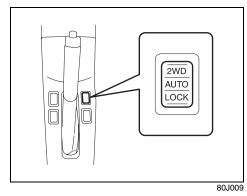
This i-AWD system enables you to select the driving mode according to the driving conditions by operating the 2WD/i-AWD switch. With this feature, you can select 3 mode positions, "2WD", "i-AWD AUTO" and "i-AWD LOCK" by operating the 2WD/ i-AWD switch even when the vehicle is moving, provided the front wheels are in the straight ahead position.
