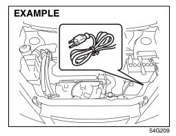
The engine block heater will help you start the engine more easily in very cold weather ( $-18^{\circ}C$  (0°F) or below). To use the engine block heater:
