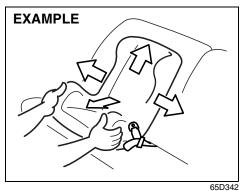
5) Make sure the child restraint is securely fastened by trying to move the child restraint system in all directions, especially forward.
