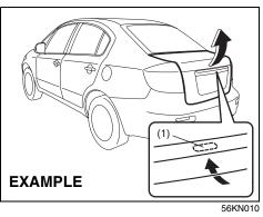
If your vehicle is equipped with a trunk lid unlatch switch (1), push and hold the trunk lid unlatch switch (1) and lift the trunk lid to open the trunk lid.
