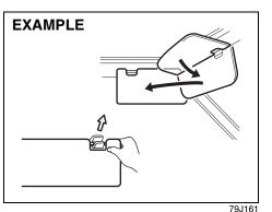
The sun visors can be pulled down to block glare coming through the windshield, or they can be unhooked and turned to the side to block glare coming through the side window.
