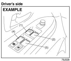
The power windows can only be operated when the ignition switch is in the "ON" position.
