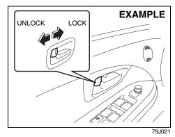
To lock a door from inside the vehicle, turn the lock knob forward. Turn the lock knob rearward to unlock the door.
