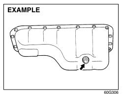
Drain the engine oil while the engine is still warm.
