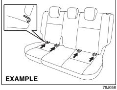
Your vehicle is equipped with lower anchors for securing up to one or two standard LATCH-type child restraint(s) in the second row seats. (LATCH stands for Lower Anchors and Tethers for Children.) The anchors are located where the rear of the seat cushion meets the bottom of the seatback.
