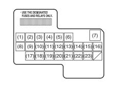
15A Rear wiper (1) (2) 15A Ignition coil 10A Back-up light (3) (4) 10A Meter (5) 15A Accessory (6) 15A Accessory 2 (7)30A Power window 30A Wiper (8) IG1 SIG 10A (9) (10)15A Air bag (11)10A Anti-lock brake system 4WD 15A (12)(13)15A Stop light (14)20A Door lock \_ (15) Blank ST SIG (16) 10A (17)15A Seat heater IG 2 SIG (18)10A (19) 10A Tail light (20)15A Dome
