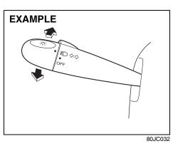
With the headlights on, push the lever forward to switch to the high beams (main beams) or pull the lever toward you to switch to the low beams. When the high beams (main beams) are on, a light on the instrument panel will come on. To momentarily activate the high beams (main beams) as a passing signal, pull the lever slightly toward you and release it when you have completed the signal.
