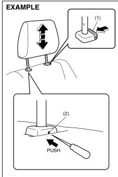
To raise the head restraint, pull upward on
