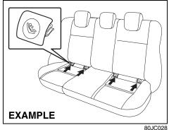
For SX4 SEDAN, the covers marked with the child restraint symbol as shown in the illustration indicate the presence of lower anchors. Remove the covers before installing the child restraint system. Cover the lower anchors when not in use.
