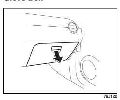
To open the glove box, pull the latch lever. To close it, push the lid until it latches securely.
