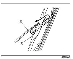
2) Squeeze lock lever (1) towards wiper arm (2) and remove the wiper frame from the arm as shown.
