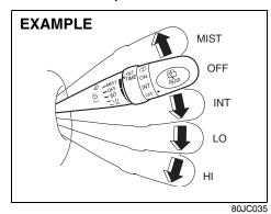
To turn the windshield wipers on, move the lever down to one of the three operating positions. In the "INT" position (if equipped), the wipers operate intermittently. The "INT" position is very convenient for driving in mist or light rain. In the "LO" position, the wipers operate at a steady low speed. In the "HI" position, the wipers operate at a steady high speed. To turn off the wipers, move the lever back to the "OFF" position.
