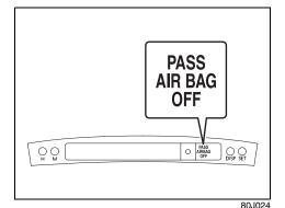
When the ignition switch is turned to the "ON" position, the "PASS AIR BAG OFF" indicator comes on for several seconds to
