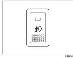
The front fog light comes on when the fog light switch is pushed in with the lighting switch turned to the third position and the beams set to the low beam position.
