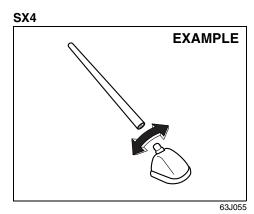
The radio antenna at the end of the roof is removable. If the antenna hits anything such as when parking in a garage with a low ceiling, remove the antenna. Turn the antenna counterclockwise. To reinstall the antenna, turn it clockwise firmly by hand.
