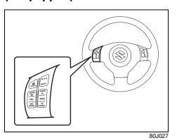
You can control basic functions of the audio system with the switches on the steering wheel. For details, refer to "Audio Systems" in the "INSTRUMENT PANEL" section.
