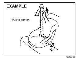
Try moving the child restraint system in all directions, to make sure it is securely installed. If you need to tighten the belt, pull more webbing toward the retractor.
