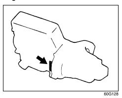
The engine serial number is stamped on the cylinder block as shown in the above illustration. Safety Certification Label: 6 Emission Compliance Label (For U.S.A.): 1, 2 Warranties: NO
