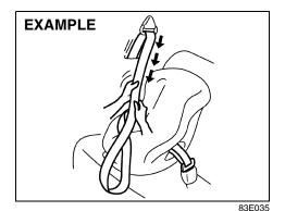
1) Pull all of the remaining webbing out of the retractor. You will hear a click, which means that the emergency locking retractor (ELR) has converted to function as an automatic locking retractor (ALR).
