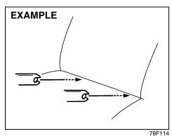
2) Place the child restraint in the second row seat, inserting the connecting bars through the slots in the seat cushion or the slots in the seatback bottom.
