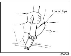
To reduce the risk of sliding under the belt during a collision, position the lap portion of the belt across your lap as low on your hips as possible and adjust it to a snug fit
