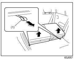
5) Pull the lock release strap (1) rearward to unlatch the seat cushion.
