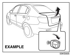
If your vehicle is equipped with a trunk lid key lock, you can open the trunk lid by using the key in the trunk lid lock. To open the trunk lid, insert the key and turn it clockwise to unlatch and lift the trunk lid.
