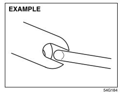
Push the child restraint toward the anchors so that the connecting bar tips are partially hooked to the anchors. Use your hands to confirm the position.
