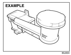
Check the brake fluid level by looking at the reservoir in the engine compartment. Check that the fluid level is between the "MAX" and "MIN" lines. If the brake fluid level is near the "MIN" line, fill it up to the "MAX" line with DOT3 brake fluid.
