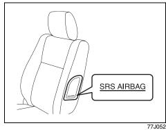
Side air bags are located in the part of the front seatbacks closest to the doors. The words "SRS AIRBAG" are molded into the side air bag cover to identify the location of the side air bags.
