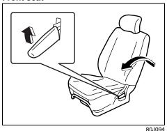
To adjust the seatback angle of front seats, pull up the lever on the outboard side of the seat, move the seatback to the desired position, and release the lever to lock the seatback in place. After adjustment, try moving the seatback to make sure it is securely locked.
