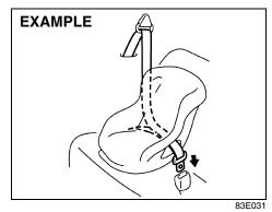
Install your child restraint system according to the instructions provided by the child restraint system manufacturer. If you install the child restraint system in the front seat, be sure to slide the seat to the rearmost position. After making sure that the seat belt is securely latched:
