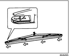
2) Install the new blade in the reverse order of removal. Make sure that the blade is properly retained by all the hooks and the end is locked in place. To remove and install some types of rear wiper blade from and to the wiper frame.
