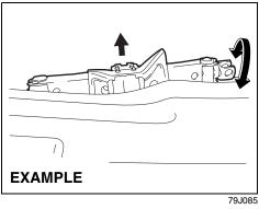
To remove the jack, turn its shaft counterclockwise and pull the jack out of the storage bracket. Accessory Socket: 8 Frame Hooks: 5, 6
