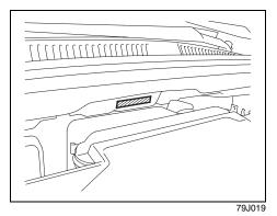
The Vehicle Identification Number (VIN) may be found in the location shown in the above illustrations. This number is used to register the vehicle. It is also used to assist your dealer when ordering parts or referring to special service information.
