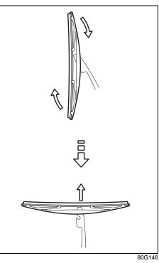
2) Remove the wiper frame from the arm as shown.
