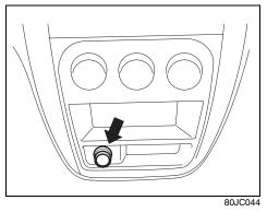
This socket can be used to provide 12 volt/ 120 watt power for electrical accessories.
