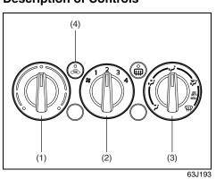
**Temperature selector (1)** This is used to select the temperature by turning the selector.
