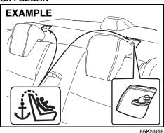
Some child restraint systems require the use of a top strap. Top strap anchor brackets are provided in your vehicle at the locations shown in the illustrations. Install the child restraint system as follows:
