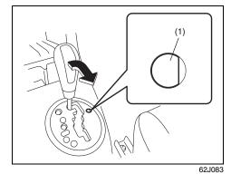
If the gearshift lever can not be shifted out of "P" (Park) in the normal way, removing the cover (1) and pushing the release button using a key or some other flat end object with the key in the "ON" or "ACC" position will permit movement of the gearshift lever out of "P" (see "If You Can Not Shift Automatic Transaxle Gearshift Lever Out of "P" (PARK)" in the INDEX). The gearshift lever can be moved back to "P" without pushing the release button.
