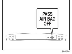
The "PASS AIRBAG OFF" indicator is located on the information display. When the ignition switch is turned to the "ON" position, this indicator comes on for several seconds to let you know the indicator is working.
