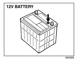
Use only a 12 volt battery to jump start your vehicle. Position the good 12V battery close to your vehicle so that the jumper cables will reach both batteries. When using a battery installed on another vehicle, DO NOT LET THE VEHICLES TOUCH. Set the parking brakes fully on both vehicles.  Turn off all vehicle accessories, except those necessary for safety reasons (for example, headlights or hazard lights).
