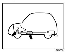
The purpose of the catalytic converter is to minimize the amount of harmful pollutants in your vehicle's exhaust. Use of leaded fuel in vehicles equipped with catalytic converters is prohibited by federal law, because lead deactivates the pollutantreducing components of the catalyst system.
