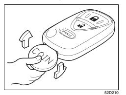
1) Put the edge of a coin or a flat blade screw driver in the slot of the transmitter and pry it open.
