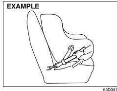
4) Return the seatback to the normal, upright position. Tighten the lower straps as described in the child restraint owner's manual. Attach the top tether strap, if applicable.
