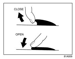
To open a window, push the top part of the switch and to close a window lift up the top part of the switch.
