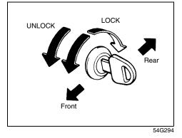
(when using the key) To lock all the doors simultaneously, insert the key in a front door lock and turn the top of the key toward the rear of the vehicle once.
