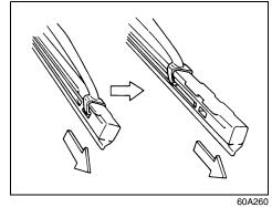
3) Pull the locked end of the wiper blade firmly to unlock the blade and slide the blade out as shown.
