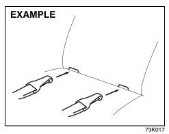
2) Place the child restraint in the second row seat, feeding the strap hooks through the slots in the seat cushion or the slots in the seatback bottom.
