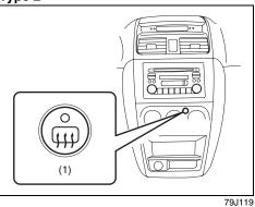
When the rear window is misted, push this switch (1) to clear the window.
