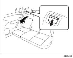
4) Pull the release lever on the top of each split seat, and fold the seatbacks forward.
