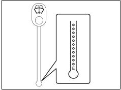
Check that there is washer fluid in the tank by looking at the washer fluid level gauge which is attached to the cap of the washer fluid tank. If the fluid level is near "E" mark, refill it.
