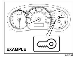
If the keyless start system blue indicator light illuminates on the instrument cluster, you can turn the ignition switch. If the red indicator light illuminates, you can not turn the ignition switch.
