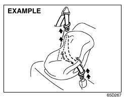
When you unbuckle the seat belt and allow it to retract to a certain length, the retractor will automatically revert back to the normal ELR mode.
