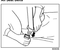
To fasten the seat belt, sit up straight and well back in the seat, pull the latch plate attached to the seat belt across your body and press it into the buckle until you hear a "click".
