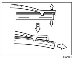
Flex the ends of blade and frame, and slide the blade out as shown.
