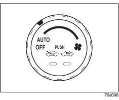
This is used to turn on the blower and to select blower speed.
