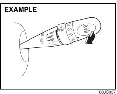
To spray windshield washer fluid, pull the lever toward you. The windshield wipers will automatically turn on at low speed if they are not already on and the "INT" position is equipped.
