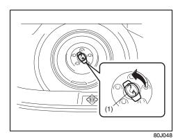
To remove the spare tire, turn its bolt (1) counterclockwise and remove it.
