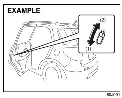
Each of the rear doors is equipped with a child lock which can be used to help prevent unwanted opening of the door from inside the vehicle. When the lock lever is in the "LOCK" position (1), the rear door can only be opened from outside. When the lock lever is in the "UNLOCK" position (2), the rear door can be opened from inside or outside.
