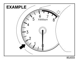
The tachometer indicates engine speed in revolutions per minute.
