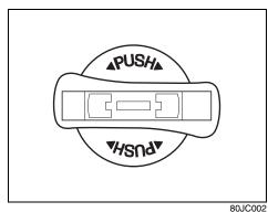
The ignition switch can be operated without using an ignition key when the remote controller is in an area of the vehicle other than the rear luggage area. To turn the ignition switch, first push in the switch.
