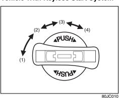
The ignition switch can be operated without using an ignition key when the remote controller is in an area of the vehicle other than the rear luggage area. To turn the ignition switch, first push in the switch.
