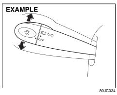
Some times, such as when changing lanes, the steering wheel is not turned far enough to cancel the turn signal. For convenience, you can flash the turn signal by moving the lever part way and holding it there. The lever will return to its normal position when you release it.
