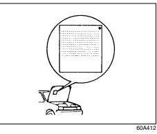
The EPA emission compliance label is located under the hood.
