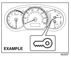
If the keyless start system blue indicator light illuminates on the instrument cluster, you can turn the ignition switch. If the red indicator light illuminates, you can not turn the ignition switch.
