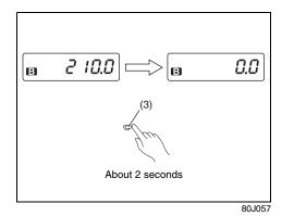
Hold in the selector knob for about 2 seconds to reset the trip meter to zero.
