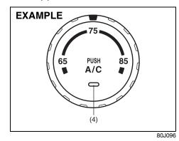
This is used to select the temperature by turning the selector.
