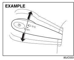
Move the lever all the way upward or downward to signal. When the turn is completed, the signal will cancel and the lever will return to its normal position.
