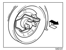
Open the engine hood. Remove the coupler and the rubber cover. Then unhook the bulb holding spring and replace the bulb.
