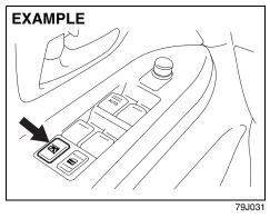
The driver's door also has a lock switch for the passenger's window. When you push in the lock switch, the passenger's window can not be raised or lowered by operating any of the switches (2), (3), (4) or (5). To restore normal operation, release the lock switch by pushing the switch again.
