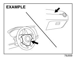
The driver's front air bag is located behind the center pad of the steering wheel. The words "SRS AIRBAG" are molded into the air bag cover to identify the location of the air bag. The front passenger's front air bag is located behind the passenger's side of the dashboard. The words "SRS AIRBAG" are molded into the air bag cover to identify the location of the air bag.
