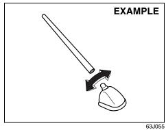
The radio antenna on the roof is removable. To remove the antenna, turn it counterclockwise. To reinstall the antenna, turn it clockwise firmly by hand.
