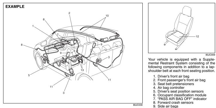
following components in addition to a lapshoulder belt at each front seating position.
