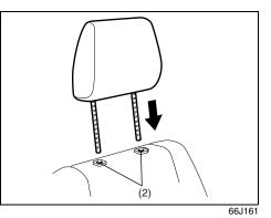
To reinstall the head restraint, insert the head restraint bars into the holes (2) and push the head restraint down.
