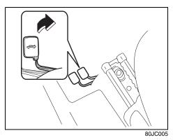
You can unlock the lid by pulling the release lever located to the outboard side of the driver's seat.
