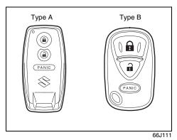
Your vehicle is equipped with either a keyless start system remote controller (Type A) or a keyless entry system transmitter (Type B). The remote controller has a keyless entry system and a keyless start system. The transmitter has only a keyless entry system. For details, refer to the following explanations.
