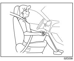
When seated as shown in the above illustration, the front passenger sensing system senses a properly-seated occupant and enables the air bag. When using a seat belt extender, follow the instructions in the "Seat Belt Extender" section.
