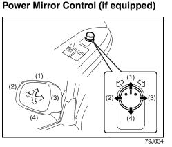
The switch to control the power rearview mirrors is located on the driver's door panel. You can adjust the mirrors when the ignition switch is in the "ACC" or "ON" position. To adjust the mirrors:
