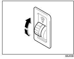
Your vehicle has a system to automatically dim the instrument panel lights when the ignition switch is in the "ON" position and the lighting switch is turned to either the second or third position. The level of brightness depends on the position of the brightness control thumbwheel.
