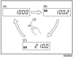
When the ignition switch is turned to "ON" with the lighting switch is in the "OFF" position, the display shows three types of indication; odometer (A), trip meter A (B) and trip meter B (C). Push the selector knob (3) quickly to switch the indication among the three.
