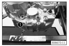
Mount and tighten screw plug • with the O-ring.
