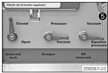
When the vacuum pressure gauge reaches the specified value, turn the Oil reservoir control lever 6 to Equalize pressure.
