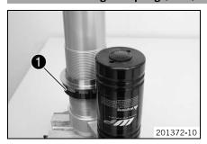
Ensure that adjusting ring • is screwed on with the intermediate washer.
