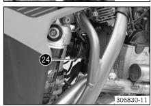
Position and tighten hose clip <a>®</a>.
