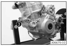
Pull oil filter 3 out of the oil filter housing.
