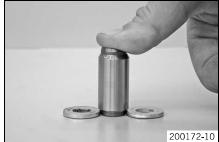
Place two compensating disks or similar aids next to the timing chain tensioner piston. This ensures that, when pressed in, the piston cannot go in all the way.
