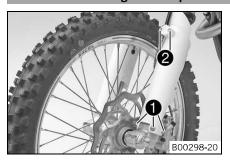
Position the fork protection on the left fork leg. Mount and tighten screws
