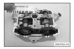
Remove camshaft bearing bridge again. Compare the Plastigauge clearance gauge with the specifications on the packaging.
