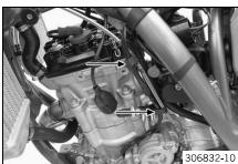
Remove the cable clips and expose the cable.
