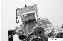
Cover the engine case opening with a cloth. Thread the timing chain through the chain shaft. Mount the piston pin.
