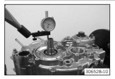
Insert the crankshaft into the right section of the engine case.
