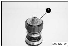
Mount the rebound shim stack with the smaller shims facing upward.
