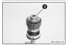
Grease the thread of the piston rod.
