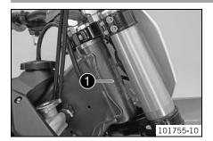
The chassis number • is stamped on the right side of the steering head.
