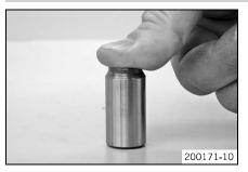
Press the timing chain tensioner together completely.
