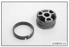
Remove the piston ring from the piston.
