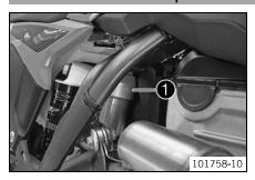
The shock absorber part number  $\bullet$  is stamped on the top of the shock absorber above the adjusting ring on the engine side.
