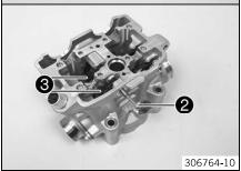
Pre-tension the valve spring using the special tool.
