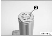
Remove the screw. Remove adjuster 3 of the compression damping.
