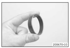
Roughen, clean and lubricate the edges of the sliding bushings using 600 grit sandpaper.
