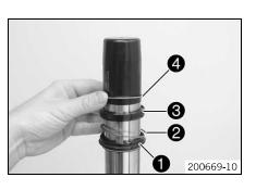
Lubricate and slide on dust boot 1.
