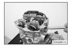
Check the valve clearance at all valves between the camshaft and cam levers.
