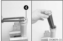
Loosen and remove screw cap 4 with the membrane holder.
