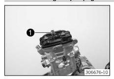
Mount and tighten the spark plug with special tool ①.
