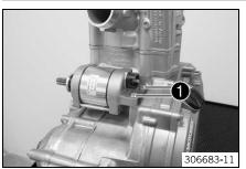
Grease the O-ring. Position the starter motor.
