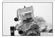
Push the cylinder upward.
