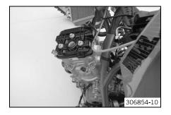
Lift out the engine from the side.
