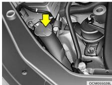
The washer fluid reservoir supplies fluid to the front and rear washer systems.
