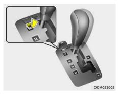
If you cannot move the shift lever from the "P" (Park) position to any other position with the brake pedal fully depressed and the ignition key in the "ON" position, remove the cap on the console and with a thin object such as a flat-head screwdriver, push the shift lock release button down.
