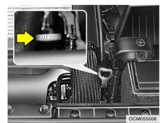
2. Remove the transaxle dipstick, wipe it clean, reinsert the dipstick as far as it will go, then remove it again. Now check the fluid level on the dipstick. It should be in the 75°C range on the dipstick.
