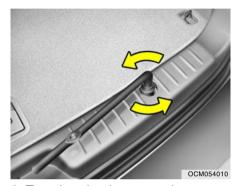
3. Turn the wheel nut wrench counterclockwise until the spare tire reaches the ground.
