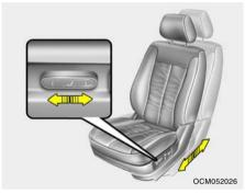
Push the control knob forward or backward to move the seat forward or backward to the desired position. Release the control knob and the seat will remain at that position.
