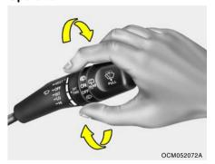
To use the intermittent wiper feature, place the wiper switch in the "INT" position. With the switch in this position, the interval between wipes can be varied by turning the interval adjuster barrel.
