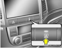
The outside rearview mirror heater is actuated in connection with the rear window defroster. To heat the outside rearview mirror glass, push in the switch for the front/ rear window defroster. The rearview mirror glass will be heated for defrosting or defogging and will give you improved rear vision in inclement weather conditions. Push the switch again to turn the heater off. The outside rearview mirror heater automatically turns itself off after 20 minutes.
