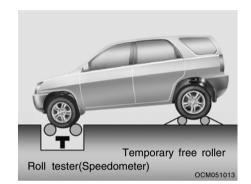
(9) For a speedometer test or inspection/ maintenance (I/M) program of a Santa Fe AWD vehicle, use a four wheel chassis dynamometer.
