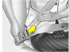
The seat belt is released by pressing the release button in the locking buckle. When it is released, the belt should automatically draw back into the retractor.
