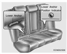
The lower anchors are located between the seatback and the seat cushion of the 2nd rear seat left and right outboard seating positions.
