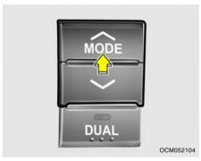
This is used to direct the flow of air. Air can be directed to the floor, dashboard outlets, or windshield. Four symbols are used to represent Face, Bi-Level, Floor and Floor-Defrost position.
