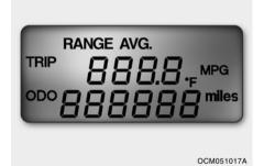
Trip computer is a microcomputer-controlled driver information system that displays information related to driving on the LCD.
