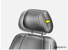
The headrest may be adjusted forward to three different positions by pulling the headrest forward. To adjust the headrest rearward, pull it fully forward to the farthest position and release it. Adjust the headrest so that it properly supports the head and neck.
