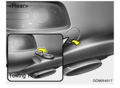
For emergency towing when no commercial tow vehicle is available. Do not attempt to tow your vehicle in this manner on any unpaved surface.
