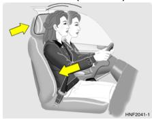
The active headrest is designed to move forward and upward during a rear impact. This helps to prevent the driver's and front passenger's heads from moving backward and thus helps prevent neck injuries.
