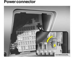
Your vehicle is equipped with a power connector to prevent battery discharge if your vehicle is parked without being operated for prolonged periods. Use the following procedures before parking the vehicle for prolonged periods.
