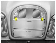
Push in the map light switch to turn the light on or off. This light produces a spot beam for convenient use as a map light at night or as a personal light for the driver and the passenger.
