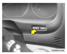
When the RESET switch is pressed for 1 second, the tripmeter will reset to 0.
