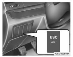
The Electronic Stability Control (ESC) system is designed to stabilize the vehicle during cornering manuevers. ESC checks where you are steering and where the vehicle is actually going. ESC applies the brakes at individual wheels and intervenes in the engine management system to stabilize the vehicle.
