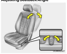
Push the upper portion of the control knob forward or backward to recline the seatback to the desired position. Release the control knob and the seatback will remain in that position.
