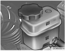
It is normal for the brake fluid level to go down slightly as the brake pads wear. The fluid level in the brake fluid reservoir should be checked periodically. The level should be between the "MIN" and "MAX" marks on the side of the reservoir. If the level is at or below the "MIN" mark, carefully add fluid to bring it up to "MAX".
