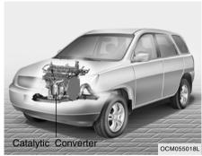
All Hyundai vehicles are equipped with a monolith type three-way catalytic converter to reduce the carbon monoxide, hydrocarbons and nitrogen oxides contained in the exhaust gas. Exhaust gases passing through the catalytic converter cause it to operate at a very high temperature. The introduction of large amounts of unburned gasoline into the exhaust may cause the catalytic converter to overheat and create a fire hazard. This risk may be reduced by observing the following:
