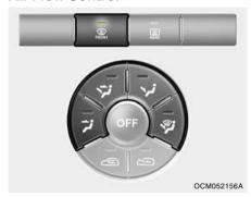
This is used to turn the blower fan on/off and to direct the flow of air. Air can be directed to the floor, dashboard outlets, or windshield. Five symbols are used to represent Face, Bi-Level, Floor, Floor-Defrost and Defrost air position.
