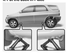
The base of the jack should be placed on firm, level ground. The jack should be positioned as shown in the drawing. D060F03E-AAT **5. Raising the vehicle**
