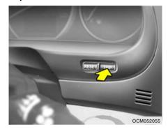
Pushing in the TRIP switch for when the ignition switch is in "ON" position changes the display as follows;
