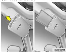
Your vehicle is equipped with sun visor extenders that may be used when the visor is in the side glass position.
