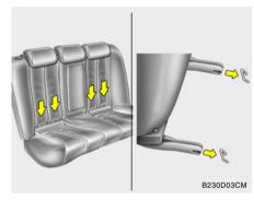
Follow the child seat manufacturer's instructions to properly install safety seats with LATCH or LATCH-compatible attachments.
