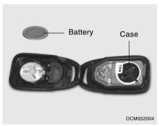
Remove the old battery from the case and note the polarity. Make sure the polarity of the new battery is the same (+side facing down), then insert it in the transmitter.
