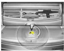
Remove the spare tire and remove the jack and tool bag from the luggage compartment.
