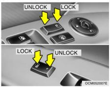
The central door locking switch is located on the driver's and front passenger's armrest. It is operated by depressing the door lock switch. If any door is open when the switch is depressed to the "LOCK" position, the door will remain locked when closed.
