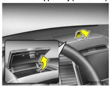
The center facia upper tray is used for storing small articles. To use the center facia upper tray, pull up the button and lift lid to open it.
