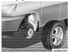
Loosen the wheel nuts and remove them. Slide the wheel off the studs and lay it flat so it cannot roll away. To put the wheel on the hub, pick up the spare tire, line up the holes with the studs and slide the wheel onto them. If this is difficult, tip the wheel slightly and get the top hole in the wheel lined up with the top stud. Then jiggle the wheel back and forth until the wheel can be slid over the other studs.
