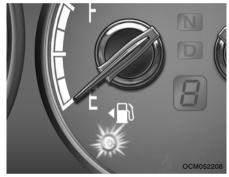
The low fuel level warning light illuminates when the fuel tank is approaching empty. When it illuminates, you should add fuel as soon as possible. Driving with the fuel level warning light on or with the fuel level below "E" can cause the engine to misfire and damage the catalytic converter.
