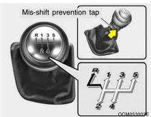
This shift pattern is imprinted on the shift knob. The transaxle is fully synchronized in all forward gears so shifting to either a higher or a lower gear is easily accomplished.
