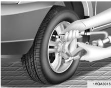
If you have a tire gauge, remove the valve cap and check the air pressure. If the pressure is lower than recommended, drive slowly to the nearest service station and inflate to the correct pressure. If it is too high, adjust it until it is correct. Always reinstall the valve cap after checking or adjusting tire pressure. If the cap is not replaced, dirt and moisture could get into the valve core and cause air leakage. If you lose a valve cap, buy another and install it as soon as possible.
