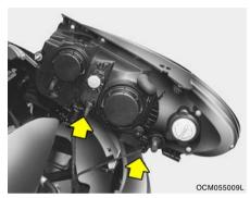
5. Disconnect the wire harness from the bulb base in the back of the headlight.
