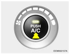
The air conditioning is turned on by pushing the A/C button on the heating/air conditioning control panel.
