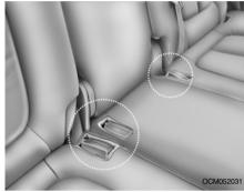
NOTE: Before folding the seatback, place the rear seat belt buckles in the buckle pouch on the seat cushion.
