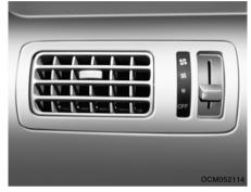
The rear ventilators are located in quarter trim. To change the direction of the air flow, move the knob in the center of the vent side to side. The blower fan speed may be controlled by setting the control lever to the desired position.
