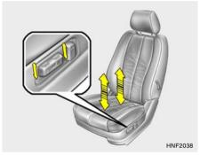
Move the front portion of the control knob up or down to raise or lower the front part of the seat cushion. Move the rear portion of the control knob up or down to raise or lower the rear part of the seat cushion.
