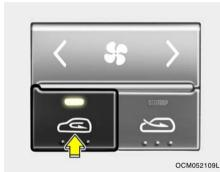
RECIRCULATION MODE (  $\stackrel{\blacksquare}{ \ \ }$  ) : The indicator light on the button is illuminated when the air intake control is recirculation mode.
