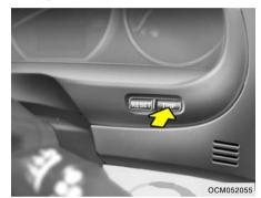
Pushing in the TRIP switch when the ignition switch is turned "ON" will display two tripmeters in kilometers or miles.
