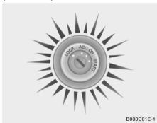
Whenever either front door is opened, the ignition switch will be illuminated for your convenience, provided the ignition switch is not in the "ON" position.
