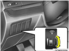
The instrument panel lights can be made brighter or dimmer by turning the instrument panel light control knob.
