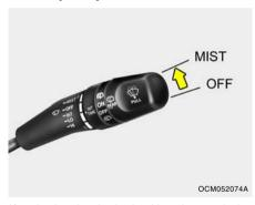
If a single wipe is desired in mist, push the windshield wiper and washer control lever upwards.
