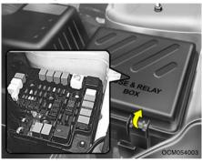
A fusible link will melt if the electrical circuits from the battery are ever overloaded, thus preventing damage to the entire wiring harness. (This could be caused by a short in the system drawing too much current.) If this ever happens, have a Hyundai dealer determine the cause, repair the system and replace the fusible link. The fusible links are located in a relay box in the engine compartement for easy inspection.
