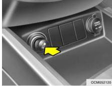
For the cigarette lighter to work, the key must be in the "ACC" position or the "ON" position. To use the cigarette lighter, push it all the way into its socket. When the element has heated, the lighter will pop out to the "ready" position. Do not hold the cigarette lighter pressed in. This can damage the heating element and create a fire hazard. If it is necessary to replace the cigarette lighter, use only a genuine Hyundai replacement or its approved equivalent.
