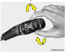
The washer fluid will be sprayed onto the rear window and the wiper operates while the rear window wiper barrel is placed in this position.
