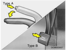
Always engage the parking brake before leaving the car. This also turns on the parking brake indicator light when the key is in the "ON" or "START" position.
