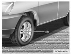
To reinstall the wheel, hold it on the studs, put the wheel nuts on the studs and tighten them finger tight. The nuts should be installed with their small diameter ends directed inward. Jiggle the tire to be sure it is completely seated, then tighten the nuts as much as possible with your fingers again.
