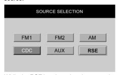
While the RSE is selected as the source by the front vehicle radio, the front vehicle radio will be able to control some RSE functions (e.g. Fast Forward / Reverse, Previous / Next Track, etc.). See your vehicle radio user manual for more information.
