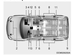
The SRS consists of the following components:
