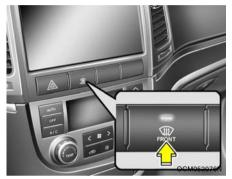
When the "Defrost" button is pressed, the "" mode will be automatically selected and the air will be discharged through the windshield defroster nozzle, side defroster nozzle and side ventilator. To assist in defrosting, the air conditioning will operate according to the ambient temperature.
