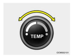
2. Turn the "TEMP" knob to set the desired temperature.
