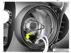
8. Push the bulb spring to remove the headlight bulb.
