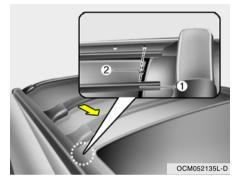
You can reposition the front crossbar more to the frontside of the vehicle to transport ski equipment or other goods. After removing the bumper molding ① and mounting bolt ②, move the crossbar frontside of the vehicle and fix it up with a bolt into the hole. And then reinstall the bumper molding.
