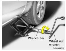
After inserting the wrench bar into the wheel nut wrench, install the wrench bar into the jack as shown in the drawing. To raise the vehicle, turn the wheel nut wrench clockwise. As the jack begins to raise the vehicle, double check that it is properly positioned and will not slip. If the jack is on soft ground or sand, place a board, brick, flat stone or other object under the base of the jack to keep it from sinking.
