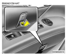
The fuel-filler lid may be opened from inside the vehicle by pulling up on the fuelfiller lid opener located on the driver's door.
