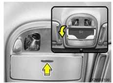
The sunglass holder is located on the front overhead console. Push the end of the cover to open the sunglass holder.
