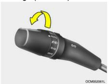
To operate the automatic light feature, turn the barrel on the end of the multi-function switch. If you set the multi-function switch to "AUTO", the tail lights and headlights will be turned automatically on or off according to external illumination conditions.
