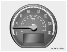
Your Hyundai's speedometer is calibrated in miles per hour (on the outer scale) and kilometers per hour (on the inner scale).
