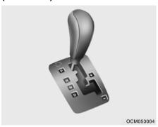
The highly efficient Hyundai automatic transaxle has four/five forward speeds and one reverse speed. The individual speeds are selected automatically, depending on the position of the speed selector lever. The selector lever has 2 gates; the main gate and the manual gate.
