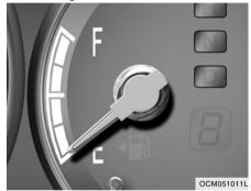
The needle on the gauge indicates the approximate fuel level in the fuel tank. The fuel capacity is given in Section 9.
