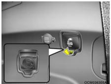
These supply 115VAC/150W electric power to operate electric accessories or equipment when the key is in the "ON" position or engine is running. The AC Inverter is turned on by pushing in the switch. To turn the AC Inverter off, push the switch a second time.
