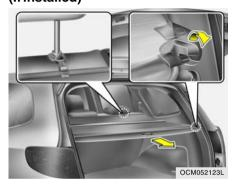
To use the security screen, pull it out of the retractor and hook it to the anchors as illustrated.
