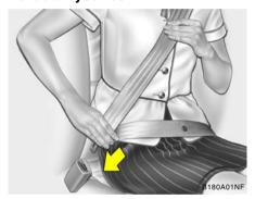
To fasten your seat belt, pull it out of the retractor and insert the metal tab into the buckle. There will be an audible "click" when the tab locks into the buckle.
