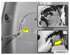
If the fuel filler lid does not open using the remote fuel filler lid release, you can open it manually. Unsnap and remove the panel in the rear cargo area. Pull the handle outward.
