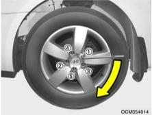
Then position the wrench as shown in the drawing and tighten the wheel nuts. Be sure the socket is seated completely over the nut. Do not stand on the wrench handle or use an extension pipe over the wrench handle.
