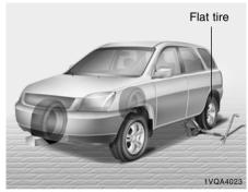
Block the wheel that is diagonally opposite from the flat to keep the vehicle from rolling when the vehicle is raised on the jack.
