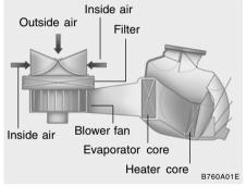
The climate control air filter is located in front of the evaporator unit behind the glove box.
