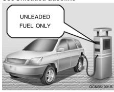
Unleaded gasoline with a Pump Octane Rating of 87(Research Octane Number 91) or Higher must be used. For improved vehicle Performance, premium unleaded gasoline with Pump Octane Rating of 91(RON 95) or higher is recommended.
