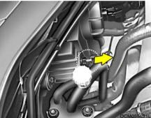
4. Using a wrench, remove the headlight assembly mounting bolts and nut.
