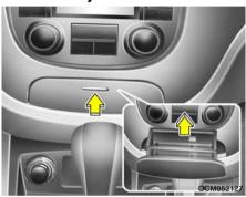
The front ashtray may be opened by pushing and releasing the ashtray lid. To remove the ashtray to empty or clean it, lift the ashtray upward and pull it out. The ashtray light will only illuminate when the external lights are on.
