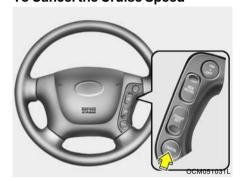
To disengage the cruise control system, push the control switch "CANCEL". Additionally, the following actions will disengage the system:
