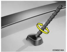
Your car uses a roof antenna to receive both AM and FM broadcast signals. This antenna is a removable type. To remove the antenna, turn the antenna counterclockwise. To install the antenna, turn the antenna clockwise.
