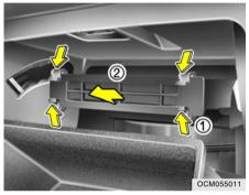
4. Pull out the climate control air filter with the hooks on both sides pressed.
