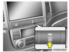
The rear window defroster and heated outside rear view mirrors are turned on by pushing in the switch when the engine is running. At the same time, the rear window defroster indicator light on the switch is turned on. To turn the defroster off, push the switch a second time. The rear window defroster automatically turns itself off after about 20 minutes. To restart the defroster cycle, push in on the switch again after it has turned itself off.
