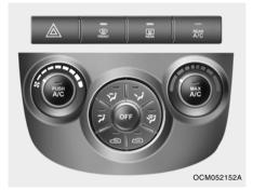
For normal heating operation, set the air intake control to the fresh air ( ) position and the air flow control to the floor ( ) position.
