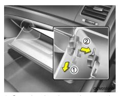
1. Open the glove box and remove the adjusting pins on both sides of the glove box.
