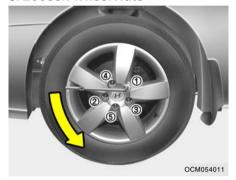
The wheel nuts should be loosened slightly before raising the car. To loosen the nuts, turn the wrench handle counterclockwise. When doing this, be sure that the socket is seated completely over the nut so it cannot slip off. For maximum leverage, position the wrench so the handle is to the left as shown in the drawing. Then, while holding the wrench near the end of the handle, push down on it with steady pressure. Do not remove the nuts at this time. Just loosen them about one-half turn.
