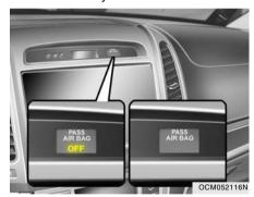
If the front passenger seat is occupied by a person that the system determines to be of adult size, and he/she sits properly (sitting upright with the seatback in an upright position, centered on the seat cushion with their seat belt on, legs comfortably extended and their feet on the floor), the passenger air bag off indicator will be turned off (The "OFF" will not illuminate) and the front passenger's air bag will be able to inflate, if necessary, in frontal crashes.
