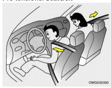
Your Hyundai vehicle is equipped with driver's and front passenger's pre-tensioner seat belts. The purpose of the pre-tensioner is to make sure that the seat belts fit tightly against the occupant's body in certain frontal collisions. The pre-tensioner seat belts can be activated together with the air bags.
