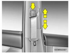
You can adjust the height of the shoulder belt anchor to one of the 4 positions for maximum comfort and safety.
