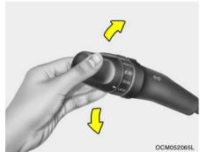
To indicate a lane change, move the lever up or down to a point where it begins flashing.
