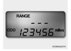
When the estimated distance to empty is less than 30 miles, the distance to empty digits (---) will blink until more fuel is added.
