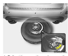
4. Pull out the spare tire and remove the retainer from the center of spare tire.
