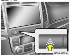
The hazard warning system should be used whenever you find it necessary to stop the car in a hazardous location. When you must make such an emergency stop, always pull off the road as far as possible. The hazard warning lights are turned on by pushing in the hazard switch. This causes all turn signal lights to blink. The hazard warning lights will operate even though the key is not in the ignition.
