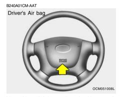
Your Hyundai is equipped with an advanced Supplemental Restraint (Air bag) System. The indications of the system's presence are the letters "SRS AIR BAG" embossed on the air bag pad cover in the steering wheel and the passenger's side front panel pad above the glove box.
