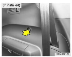
The power outlets are designed to provide power for mobile telephones or other devices designed to operate with vehicle electrical systems. The devices should draw less than 10 amps with the engine running.
