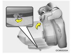
3. Pull the seat cushion release lever and then fold up the seat cushion.
