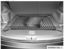
When loading objects in the luggage compartment, use the four rings located in the luggage compartment to attach the luggage net as shown illustration. This will help prevent the objects from sliding.
