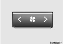
The fan speed can be set to the desired speed by pressing the appropriate fan speed control button. The higher the fan speed is, the more air is delivered. Pressing the "OFF" button turns off the fan.
