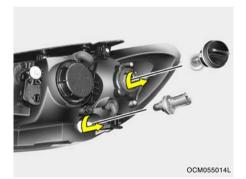
12. To replace the front turn signal light bulb or the front position light bulb, take it out from the bulb holder and install the new bulb.
