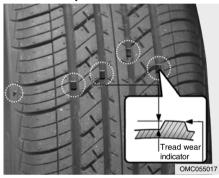
The original tires on your car have tread wear indicators. The location of tread wear indicators is shown by the "TWI" or "\(\times\)" marks, etc., The tread wear indicators appear when the tread depth is 0.06 in. (1.6 mm). The tire should be replaced when these appear as a solid bar across two or more grooves of the tread. Always replace your tires with those of the recommended size. If you change wheels, the new wheel's rim width and offset must meet Hyundai specification.
