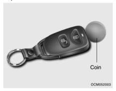
1. Carefully separate the case with a coin as shown in the illustration.
