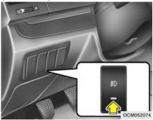
To turn on the front fog lights, push the switch in the "ON" position. They will light when the headlight switch is in the second position.
