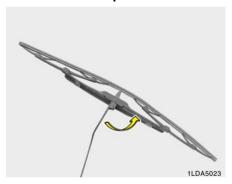
Raise the wiper arm and turn the wiper blade assembly to expose the plastic locking clip.
