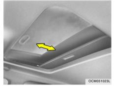
Your vehicle is equipped with a sliding sunshade which you can manually adjust to let in light with the sunroof closed, or to block sunlight.
