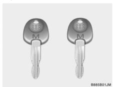
All of the locks fitted to the vehicle are operated by the same key. However, since it is possible to lock the doors without the use of the key, care should be exercised to ensure that the key does not become locked inside the vehicle by mistake.
