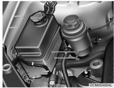
The coolant level can be seen on the side of the plastic coolant reservoir. The level of the coolant should be between the "L" and "F" lines on the reservoir when the engine is cool. If the level is below the "L" mark, add engine coolant to bring it up between "L" and "F". If the level is low, inspect for coolant leaks and recheck the fluid level frequently. If the level drops again, visit your Hyundai dealer for an inspection and diagnosis of the reason.
