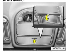
To use the mirror, push the cover and open it. Adjust mirror angle to the desired position.
