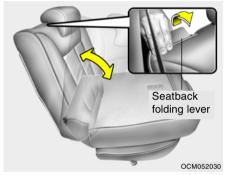
To recline the seatback, pull the seatback folding lever and release it after the desired seatback angle is achieved.
