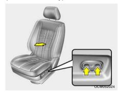
To adjust the lumbar support, press the control switch on the outboard side of the seat cushion. To increase the amount of lumbar support, press the front portion of the switch. To decrease lumbar support, press the rear portion of the switch.
