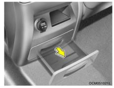
The rear console box is located on the rear main console and may be used for small articles. It is opened by pulling forward.
