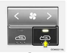
FRESH MODE ( ): The indicator light on the button goes on when the air intake control is fresh mode.
