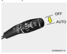
When the windshield wiper switch is placed in the "AUTO" position, the rain sensor located on the upper end of windshield glass senses the amount of rainfall and controls for the appropriate length of the intervals between wipes appropriately.
