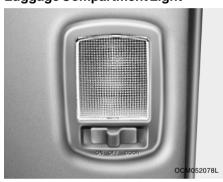
Luggage compartment light has a 3-position switch. The three positions are:
