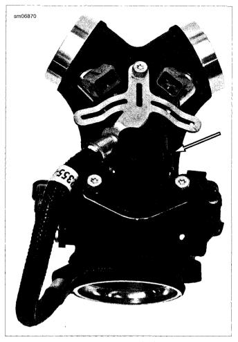
Figure 4-57. Idle Air Control (IAC): XR Models
