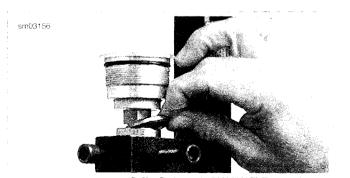
Figure 2-166. Install Keeper
