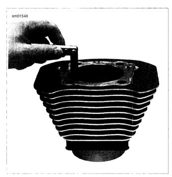
Figure 3-141. Measuring Ring End Gap
