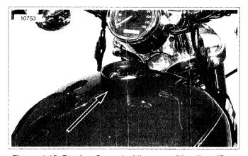
Figure 4-15. Placing Console Alignment Ring Tool (Part No. HD-47114)
