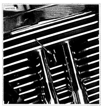
Figure 4-31. Engine Temperature (ET) Sensor Location
