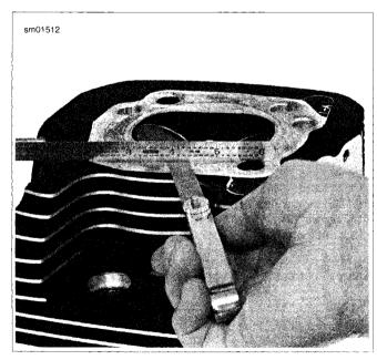
Figure 3-115. Gasket Surface: Flat Within 0.006 in (0.152 mm)
