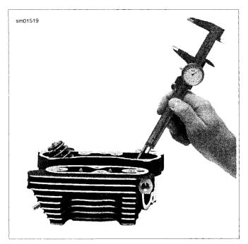
Figure 3-120. Measuring Valve Stem Protrusion
