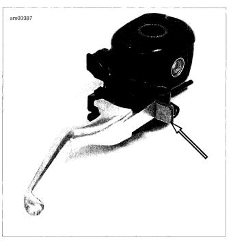
Figure 6-138. Install Cardboard Insert
