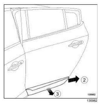
□ Remove the rear side door protective strip at (2) then at (3).
