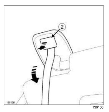
Unclip the locking blanking plug (2) using the tool (Car. 1597).
