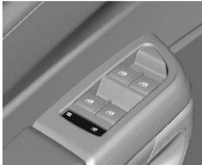
Pulse el interruptor
