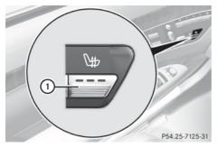
The system automatically switches down from level **3** to level **2** after approximately eight minutes.
