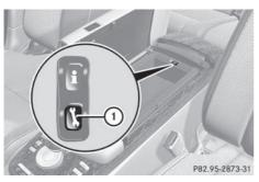
Press and hold Roadside Assistance button ① for more than two seconds. This initiates a call to the Mercedes-Benz Customer Assistance Center. The indicator lamp in Roadside Assistance button ① flashes while the call is active. The Connecting Call message appears in the multifunction display and the COMAND display. The audio output is muted.
