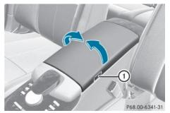
► **To open:** press button ① and fold the armrest to the left or right.
