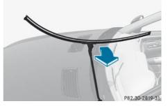
Remove the wiper blade from the retaining pin on the wiper arm in the direction of the arrow.
