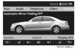
► To activate/deactivate automatic mirror folding: select Vehicle in the main function bar by sliding ← ⊙ → and turning ( ○ ) the COMAND controller and press
