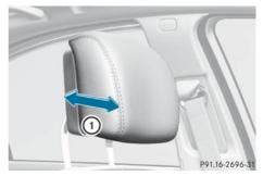
▶ Pull or push the bottom of NECK-PRO head restraint ①.
