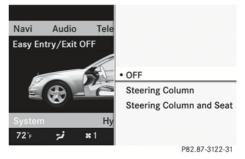
► To set the EASY-ENTRY/EXIT feature: select Vehicle in the main function bar by sliding ←⊙→ and turning () the COMAND controller and press  $\textcircled{\sc b}$  to confirm.
