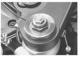
• Apply grease onto the right handlebar before installing the throttle grip.
