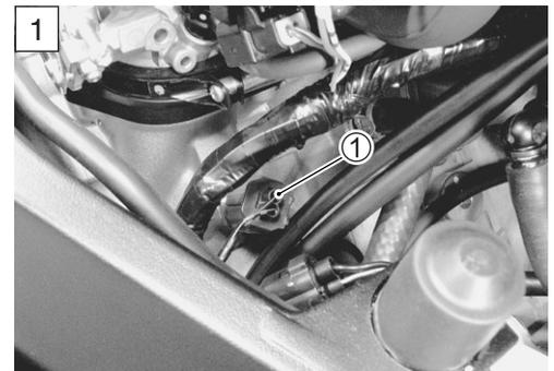
**DATA** ECT sensor voltage: 4.5 – 5.5 V
