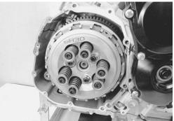
• Install the clutch springs and bolts.
