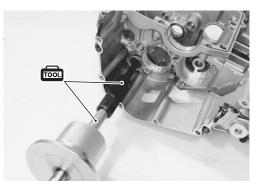
• Remove the gearshift cam bearing with the special tools.
