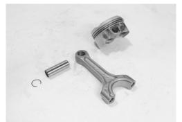
• Remove the piston pin circlip 1.
