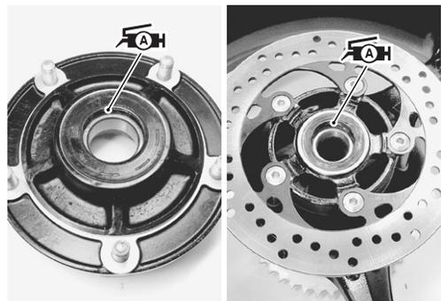
**REAR SPROCKET AND SPROCKET MOUNTING DRUM**
