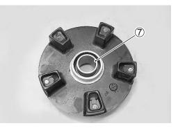
• Remove the dust seal with the special tool.
