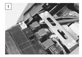
Is the cooling fan relay OK?
