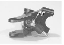
Apply SUZUKI SILICONE GREASE to the bushing and clutch lever pivot bolt.
