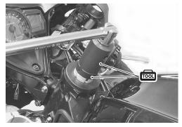
• Remove the dust seal cover ④, dust seal ⑤, steering stem upper bearing inner race ⑥ and bearing ⑦.
