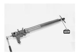
• Remove the inner rod/damper rod (cartridge) 1 .
