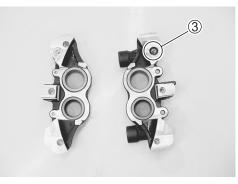
• Place a rag over the pistons to prevent it from popping out and then force out the pistons using compressed air.
