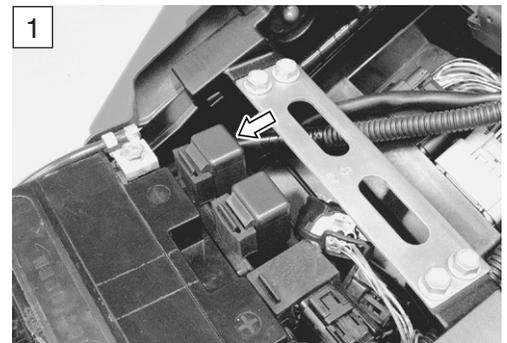
Is the cooling fan relay OK?
