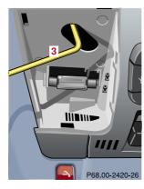
To slide the roof closed or to raise the roof at the rear: turn crank clockwise.
