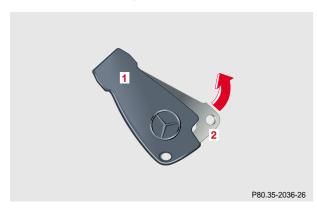
The electronic reserve key is without remote control functions, but with removable mechanical key.
