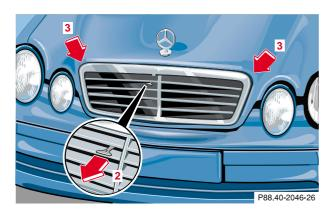
Pull handle (2) to its stop out of radiator grill and open hood (do not pull up on handle).
