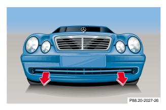
The rear towing eye is located at the right, below the bumper. The front towing eye is located on the passenger side behind the grille in the bumper panel.
