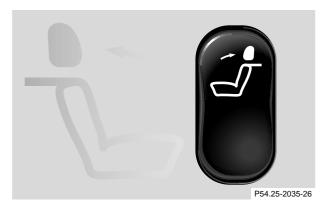
Folding head restraints backward (with engine running):
