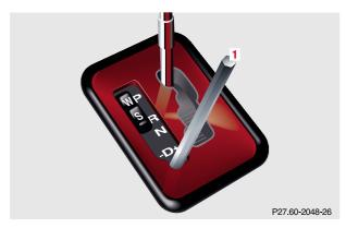
In the case of power failure the transmission selector lever can be manually unlocked, e.g. to tow the vehicle.
