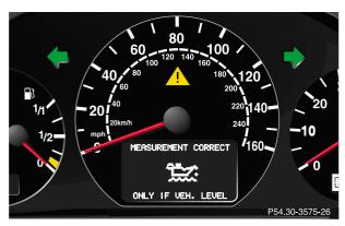
To check the engine oil level, park vehicle on level ground, with engine at normal operational temperature.
