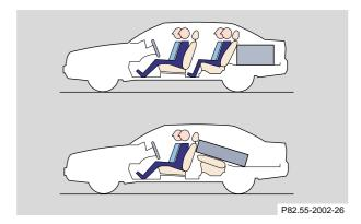
The total load weight including vehicle occupants and luggage/cargo should not exceed the vehicle capacity weight indicated on the certification label which can be found on the left door pillar.
