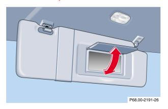
With the visor engaged in its inner mounting, the lamp is switched on by opening the cover.
