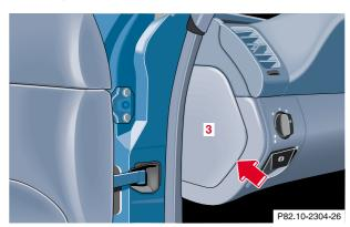
**3** Auxiliary fuse box to left of exterior lamp switch To gain access, open door, pry off cover (3) and remove.
