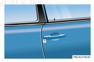
7 Infrared receiver in passenger door handle
