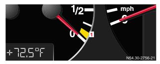
When the warning lamp (1) comes on after starting the engine, or if it comes on while driving, it indicates that the fuel level is down to the reserve quantity of approximately 2.1 gal (8 liters).
