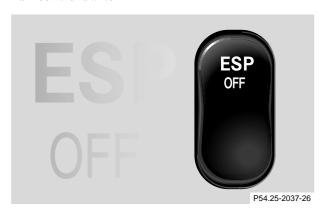
ESP control switch located on center console.
