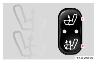
The front seat heater switches are located in the center console.
