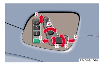
The slide switches are located in each door.
