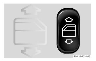
Power window switches located on center console
