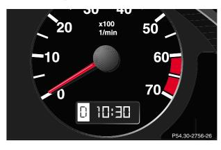
The current selector lever position is indicated in the gear range indicator display. The automatic gear shifting process can be adapted to specific operating conditions using the selector lever.
