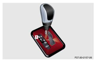
The transmission is provided with a selector switch (1) for Standard "S" and Winter/Wet (snow and ice) "W" program modes.
