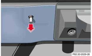
If the trunk is to remain open for a long period of time, the trunk lamp can be switched off by pulling out the plunger in the switch (arrow). This prevents the vehicle battery from being discharged.
