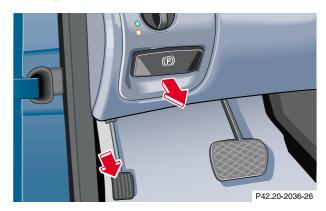
To engage, firmly depress parking brake pedal. When the electronic key is in steering lock position 2, the brake warning lamp in the instrument cluster should come on brightly.
