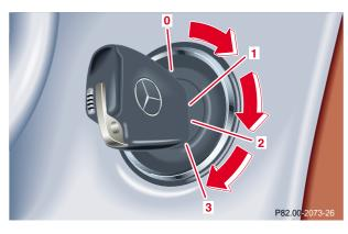
O The electronic key can be withdrawn in this position only. The steering is locked when the electronic key is removed from the steering lock. If necessary, move steering wheel slightly to allow the locking mechanism to engage. The electronic key can only be removed with the selector lever in position "P". After removing the electronic key or with the electronic key in steering lock position 0, the selector lever is locked in position "P".
