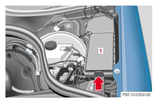
1 Main fuse box in engine compartment
