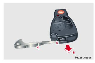
Insert mechanical key (4) in side opening (5) to open latch. Press briefly (do not use mechanical key as lever) to release battery compartment.
