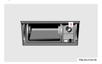
Turn electronic key in steering lock to position 1 or 2. Push in lighter (1); it will pop out automatically when hot.
