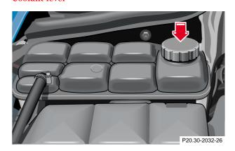
To check the coolant level, the vehicle must be parked on level ground and the engine stopped.
