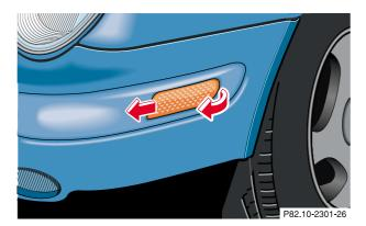
Carefully slide lamp towards front (arrow), and remove back and first.
