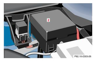
**2** Auxiliary fuse box below the trunk floor. To gain access, lift trunk floor.
