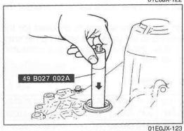
22. Install the **SST** to the differential side gear through the transaxle case.
