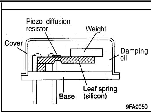
The semiconductor strain gauge type sensor, constructed as shown at the left, consists of a weight mounted at the free end of an N-type silicon leaf spring, and four P-type diffusion layers made on the surface of the leaf spring to constitute piezo diffusion resistors. The case is filled with a damping oil to prevent breakdown that may be caused by resonance.
