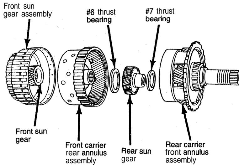
The entire planetary gear-train is located behind the input clutch assembly and is inside the 2-4 and L/R clutch assemblies. The planetary geartrain consists of two sun gears, two planetary carriers, two annulus (ring) gears, and one output shaft.
