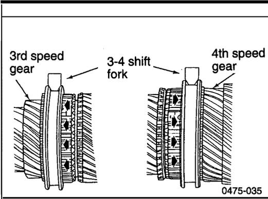
When the 3-4 shift fork moves to the front of the transaxle, third gear is obtained. When it moves to the rear of the transaxle, fourth gear is obtained.
