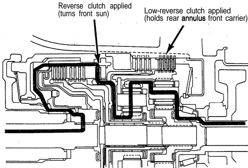
In reverse, input power is through the reverse clutch. When applied, the reverse clutch drives the front sun gear through the overdrive hub and shaft. The L/R clutch is applied to hold the front carrier/rear annulus assembly stationary. The front sun gear
