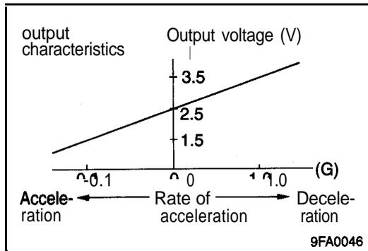
The output characteristics vary as shown at the left in the direction of acceleration with 2.5 V as 0 G.
