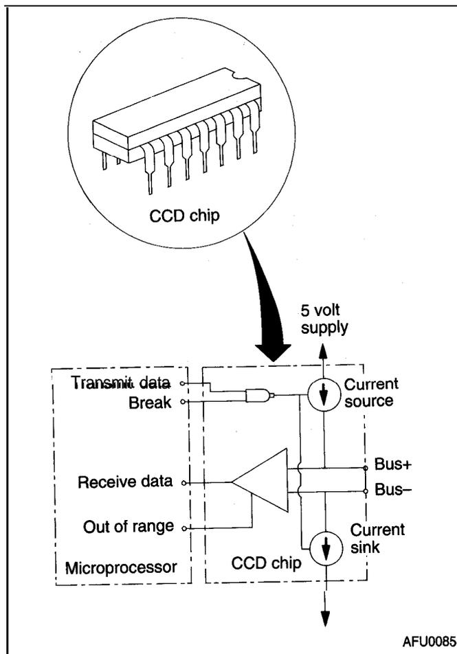
The bus circuits connect inside all modules to a communication chip. The illustration at left shows a representative communication chip block diagram. For communication to occur, the bus must have Biasing and Termination (see the following sections.)
