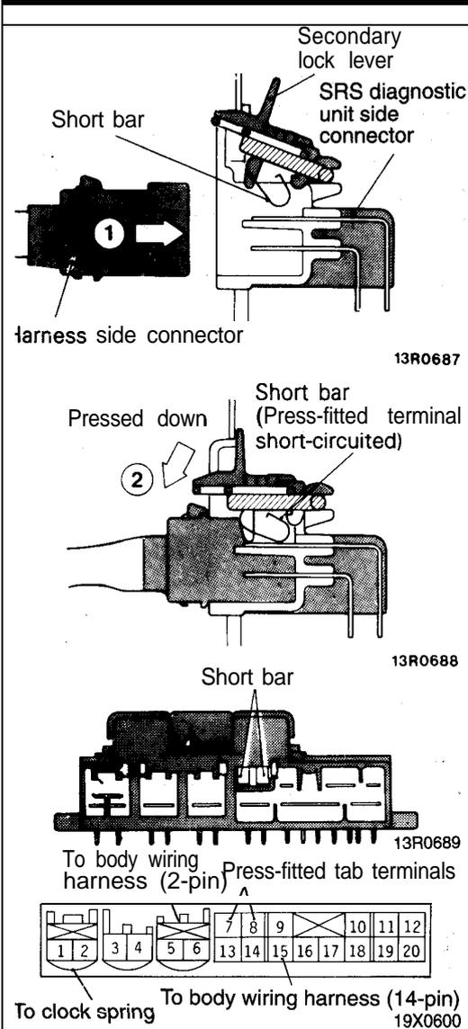
**FIT VERIFICATION MECHANISM**
