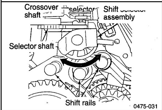
The selector housing blocks the other shift forks and prevents a shift into two gears at the same time. The selector pivots in an arc to select the different shift forks.
