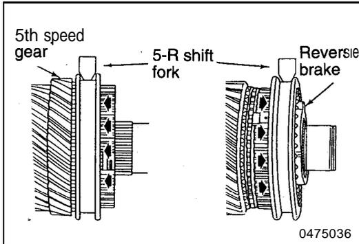
When the 5-R shift fork moves to the front of the transaxle, fifth gear is obtained. When the 5-R shift fork and the reverse shift fork move to the rear of the transaxle, reverse gear is obtained.
