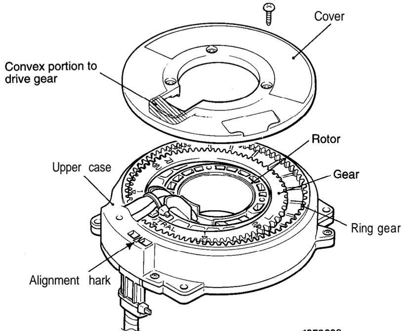
**How the gear operates when the rotor is turned one rotation clockwise**
