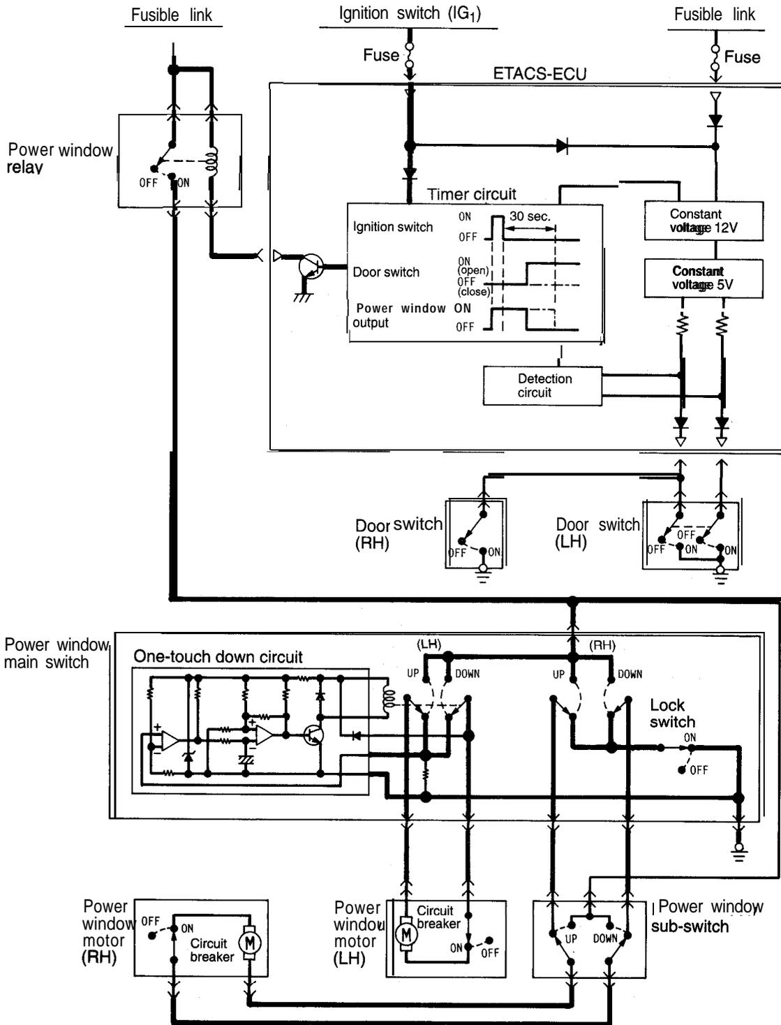
**2. Operation of Power Windows When Controlled by Sub Switches**
