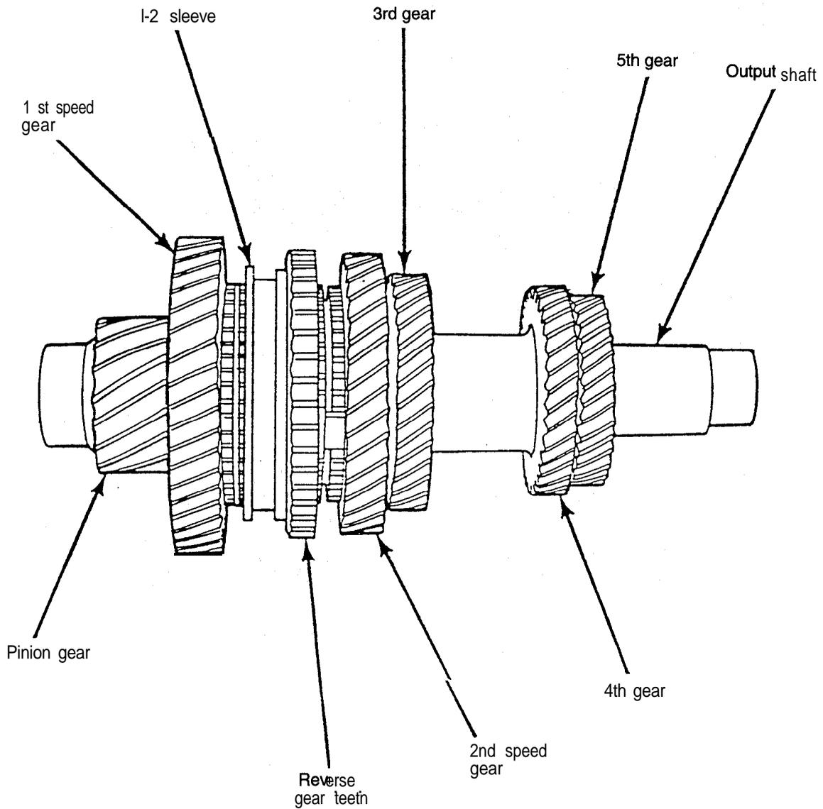
The assembly consists of the output shaft, I-2 synchronizer assembly, first and second speed gears, snap rings and needle bearings. First and second speed gears use caged needle bearings that rotate on the shaft journals. Third, fourth and fifth gears
