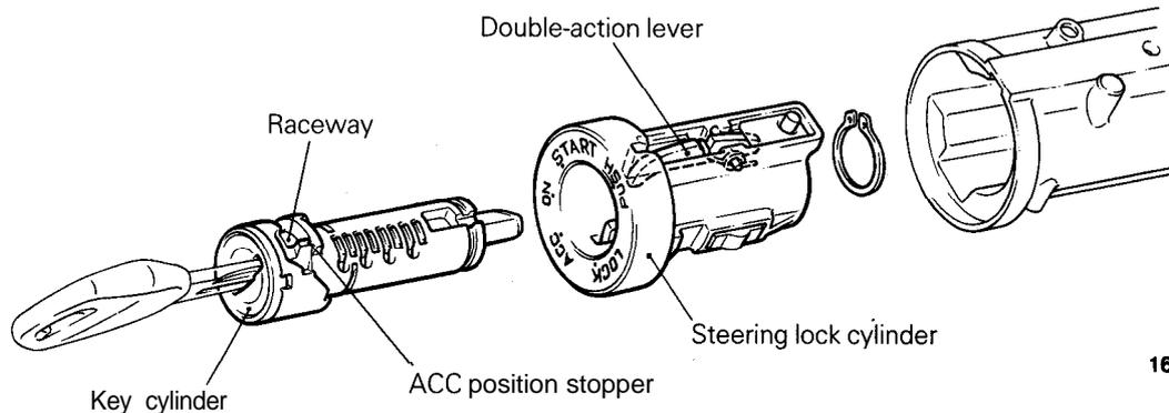
**OPERATION****With the ignition key not pushed in (at the ACC position)**
