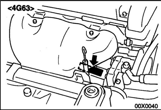
2. The 4G63 engine serial number is stamped near the engine model number, and the serial number cycles, as shown below.
