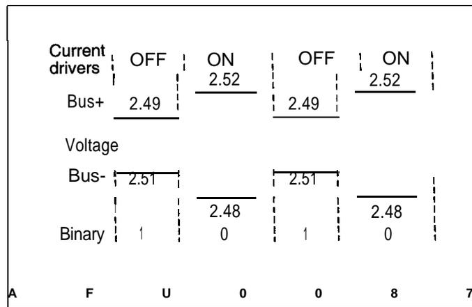
When the bus circuits are not allowing current to flow, there is a “1” condition. When the bus is idle and no messages are being sent, the bus is in the “1” condition.
