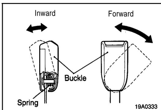
**CONSTRUCTION AND OPERATION OF THE BUCKLE**
