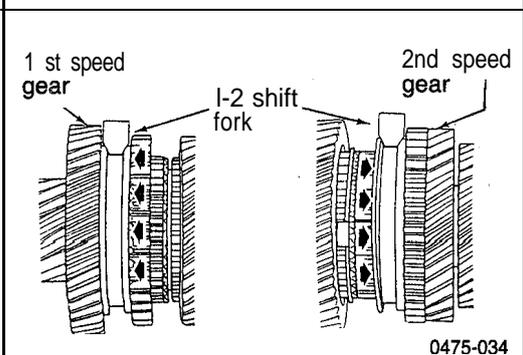
When the 1-2 shift fork moves to the front of the transaxle, first gear is obtained. When it moves to the rear of the transaxle, second gear is obtained.
