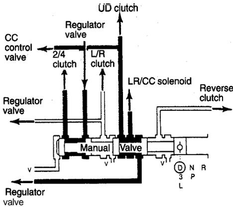
**Low Reverse/Converter Clutch and Overdrive Solenoids**
