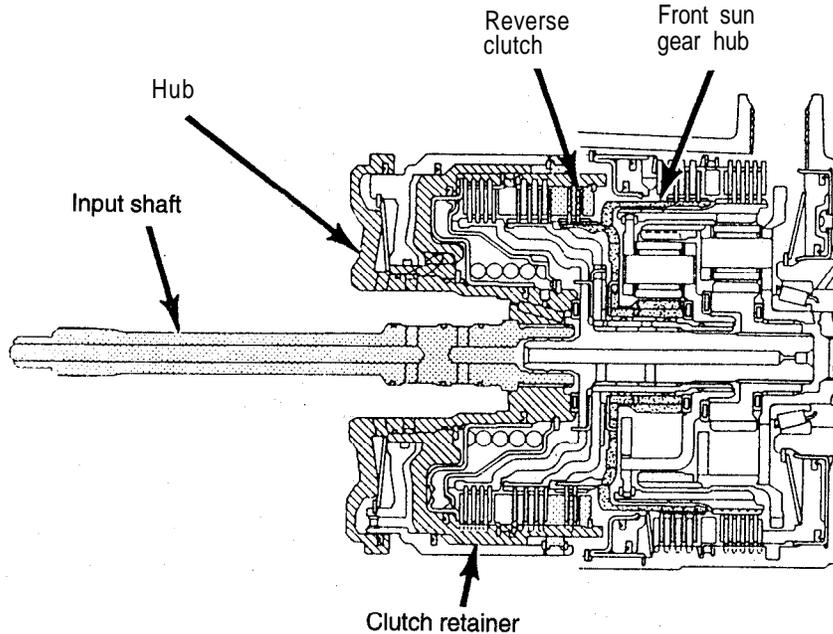
The reverse clutch is located in the back of the input clutch assembly. The reverse clutch is operated by the same piston, pressure plate and belleville spring that operates the overdrive clutch. Line pressure that applies the reverse clutch comes from the valve body, directed through passages in the case, oil pump and reaction shaft support. The line pressure then goes through the input hub to the front side of the OD/REV piston. The pressure
