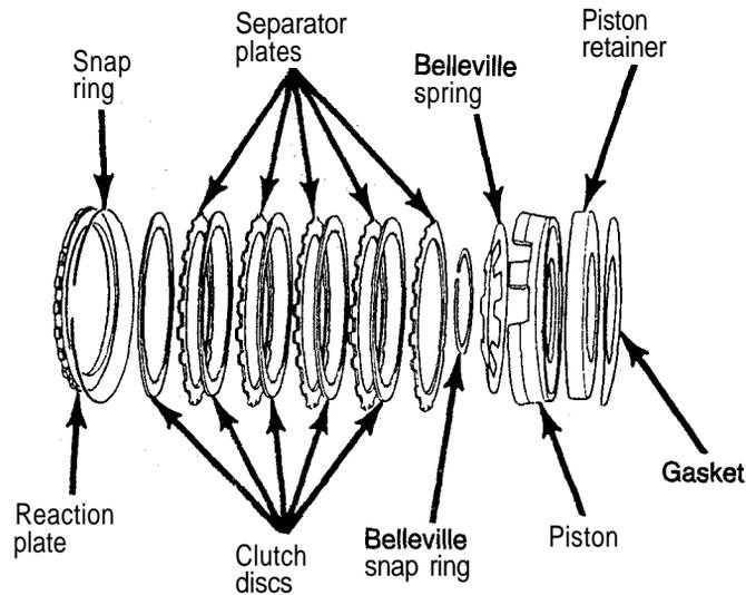
The second clutch, located in the rear of the transaxle case, is the Low Reverse (L/R) clutch. The L/R clutch is located in the very back of the case and, as previously mentioned, shares the reaction plate with the 2-4 clutch. Behind the reaction plate is the clutch pack, belleville spring, L/R piston, and piston retainer. The piston retainer is secured to the case with three screws and sealed with a gasket.
