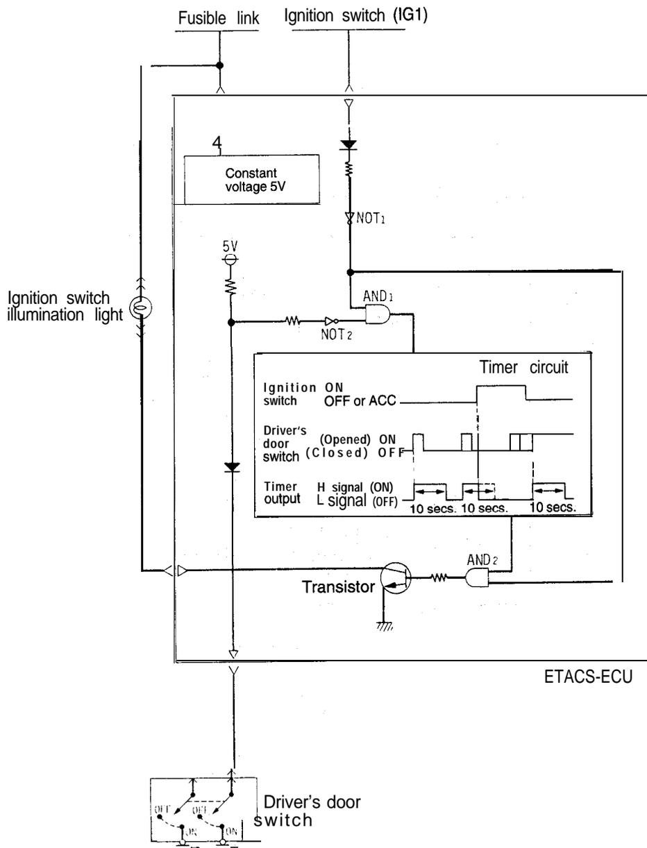
**DOMe LIGHT AND FOOT LIGHT DIMMING TIMER FUNCTION**
