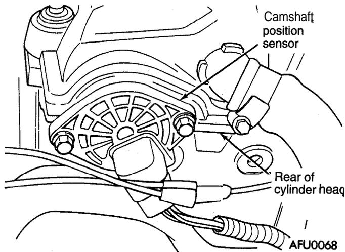
The camshaft position sensor attaches to the rear of the cylinder head. A target magnet attaches to the rear of the camshaft and indexes to the correct position. The target magnet has four different poles arranged in an asymmetrical pattern. As the target magnet rotates, the camshaft position sensor senses the change in polarity. The sensor output
