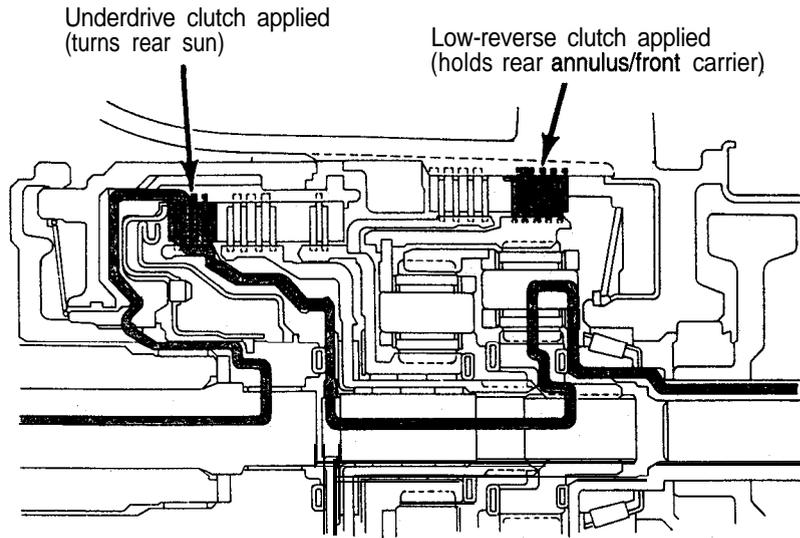
In first gear range, torque input is through the underdrive clutch to the underdrive hub assembly. The underdrive hub is splined to the rear sun gear. When the underdrive clutch is applied, it rotates the underdrive hub and rear sun gear. The L/R clutch is applied to hold the front carrier/rear annulus (ring gear) assembly.
