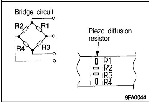
The piezo diffusion resistors, arranged as shown at the left, complete a bridge circuit which constitutes a semiconductor strain gauge. When the sensor is placed under strain by acceleration, the piezoelectric effect changes its electrical resistance, causing the bridge circuit to go out of balance. If a voltage is applied across the bridge circuit, the acceleration can be measured by detecting the amount the bridge circuit goes out of balance in terms of a change in the voltage.
