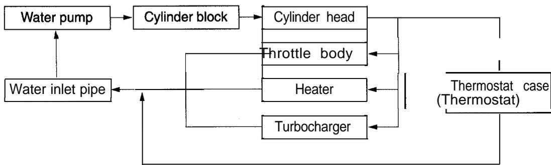
When engine is hot (Thermostat open):
