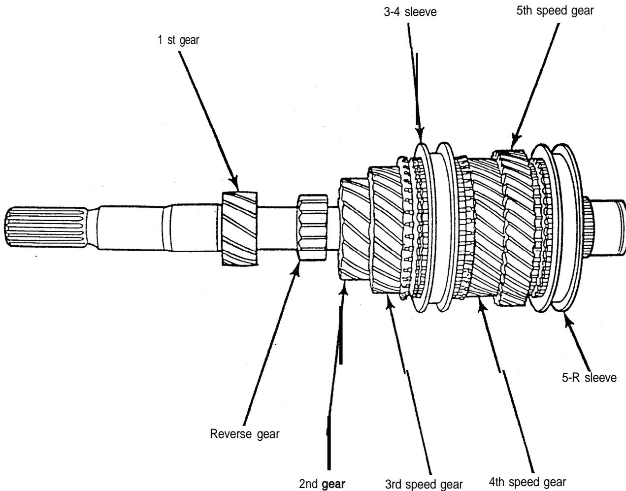
First, second and reverse gears are machined on the shaft. Third, fourth and fifth speed gears ride on caged needle bearings that rotate on the shaft journals. All of the forward gears are helical-type gears, and are in constant mesh with the output
