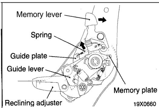
The reclining memory mechanism consists of a memory lever, memory plate, guide plate, guide lever and spring.
