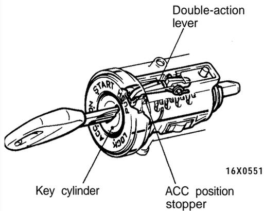
**With the ignition key pushed in (at the ACC position)**
