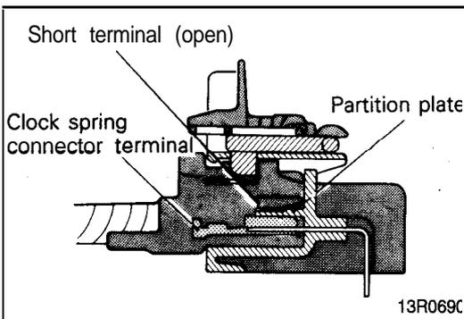
**CONNECTOR SHORTING MECHANISM**
