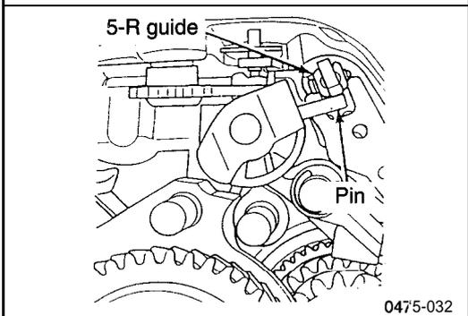
A shift from fifth-to-reverse is blocked by a 5-R guide (guides from 5th to 4th). The shift assembly has a pin sticking out of one side that engages the guide as it comes out of fifth gear. The guide pushes the pin and shift assembly away from reverse gear.
