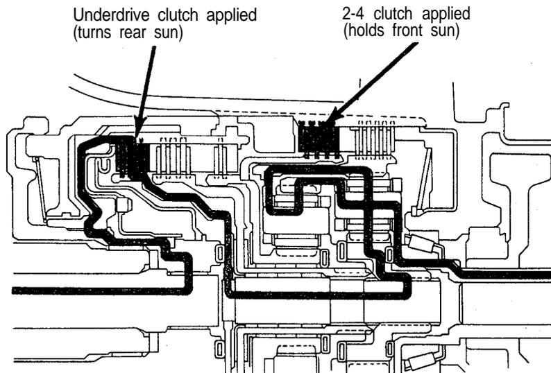
Second gear is achieved by having both planetary gear sets contribute to torque multiplication. As in first gear, torque input is through the underdrive clutch to the rear sun gear. The 2-4 clutch is applied to hold the front sun gear stationary. The rotating rear sun gear turns the rear planetary pinions. The
