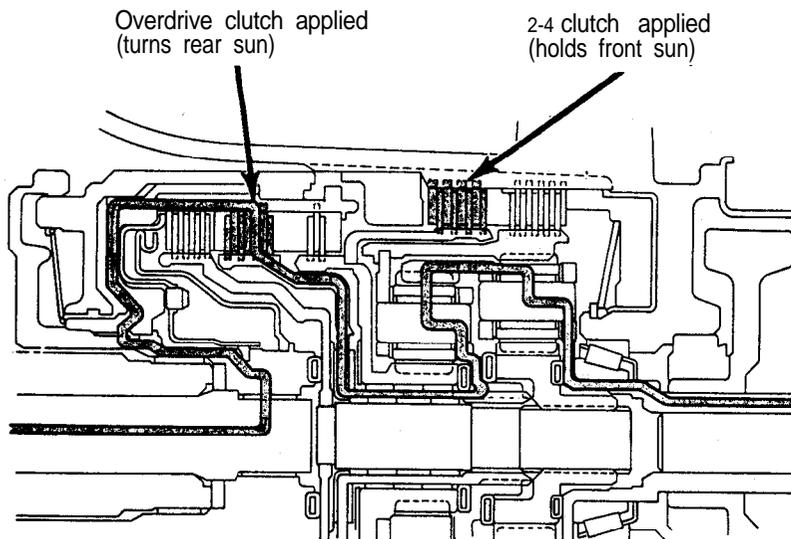
In fourth gear input torque is through the overdrive clutch which drives the front carrier. The 2-4 clutch is applied to hold the front sun gear. As the overdrive clutch rotates the front carrier, it causes the pinions of the front carrier to “walk around” the stationary front sun gear. This causes the front carrier pinions
