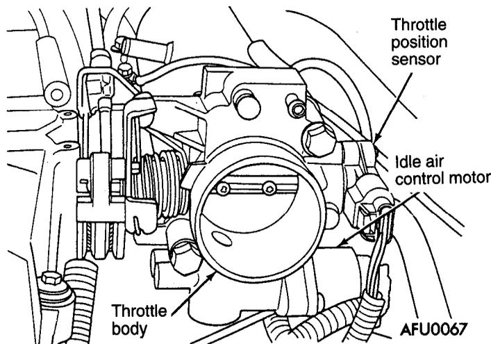
The throttle position sensor (TPS) connects to the throttle blade shaft. The TPS is a variable resistor that provides the powertrain control module (PCM) with an input signal (voltage). The signal represents throttle blade position. As the position of the throttle blade changes, the resistance of the TPS changes.
