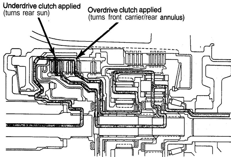
In third gear, two input clutches are applied to provide torque input; the underdrive and overdrive clutches. The underdrive clutch rotates the rear sun gear, while the overdrive clutch rotates the front carrier/rear **annulus** assembly. The result is two compo-
