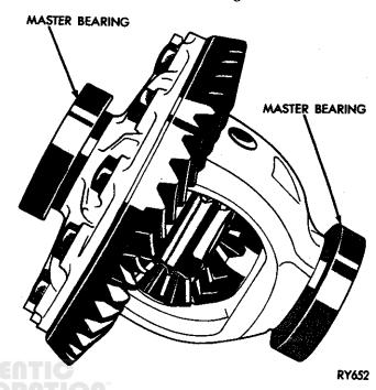
Fig. 28 Master Bearing Tools On Hubs
