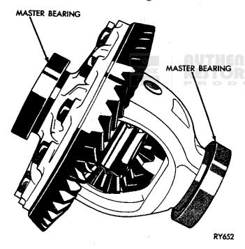
Fig. 41 Master Bearing Tools On Hubs
