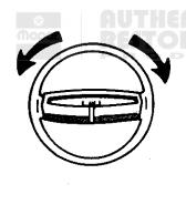
TURN STEERING WHEEL ALL THE WAY LEFT AND RIGHT. RECORD HIGHEST PRESSURE AT EACH STOP.
