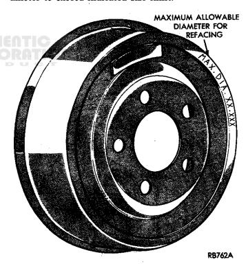
Fig. 9 Location Of Brake Drum Maximum Allowable Diameter
