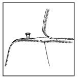
Pull up on the knob located on the top of the seatback on the outboard side to release the seatback. With your other hand, pull the seatback forward.
