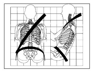
The lap part of the belt should be worn low and snug on the hips, just touching the thighs. In a crash, this applies force to the strong pelvic bones. And you would be less likely to slide under the lap belt. If you slid under it, the belt would apply force at your abdomen. This could cause serious or even fatal injuries.
