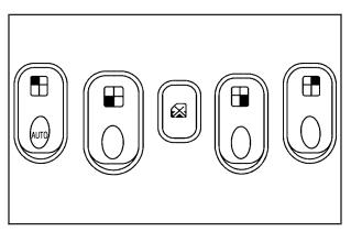
The window switches for all doors are located on the center console. A window switch for each rear window is located on each rear door.
