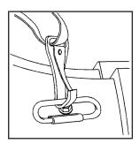
5. Attach the strap to the cargo tie-downs in the rear of the vehicle.
