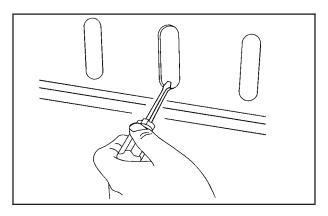
3. Insert a screwdriver, with a minimum four-inch shaft, into the access hole.
