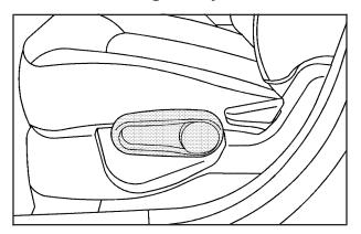
If your vehicle has this feature, the driver's seat height adjuster is located on the outboard side of the seat.
