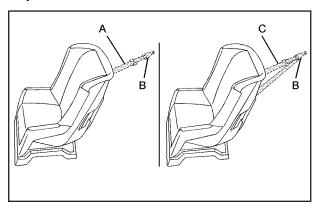
A top tether (A, C) anchors the top of the child restraint to the vehicle. A top tether anchor is built into the vehicle. The top tether attachment (B) on the child restraint connects to the top tether anchor in the vehicle in order to reduce the forward movement and rotation of the child restraint during driving or in a crash.
