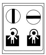
The rear door security locks are located on the inside edge of each rear door. You must open the rear doors to access them.
