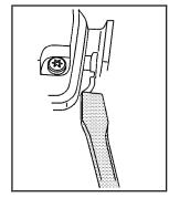
Keep the screwdriver blade horizontal and push the release lever rearward.
