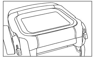
Continue to fold the seat forward until it locks in the folded position. Pull up on the seatback to be sure it is locked.
