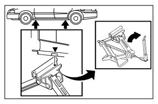
Position the jack and raise the jack lift head to fit over the car flange under the down arrow markings on the rocker panel.
