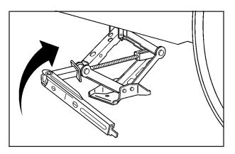
Raise the vehicle by turning the jack handle clockwise. Raise the vehicle far enough off the ground so there is enough room for the compact spare tire to fit underneath the wheel well.
