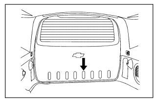
Remove the trim plug, located on the inside of the liftgate near the center, using a flat-bladed tool such as a screwdriver.
