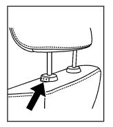
Pull the head restraint up to raise it. To lower the head restraint, press the button, located on the top of the seatback, and push the restraint down. Only the front head restraints are adjustable.
