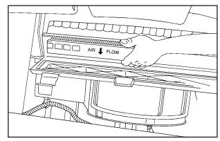
Pull the filter out, keeping it face up so as not to drop any dust into the passenger compartment upon removal.
