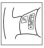
The cruise control buttons are located on the steering wheel.
