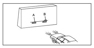
The top edge of the cut-off should be positioned at the bottom edge of the horizontal tape line.
