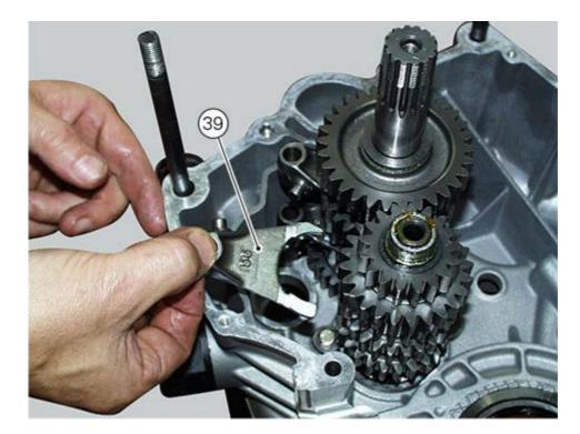
Fit the fork selector drum (40) with the calculated shims on crankcase half.
