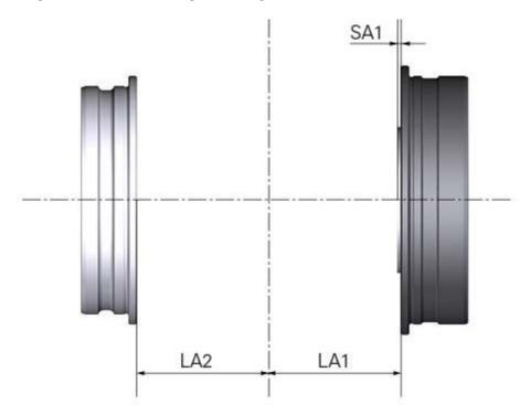
Add a pre-load of 0.30 mm to allow the axial-type bearings of the crankshaft to correctly settle in their seat.
