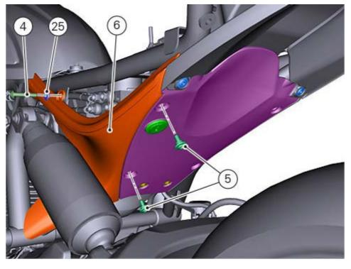
Tighten screw (4) and the two screws (5) to a torque of 8 Nm  $\pm$  10%.
