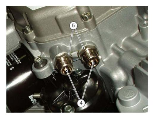
Loosen and remove the oil filter cartridge. Loosen and remove oil filter supporting nipple (6).
