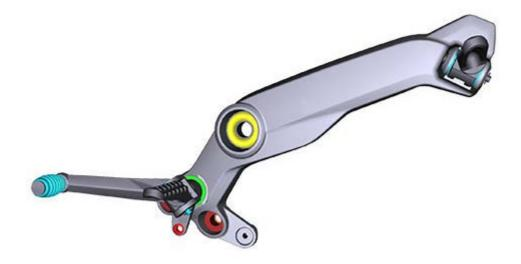
Remove the circlip (8) thereby releasing the pin (9). Slide out pin (9), while supporting the footpeg (10). Slide out footpeg (10) from its seat and collect spring (11).
