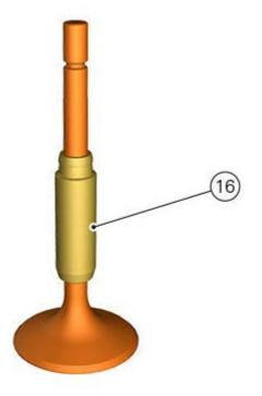
Check for signs of wear, grooves or chrome flaking off. Check the conditions and the diameter of rocker arm bore and shaft:
