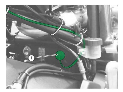
To check the operation of gear sensor (1), connect the DDS 2.
