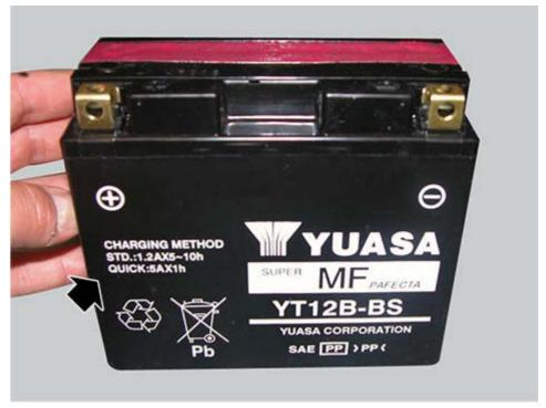
Charge the battery if the open circuit voltage is lower than 12.8 V. Leaving the battery discharged for more than one month could damage it. Check the battery charge with a voltmeter.
