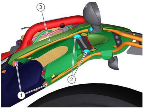
Remove screws (4) that retain the rear mudguard (3) on both sides of the vehicle. Remove the frame/mudguard assembly.
