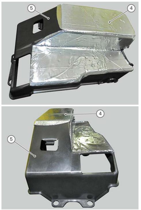
Pay attention to avoid any air bubbles between the heat reflective material and the electrical components compartment.
