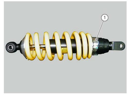
The only possible adjustment on the rear shock absorber is spring preload. Turn adjuster (1) using the suitable wrench to set. Turn adjuster clockwise to decrease spring preload, turn counter clockwise to increase preload.
