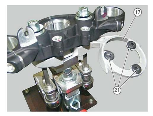
Position handlebar (9) in its seat on the lower U-bolt (17) with the arrows facing the rear side of the vehicle.
