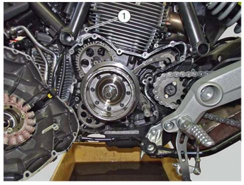
Position 1: the pick-up sensor detects the "full area" (i.e. the tooth); Position 2: the pick-up sensor detects the "empty area" (i.e. the gap between the teeth).
