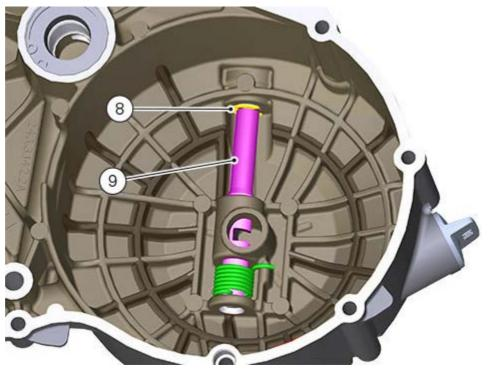
Remove the clutch layshaft (9).
