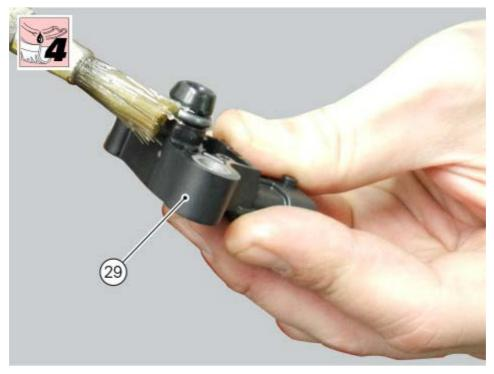
Fit MAP-SENSOR (29) on the support by introducing the pin with O-ring in the support recess and, at the same time, pin in the MAP-SENSOR hole.
