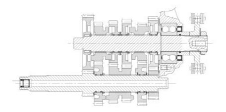
Engage the gears and check that the gearchange mechanism does not stick (selector fork-gear groove, and fork pin-desmodromic drum groove) due to incorrect end float. Restore the correct end float by shimming the gearbox shafts and the selector drum with suitable shims.
