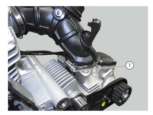
Remove intake manifold.
