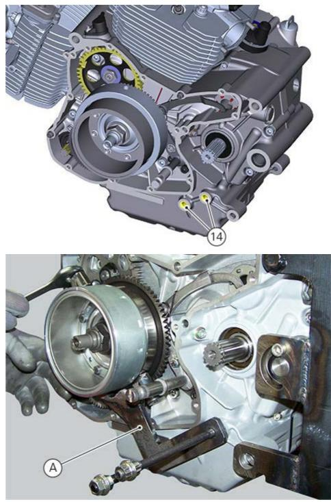
Loosen nut (15) securing the generator flywheel by heating it up with an "industrial heating gun"; we recommend not to use naked-flame heating methods that could damage the starting components.
