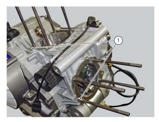
Apply a layer of sealing compound on the gasket (8) contact surface, as required for the vertical cylinder (V) and the horizontal cylinder (O). The sides touching gasket (6) are: Side touching the vertical cylinder.
