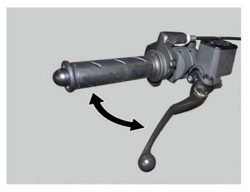
Loosen the bleed value of the calliper (5) and then take the lever through the whole stroke to allow fluid to flow out. The lever is resting against the handgrip.
