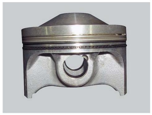
Clean the piston crown and piston ring grooves, removing any carbon deposits. Visually inspect the piston and check its dimensions carefully: there must be no signs of scuffing, scoring, cracks, or other damage. Check the piston diameter.
