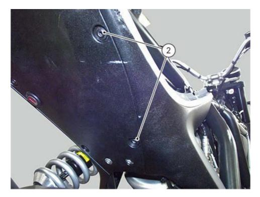
Remove the side body panel by pulling it outwards.
