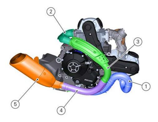
Remove the silencer (Removing the silencer).
