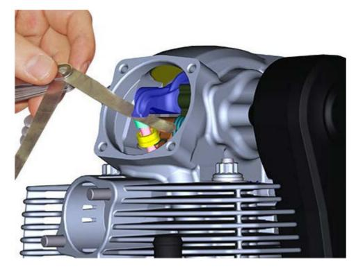
With the valve in the rest position, slide a feeler gauge between closing rocker arm and shim to measure the clearance.
