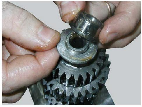
Match gearbox shafts, fit the calculated shims and fit them to the clutch-side crankcase half.
