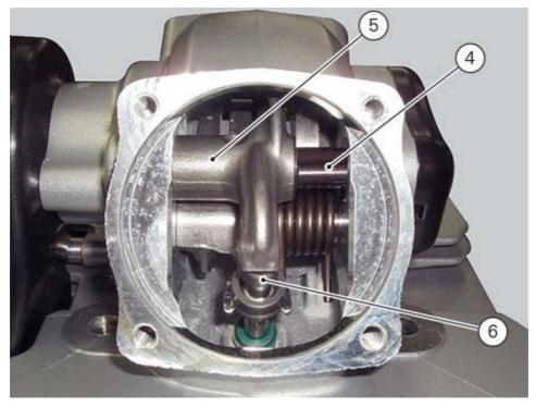
Screw tool no. **88713.2837** on the threaded end of the opening rocker arm shaft (7). Slide out rocker arm shaft (7) and recover opening rocker arm (5) and the two shims (8) and (9).
