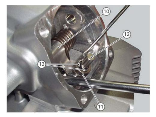
Slide out valve closing shim (11) from the valve (12). Withdraw valve (12) from the lower side of the cylinder head.
