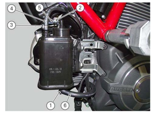
Remove clips (1), (2) and (3) and release hoses (4), (5) and (6) respectively.
