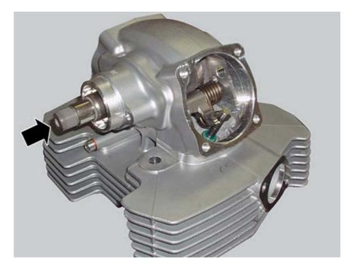
Use a suitable tool to block the closing rocker arm (10) in the position with valve open.
