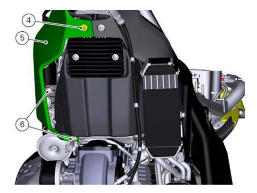
LH cover Loosen the upper screw (4) of the LH airbox cover (7), the lateral and lower screws (8). Remove the LH airbox cover (7).
