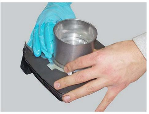
Remove any deposits and degrease the contact surfaces of the crankcase half and the cylinders. Check that pin (1) is installed on the engine block.
