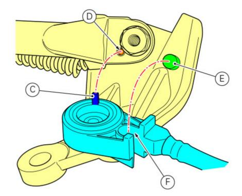
Start and tighten the screw (6) with pre-applied threadlocker to a torque of 5 Nm  $\pm$  10%.
