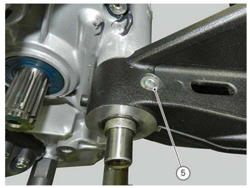
Slide out swingarm shaft (4) from the vehicle LH side. Remove the swinging arm.
