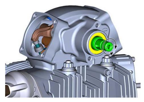
If previously removed, reposition spring (9) of the opening rocker arm (10).
