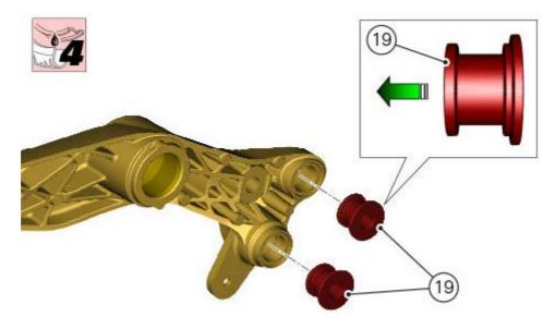
Use a suitable press to fit the silent block (20)
