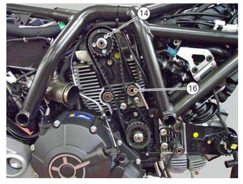
Check proper tensioning using the suitable tool (D) part no. **97900.0253**, frequency reading for proper tensioning is **140** Hz with a new belt. If this value is not reached, work the mobile tensioner (16) until getting the proper reading.
