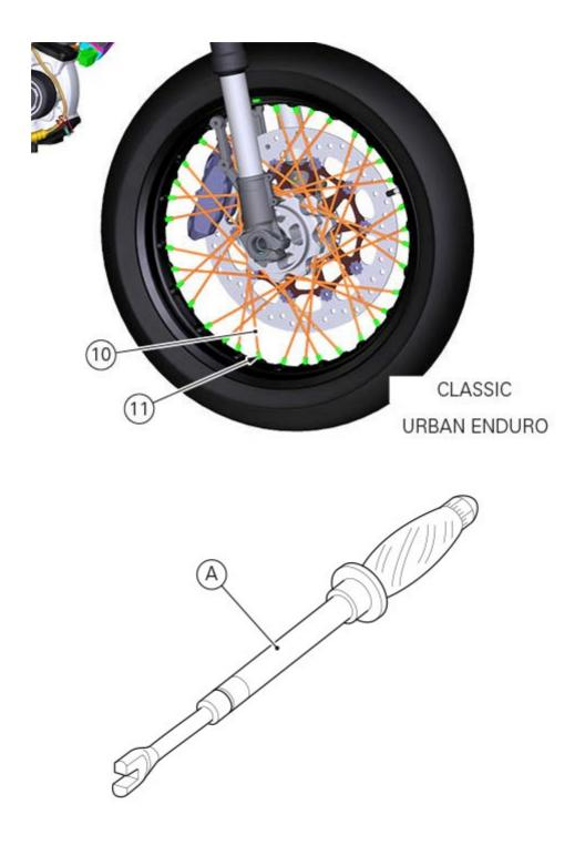
Check that none of spokes (10) emits a hollow sound when hit with a metallic object: this to avoid that seizure or oxidation of spoke and nipple coupling cancels the action of the applied torque; if necessary, restore the correct coupling ensuring not to use products that are aggressive for the wall and the tube.
