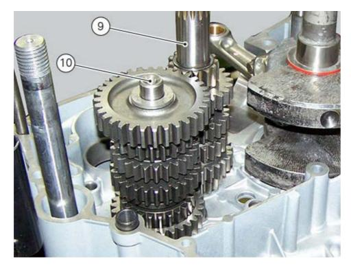
Remove them from the shaft ends and fit them in the relevant bearings on the crankcase half.
