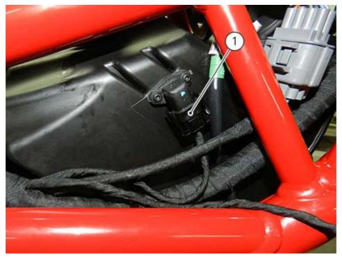
Check the operation of sensor (1) using the DDS 2.
