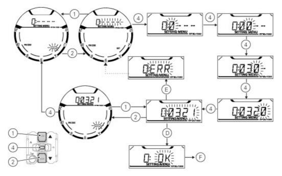
After pressing button (4) to confirm the fourth and last figure, the 4-digit code starts flashing. Press button (4) to check the entered PIN CODE. After you press the button:
