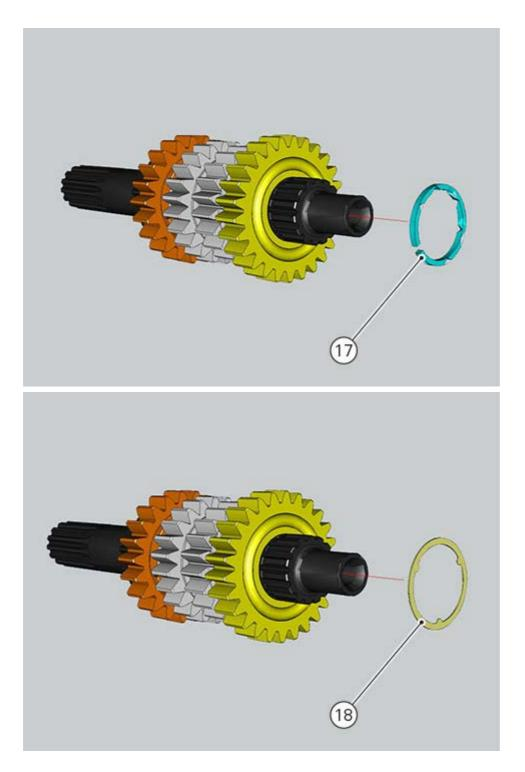
Take care to avoid damaging the surface of the shaft while removing the snap ring.
