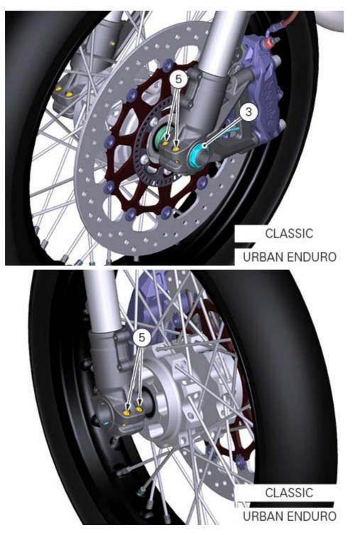
Working from the left-hand side, use a plastic mallet to drive the wheel shaft (6) out from the opposite side and remove it.
