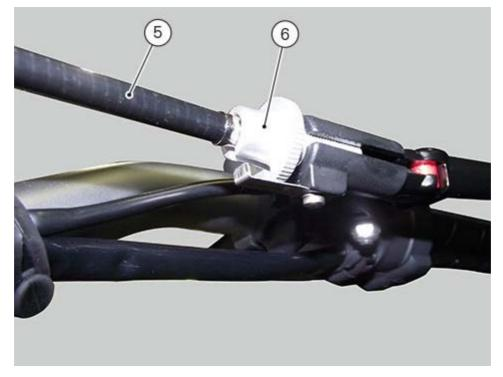
Remove the clutch cable (5) from the clutch cover.
