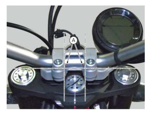
Apply recommended product to screws (7) and tighten to 22 Nm  $\pm$  5% in the 1-2-3-4-3 sequence.
