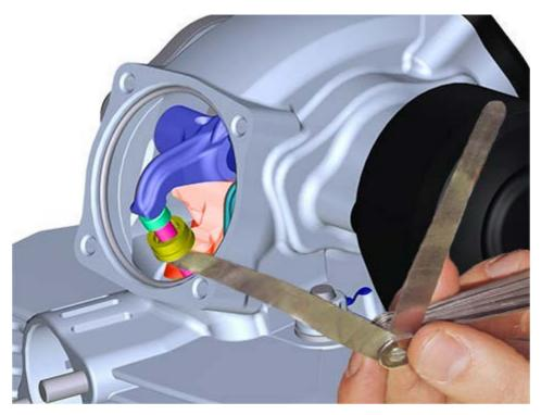
If detected values exceed the specified limits, replace opening and/or closing shims, as described in
