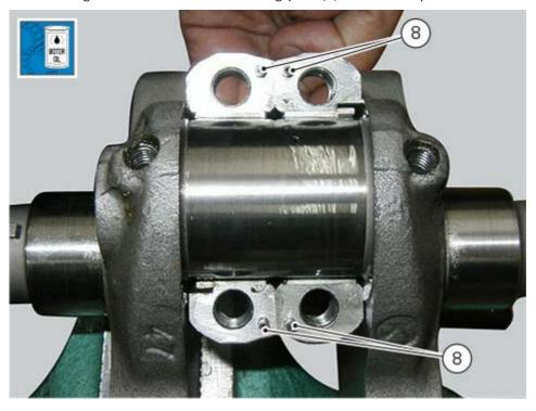
If the crankshaft or one or both con-rods need to be replaced, you must match crankshaft and con-rods according to their weight, as described in the procedure below:
