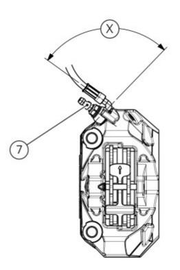
Lubricate the two screws (9) with the recommended product. Fasten calliper (10) by tightening the two screws (9) to a torque of 45 Nm  $\pm$  5%. Tighten screw (7) with seals (8) to a torque of 23 Nm  $\pm$  10%.
