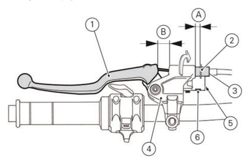
Adjuster (3), located on the lever, allows a maximum adjustment (C) of 11 mm, whereas the standard adjustment (starting one) is of 5 mm.
