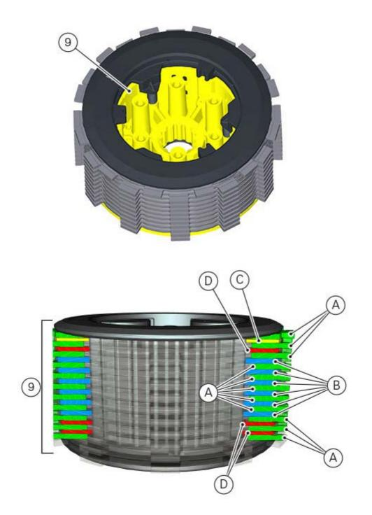
Fit the clutch plate pack with hub inside drum. Fit the two service pins.
