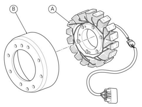
Rotor (B) is manufactured with strong permanent magnets and features a lot of pin pairs for each stator phase. This allows generating alternate voltage at a higher frequency compared to a standard generator. The result: at low rpm it is possible to generate higher current.
