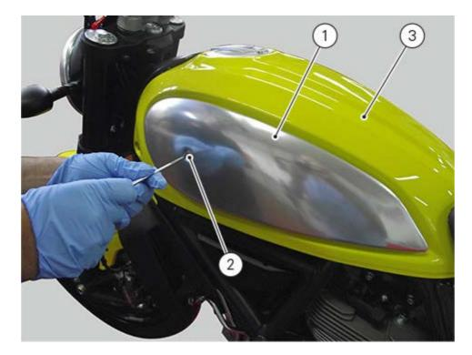
Remove side body panel (1) by sliding it towards the vehicle front side.
