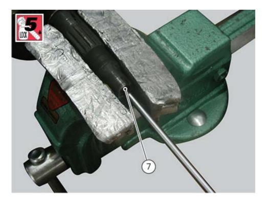
Tighten plugs (5) and (7) to a torque of 13 Nm (Min. 11 Nm - Max. 15 Nm) and plug (6) to a torque of 15 Nm (Min. 13.5 Nm - Max. 16.5 Nm).
