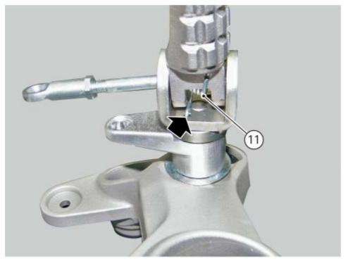
Fit front footpeg (10) in place. Apply the recommended grease to pin (9). Fit pin (9) as shown. Lock shaft using circlip (8).
