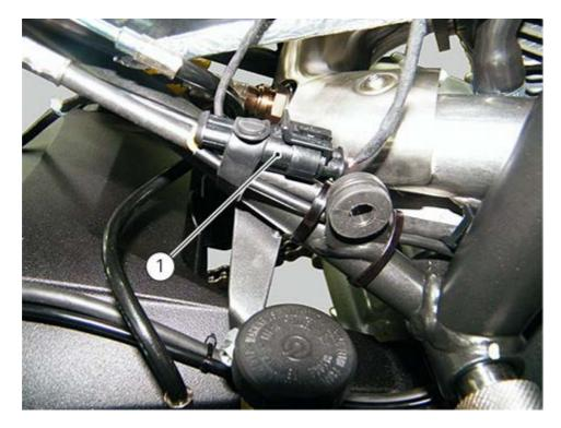
Fill the rear braking system (Changing the rear brake system fluid).
