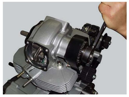
Apply a thin layer of specified grease on the thread and on the underhead of ring nut (8), fit washer (9) and the ring nut.
