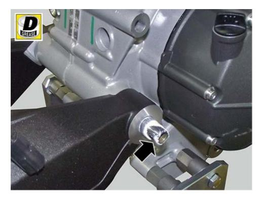
Fit circlip (3) in wheel shaft (4).
