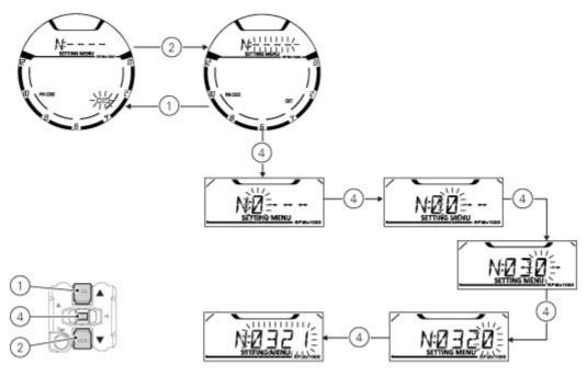
Press button (4) to confirm the fourth and last figure: the 4-digit code starts flashing.
