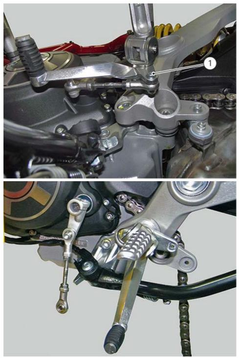
Loosen the screws (2) and (3) retaining footpeg holder to the frame. Undo screw (4) securing footpeg holder to exhaust.
