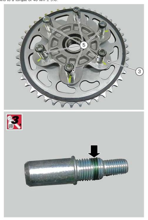
Position rear sprocket (1) on rear sprocket flange (3) and start nuts (2).
