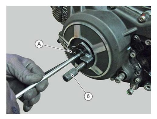
Working on the opposite side, align the reference mark on belt roller (7) with the reference mark on crankcase (8) turning tool (A).
