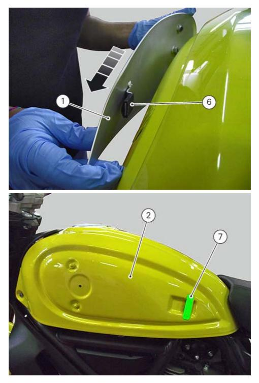
Tighten screw (2) retaining side body panel (1) to tank (3) to a torque of 5 Nm  $\pm$  10%.
