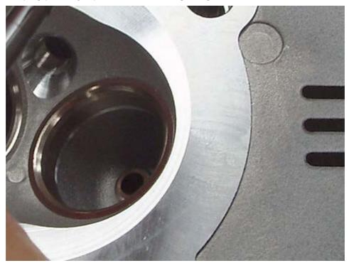
Leave them cool down and grind them, the union of the ducts with the new seats and lap the valves.
