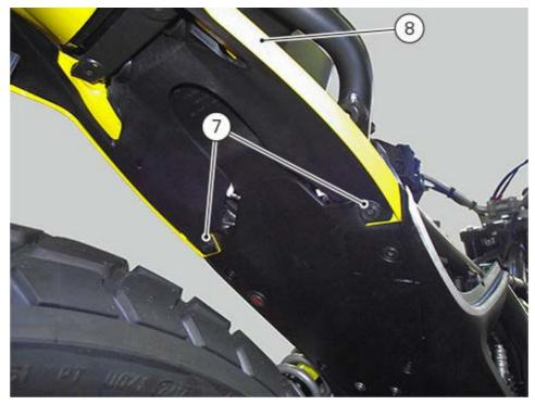
Tighten the screws (9) and (10) to a torque of 5 Nm  $\pm$  10% and the screws (7) to a torque of 8 Nm  $\pm$  10%.
