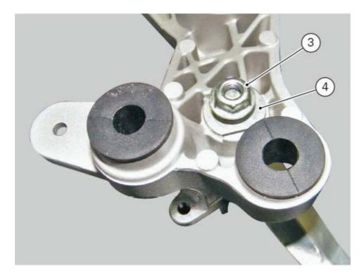
Separate the footpeg/gearchange lever assembly (6) from the footpeg holder (5).
