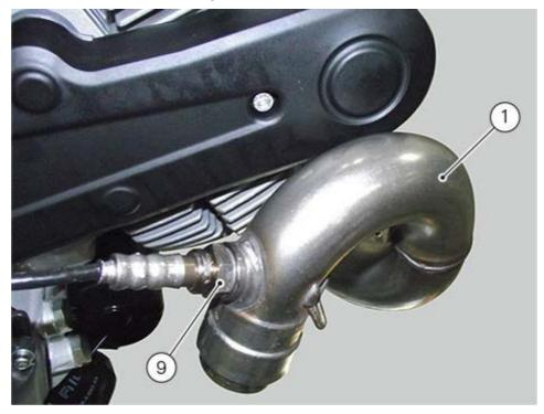
Remove the exhaust manifold (1) from the horizontal head by loosening the two retaining screws (10).
