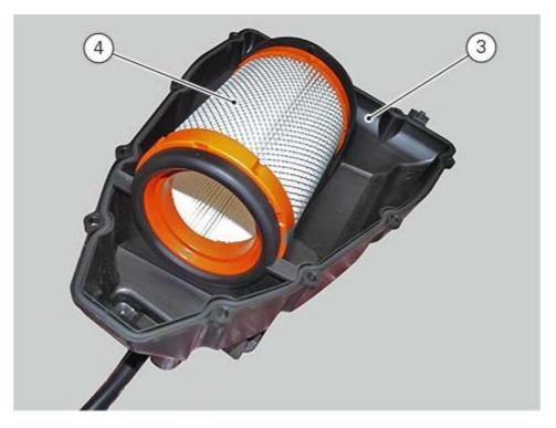
Blow cartridge clean using compressed air or change it.
