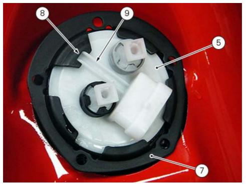
Turn flange (7) and pump (5) assembly by centring flange hole with the holes on the tank. Start screws (2) and tighten them to a torque of 5 Nm  $\pm$  10% respecting the indicated sequence.
