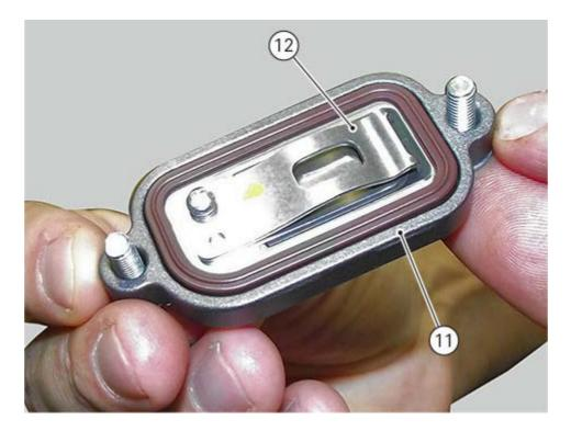
Position the secondary air system cover (11) on the vertical and horizontal cylinder head cover, as shown in the figure. Tighten the screws (17) to a torque of 6 Nm (Min. 5 - Max. 7).
