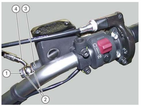
Undo the screws (5) securing the clamp (6), and then remove the front brake master cylinder assembly (3) from the handlebar.
