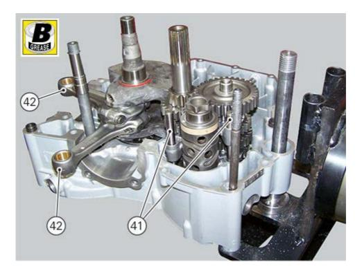
Fit crankshaft with the specially calculated shims inside clutch side crankcase half bearing, positioning connecting rods (42) in the relevant seats of the cylinders. Check that the two centring bushes (43) are correctly fitted.
