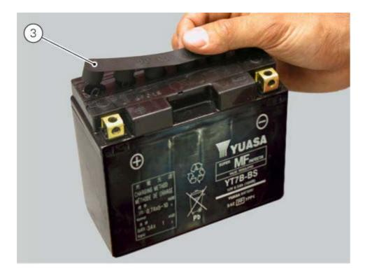
3-12 Ah batteries: leave to stand for at least 30 min.
