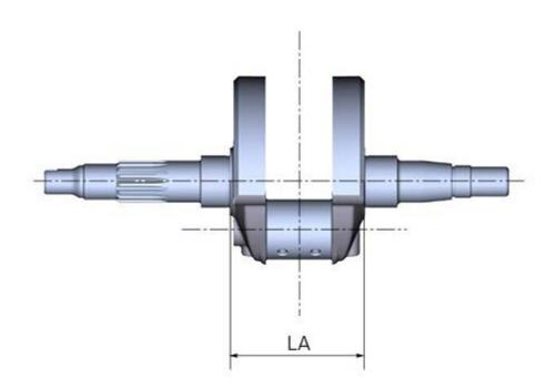
Measure "LA1" and "LA2" corresponding to the distance from the mating surface between the crankcase halves to the mating surface of the bearing inner ring;
