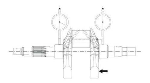
Use a dial gauge to measure the alignment of the main journals by positioning the crankshaft between two
