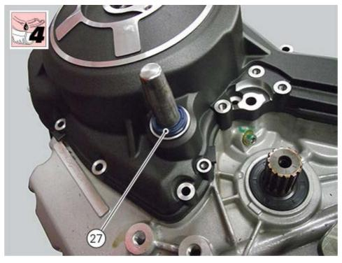
Fit the oil seal fully home with tool (C) no. **88713.3394**. Remove tools (B) and (C).
