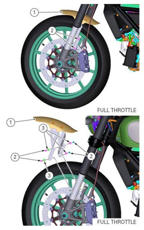
Tighten the four screws (2) to a torque of 8 Nm  $\pm$  10%.
