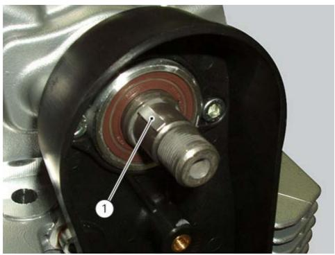
Fit the pulley assembly (10) on the camshaft and push it fully home.
