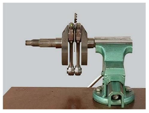
Using a torque wrench as shown in the figure, tighten screws (3) to the values specified here below: tighten to 35 Nm;
