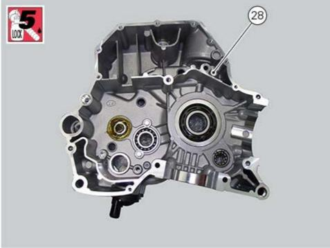
Install the timing layshaft (2) in the roller bearing (29) on the clutch-side crankcase half.
