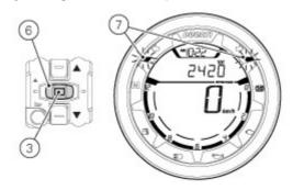
After activating the "Hazard" function, if motorcycle is switched OFF (key set to OFF), the function will stay active until manually disabled by user or it will be automatically disabled after 120 minutes (2 hours) to save battery charge.
