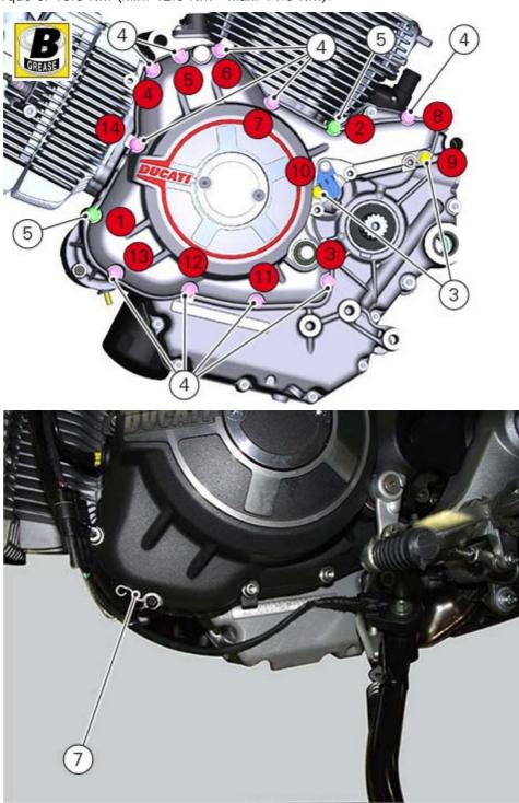
Use tool (B) part no. 88713.3394 on the gearbox driving shaft.
