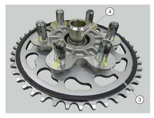
Loosen the nuts retaining the rear sprocket to the rear sprocket flange previously loosened.
