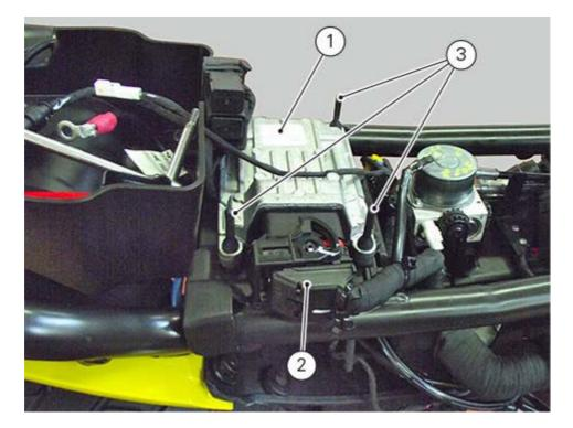
Refit control unit (1) by engaging it on pins (3), ensuring it is properly in seat. Connect connector (2). Refit the seat (Refitting the seat).
