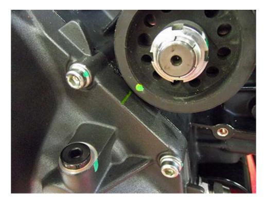
This condition is the TDC in the combustion stage with the horizontal cylinder. Check it by inserting tool (B) in the spark plug hole.
