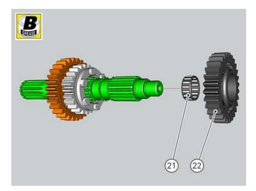
Fit the three-pointed washer (21), which has a bigger outer diameter than the other one (18), in the gear.
