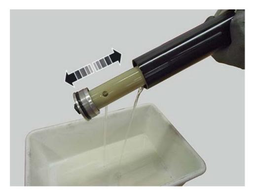
Draining all fluid from the fork is very important. because, due to fork construction and design, it is not possible to measure the air volume from fluid surface to fork edge when filling the fork with fluid.
