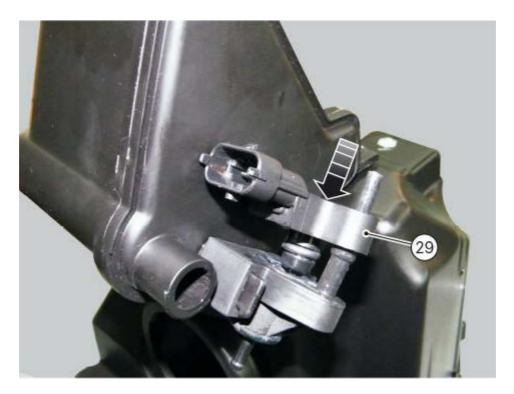
To ensure a correct assembly, pin must be pulled, letting the poppet (30) get completely out on the side opposite to insertion.
