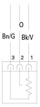
The ignition coil increases the input voltage of the current alternator and brings the voltage to a value that allows the spark creation in the spark plug.
