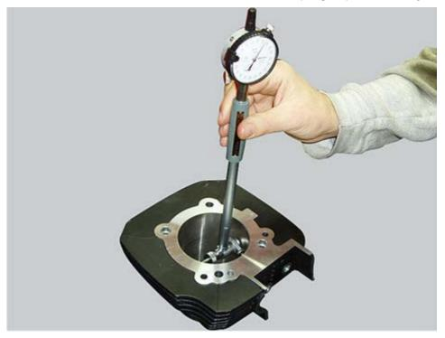
In the event of damage or excessive wear the cylinder must be replaced as it has a silicon carbide coating (which provides the cylinder walls with excellent anti-friction and anti-wear properties) and therefore cannot be ground.
