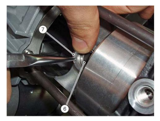
Working from the opposite side, drive out the gudgeon pin (6) sufficiently to release the connecting rod of the crankshaft. Lift the cylinder-piston assembly clear of the engine block stud bolts.
