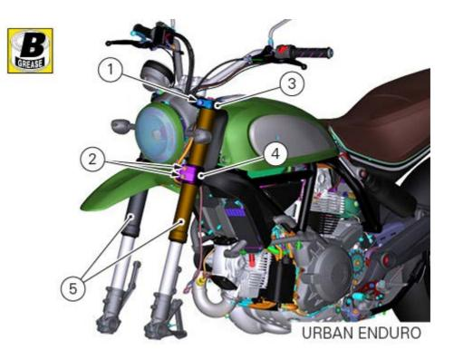
Refit the previously removed components: Front brake calliper (Refitting the front brake system). Front wheel (Refitting the front wheel). Front mudguard (Refitting the front mudguard). (NOT VALID FOR URBAN ENDURO). Headlight. Phonic wheel sensor (Replacing the front phonic wheel).
