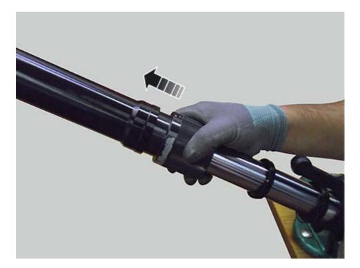
Then, using the same tool, install oil seal (8). Fit snap ring (6) and dust seal (5). Remove the adhesive tape previously applied. Fit the sliding bushing (11) in its housing.
