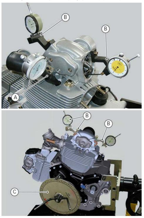
Turn the degree wheel (C) counter clockwise until the gauge dial (B), on the exhaust side, shows a lift of **1** mm. Check that the value of the angular displacement read on the degree wheel (C) is the specified one.
