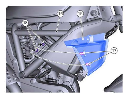
Secure side body panel (1) by tightening screw (2). Repeat this procedure on the vehicle opposite side.
