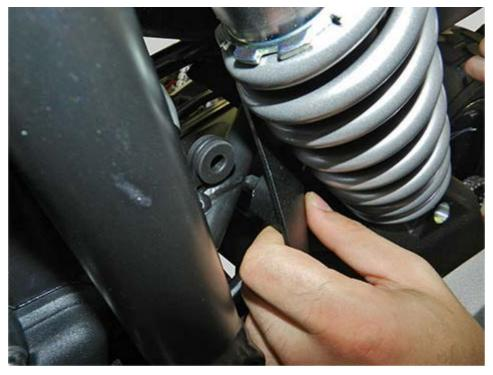
Slide out the side body panel by sliding it first downwards and then towards the rear side so as to release it from the shock absorber.
