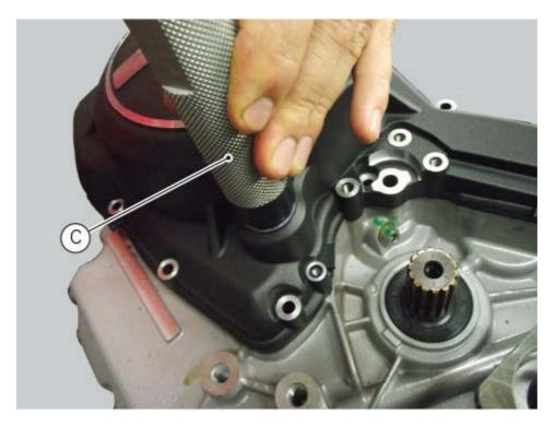
Make sure that the O-ring (28) is installed on the cover (2). Apply grease to the screws (1). Tighten the two fixing screws (1) of the cover (2) matching the crankshaft to a torque of 5 Nm (Min. 4.5 Nm - Max. 5.5 Nm).
