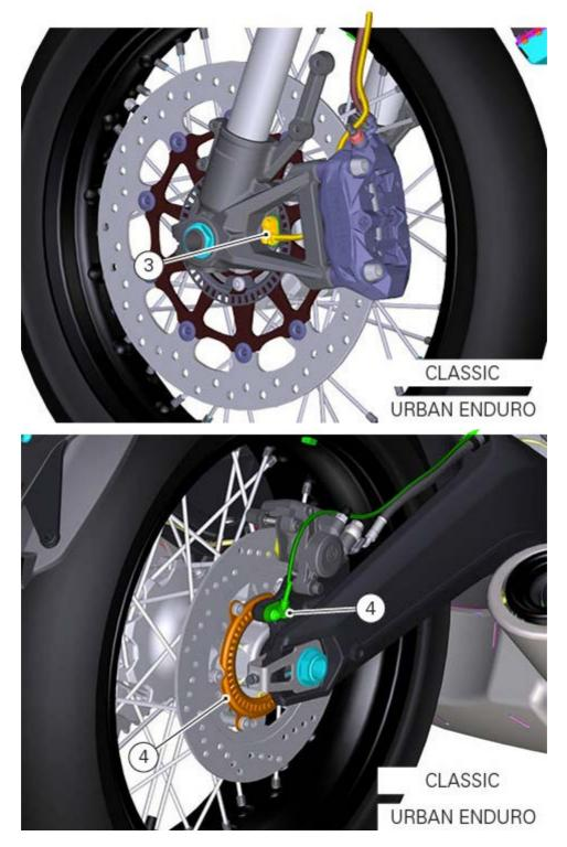
Tighten the sensor securing screw fully home every time you add or remove a shim. Measure the AIR-GAP. Put the required shims.
