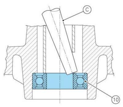
Before fitting new bearings, check that the seat is clean and free from scoring and damage. Grease the bearing seat and then push the new bearing into its seat. Using a tubular drift (D) that only bears on the outer ring of the bearing (10) to drive the latter fully into its seat.
