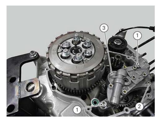
Check the backlash with the front sprocket. Move the gear slightly to measure the backlash; take four readings in opposed positions. The backlash must be 0.10 mm. To take the measurement use a dial gauge.
