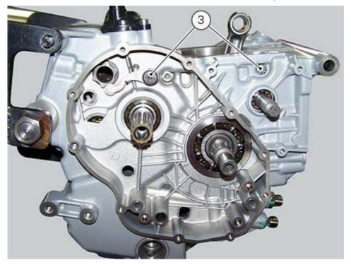
Reuse the generator cover or a service cover with puller (A) part no. **88713.1749** fitted. Secure cover to crankcase half with some of the original screws and begin separation by turning the central pin of the tool. Tap the end of the gearbox secondary shaft with a plastic mallet to separate the crankcase halves.
