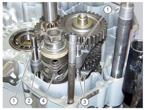
Remove gear selector forks (2) and (3).
