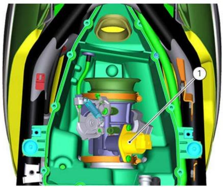
To remove and refit the stepper motor, refer to chapters "Removing the airbox and throttle body" and "Refitting the airbox and throttle body".
