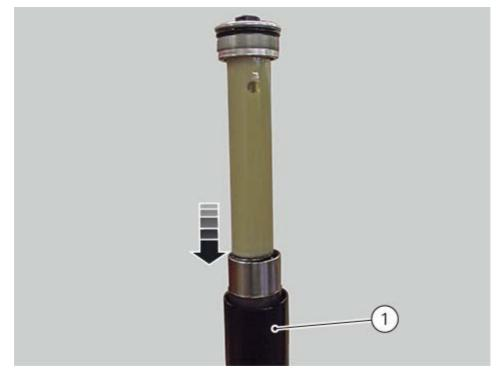
Drain all fluid from the sleeve. To help draining, move damper rod a few times, then leave sleeve upside-down until fluid has completely drained.
