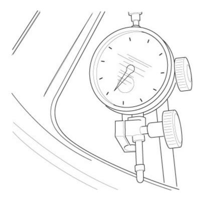
If the values measured are not within the tolerance limits, replace the wheel.
