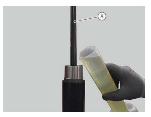
Activate the damper rod a few times. Fit spring (4).
