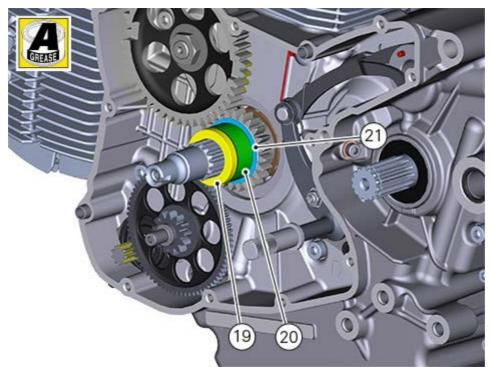
Install the flywheel-rotor-driven gear assembly on the crankshaft ensuring not to move the internal ring (19) in washer (21).
