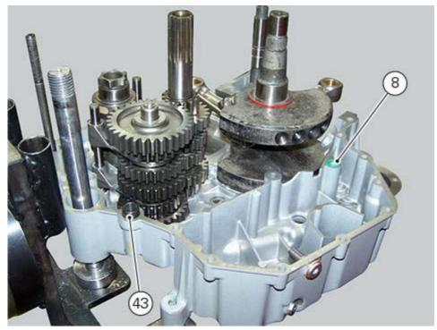
Apply an even and continuous bead of DUCATI sealing compound to the mating surface of the crankcase halves, going around all the holes as shown in the figure.
