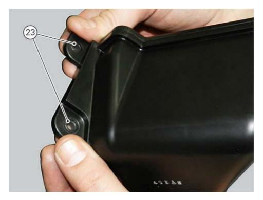
Fit blow-by box (24) fully home on airbox by inserting union in the relevant seat.
