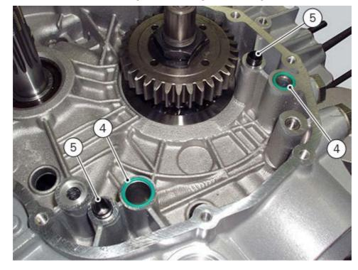
Position the reference bushes (5) and O-rings (4) according to the casing lubrication channels.
