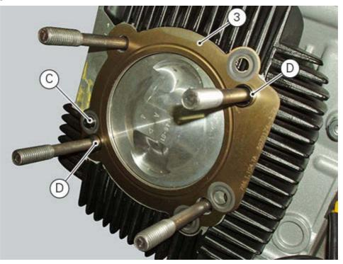
Fit the complete head on the casing stud bolts and bring it fully home on the cylinder.
