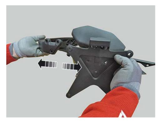
Remove the number plate light (17) by loosening the two screws (16).
