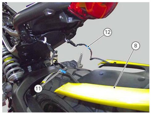
Position tail guard (8) on the frame and start the two screws (9) and (10). Make sure that washers (18) are present on the screws.
