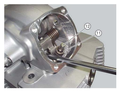
Position the two split rings (13) on the valve stem. Remove the screwdriver and position the closing rocker arm (10) in its rest position.
