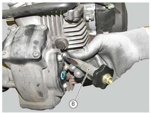
Now tool (A) pin (6) should be aligned with one of the two holes (5) on generator casing. Tighten pin (6) so as to lock out tool (A) rotation.
