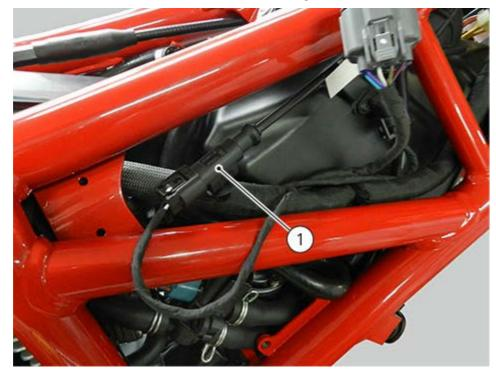
Disconnect front ABS sensor (2) connector (1) from main wiring.
