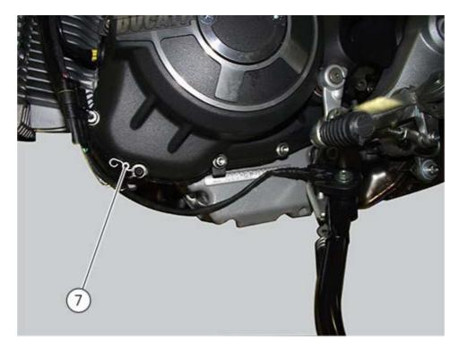
Use tool (A) no. 88713.1749 to the holes of the just-removed screws (1) and remove the cover.
