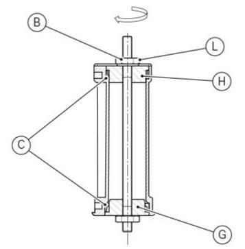
steering shaft after heating it for about 10 minutes to 120 °C. Insert drift no. **88713.1072**. Push the inner ring (7) on dust seal (8), manually pushing for at least 10-15 seconds.
