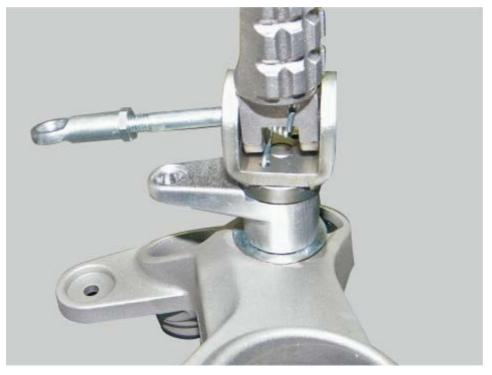
Loosen screw (7) and separate the gearbox rod (2) from the gearbox pedal (8).
