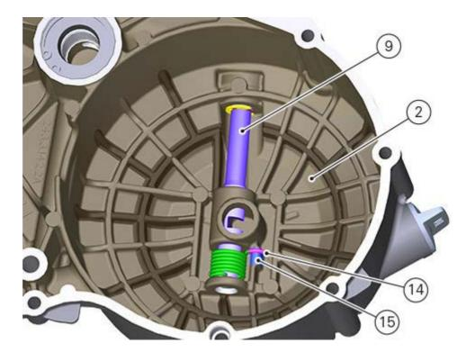
Fit snap ring (8) on pin (9) and perform a functional test.
