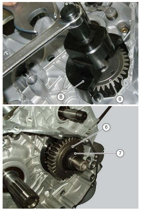
Refit the oil pump and check the backlash between the oil pump gear and the primary drive gear on the crankshaft.
