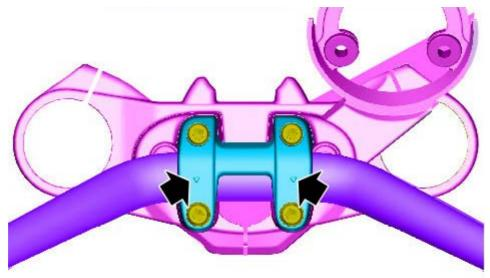
Reference points (A) on handlebar must be at the same distance from U-bolt (8) and flush with the U-bolt surface.
