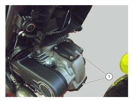
Fit tool part no. **88713.011** and ensure the two tool pins match the two slots on crankcase following the same procedure as for "Changing the belts". Turn the crankshaft so that the value to be inspected is in rest position.
