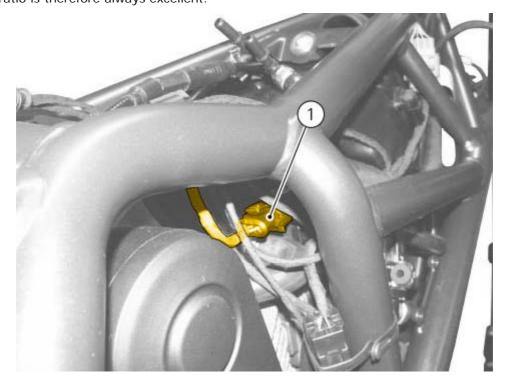
Check the correct operation of MAP sensor (1) using the DDS 2.
