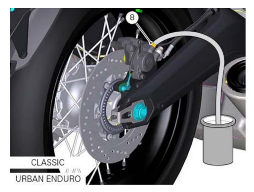
Siphon the fluid from the reservoir (6). Fill the reservoir (7) with new oil up to the MAX mark.
