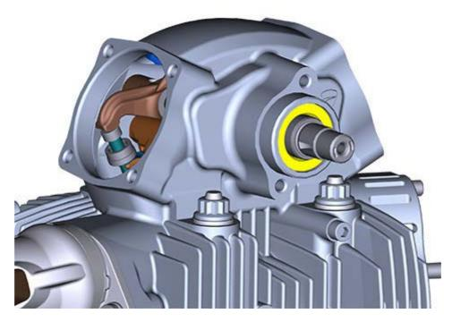
Rotate camshaft to evenly lubricate contact areas.
