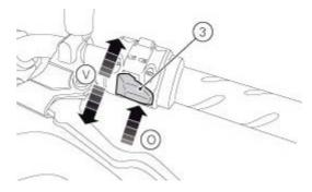
The low beam lights are turned on the first time it is pressed; from this moment, the same button can be used to switch on (and off) the high beam light: if the engine is not started within 60 seconds, the low beam and high beam that were turned on will turn off. If the headlight was turned on before starting the engine with the procedure described above, the headlight will turn off automatically when starting the vehicle and will turn ON again when the engine has been completely started.
