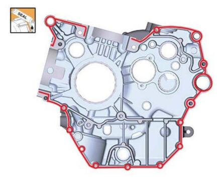
Bring the crankcase halves (44) and (45) together, tapping with a rubber mallet in the area of the shafts if necessary.
