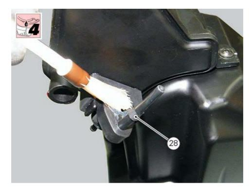
Lubricate MAP-SENSOR seal (29) using the specified product.
