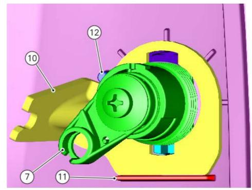
Fit lock (7) by tightening nut (6) to a torque of 3 Nm  $\pm$  10%.
