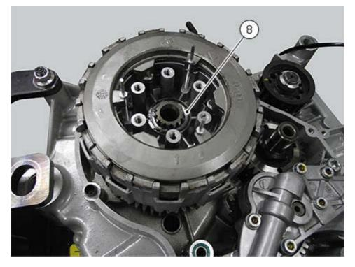
Slide the hub-plates-drum assy (9) out of clutch housing (10), marking them so as to refit them in the same position in which they were removed.
