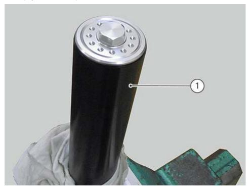
Apply some adhesive tape on the hexagon flat to prevent any damage. Slacken the top plug (2).
