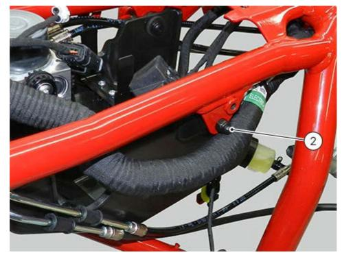
Working on the vehicle left side, loosen nut (3) and remove the screw from the internal side.
