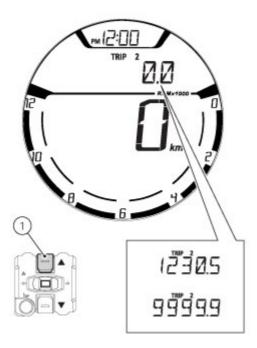
The trip meter counts and displays the partial distance covered by the motorcycle with the set unit of measurement (km or mi).
