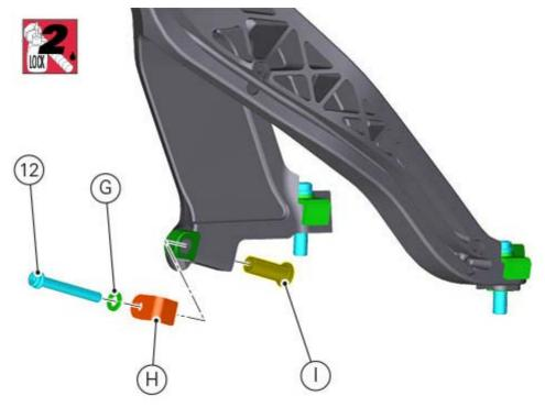
Position the number plate holder subframe on the swinging arm by starting the screw by hand without tightening to torque.
