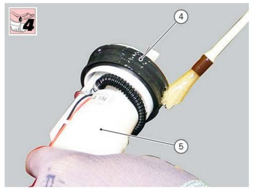
Insert the pump unit (5) in the tank seat (6) as shown in the picture.
