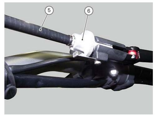
Reposition cable (5) on the clutch cover.
