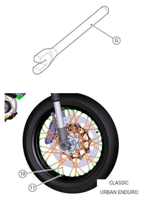
In case of axial runout, tension the spokes on the side featuring a value increase and loosen those on the opposite side. Always work on several spokes, at least on two spokes per side, by letting them perform small rotations between one check and the following one. In case of radial runout, loosen the rim spokes featuring a value increase and tension those on the opposite
