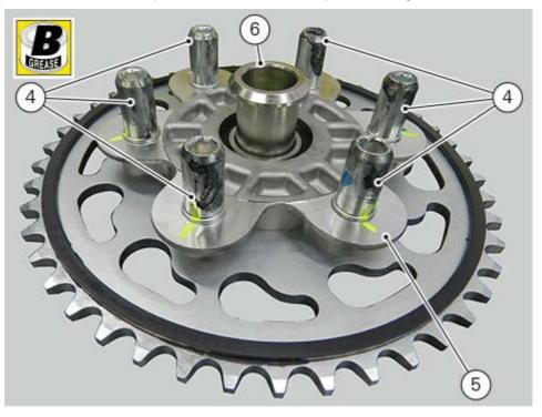
Place rear sprocket flange (5) with spacer (6) inside vibration damping pads (7).
