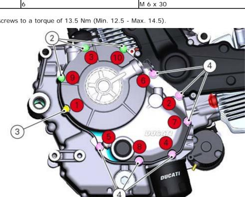
Tighten the screws to a torque of 13.5 Nm (Min. 12.5 - Max. 14.5).
