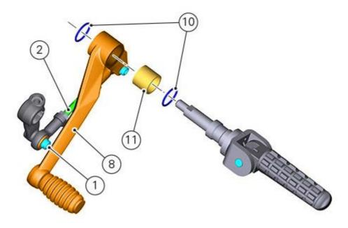
If the bush (11) inside the pedal (8) needs to be replaced, grease the external surface and drive the bush into place using a press. The bush must be seated 2 mm below the outer face of the pedal.
