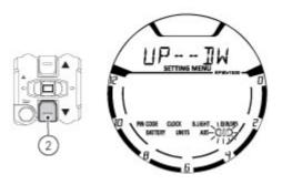
For safety reasons, the setting menu can be accessed only when vehicle speed is below or equal to 20 Km/h; if this menu is accessed and vehicle speed is above 20 Km/h, the instrument panel will automatically quit it and shift back to main screen.
