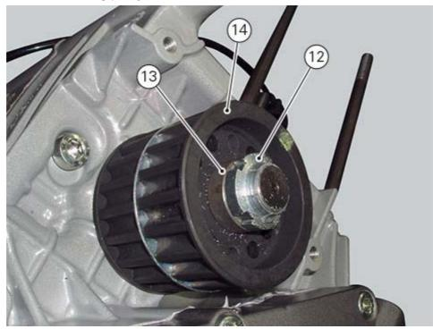
Block with the key of tool (A) no. **88700.5644** the pulley rotation and use the bush inserted in a torque wrench to tighten the self-locking ring nut to a torque of 71 Nm (Min. 64 Nm - Max. 78 Nm).
