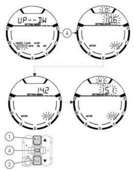
If the instrument panel is not receiving battery voltage value, a string of three dashes "- - -" is displayed. To quit the menu and go back to Setting Menu main page, select EXIT and press button (4).
