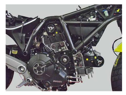
Fit belt (14) and tension it by hand using the mobile belt tensioner (16).
