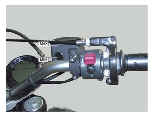
Remove the reservoir cover (5) by loosening the two screws (6). Remove reservoir inner membrane. Top up with recommended fluid up to maximum level. Refit the removed components.
