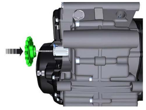
Insert stop plate (4) on the gearbox secondary shaft (5) and rotate it inside groove (7) until the plate holes match the sprocket threaded holes: orient the stop plate with the rounded edge facing the sprocket. Apply threadlocker on screw threading (3). Engage the first gear.
