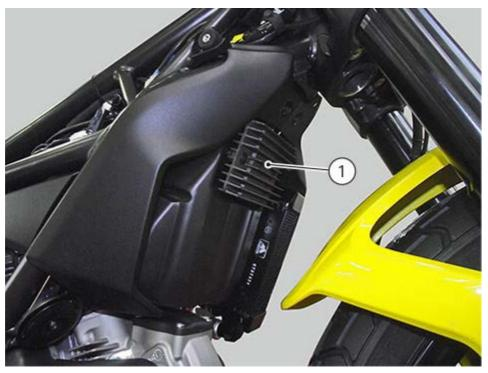
The rectifier/regulator consists of an aluminium casing containing the diodes that rectify the current produced by the generator. It also contains an electronic device that regulates the current supplied by the generator in accordance with battery voltage.
