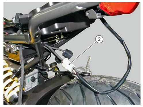
Loosen the two retaining screws (3) and remove the tail light (4).
