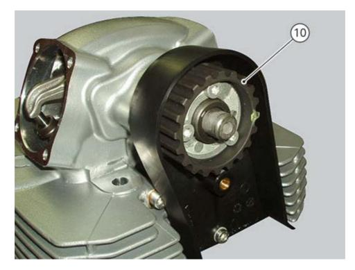
Insert tool 88713.3152 in the pulleys to block its rotation.
