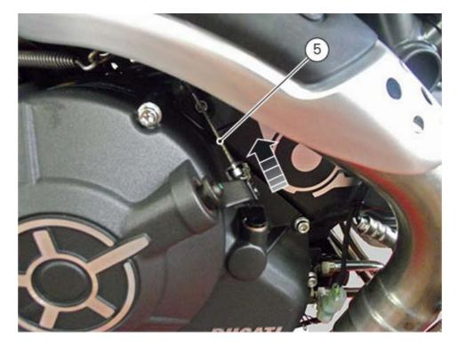
Working on clutch cover lever, slowly remove cover to release it from clutch control pin.
