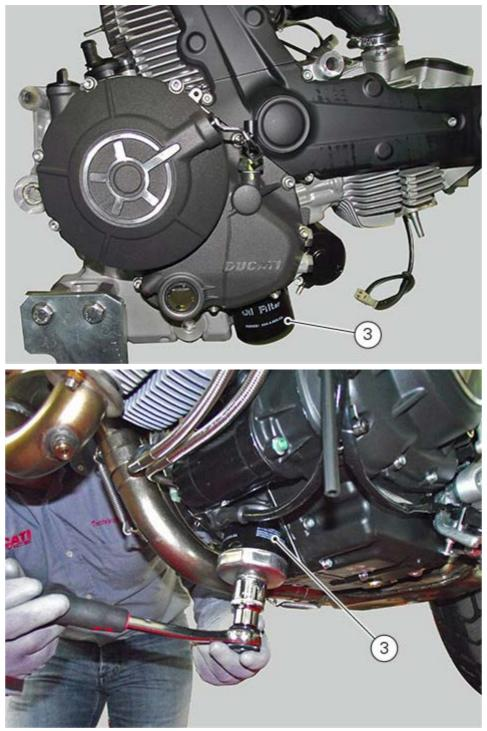
Screw it into relevant seat and tighten it to 11 Nm (Min. 10 Nm - Max. 12 Nm).
