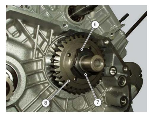
Lock the primary drive gear (8) with holding tool (A) no. **88713.2423** and loosen sprocket threaded ring nut (7).
