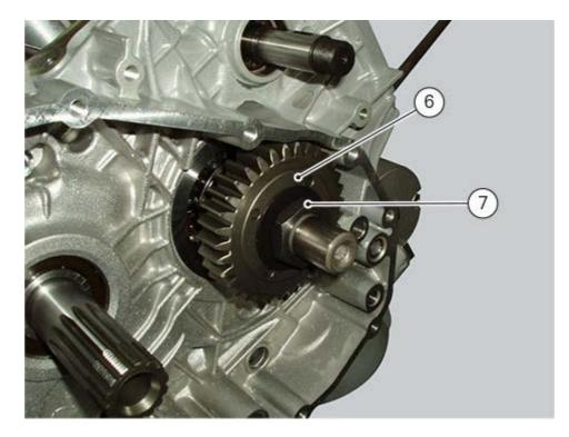
Remove the primary drive driving gear (8) using puller (B) no. **88713.2092** and place between crankshaft and puller screw an aluminium or brass pad.
