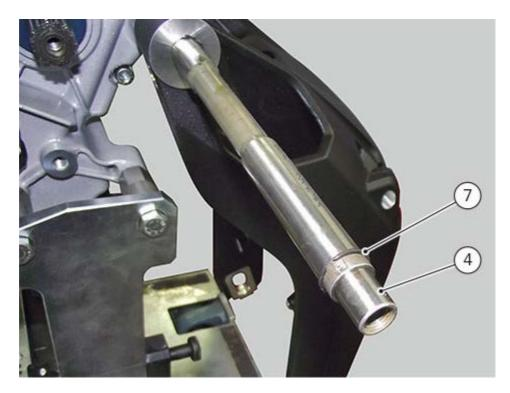
Bring the swinging arm seat close to the seat on the crankcase. Insert pin (4) fully home.
