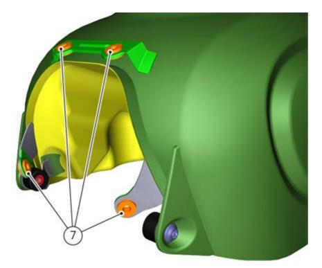
Fit the tank cover (6) by pulling it inwards to engage pins (4) in fixing points (5).
