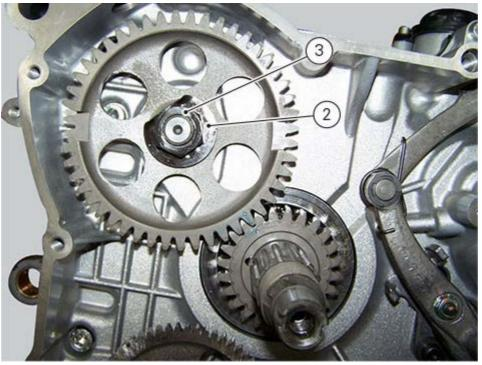
Slide out nut (3), washer (2) and driven timing gear (4).
