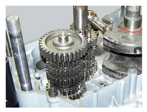
Insert the forks of 1st - 4th and 2nd - 3rd speed (38) inside the sliding grooves of the secondary shaft driven gears.
