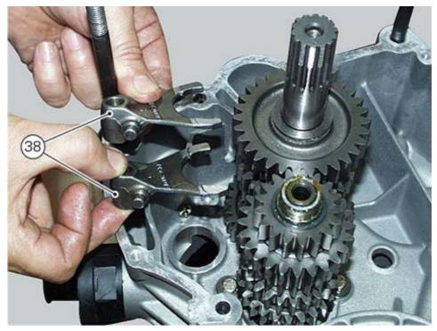
Insert the fork of 5th - 6th speed (39) inside the primary shaft driven gear.
