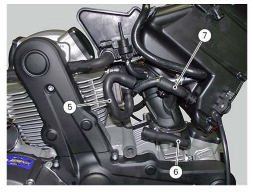
Connect the secondary air system sensor to the vertical head through hose (5); repeat the operation with the horizontal cylinder head hose (6) and hose (7) coming from the airbox. Fix the three hoses with clips (4). Connect the secondary air sensor connector (3).
