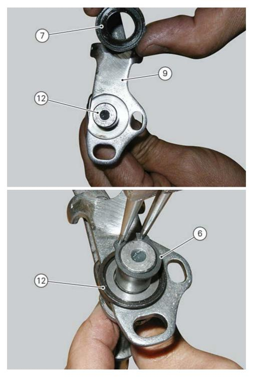
Position lever (12) correctly according to the plate (9) position. The lever pin must be equidistant from the plate edges; to modify its position, work on the suitable eccentric pin (11) after loosening lock nut (13).
