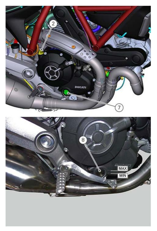
Check that there are no oil leaks and that the relevant warning light on the instrument panel switches off a few seconds after starting up the engine. If not, stop the engine and trace the fault. After a few minutes, check that the oil level is the specified one; if necessary, restore the MAX. level (8).
