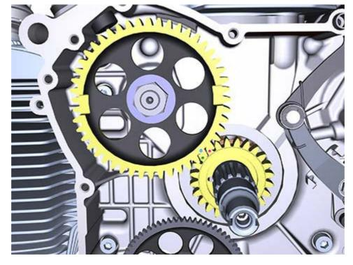
On completion of the refitting operations, check that washer (2) is staked against nut (3) in such a way to prevent the nut from working loose.
