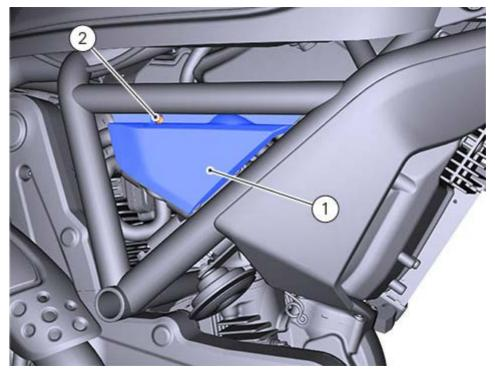
Remove the side body panels (Fitting the airbox cover). Remove the fuel tank (Refitting the fuel tank). Remove the seat (Refitting the seat).
