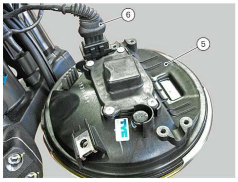
Fit headlight (5) by matching seats (A) with the two pins (6) on the headlight support subframe (7).
