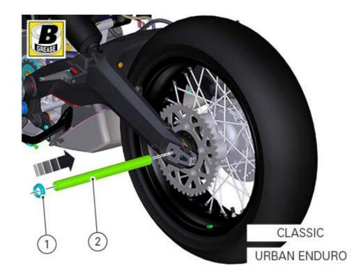
Before tightening nut (1) keep the chain tensioned (Adjusting the chain tension).
