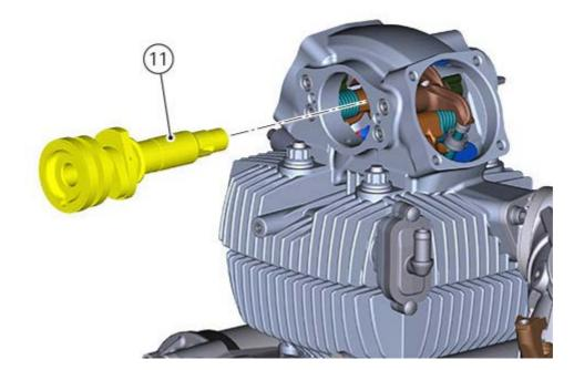
While fitting the camshaft, pay attention not to damage the seal.
