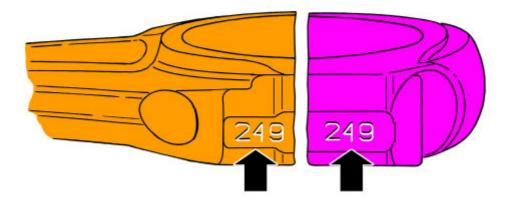
Couple crankshaft and connecting rod big end bearings following the indications provided in the table.
