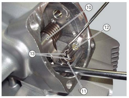
Use a suitable tool to compress the spring as much as possible while holding valve, shim and split rings in the valve closed position. Release the closing rocker arm (10) with a quick movement, so that the split rings seat in the shim.
