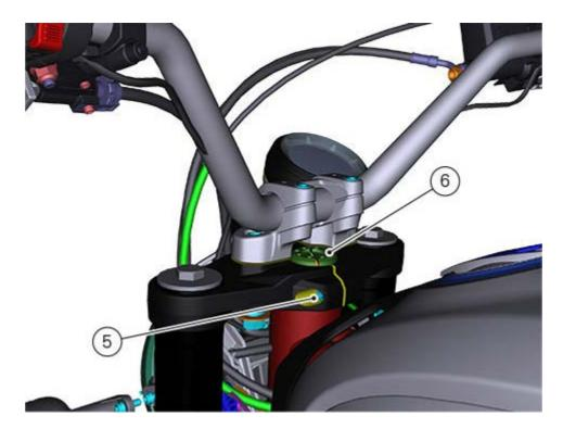
Tighten screws (4) and (5) previously loosened to a torque of 24 Nm  $\pm$  5%.
