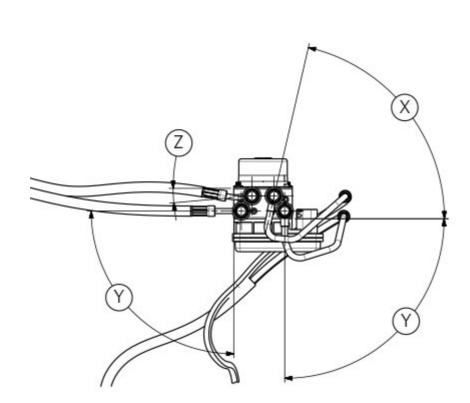
Hoses (3), (4), (5) and (6) must be secured in place using new sealing washers (2) on unions. Fasten the ABS control unit (8) by tightening the screws to the torque of 6.8 Nm  $\pm$  10%. Tighten screws (1) securing the hoses indicated below to the ABS control unit to a torque of 23 Nm  $\pm$  10%:
