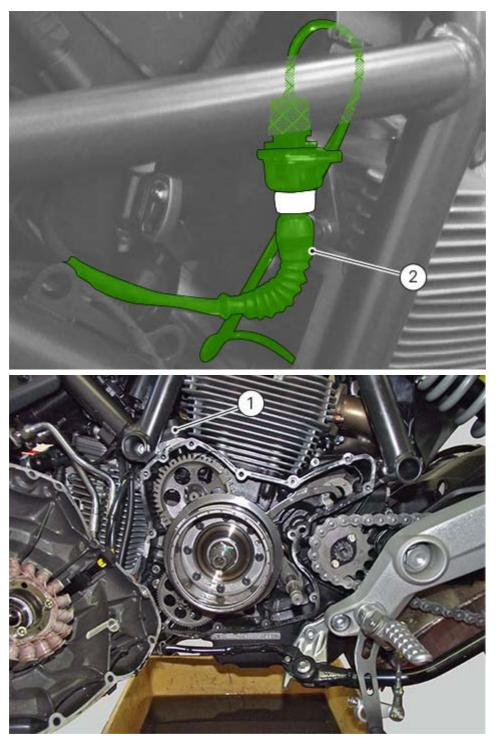
Check for rpm/timing sensor (pick-up) correct operation with the diagnosis instrument DDS 2.
