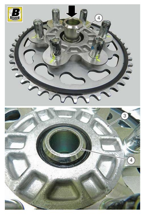
Position the rear sprocket flange-rear sprocket assembly in the rear wheel. Fit spacer (6) and tighten nuts (2) to a torque of 46 Nm  $\pm$  5%.
