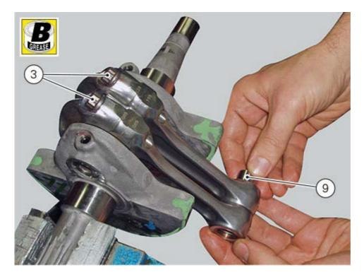
Put the spacer of tool no. 88713.2878 between the con-rods and take up residual axial clearance with the fork feeler gauge of tool no. 88713.2878 which has shims of the following sizes: - 0.1 mm - 0.2 mm - 0.3 mm.
