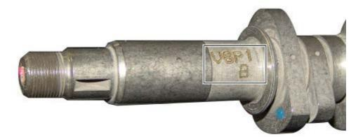
Lubricate the camshaft seats and "tank" (13) and (A) so that during the first engine rotations the camshaft is lubricated.
