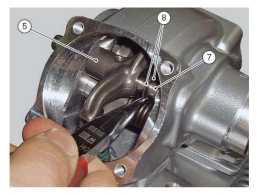
Refit the timing side cap (Refitting the camshafts).
