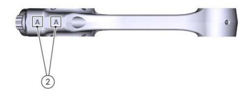
It is good practice to replace the bearings (A) each time the engine is overhauled. Spare bearings are supplied ready for fitting and they must not be reworked with scrapers or emery cloth.
