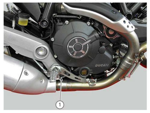
To check operation of the rear (1) STOP switch, use a multimeter: when the rear brake lever is operated, there must be electric continuity between the terminals of the corresponding switch. No electric continuity should be available when brakes are not operated.
