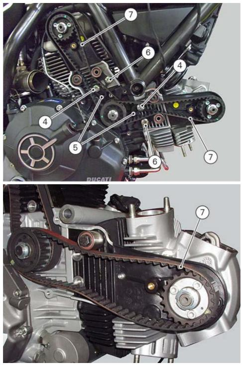
Perform the same operation sequence to remove the vertical cylinder timing belt.
