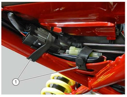
Disconnect tail light connector (2) from main wiring.
