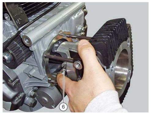
If work is to be carried out on the piston, carefully withdraw it from the cylinder.
