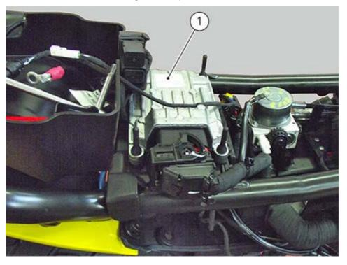
The ECU control unit (1) controls both the injectors and the coils, thus controlling fuel injection and ignition in accordance with the engine operating conditions detected by the following sensors:
