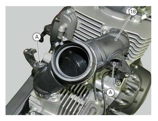
In order to avoid damaging the O-rings of the injectors, fit the injectors into the unions fully home, keeping them in line with their relevant seat.
