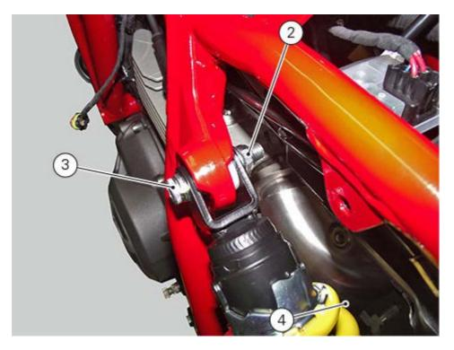
Apply specified grease to the thread and underhead of the lower screw (4), insert the shock absorber lower part in the swinging arm and tighten screw (4) to a torque of 42 Nm  $\pm$  5%.
