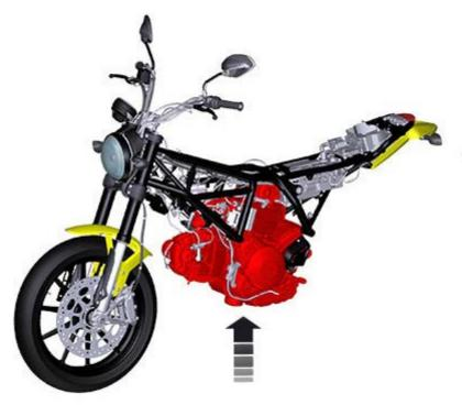
Remove the two pins (1) that retain the engine to the frame. Remove the engine from the frame.
