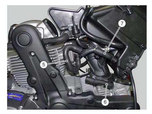
Work on the vertical head and remove clip (8) and disconnect pipe (5).
