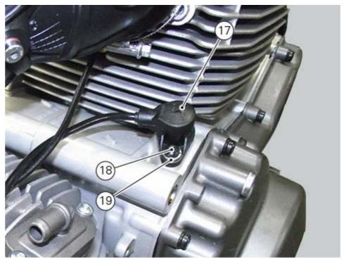
Use a feeler gauge to check the clearance between the engine sensor (17) and the timing gear (23). The value must be between 0.6 and 0.8 mm.
