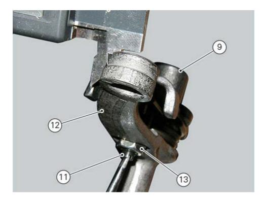
Position spring (16) between shaft (12) and fork (5). Fit ring (14) to block the coupled elements. Check that the spring (16) is installed correctly as shown in the figure. Then tighten nut (13) to a torque of 10 Nm (Min. 9 Nm - Max. 11 Nm)
