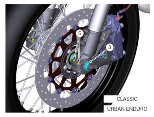
Loosen screws (5) that have been previously tightened. Lower the bike to the ground by removing the support. Push on the handlebar to load the suspensions and to allow the fork legs to settle on the wheel shaft. Tighten the screws (5) to a torque of 10 Nm  $\pm$  5%, following a 1-2-1 sequence.
