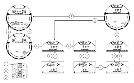
To confirm (store) the new set time press button (4). The EXIT box starts flashing, press button (4) to go back to the setting menu.
