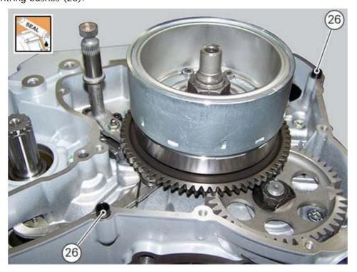
Spread a continuous uniform bead of DUCATI sealing compound on the cover mating surface, and around the holes of the screws and bushes.
