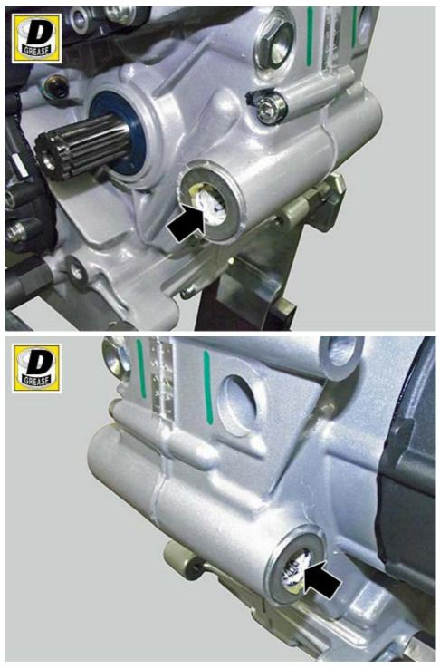
Position the shims as described in chapter "Overhauling the rear swinging arm".
