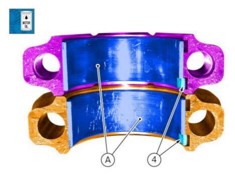
Check that the progressive number punched on the two parts sides is the same, as shown in the figure.
