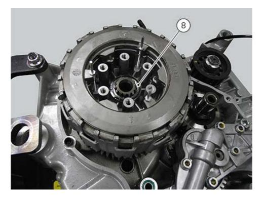
Apply the specified grease on nut (7) mating surface and on primary shaft thread, then insert nut driving it fully home by hand inside primary shaft. Lock clutch housing with tool (T) no. **88713.2556**, so as to hold it when tightening nut (7). Tighten nut (7) to a torque of 190 Nm (Min. 180 Nm - Max. 200 Nm). Remove tool (T) no. **88713.2556**.
