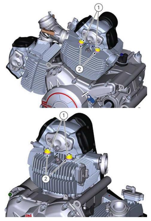
Remove the complete head from the engine by sliding it out of the stud bolts. Remove the cylinder head gaskets (3).
