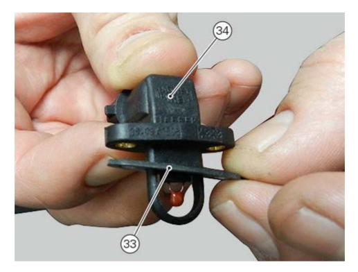
Fasten sensor (34) to the airbox and tighten the two screws (35) to a torque of 1 Nm  $\pm$  10%.
