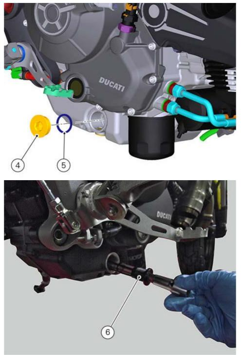
Restore proper engine oil level.
