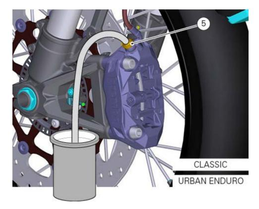
Tighten the bleed valve (5) to a torque of 4 Nm  $\pm$ 10% and then release the lever. Repeat the above operation until the old fluid flows out completely. Then, with the bleed valve definitely closed to the specified torque actuate repeatedly the lever until a pressure is detected in the brake system.
