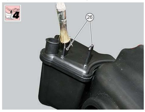
Engage the MAP\_SENSOR support fully home on the just-lubricated tabs. Apply the specified lubricant in the hole and on pin (28).
