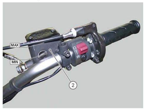
Pull the lever to make a 20 - 30 mm stroke and keep the lever in this position using a non-elastic clamp.
