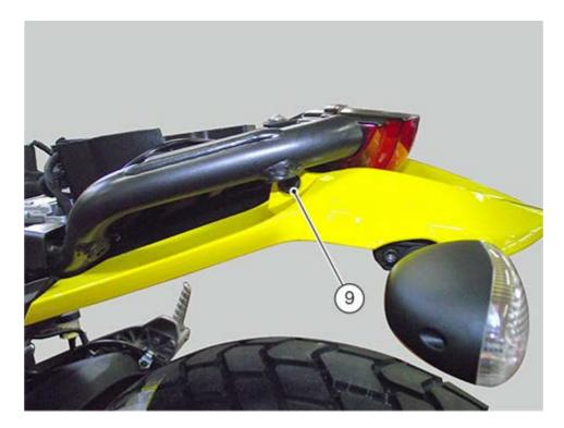
Separate tail guard (8) from the frame and disconnect the connectors of RH (11) and LH (12) turn indicators. Remove tail guard (8).
