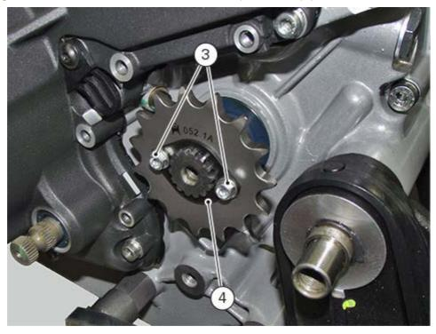
Remove plate (4) of the gearbox secondary shaft (5).
