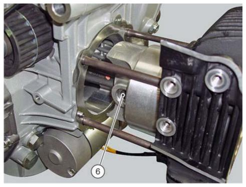
Since insertion of piston in the cylinder is a difficult operation to perform at the time of reassembly, remove the cylinder together with the piston as described below.
