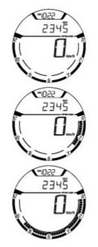
The thresholds before the rpm limiter are: 1st threshold 8900 rpm (A). When the rev limiter value (B) is reached, the warning lights start flashing.
