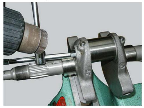
Clean all the oilways using suitable diameter metal brushes and then blow with compressed air to remove any residues that may have accumulated and are restricting the oil flow.
