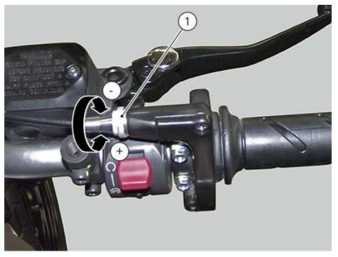
Check the outer sheath of the throttle control cable for damage at regular intervals.
