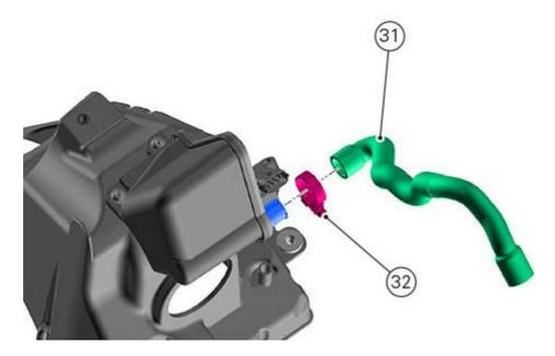
Aim hose (31) and the clip as shown in the figure. Tighten the clip to a torque of 1.5 Nm  $\pm$  10%.
