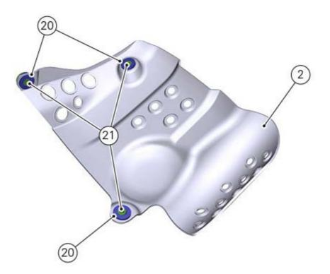
Fix heat guard (2) by tightening screws (1).
