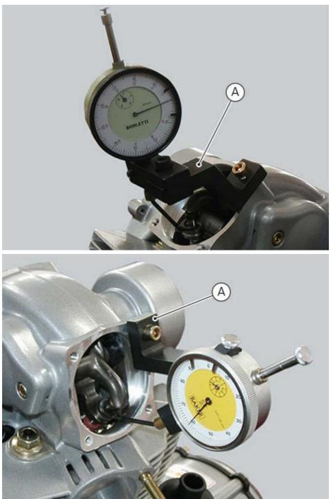
Check that the feeler gauge fork probe is centred on the valve axis and against the closing shim collar. Set the dial gauge to zero when the valve is fully closed.
