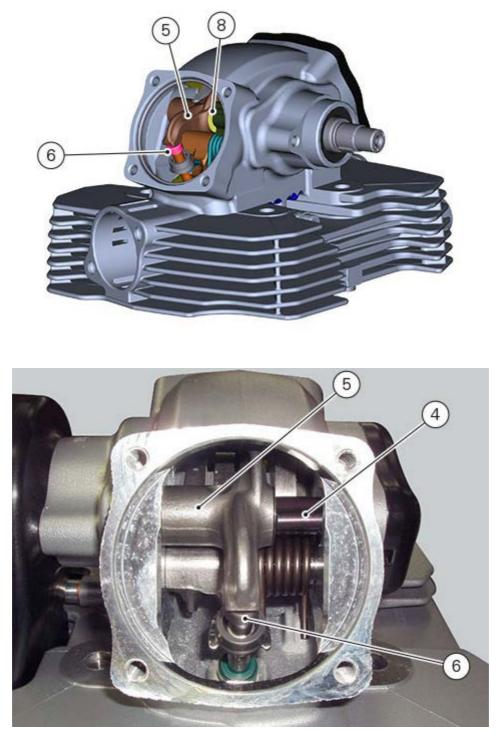
Refit the caps, the camshafts and the valve covers (Refitting the camshafts).
