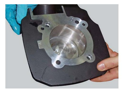
To remove the vertical cylinder-piston assembly follow the procedure performed on the horizontal cylinder. Remove gaskets (8) between cylinder and casing.
