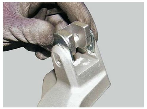
Smear the recommended grease on pin (13) and insert as shown. Lock shaft using circlip (12).
