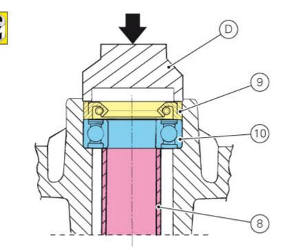
Use the same method to install the sealing rings (9). Ensure that spacer (8) is fitted between the two wheel hub bearings.
