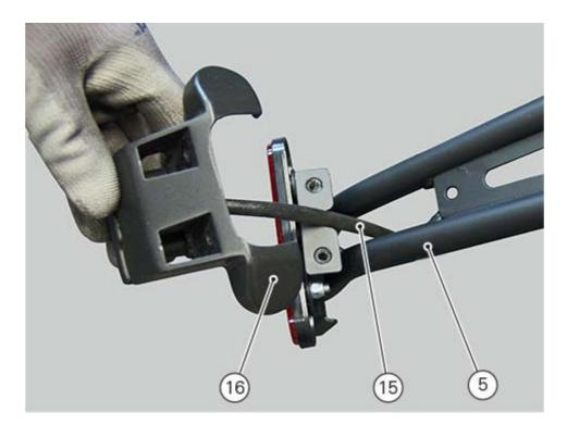
Fix the number plate light (16) by means of screws (17).
