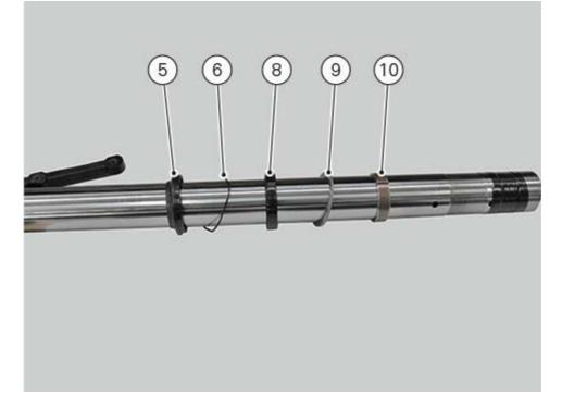
Note Pay attention to the direction of installation of oil seal, spring must face outward.
