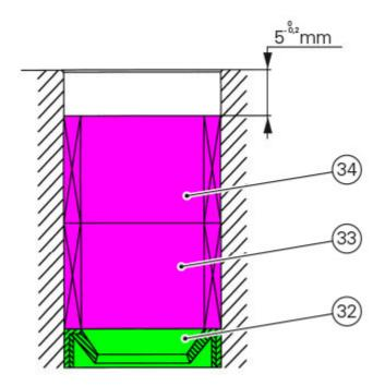
Orient the seal ring (32) as shown. The arrow refers to the insertion direction.
