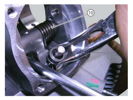
With the valve in rest position and by counter-holding the return spring, push on the rocker arm and check that the clearance between the rocker arm sliding shoe and the closing shim is the specified one. If this is not the case, adjust the valve clearance.
