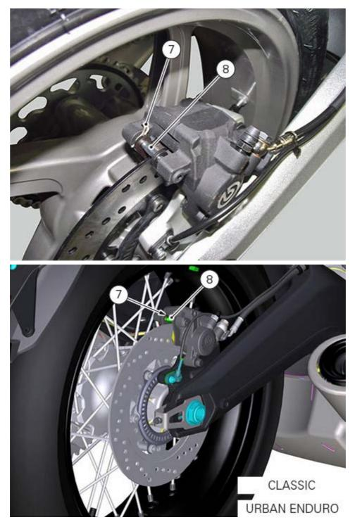
Fit the new pads. Fit the centring pin (8) and fasten it with the snap ring (7).
