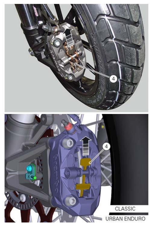
Operate the brake lever repeatedly so that the pads firmly bed in against the disc thanks to the brake fluid pressure.
