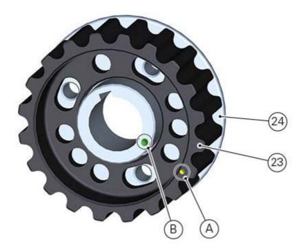
Fit washer (22) fully home on the pulley, aligning the reference notch (C) with pulley reference point (A) and hub reference mark (B). Tighten screws (21) in the hub threaded holes.
