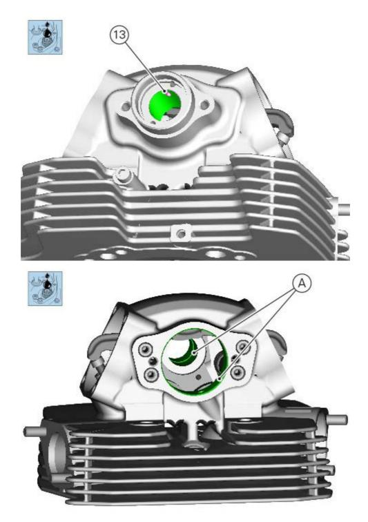
Fit the camshaft (11) from the head LH side.
