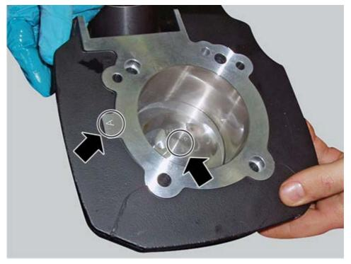
If the pistons have been separated from their cylinders, before reassembling these components, position the piston ring gaps at 120° from one another (the markings must always face the piston crown). Using a universal tool, gently insert the piston in the cylinder (lubricate the cylinder inner side with engine oil before inserting the piston).
