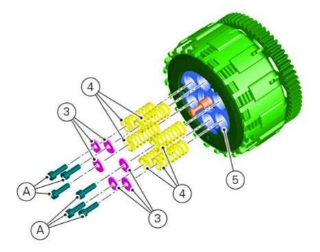
Slide out the pusher plate (5) with the clutch control pin (6).
