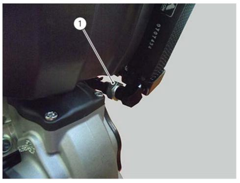
To test the operation of the engine oil pressure sensor (1), proceed as follows.
