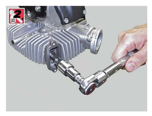
Position the spark arrestor plate (13) and pay attention to the insertion direction.
