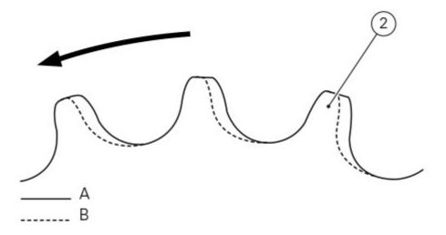
Make sure that the rear sprocket, front sprocket and chain are all replaced together as a set.
