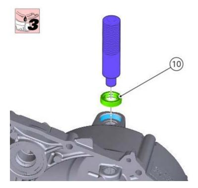
Insert clutch layshaft (9) in seal ring (10) having care not to damage it. Position spring (11). Part (12) must be engaged in recess (13) of shaft (9).
