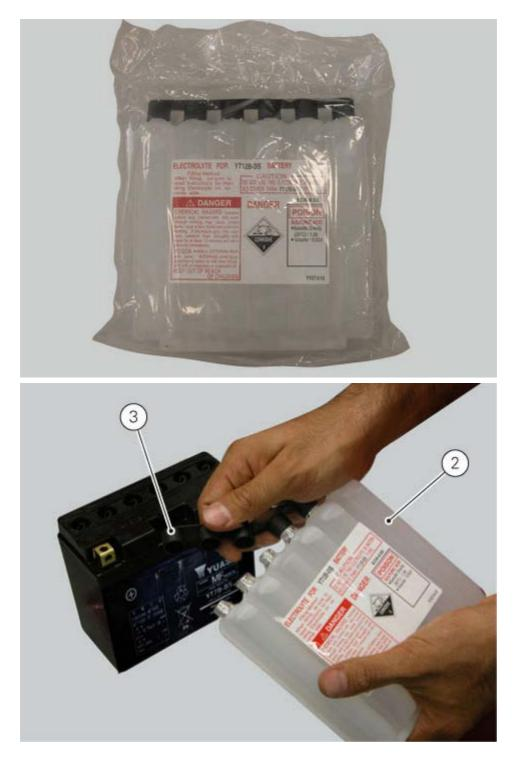
**D**Important Keep the cap strip (3) to hand because it will be used later to plug the battery cells.
