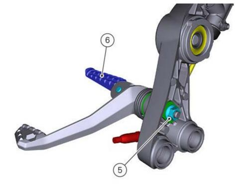
Slide out brake control lever (7) and footpeg (6) of the footpeg holder plate (8). Collect washer (9).
