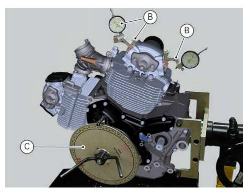
Continue to rotate in the same direction until you obtain a lift of **1** mm on the intake side. Check the angular value on the degree wheel.
