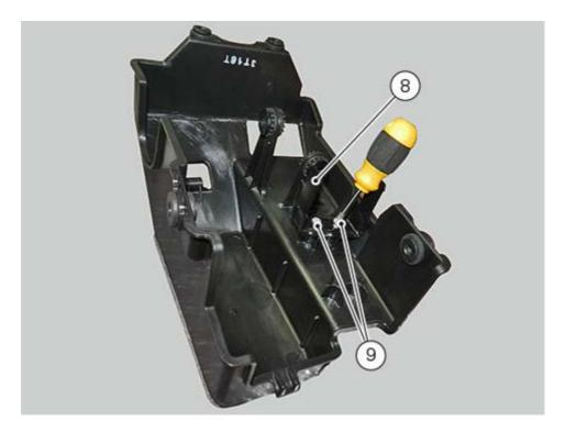
Position electrical components compartment in the frame. Start screws (1) and tighten them to a torque of 5 Nm  $\pm$  10%.
