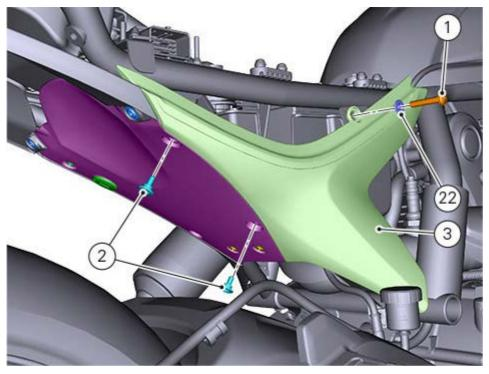
Tighten screw (1) with washer (22) and the two screws (2) to a torque of 8 Nm  $\pm$  10%.
