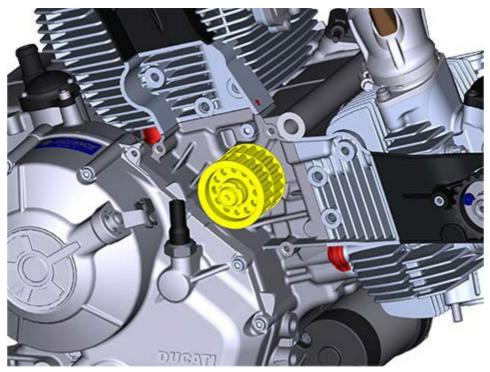
Block with the key of tool (A) no. **88700.5644** the driving pulley rotation on the crankcase and use the tool bush to loosen the retaining ring nut (12). Remove ring nut (12), washer (13) and the outer pulley (14).
