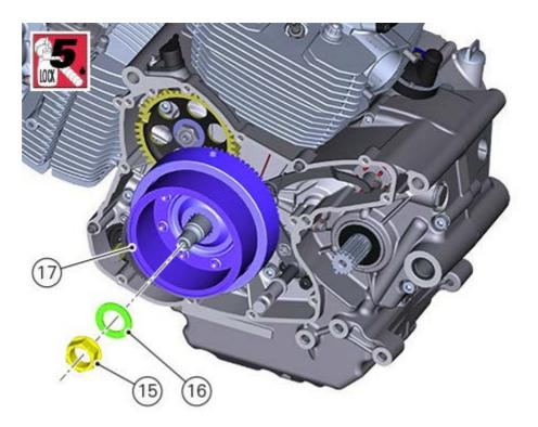
Block the flywheel rotation with the suitable tool (A) no. **88713.2036**. Tighten nut (15) to a torque of 270 Nm (Min. 256 Nm - Max. 284 Nm)
