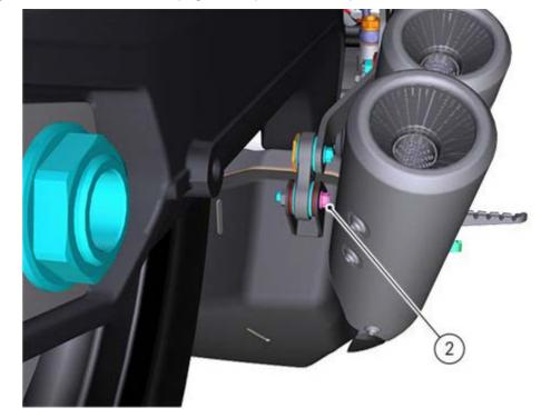
Start and tighten screw (2) in the footpeg holder plate to a torque of 10 Nm  $\pm$  10%.
