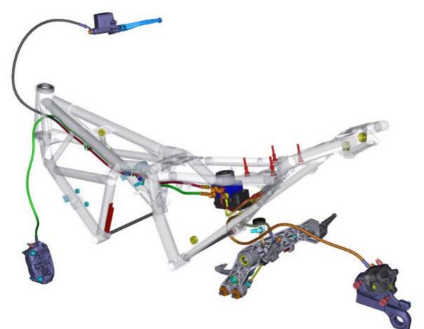
Loosen special screws (1), collect seals (2) and remove the following hoses: (3) Front brake master cylinder;
