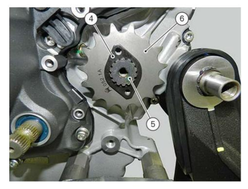
Remove the front sprocket (6) from the gearbox secondary shaft (5).
