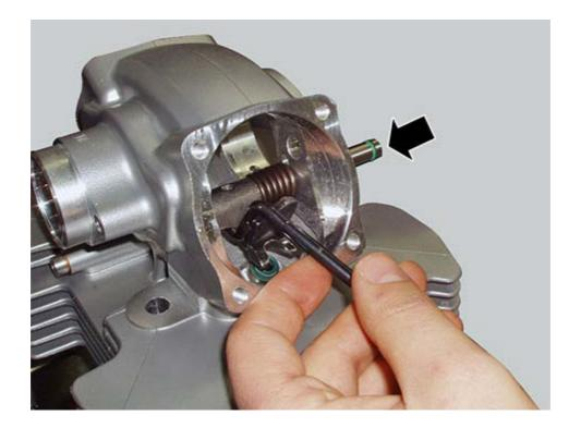
When refitting the rocker arm shafts, make sure that the threaded hole is on the head outer side.
