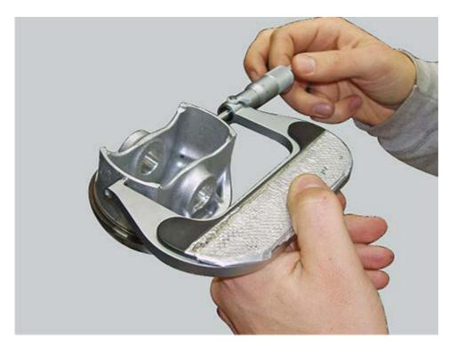
The pistons must always be replaced as a pair.
