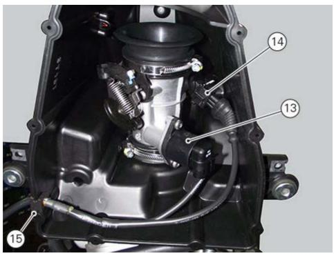
Secure the throttle body with clamp (16).
