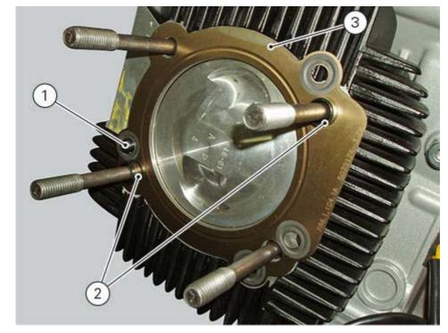
Slide out of the cylinder surface the pin (1), bushings (2) and head gasket (3).
