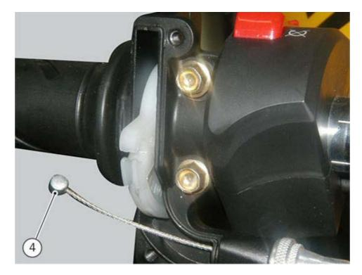
Carefully close the control while engaging cable (4) into slide (5) on cover (2). Fasten cover and tighten two screws (3) to the torque of  $1.8 \text{ Nm} \pm 10\%$ .
