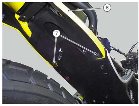
Remove the two lower screws (7) of tail guard (8).
