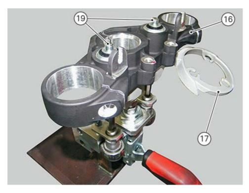
Fit two washers (20) on screws (19) and start two nuts (15). Screw two nuts (15).
