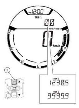
The odometer counts and displays the total distance covered by the motorcycle with the set unit of measurement (km or mi).
