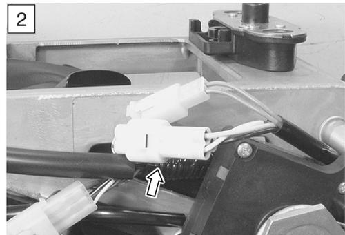
**DATA** Position sensor input voltage: 4.5 – 5.5 V
