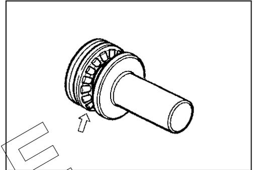
**CLUTCH SLEEVE HUB/PRIMARY DRIVEN GEAR ASSEMBLY**
