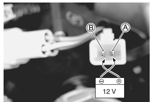
Measure the position sensor output voltage at fully open position.
