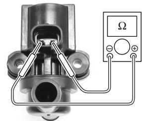
If the resistance is not within the standard range, replace the PAIR control solenoid valve with a new one.
