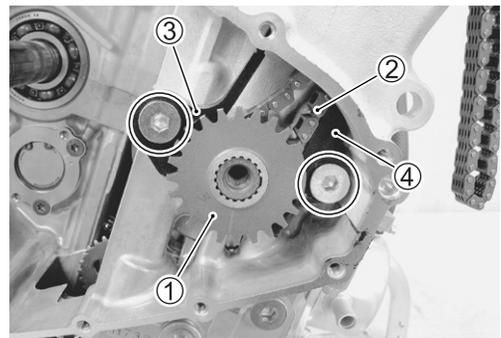
**GENERATOR ROTOR AND STARTER DRIVEN GEAR**
