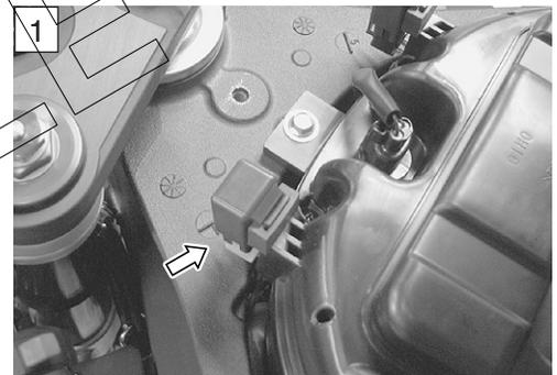
Is the cooling fan relay OK?
