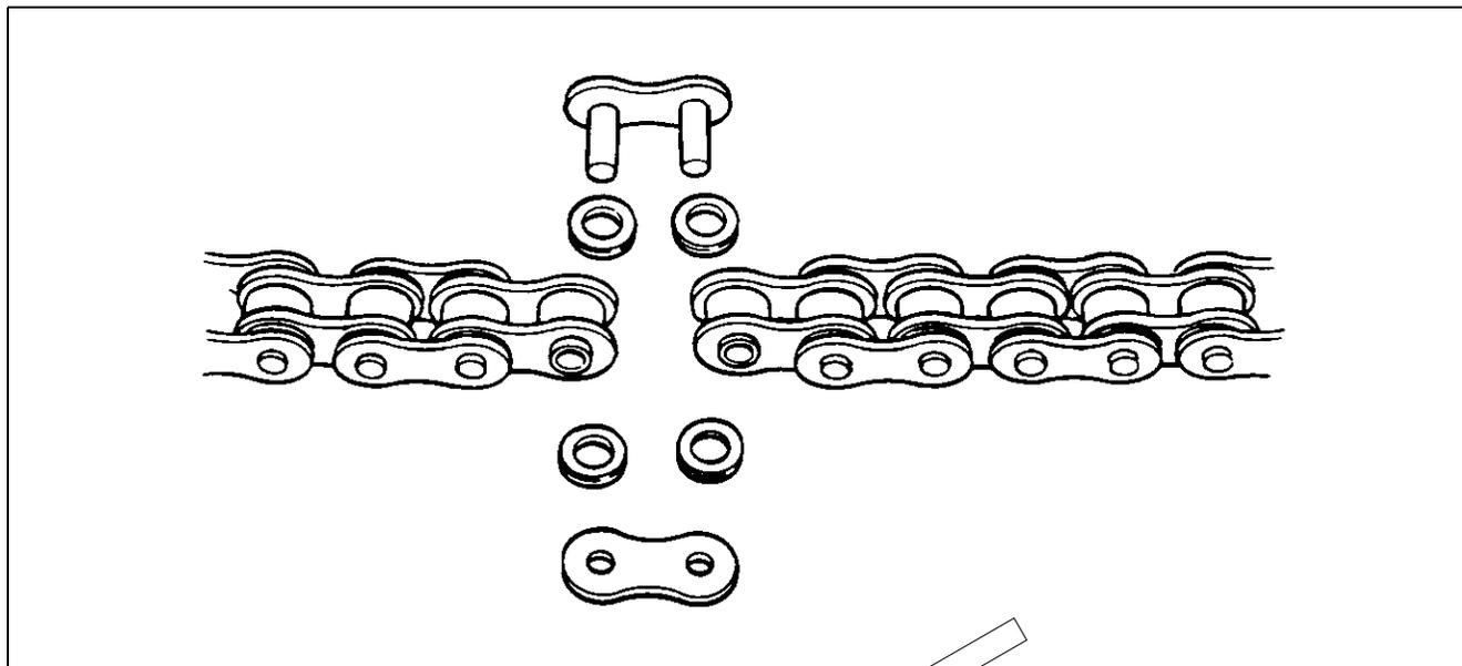
Use the special tool in the following procedures, to cut and rejoin the drive chain.
