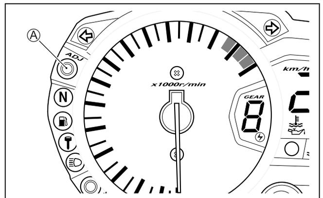
Pointer will return to the starting point right after the completion of the operation. In the case of the pointer not returning to the proper position after doing above, replace the combination meter unit.
