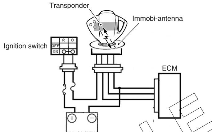
Also, when the ignition switch is turned ON, the indicator light flashes as many as the number of IDs registered in ECM. Thereafter, if the IDs are in agreement, the indicator light turns on for two seconds to notify of completion in successful communication.
