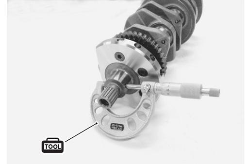
**TOOL** 09900-20202: Micrometer (25 – 50 mm)**DATA** Bearing thickness specification
