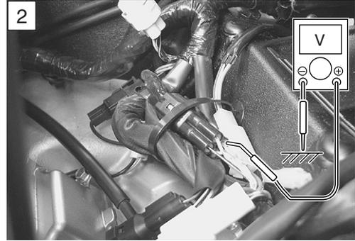
**DATA** Heater voltage: Battery voltage
