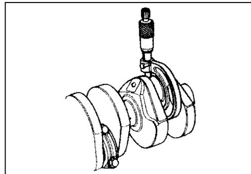
**TOOL** 09900-20202: Micrometer (25 – 50 mm)**DATA** Bearing thickness
