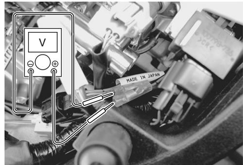
**DATA** TP sensor output voltage at idle position: Approx. 1.125 V
