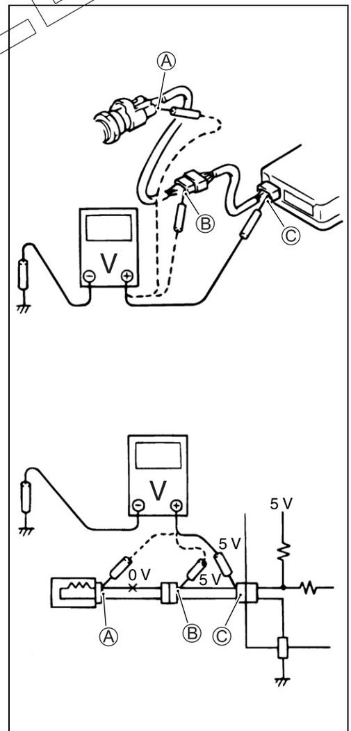
**SHORT CIRCUIT CHECK (WIRE HARNESS TO GROUND)**
