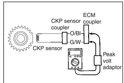
If the peak voltage is lower than the standard range, check the peak voltage at the CKP sensor lead wire coupler.
