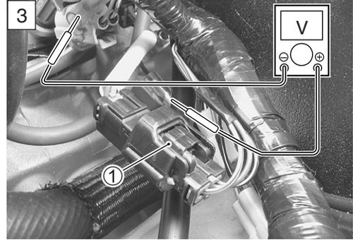
**DATA** TP sensor output voltage
