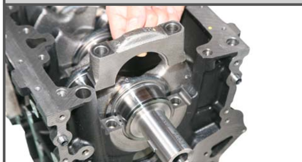
Selection of lower main bearing
