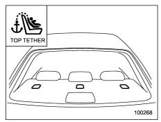
Three tether anchorages are installed on the rear shelf behind the rear seat head restraint. Open the cover flap to use each anchorage.
