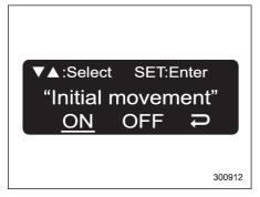
4. Select "ON" for activated initial movement or "OFF" for deactivated initial movement by pressing the "▲" or "▼" switch. And press the "[]/SET" switch to decide the desired setting.
