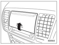
To open the center panel compartment, pull up the edge of the bottom of the panel lid.
