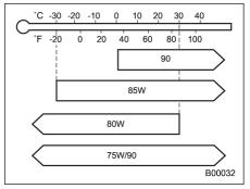
SAE viscosity No. and applicable temperature
