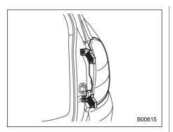
Tighten the upper and lower screws.
