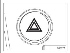
The hazard warning flasher is used to warn other drivers when you have to park vour vehicle under emergency conditions. The hazard warning flasher works with the ignition switch in any position.
