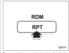
To repeat the currently playing disc/folder, press the "RPT" button twice while a track/ file (track) is playing. The display will show "D-RPT" for non-MP3/WMA disc, "F-RPT" for MP3/WMA folder. And the disc/folder will be played repeatedly.
