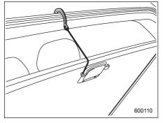
1. Open the lid and hang the hook provided on the under side of the lid on
