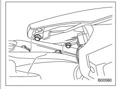
8. Reinstall the rear combination light assembly by sliding the two-pronged part of the combination light assembly securely to each holder of the vehicle side.
