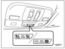
on or 💥 : Front passenger's frontal airbag ON indicator
