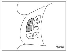
Press the "+" button to increase the volume. Press the "-" button to reduce the volume.
