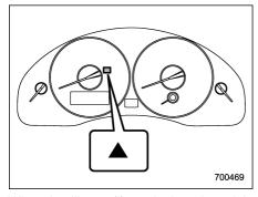
When Intelligent (I) mode is selected in vehicles equipped with a manual transmission, a shift-up indicator "\( \bigcap \)" in the tachometer will blink to signal the best time to shift gears for maximum fuel efficiency.
