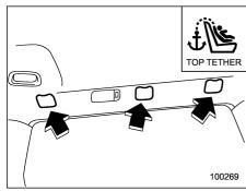
Three tether anchorages, i.e., ones for the right, center and left positions, are already installed on the rear edge of the roof.
