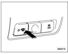
The windshield wiper deicer operates only when the ignition switch is in the "ON" position.
