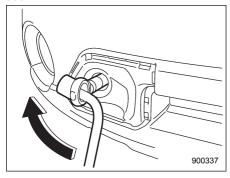
5. Tighten the towing hook securely using a wheel nut wrench.
