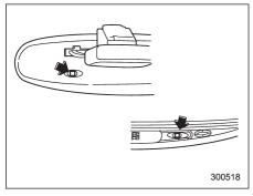
The mirror has a photosensor attached on both the front and back sides. If the glare from the headlights of vehicles behind you strikes the mirror, these sensors detect it and make the reflection surface of the mirror dimmer to help prevent you from being blinded. For this reason, use care not to cover the sensors with stickers, or
