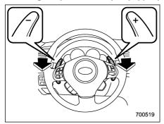
Pull the "+" of the paddle shift to upshift one level. Also pull the "-" of the paddle shift to downshift one level.
