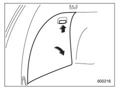
A stowage box is located on each side of the cargo area. You can access each one by pushing up and pulling the knob on the lid.
