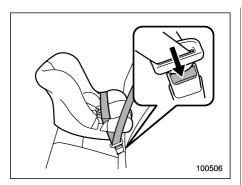
8. To remove the child restraint system, press the release button on the seatbelt buckle and allow the belt to retract completely. The belt will return to the FLR mode.
