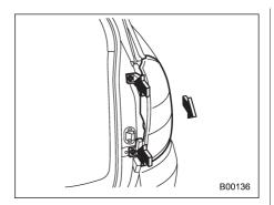
3. Remove the upper and lower screws. Then, straightly slide the rear combination light assembly rearward and remove it from the vehicle.
