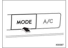
Select the desired air flow mode by pushing the air flow mode selection button. The selected air flow mode is shown by the display.
