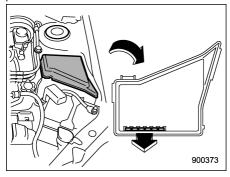
2. Pull any one spare fuse out of the spare fuse holder. Spare fuses are attached on the back side of the fuse holder cover in the engine compartment. You may pick up any one fuse in the spare fuse holder.
