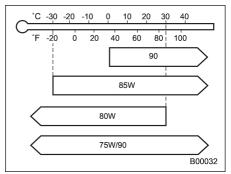
SAE viscosity No. and applicable temperature
