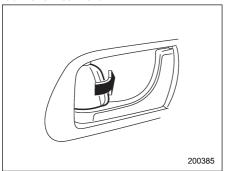
To unlock the door from the inside, rotate the lock lever forward.
