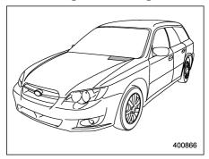
Always keep the front ventilator inlet grille free of snow, leaves, or other obstructions to ensure efficient heating and defrosting. Since the condenser is located in front of the radiator, this area should be kept clean because cooling performance is impaired by any accumulation of insects and leaves on the condenser.
