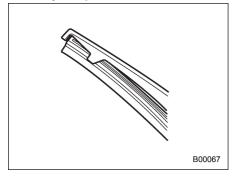
Securely retain both ends of the rubber with the stoppers on the plastic support ends. If the rubber is not retained properly, the wiper may scratch the rear window alass.
