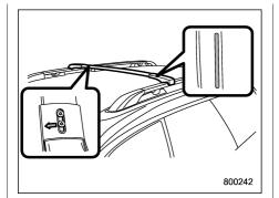
3. The crossbar with the 100 LBS Load Label attached onto it is the front crossbar. An arrow is marked on the back of the front crossbar for correct installation. Install the front crossbar so that the arrow faces the front of the vehicle.
