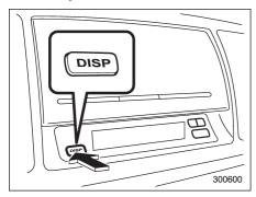
With the ignition switch in the "ON" position, each successive push of the "DISP" button toggles the display in the following sequence:
