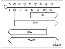
SAE viscosity No. and applicable temperature
