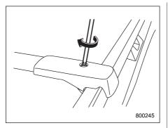
6. Adjust the alignment of the crossbar on the roof rails, and if available, use a T-30 torx® bit and torque wrench and tighten the T-30 torx® head screws to 30 to 35 lbf·in (3.4 to 4.0 N·m, 0.35 to 0.41 kgf·m) of torque (or tighten securely with the torx® wrench provided).
