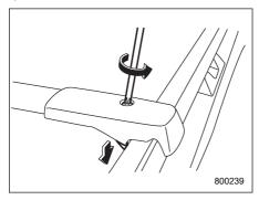
1. Loosen and remove the T-30 torx® head screw from the top of each crossbar end support.
