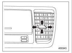
Move the tab up and down or right and left to adjust the flow direction.
