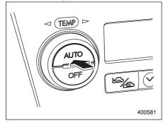
When the "AUTO" button is pressed, the indicator light "AUTO" on the display illuminates. In this state, fan speed, air flow distribution, air-inlet control, and air conditioner compressor operation are automatically controlled.
