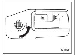
When you entrust your vehicle key to another person, you can lock the trunk lid release lever to prevent luggage in the trunk from being stolen. To lock the trunk lid release lever, insert the master key or submaster key into the key cylinder at the rear of the release lever and turn it counterclockwise. To unlock the trunk lid release lever, turn the key clockwise.
