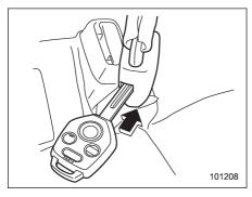
1. Insert a key or other hard pointed object into the slot in the connector (buckle) on the right-hand side and push it in, and the connector (tongue) plate will disconnect from the buckle.
