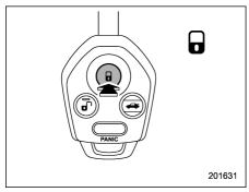
Press the "a" button to lock all doors and rear gate (Station wagon). An electronic chirp will sound once and the turn signal lights will flash once.
