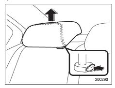
1. Remove the head restraint at the seating position where the child seat has been installed with the seatbelt or lower anchorages; lift up the head restraint while pressing the release button.
