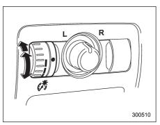
The brightness of clock display, audio, air conditioner, information display and meter/gauge illumination dims when the light switch is in the "aboa" or "aposition. You can adjust brightness of the meter/gauge illumination for better visibility.
