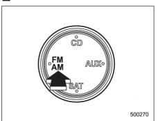
Push the "FM AM" button when the radio is off to turn on the radio.
