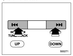
Press "I of the TUNE TRACK button to select the next channel and press "I of the button to select the previous channel. Keep pressing "I of the button to change to the next channel continuously and keep pressing "II of the button to change to the previous channel continuously.
