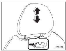
The head restraint should be adjusted so that the center of the head restraint is closest to the top of the occupant's ears.
