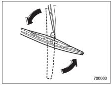
2. Turn the wiper blade assembly counterclockwise.
