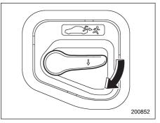
To open the trunk lid from inside the trunk, press the yellow handle downward as indicated by the arrow on the handle. This operation unlocks the trunk lid. Then, push up the lid.
