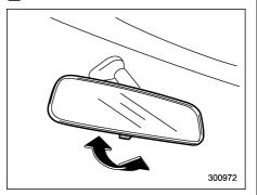
The inside mirror has a day and night position. Pull the tab at the bottom of the mirror toward you for the night position. Push it away for the day position. The night position reduces glare from headlights.
