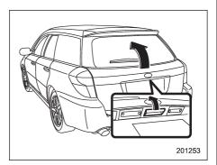
The rear gate can be locked and unlocked using either the remote keyless entry system or power door locking switch.
