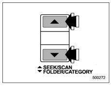
If you press the "\( \bigcap \)" or "\( \bigcup \)" side of the SEEK/SCAN button briefly, the radio will automatically search for a receivable station and stop at the first one it finds. This function may not be available, however, when radio signals are weak. In such a situation, perform manual tuning to select the desired station.
