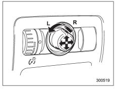
The remote control mirrors operate only when the ignition switch is in the "ON" or "Acc" position.
