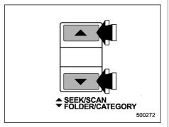
The scan mode lets you listen to the first 10 seconds of each track/file (track) in succession. Press the "♠" side of the SEEK/SCAN button for 0.5 second or longer to start scanning upward beginning with the track/file (track) following the currently selected one. Press the "♥" side of the button to start scanning downward beginning with the track/file (track) preceding the currently selected one.
