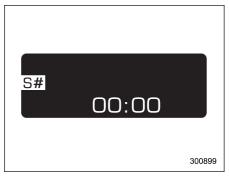
The clock receives the correct time from the navigation system. To adjust the time shown by the clock, refer to the Owner's Manual supplement for the monitor system and adjust the time of the navigation system.
