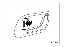
To lock the door from the inside, rotate the lock lever rearward.
