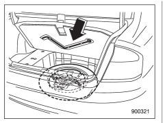
Sedan: Open the floor cover and remove the jack handle from the back of the floor cover.
