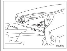
8. Reinstall the rear combination light assembly by sliding the two-pronged part of the combination light assembly securely to each holder of the vehicle side.
