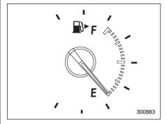
The dial of the fuel gauge flashes five times when the amount of remaining fuel reaches 2.6 US gal (10 liters, 2.2 lmp gal). If you turn the ignition switch to the "LOCK" position and back to the "ON" position, the dial will again flash five times.
