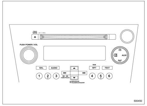
The audio set will operate only when the ignition switch is in the "Acc" or "ON" position.
