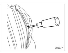
2. Wrap tape around a flat-head screwdriver, then insert the screwdriver into the gap between the side cover and rear combination light and use it as a lever to undo clip 1 in the illustration shown. Undo clips 2 and 3 in the same way, then remove the side cover.
