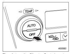
The Automatic Climate Control system turns off (the air conditioner compressor and fan turn off) when the "OFF" button is pressed.
