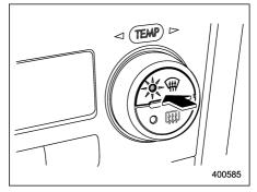
To defrost or dehumidify the windshield and front door windows, push the defroster button "w". When the "w" button is pushed, outside air is drawn into the passenger compartment, air flow is directed towards the windshield and front door windows, and the indicator light on the button illuminates.
