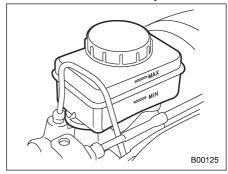
Check the fluid level on the outside of the reservoir. If the level is below "MIN", add the recommended brake fluid to "MAX".
