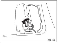
2. Turn the bulb socket counterclockwise and remove it.
