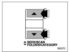
If you press the "▲" or "▼" side of the SEEK/SCAN button for 0.5 second or longer, the radio will switch to scan mode. In this mode, the radio scans through the radio band until a station is found. The radio will stop at the station for 5 seconds while displaying the frequency, after which scanning will continue until the entire band has been scanned.
