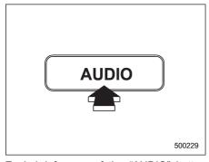
Each brief press of the "AUDIO" button changes control modes in the following sequence starting from volume control mode. (When the radio is first turned on, the control mode is in the volume control.)
