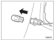
3. Pull the bulb out of the bulb socket and
