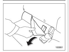
Peel off the anchorage cover from the selected side of the rear seatback to expose the anchorages (bars) to be used for installation of the child restraint system.
