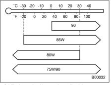
SAE viscosity No. and applicable temperature
