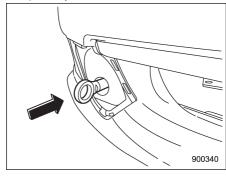
5. Screw the towing hook into the thread hole until the threads can no longer be seen.
