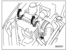
3. Unsnap the two clamps holding the air cleaner case cover.
