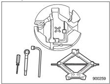
Screwdriver Towing hook Wheel nut wrench
