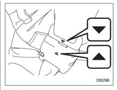
4. After fastening the seatbelt, make sure that the "\(\nblue{T}\)" mark on the connector (tongue) and the "A" mark on the buckle face outwards.
