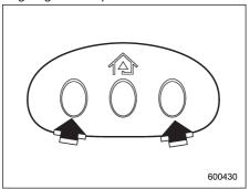
2. Press and hold the two outside buttons until the HomeLink® indicator light begins to flash (after 20 seconds). Release both buttons.
