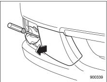
4. Likewise, insert the screwdriver still wrapped with cloth or vinyl into the cutout between the towing hook cover and the bumper. Pry out the cover.
