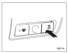
Pressing the switch to deactivate the Vehicle Dynamics Control system can facilitate the following operations:
