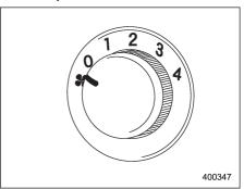
The fan operates only when the ignition switch is turned to the "ON" position. The fan speed control dial is used to select four fan speeds.
