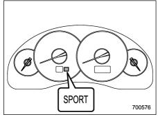
When selected, the SPORT mode indicator light on the instrument panel will turn on.
