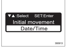
3. When the setting screen is displayed, select "Date/Time" by pressing the "A" or "V" switch. And press the "IVSET" switch to enter the "Date/Time" settings.
