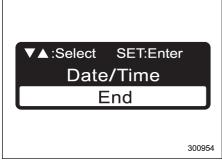
5. Select "End" by pressing the "\( \Lambda \)" or "\( \mathbb{\bar} \)" switch. And press the "\( \mathbb{\bar} \)/SET" switch to finish the meter setting menu.
