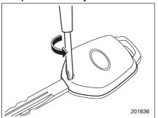
1. Remove the screw on the key head.
