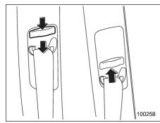
The shoulder belt anchor height should be adjusted to the position best suited for the driver/front passenger. Always adjust the anchor height so that the shoulder belt passes over the middle of the shoulder without touching the neck.
