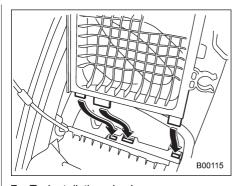
7. To install the air cleaner case cover, insert the three projections on the air cleaner case cover into the slits on the air cleaner case and then snap the two clamps on the air cleaner case cover.
