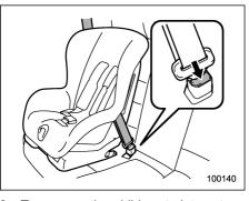
9. To remove the child restraint system, press the release button on the seatbelt buckle and allow the belt to retract completely. The belt will return to the ELR mode.
