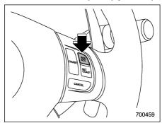
Push the "RES/ACC" button and hold it until the vehicle reaches the desired speed. Then, release the button. The vehicle speed at that moment will be memorized and treated as the new set speed.
