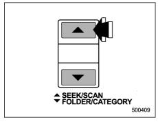
Press the "\( \bigsep \)" side of the SEEK/SCAN button to change the radio to the SCAN mode. In this mode, the radio scans through the channel until a station is found. The radio will stop at the station for 5 seconds while displaying the channel number, after which scanning will continue until the entire channel has been scanned from the low end to the high end.
