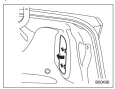
1. Push the knobs of the cover to open the cover.
