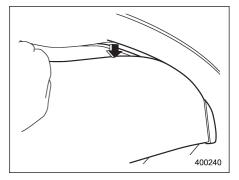
1. Remove the top of the rear gate board from the groove in the rear gate panel.
