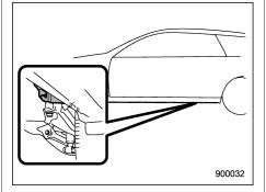
The rear tie-down hooks are located near each of the jack-up reinforcements.
