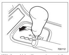
With the vehicle either moving or stationarv. move the selector lever from the "D" position to the manual gate to select the manual mode.
