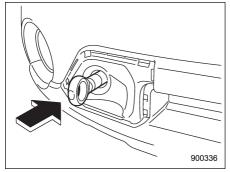
4. Screw the towing hook into the thread hole until the threads can no longer be seen.
