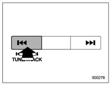
Press the " " side of the TUNE/TRACK button continuously to fast-reverse the disc/folder.
