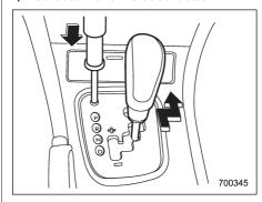
If you inadvertently have turned the ignition switch to the "LOCK" position with the selector lever in the "N" position, proceed as follows. By referring to the "Shift lock release" section in this chapter, remove the shift lock release cover. Then, with the screwdriver inserted into the hole, move the selector lever to the "P" position. If the selector lever reverse inhibiting function fails, have the vehicle inspected by the nearest SUBARU dealer.
