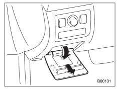
Open the lid that is located above the hood release knob and pull it toward you to remove it.
