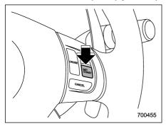
Push the "SET/COAST" button and hold it until the vehicle reaches the desired speed. Then, release the button. The vehicle speed at that moment will be memorized and treated as the new set speed.
