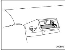
Pull the trunk lid release lever upward.
