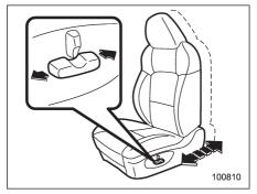
To adjust the seat forward or backward, move the control switch forward or backward.
