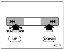
Press the "I side of the TUNE/TRACK button to increase the tuning frequency and press the tuning button marked "I to decrease it.
