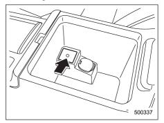
By connecting a commercial audio product to the vehicle, such as a portable audio player, you can hear its sound via the vehicle's speaker.
