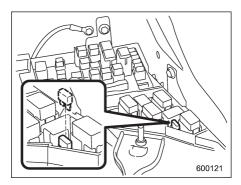
3. Put a spare fuse inside the FWD socket located in the fuse panel and confirm that the "AWD" warning light on the combination meter illuminates. The All-Wheel-Drive capability of the vehicle has now been deactivated.
