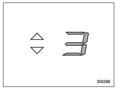
When the manual mode is selected, the gear position indicator (which shows the current gear selection) and the upshift/ downshift indicator light up. Refer to the "Automatic transmission - 4-speed" section in chapter 7.
