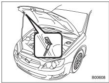
4. Lift up the hood, release the hood prop from its retainer and put the end of the hood prop into the slot in the hood.
