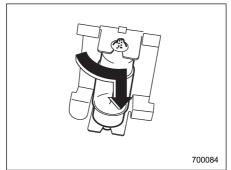
2. Turn the bulb until the flat surfaces at its ends are aligned vertically. Pull the bulb straight downward to remove it. Install a new bulb.
