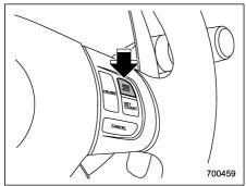
To resume the cruise control after it has been temporarily canceled and with vehicle speed of approximately 20 mph (32 km/h) or more, push the "RES/ACC" button to return to the original cruising speed automatically.
