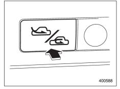
Select air flow by pushing the air inlet selection button " air inlet".
