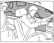
The SRS side airbag and SRS curtain airbag can function only when the ignition switch is in the "ON" position.
