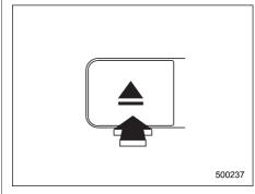
2. Briefly press the "\(\to \)" button. The selected disc will be ejected. The disc number indicator will flash at this time. When you remove the ejected disc, the disc number indicator will go off.
