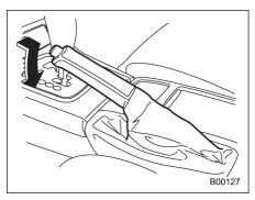
Check the parking brake stroke according to the maintenance schedule in the "Warranty and Maintenance Booklet". When the parking brake is properly adjusted, braking power is fully applied by pulling the lever up five to six notches gently but firmly (approximately 44 lbf, 196 N, 20 kgf). If the parking brake lever stroke is not within the specified range, have the brake system checked and adjusted at vour SUBARU dealer.
