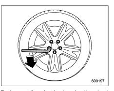
7. Loosen the wheel nuts using the wheel nut wrench but do not remove the nuts.
