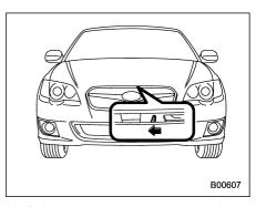
3. Release the secondary hood release located under the front grille by moving the lever toward the left.
