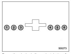
Press the desired disc select button for which the disc number indicator is lit. The player will then start playback of the selected CD, beginning with the first track. If a disc that the player cannot read has been loaded, the player will display the message "CHECK DISC".
