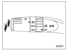
To change from low beam to high beam, push the turn signal lever forward. When the headlights are on high beam, the high beam indicator light "\( \bigcirc \)\" on the instrument panel is also on.
