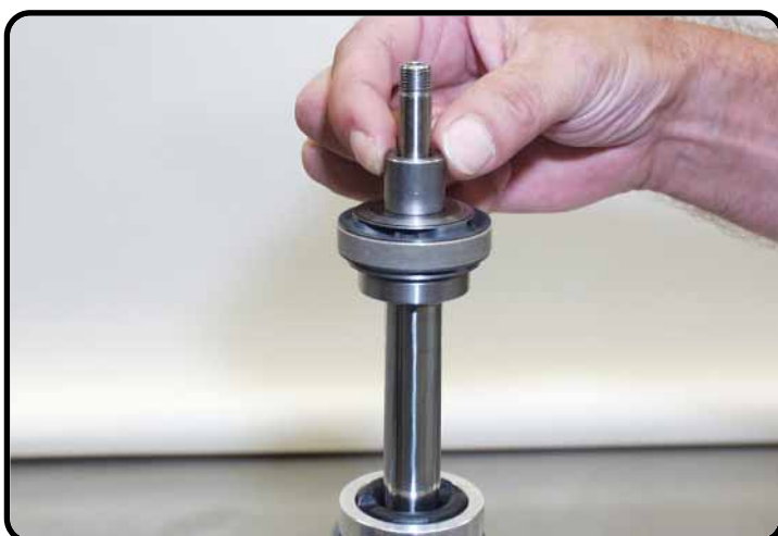
Replace the intermediate bush.
