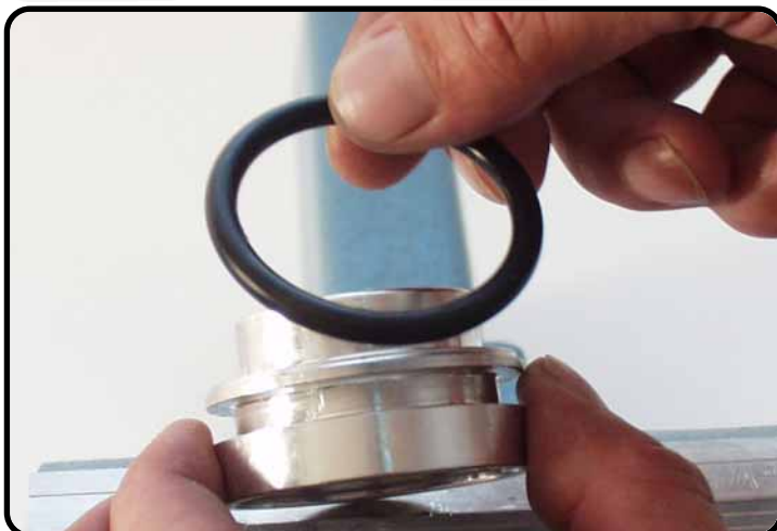
Remove the O-ring
