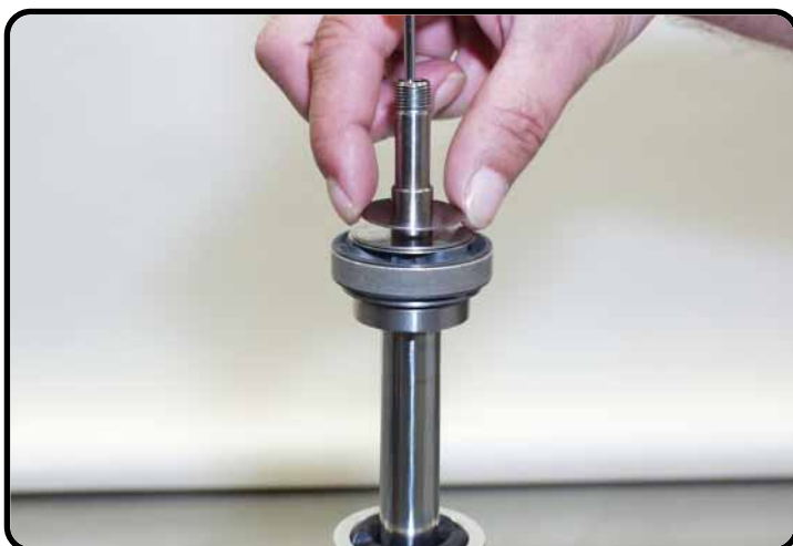
Assemble rebound setting 1.
