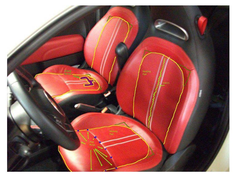
This is an outline of how the seat heaters fit. The seam around the bolsters on the seat bottom and back are formed and held in place with metal hog rings attached to wires embedded in the seat foam during manufacturing. You should only need to deal with the hog rings on the seat bottom (marked in blue). You'll be replacing the removed hog rings with plastic zip ties so you won't have to worry about shorting out the seat heaters or swearing about dropped and lost hog ties.
