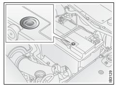
Electrolyte level indicator. Level correct if level indicator dark. Battery should be changed if indicator is light
