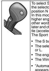
To select Sport mode, press the "S" button on the selector lever when the selector lever is in position N or D.
