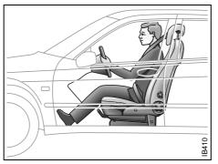
Correctly positioned safety belt
