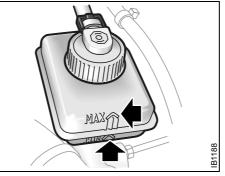
Brake and clutch-fluid reservoir
