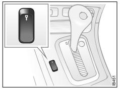
Switch for operation of central locking
