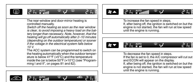
Recirculation is selected automatically for effective cooling, but it can also be switched on/off manually. Although recirculation does not substantially affect the air quality, it is useful to prevent unpleasant smells or fumes being drawn into the car from
