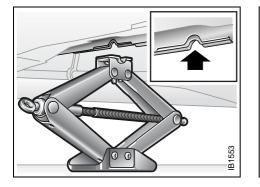
The collapsible jack handle is stowed in a cloth bag by the spare wheel. With the help of your foot, extend the handle as illustrated
