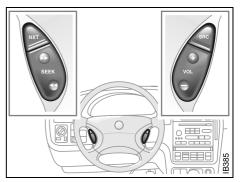
Audio System controls on steering wheel
