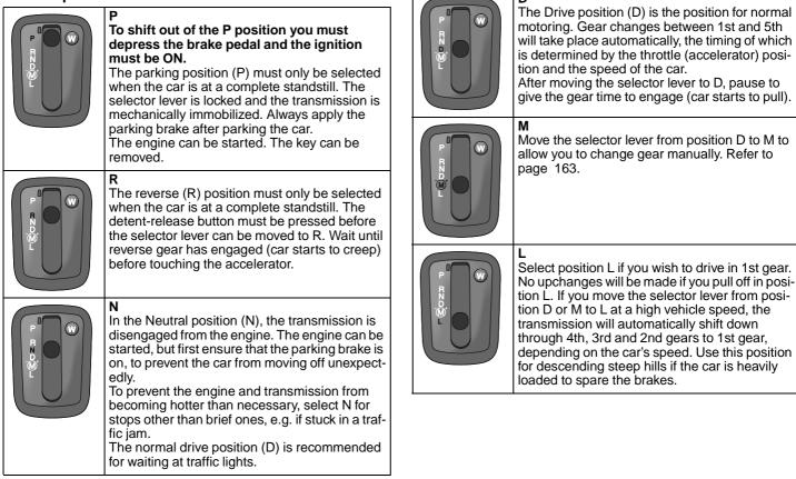
D The Drive position (D) is the position for normal motoring. Gear changes between 1st and 5th will take place automatically, the timing of which is determined by the throttle (accelerator) position and the speed of the car. After moving the selector lever to D, pause to give the gear time to engage (car starts to pull).
