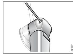
Adjusting the washer jet on the rear window wiper, 9-5 Wagon
