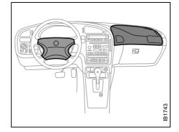
Accessories and other equipment must not be fitted to the surfaces marked as these are where the airbags inflate in the event of a crash.
