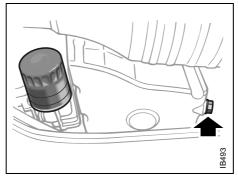
Drain plug and oil filter
