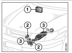
Oxygen-sensor-controlled injection system 1 Engine control module
