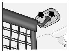
Attaching the cargo net to the roof
