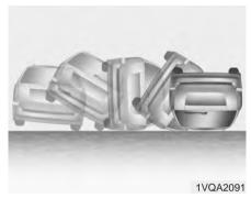
Air bags may not inflate in rollover accidents because air bag deployment would not provide proper protection to the occupants.
