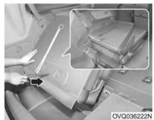
Release the strap and push the seat forward firmly until it clicks into place to insert the catches into the anchors.
