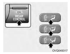
When the rear climate control selection (REAR CONTROL) button in the front climate control panel is in the ON position, the rear mode is selected by pushing the rear mode selection button on the rear control panel as follows:
