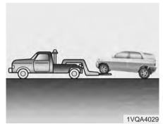
It is acceptable to tow the vehicle with the rear wheels on the ground (without dollies) and the front wheels off the ground. When being towed by a commercial tow truck and wheel dollies are not used, the front of the vehicle should always be lifted, not the rear.
