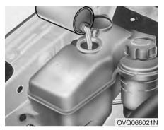
The coolant level should be filled between F and L marks on the side of the coolant reservoir when the engine is cool.
