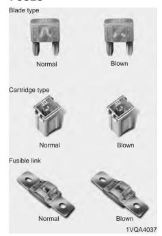
A vehicle's electrical system is protected from electrical overload damage by fuses. This vehicle has three fuse panels, one located in the driver's side panel bolster, another in the cargo area, the other in the engine compartment near the battery.
