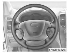
To sound the horn, press the horn symbol on your steering wheel.
