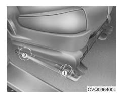
If the rear catches of the seat are locked into the rear anchors (2) while the front catches are not locked into the front anchors (1), do the followings to release the rear catches from the rear anchors.
