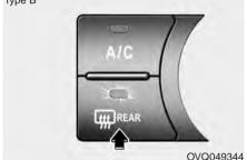
The defroster heats the window to remove frost, fog and thin ice from the interior and exterior of the rear window, while engine is running.
