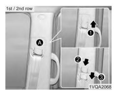
5. Adjust the shoulder anchor position to your size. To raise the anchor position, push the anchor up (1). To lower the anchor position, press (2) the button (A) and slide the anchor down (3). After adjustment, make sure the anchor is locked in position. (if equipped)
