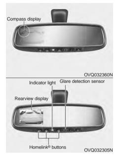
Your new mirror comes with an integrated HomeLink® Universal Transceiver, which allows you to program the mirror to activate your garage door(s), estate gate, home lighting, etc. The mirror actually learns the codes from your various existing transmitters.
