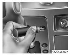
Insert the screwdriver into the access hole and press down on the screwdriver.
