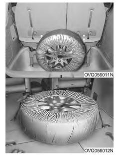
2. Place the flat tire in the cargo area when the 3rd row seat is upright position or on the floor when the 3rd row seat is stowed in the cargo area.
