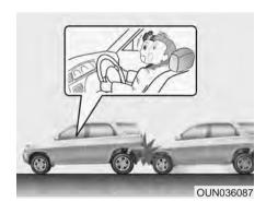
Frontal air bags are not designed to inflate in rear collisions, because occupants are moved backward by the force of the impact. In this case, the air bags do not provide proper protection.
