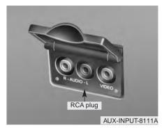
Connecting Other Devices to the RSE Electronic devices such as video game systems, VHS players, Camcorder or etc, can be played through the RSE. These external devices can be connected to the unit via RCA plugs available throughout the vehicle. DC power for additional electronic equipment is provided by one of the 12-volt power outlets located in the dash. Additional information can be found in the vehicle manual.
