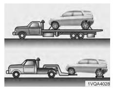
If emergency towing is necessary, we recommend having it done by an authorized Kia dealer or a commercial tow-truck service. Proper lifting and towing procedures are necessary to prevent damage to the vehicle. The use of wheel dollies or flatbed is recommended.
