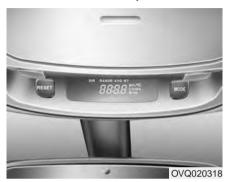
The trip computer is a microcomputercontrolled driver information system that displays information related to driving, including compass, distance to empty, driving time, average fuel consumption and outside temperature on the display when the ignition switch is in ON position. All stored driving information is reset if the battery is disconnected.
