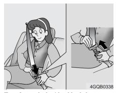
To unfasten the lap/shoulder belt: Press the release button on the buckle and allow the belt to slowly retract.
