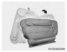
3. Lift the rear portion of the seat cushion then push down firmly to lock the catches into the rear anchors until an audible "click" is heard.
