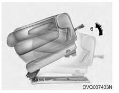
4. Remove the seat while lifting up the rear portion of seat cushion (6).
