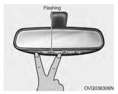
When programming the buttons for the first time, press and hold the left and center buttons ( P, P) simultaneously until the indicator light begins to flash after approximately 20 seconds. (This procedure erases the factory-set default codes. Do Not perform this step to program additional hand-held transmitters.)
