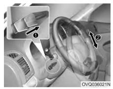
To change the steering wheel angle, pull up the lock release lever (1), adjust the steering wheel to the desired angle (2), then release the lock-release lever to lock the steering wheel in place. Be sure to adjust the steering wheel to the desired position before driving.
