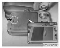
To use the storage compartment of side table, push the cover. Do not fold the table when some items be placed in the storage compartment, since those may damage the items.
