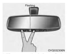
When programming the buttons for the first time, press and hold the left and center buttons (♠,♠) simultaneously until the indicator light begins to flash after approximately 10 seconds. Release both buttons. Do not hold for longer than 20 seconds. (This procedure erases the factory-set default codes. Do Not perform this step to program additional hand-held transmitters.)
