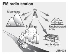
FM broadcasts are transmitted at high frequencies and do not bend to follow the earth's surface. Because of this, FM broadcasts generally begin to fade at short distances from the station.
