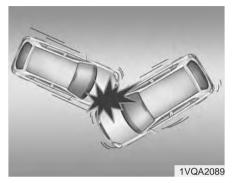
In a slant or angled collision, the force of impact may direct the occupants in a direction between the front and side air bags, and thus the sensors may not deploy any air bags.
