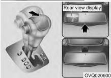
The rearview camera will activate when the back-up light is ON with the ignition switch ON and the shift lever in the R (Reverse) position.
