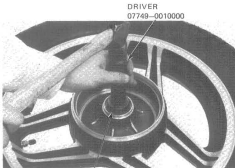
ATTACHMENT, 42 x 47 mm 07746-0010300 PILOT, 17 mm 07746-0040400
