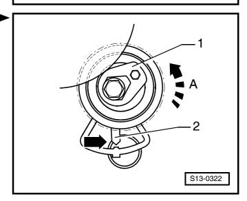
Loosely fit the tensioning pulley with the fixing screw and turn with the Allan screw in the -direction of the arrow-.
