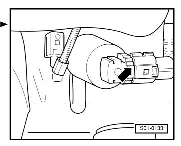
Connect test box -V.A.G 1598/31- to the wiring loom
