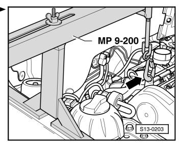
Take up the weight of the engine and remove the fixing screws -A- of the engine console on the support of the cylinder head.
