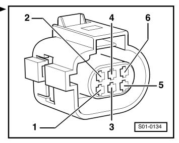
Check wiring between the test box and the plug for interruption according to the Current Flow Diagram.
