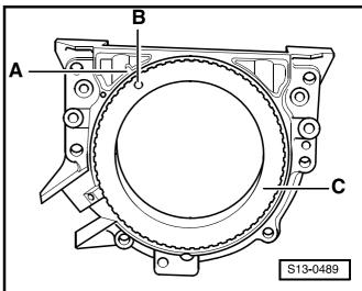
.... or on the sealing flange for the assembly device -T 10134-.
