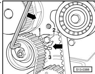
Now rotate crankshaft two revolutions in direction of rotation of engine until it is again positioned at TDC of cylinder 1. The chamfered tooth must correspond with the marking on the sealing flange -arrow- in the fig. -A-.
