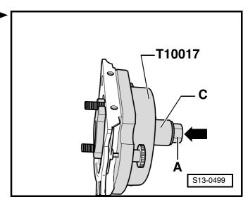
Screw assembly device with Allan screws -A- up to the stop onto the crankshaft flange.
