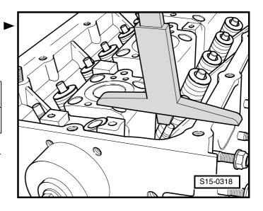
1) The max. permissible reworking dimension is shown in the figures for reworking the valve seats as dimension "b".
