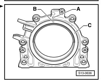
Lay the sealing flange with the front side on theassembly device -T 10017- in such a way that the positioning pin -A- sinks into the hole -B- of the rotor.
