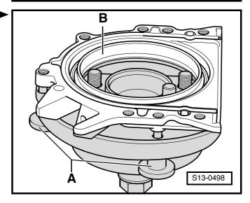
Unscrew hexagon nut -A- up to the end of the thread- ►
