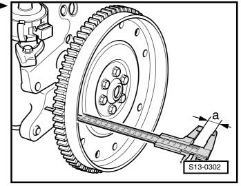
Remove driver disc and use compensating washer
