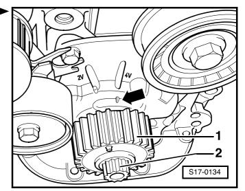
The third tooth to the right -arrow- of the chamfered tooth -A- of the toothed belt gear must be flush with the TDC marking on the oil pump housing.
