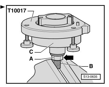
Securing clip -A- from the new sealing flange (flange for assembly device -T 10017-)
