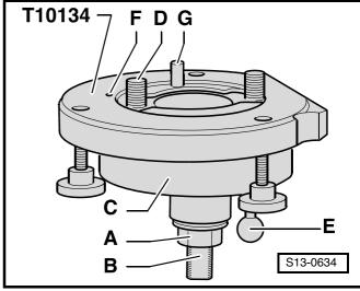
Grip assembly device -T 10017- or -T 10134- on clamping surface -B- of the threaded spindle in a vice.
