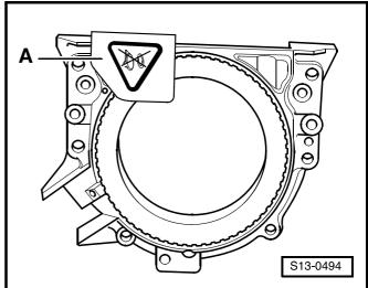
.... or remove from new sealing flange -arrow- for assembly device -T 10134-.
