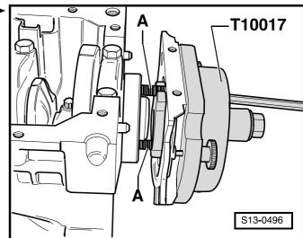
Screw in two M6x35 mm screws -A- by about 3 turns for sealing flange guide into the cylinder block.
