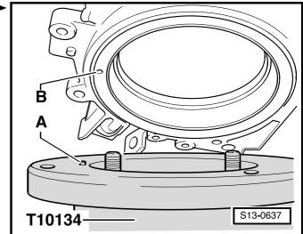
When tightening the knurled screws -A- press the rotor -B- on the surface of the assembly device in such a way that the positioning pin cannot slide out of the rotor hole.
