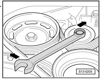
Position clamping lever -MP 1-203-, secure by inserting a pin and and push AC generator towards the crankshaft.
