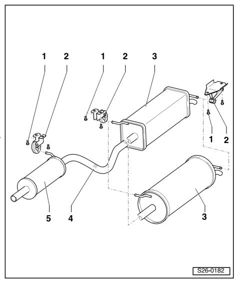
Fig. 1: Separation point at exhaust pipe
