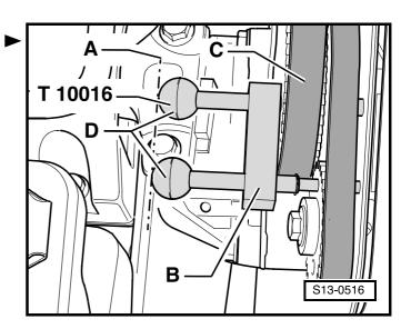
Fig. 2: Checking the axial play of the camshafts
