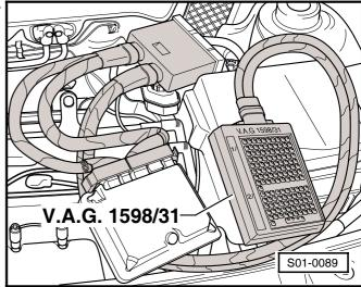
Check the cable from contact -6- of the plug to bush 100 of the test box -V.A.G 1598/31- for interruption.
