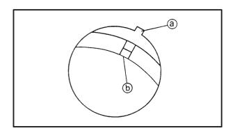
b. Check that the stationary pointer (a) is within the firing range (b) on the generator rotor.
