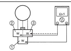
°Measure the stator coil assembly resistances.
