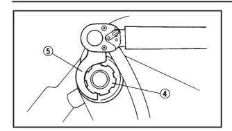
b. Loosen the lower ring nut 4 and then tighten it to specification with a ring nut wrench 5.
