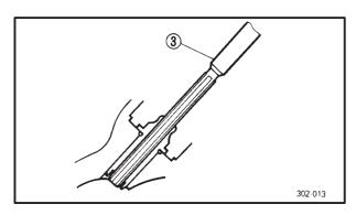
Out of specification  $\rightarrow$  Replace the valve guide.
