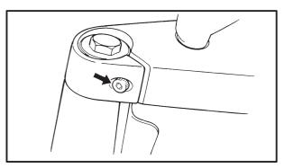
7. Tighten: °Upper bracket pinch bolts
