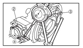
c. Install the final gear backlash band ② and dial gauge ③
