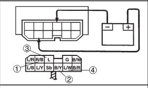
° Does the starting circuit cutoff relay have continuity between blue and blue/white?
