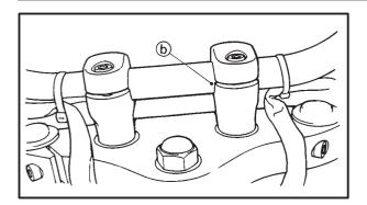
°Align the match marks (b) on the handlebar with the upper surface of the lower handlebar holders.
