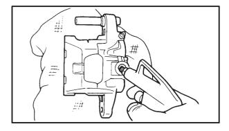
b. Remove the brake caliper piston seals.
