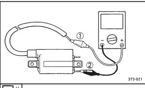
Secondary coil resistance 10.7  $\sim$  14.5 k $\Omega$  20°C (68°F)
