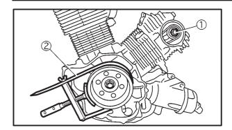
d. Remove the screwdriver, make sure that the timing chain tensioner rod releases, and tighten the cap bolt to the specified torque.
