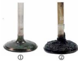
Intake valve: 10,000 miles with TOP TIER Detergent Gasoline
