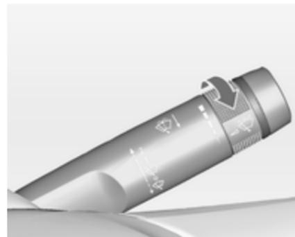
Palanca del limpiaparabrisas en posición
