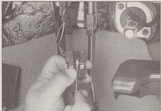
11.8 Pry open the locking tab on the electrical connector and unplug the connector from the switch
