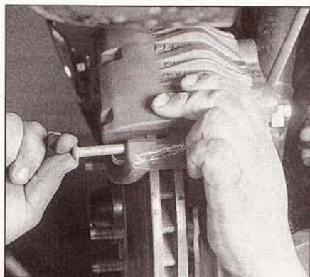
3.7o ... then insert the caliper pin, ...
