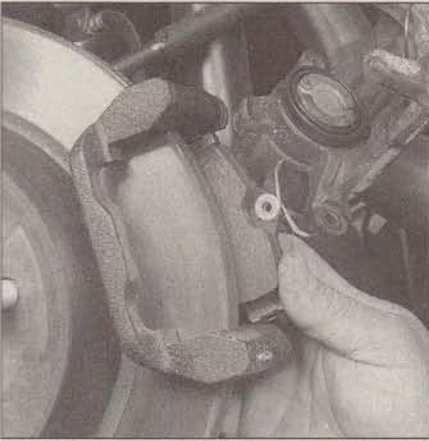
3.8f Remove the inner brake pad
