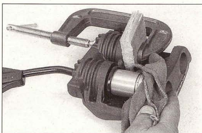
4.22c If the pistons are cocked or stuck, compress one all the way into the caliper, clamp it in place with a small block of wood and a C-clamp and remove the other piston; then move the block of wood and C-clamp to the bore of the piston you just removed and remove the other piston
