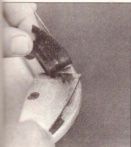
28.2 Be sure to clean all traces of the old gasket from the pan before installing a new one
