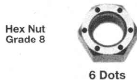
Standard hex nut strength markings
