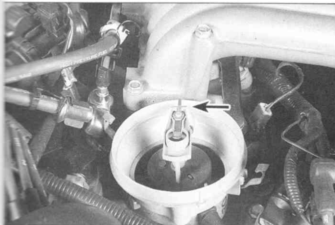
3.7 The rotor tip should be pointing at the mark (arrow) on the distributor
