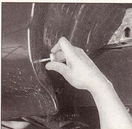
11.4 Detach the retaining screws securing the bumper cover to the inner fenderwell splash shield
