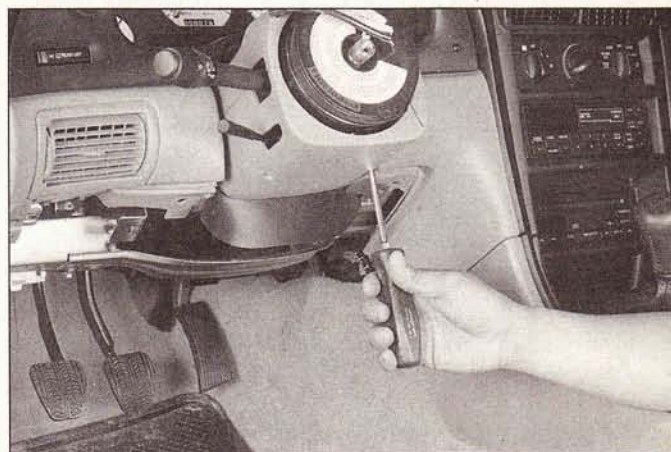
26.3 Detach the screws - then separate the steering column cover halves to remove them from the steering column
