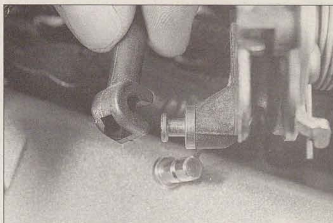
10.3 Remove the cruise control cable from the throttle lever
