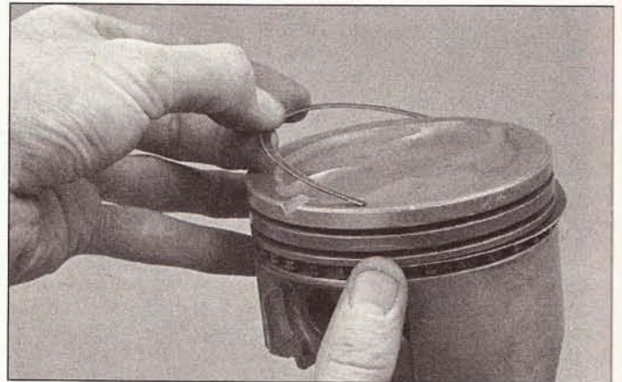
22.8b . . . followed by the side rails - DO NOT use a piston ring installation tool when installing the oil ring side rails
