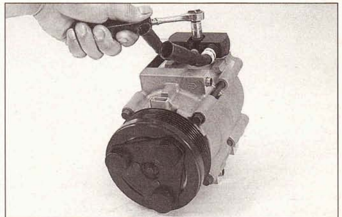
16.3a Unbolt the refrigerant line block from the back of the compressor (shown removed from vehicle)
