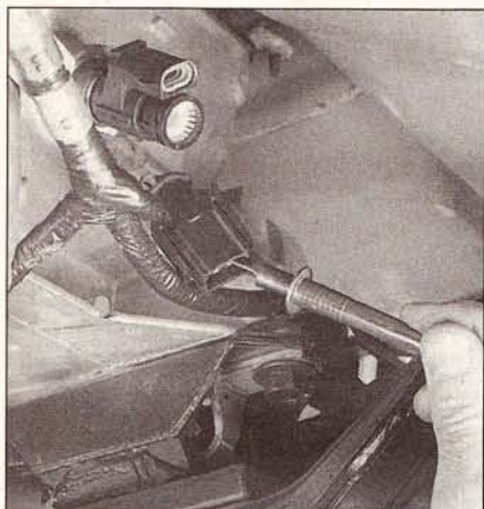
4.52 Disconnect the VSS harness connector and check for battery voltage
