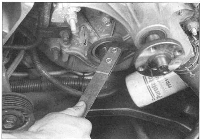
16.6 Use a screwdriver or seal removal tool (shown) to work the seal out of the timing chain cover - be very careful not to damage the cover or nick the crankshaft!
