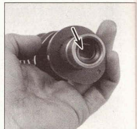
7.5b The camshaft positioning tool is installed at the rear of the camshaft and inserts into a flat-sided hole (arrow)
