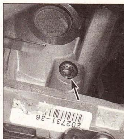
28.5a The block drain plugs (arrow) are generally located about one to two inches above the oil pan rail - there is one on each side of the engine block
