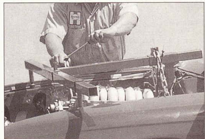
14.7 Raise the engine about two inches front and rear with an engine support fixture
