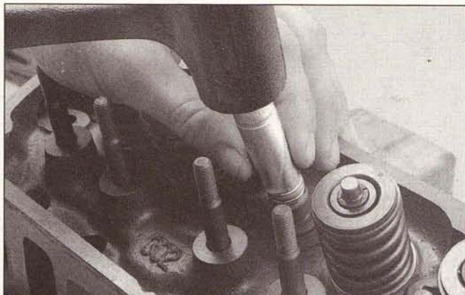
12.3a On pushrod models with the type of seal shown, use a hammer and a seal installer (or a deep socket, as shown here) to drive the seal onto the valve guide/head casting boss (umbrella-type seals don't need to be driven into place)
