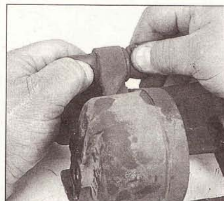
4.14 Push the new dust boots through the holes in the caliper ears, making sure they're installed all the way
