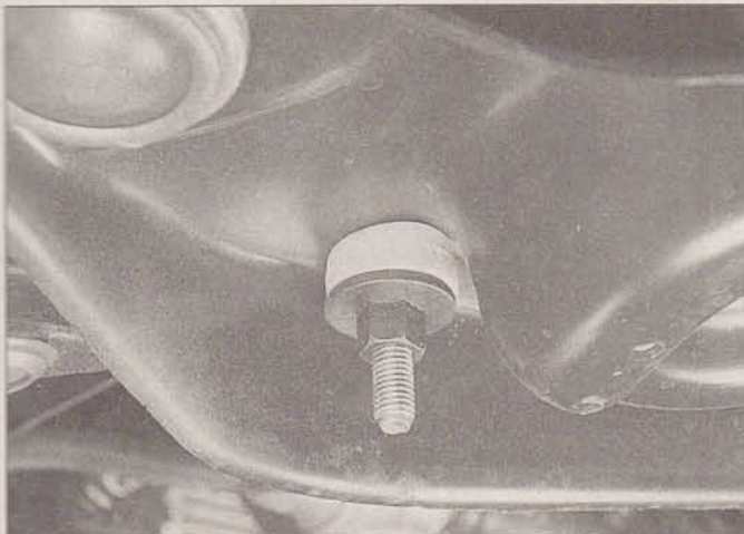
3.2b To disconnect either link from a lower control arm, remove this nut; be sure to note the order in which the washers and bushings are installed
