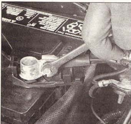
2.1 Detach the battery cables - negative first, then positive
