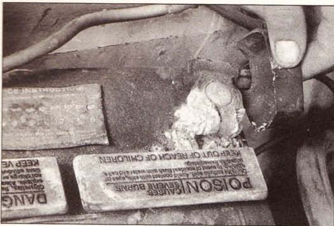
10.6a Battery terminal corrosion usually appears as light, fluffy powder
