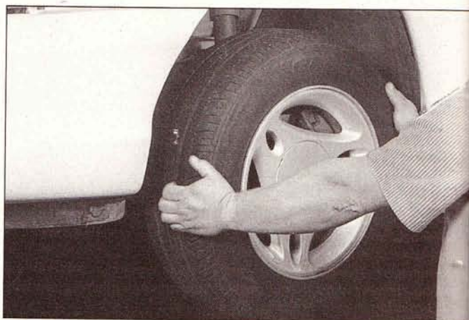
17.11 With the steering wheel in the lock position and the vehicle raised, grasp the front tire as shown and try to move it back-and-forth - if any play is noted, check the steering gear mounts and tie rod ends for looseness
