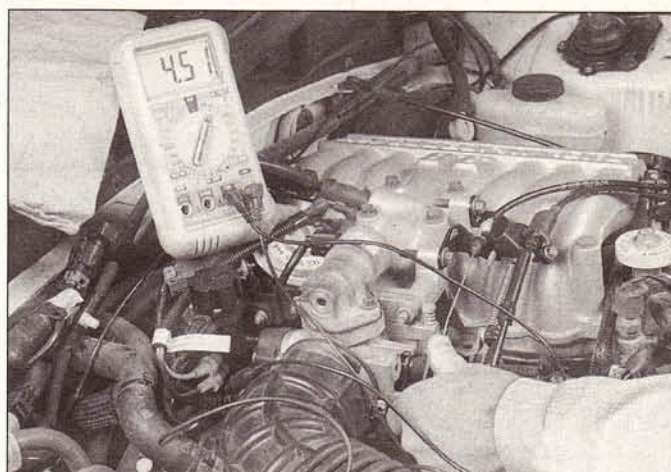
4.24 Rotate the accelerator completely to wide open throttle and observe the voltage increase steadily to 4.5 to 5.0 volts
