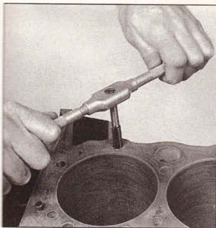
15.8 All bolt holes in the block - particularly the main bearing cap and head bolt holes - should be cleaned and restored with a tap (be sure to remove debris from the holes after this is done)
