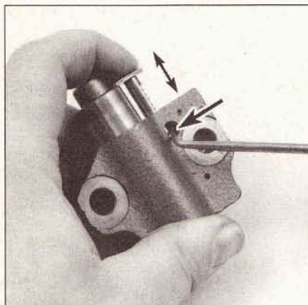
7.16a To fully retract the primary tensioner, release the plunger lock (arrow) and push the plunger into the tensioner body
