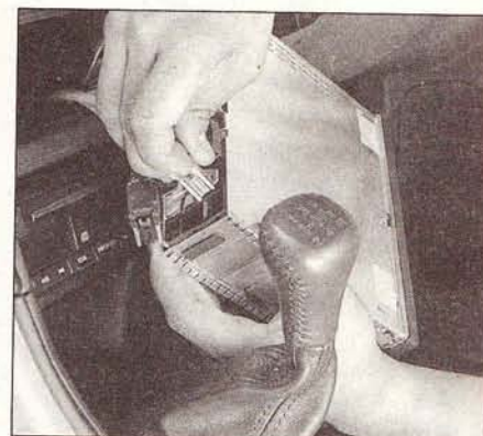
12.3b Detach the electrical connector and the antenna lead from the back side of the radio
