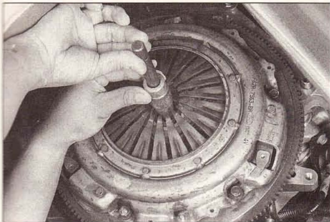
4.16 Center the clutch with an alignment tool, then tighten the bolts in a criss-cross fashion to the torque listed in this Chapter's Specifications
