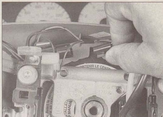
14.6 Unplug the electrical connector for cruise control, if equipped
