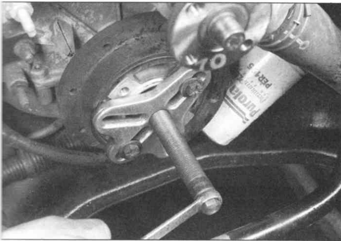
16.5 Use the recommended puller to remove the vibration damper - if a puller that applies force to the outer edge is used, the damper will be damaged!
