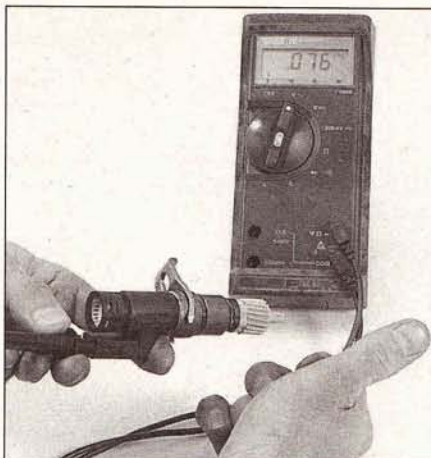
4.53 Remove the VSS and check for a pulsing AC voltage signal as the VSS gear is slowly turned
