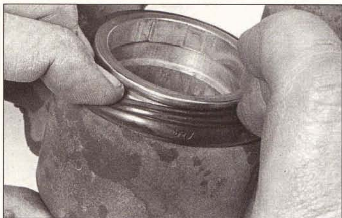
4.21 Install the lip of the dust boot in the groove on the caliper piston
