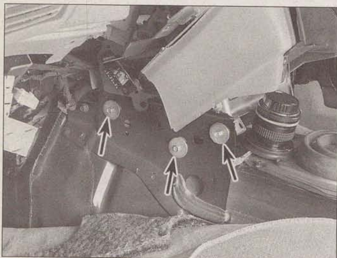
27.7b Peel the carpeting back to access the instrument panel to floor pan bolts
