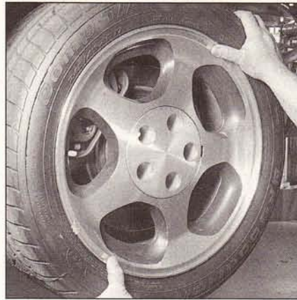
6.3 To check a balljoint, raise the front of the vehicle and place it securely on jackstands, support the lower control arm with a floor jack, then try to rock the wheel in and out; if there's any play in the balljoint, replace it
