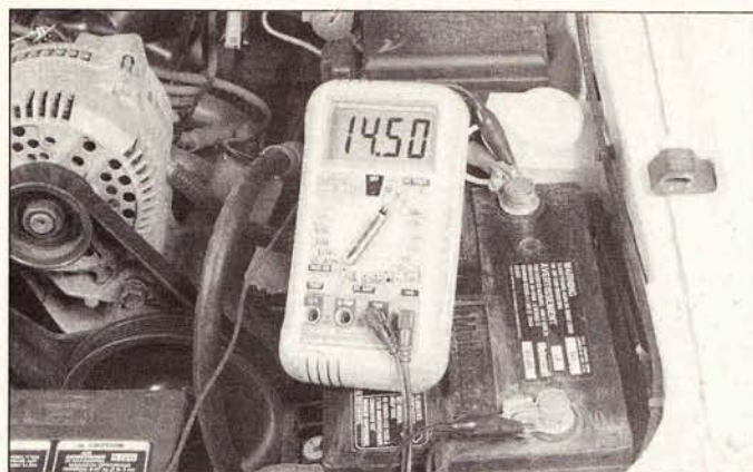
12.2 To measure charging voltage, attach the voltmeter leads to the battery terminals, start the engine and record the voltage reading
