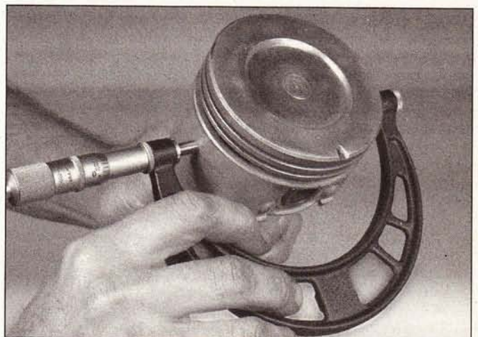
18.11 Measure the piston diameter at a 90-degree angle to the piston pin and in line with it
