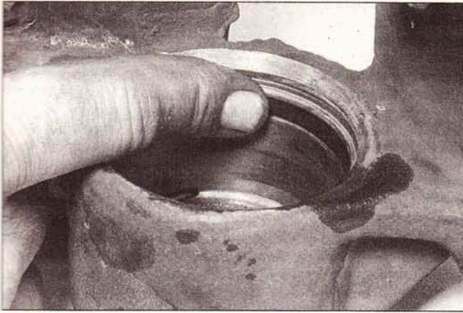
4.17 Push the new seal into the groove with your fingers, then check to see that it isn't twisted or kinked
