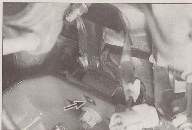
18.13 Make sure the projecting nub on the engine mount is located in the hole (arrow) in the crossmember before tightening the mounting bolts
