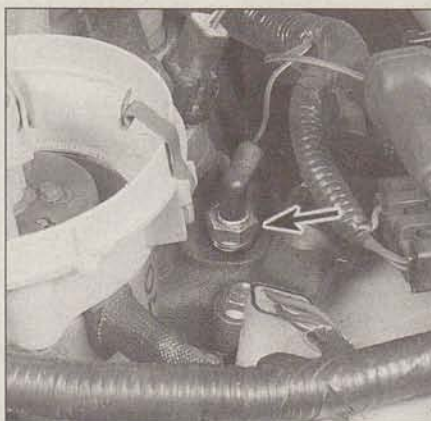
6.1a The coolant temperature sending unit on 5.0L engines is located at the front of the intake manifold near the distributor
