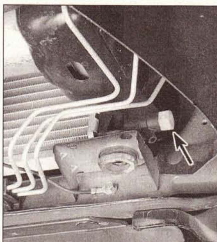
28.4 The radiator drain fitting is located at the lower corner of the radiator (arrow)
