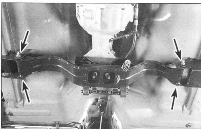
5.10 After you've unbolted the transmission mount from the transmission, raise the transmission slightly and remove the crossmember bolts and nuts (arrows)
