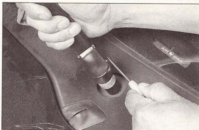
20.7 Pry out the locking tab, then pull straight up to remove the wiper arm assembly
