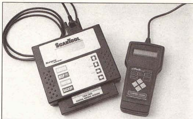
2.2 Scanners like the Actron Scantool and the AutoXray XP240 are powerful diagnostic aids - programmed with comprehensive diagnostic information, they can tell you just about anything you want to know about your engine management system
