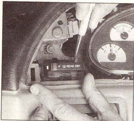
11.13 Detach the retaining clips on each side of the rear defogger switch
