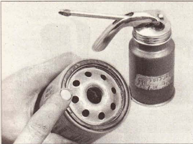
8.16 Lubricate the oil filter gasket with clean engine oil before installing the filter on the engine
