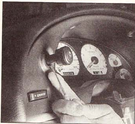
11.3 Using a small screwdriver depress the headlight switch knob retaining clip
