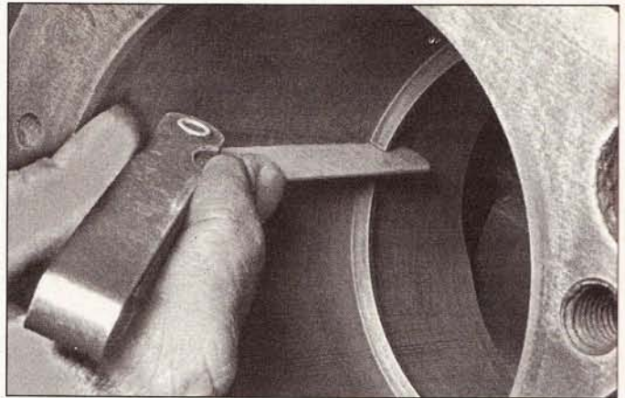
22.4 With the ring square in the cylinder, measure the end gap with a feeler gauge
