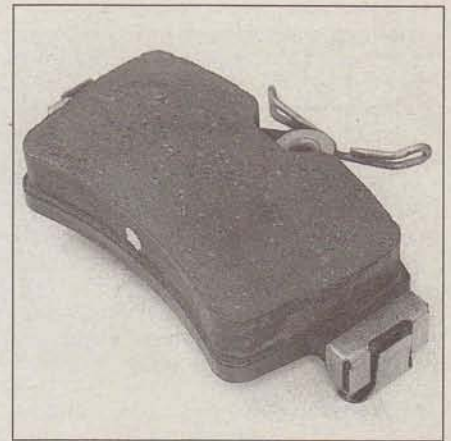
3.8h ... and swap them over to the new pads; make sure they're installed exactly as shown
