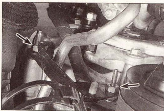
16.3b At the front of the compressor, remove these two nuts (arrows) to release the support bracket on the line carrying the inline filter - this view is looking up from below
