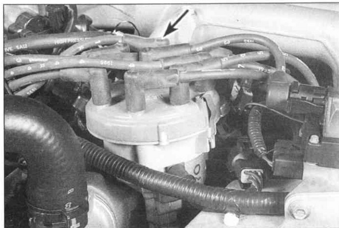
3.4 Make a mark on the distributor body directly below the number 1 plug spark plug wire terminal (arrow)
