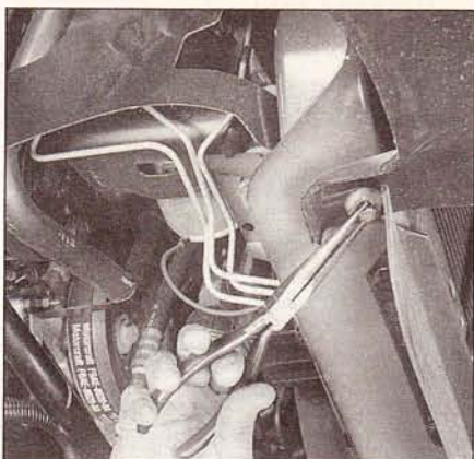
11.3 Pull downward on the center pin to release the clips from the lower edge of the bumper cover
