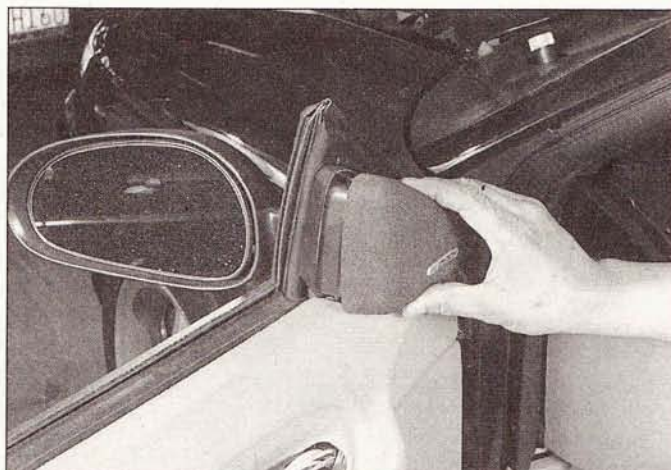
17.6a Pull straight out to remove the side view mirror trim cover or speaker cover (if equipped)
