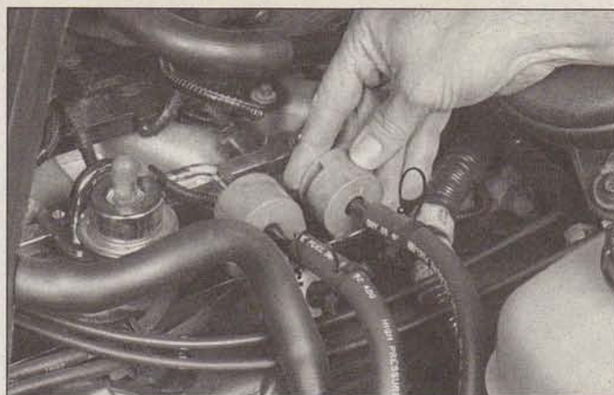
13.36b Install the correct diameter spring lock coupling tool and push away from the fuel rail to release the internal locking mechanism
