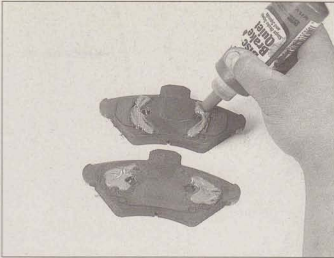
3.6h Apply some anti-squeal compound to the backing plates of the new pads
