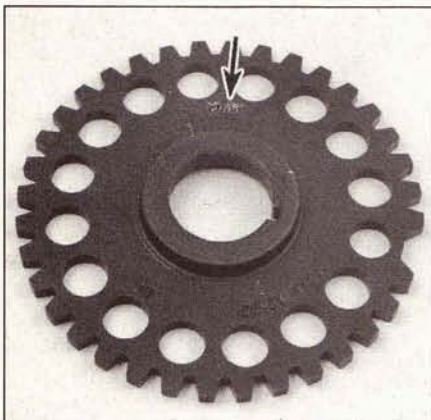
7.4 The crankshaft sensor tooth wheel has a specific direction to be installed, look for the word "rear" stamped in (arrow)
