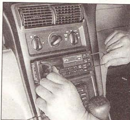
12.3a Insert the tools until they seat, then push outward simultaneously on both tools to release the clips and withdraw the radio from the dash
