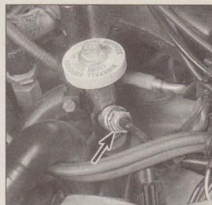
6.1b Coolant temperature sending unit (arrow) location - V6 models
