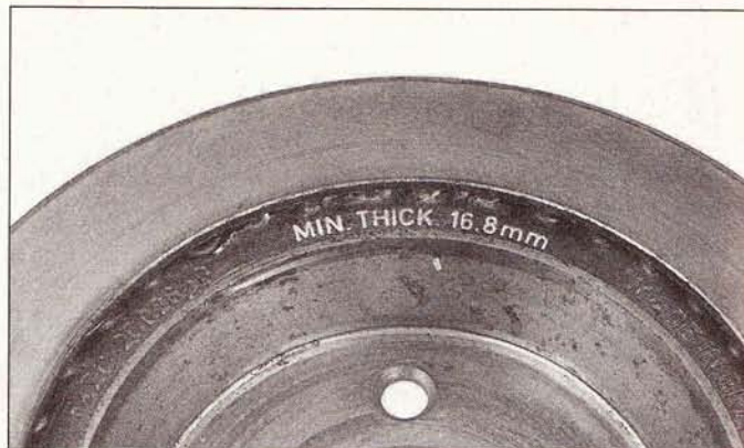
5.6a The minimum thickness limit is cast into the inside of the disc
