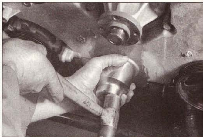
17.6 There is special tool for installing the front oil seal into the timing chain cover, but if the tool is unavailable a large socket (the same diameter as the seal) can be used to drive the seal into place
