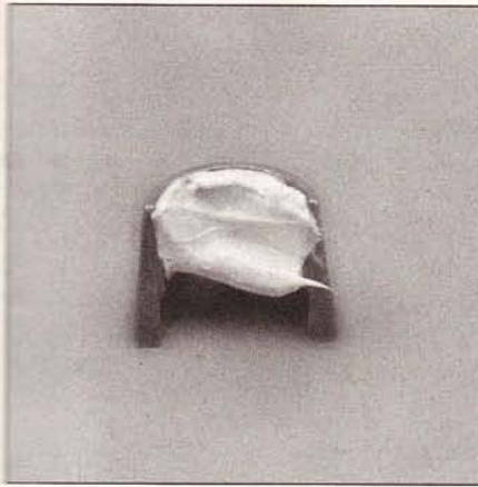
12.7a Apply a small dab of grease to each keeper as shown here before installation - it'll hold them in place on the valve stem as the spring is released
