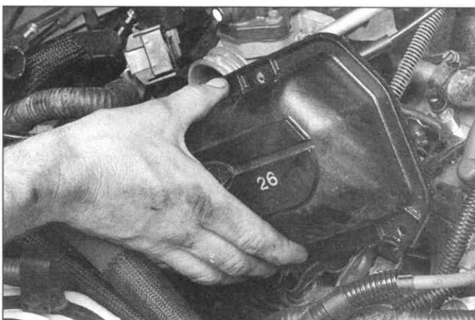
4.7b Move the hoses and slip the cover off (V6 engine shown, V8 similar)
