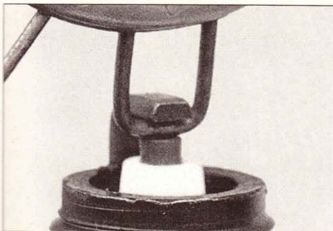
30.5a Spark plug manufacturers recommend using a wire-type gauge when checking the gap - if the wire does not slide between the electrodes with a slight drag, adjustment is required
