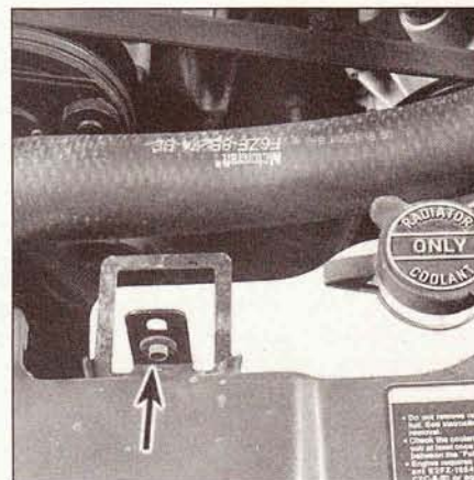
5.2a Location of the coolant reservoir on V6 and 5.0L models - arrow indicates upper mounting bolt (the bottom of the reservoir is secured by a tab that fits into a lower bracket)
