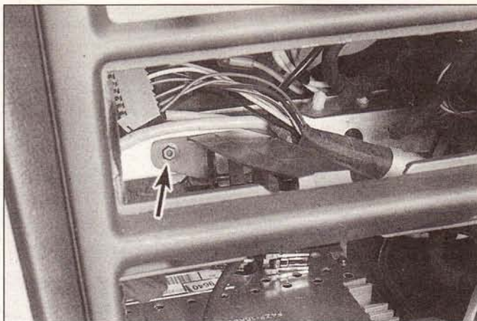
25.7b Remove the screw (arrow) located behind the radio
