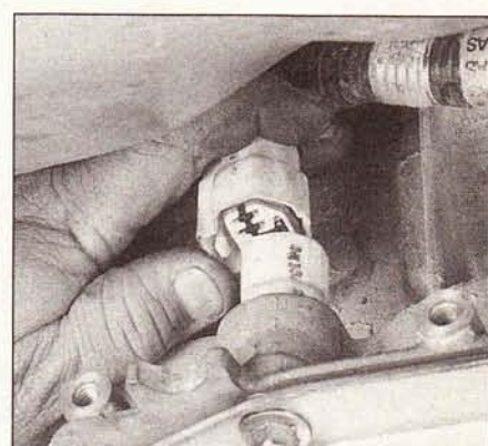
6.10c ... and the torque converter clutch solenoid
