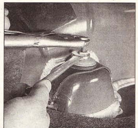
10.3 Locate the upper retaining nut for the shock absorber inside the trunk; to prevent the piston rod from turning, hold it with a wrench or locking pliers while you break loose the nut
