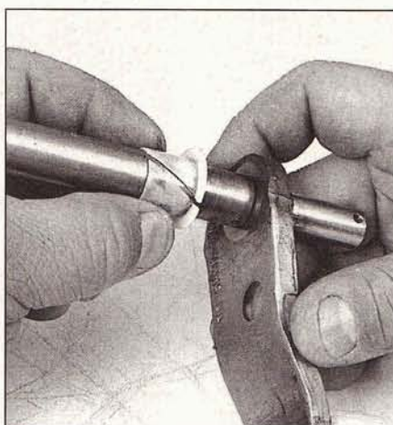
3.25b ... and the right shaft bushing; inspect both bushings for cracks and wear, and replace them if necessary
