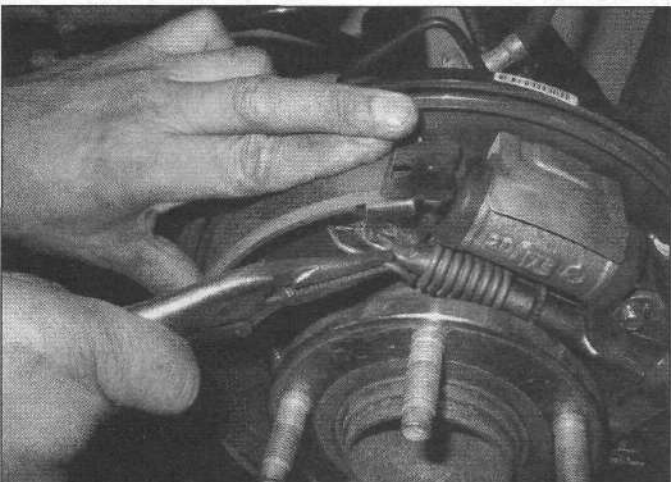
6.6w Attach the upper return spring to the hole in the front shoe
