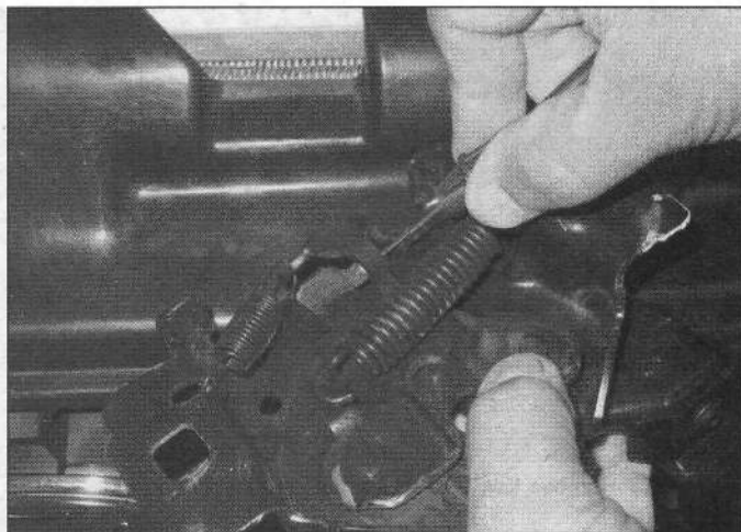
10.2b Remove the cable end from the slotted portion of the latch mechanism
