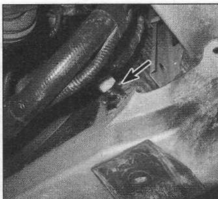
22.4 The radiator drain fitting is located at the bottom of the radiator - before opening the valve, push a short length of rubber hose onto the plastic fitting to prevent the coolant from splashing
