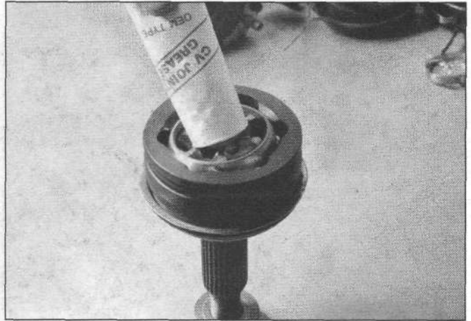
9.25a Pack the outer CV joint assembly with CV grease . . .
