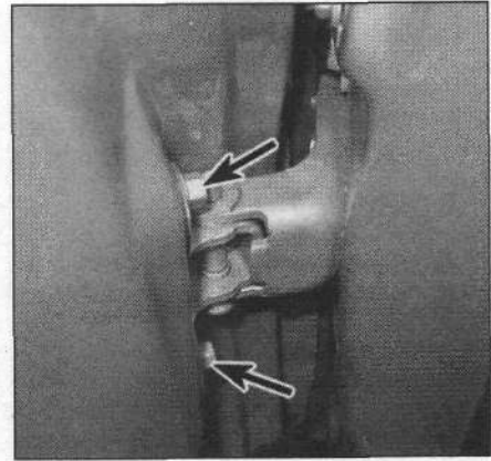
16.8 Remove the door hinge bolts with the door supported (bottom hinge similar)
