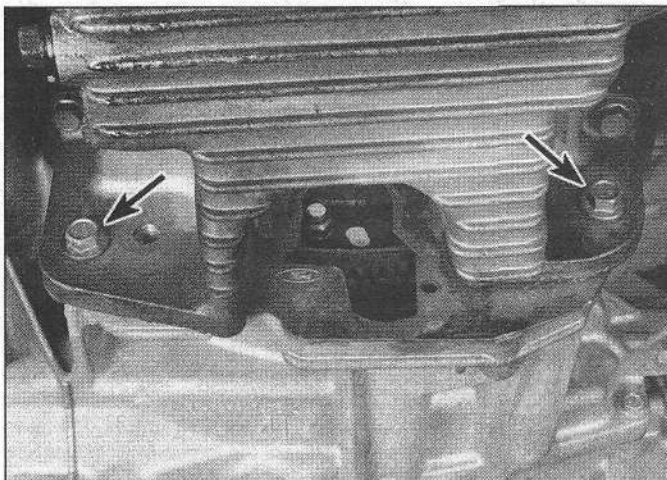
12.8a Remove these bolts that secure the oil pan to the transaxle . . .
