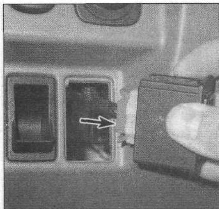
9.8 Disconnect the electrical connector from the instrument panel dimmer switch and remove the switch
