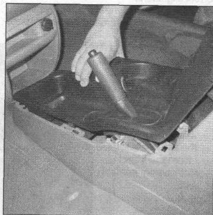
23.3 Remove the finish panel from the console by carefully lifting the edges out of the locking tabs
