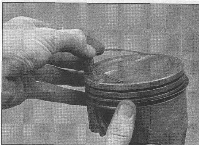
9.19b DO NOT use a piston ring installation tool when installing the oil control side rails
