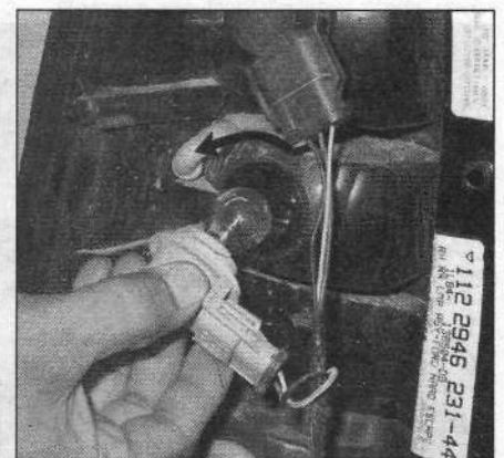
19.12b To remove a brake/tail light, turn signal or back-up light bulb socket, turn it counterclockwise 1/4-turn and pull it out
