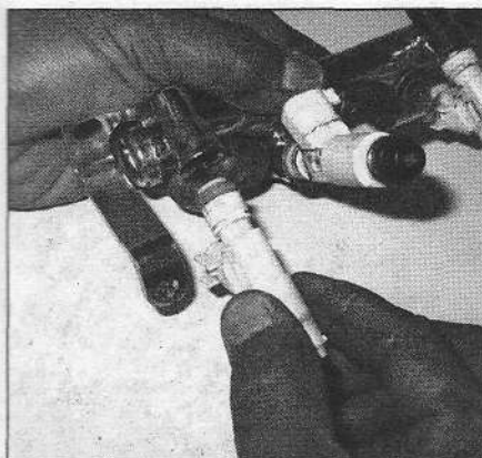
14.21 To detach an injector from the fuel rail, simply wiggle it side to side a little to loosen the O-ring and then pull it straight out as shown (V6 models)
