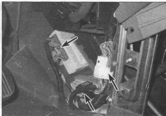
26.15 Disconnect the instrument panel connectors below the center dash
