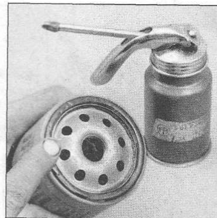
6.15 Lubricate the oil filter gasket with clean engine oil before installing the filter on the engine
