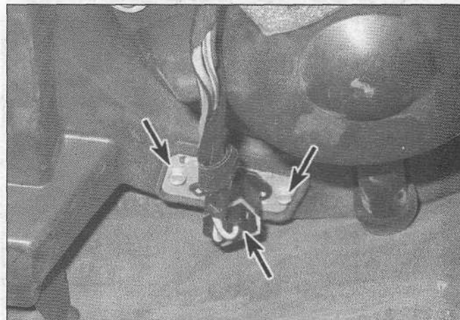
10.2 Unplug the blower motor resistor connector, then remove the mounting screws
