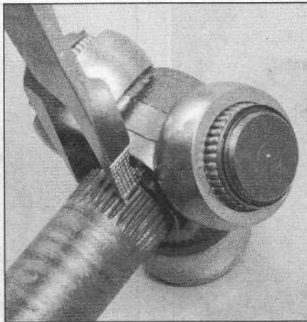
9.6a Spread the ends of the stop-ring apart and slide it towards the center of the shaft ...
