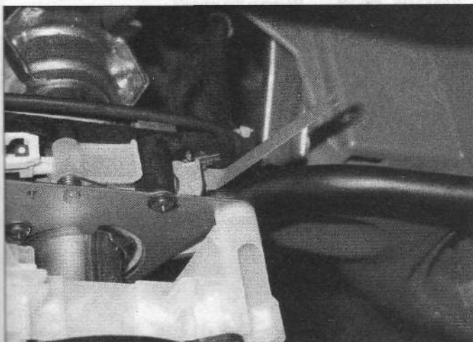
4.7 Insert a feeler gauge between the shift lever and the shift lever detent
