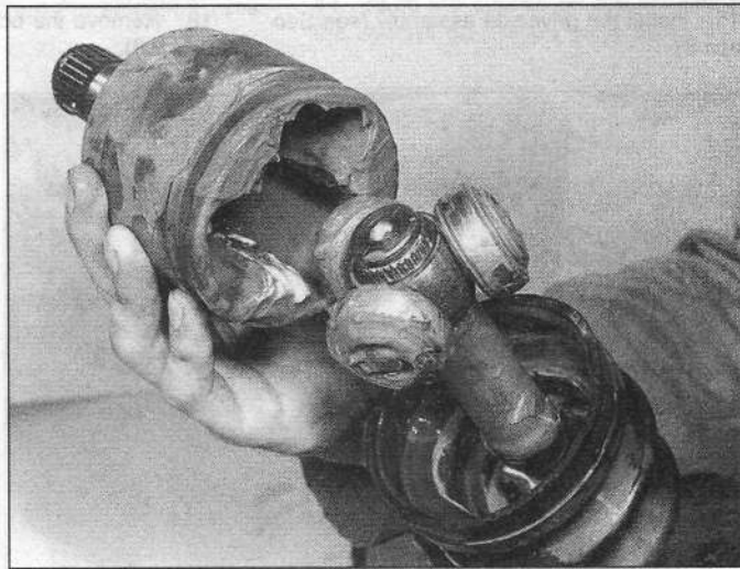
9.14 Pack the outer race with CV joint grease and slide it over the tri-pod assembly - make sure the match marks on the CV joint housing and tri-pod line up
