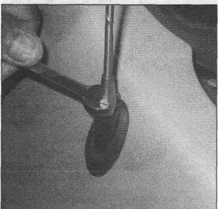
13.1 Unscrew the antenna mast with a 10 mm wrench
