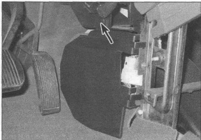
26.14 Remove the cover panel fastener
