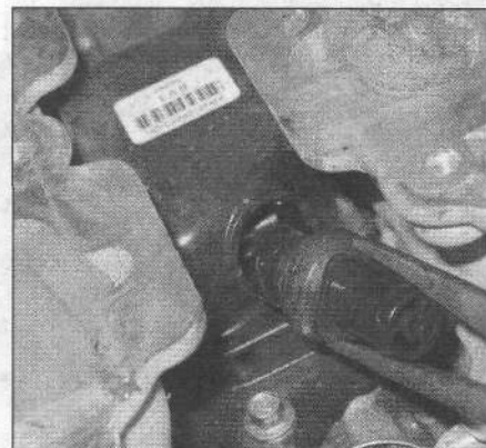
22.29 Unscrew the PCV valve to remove it from the crankcase vent oil separator (V6 models)
