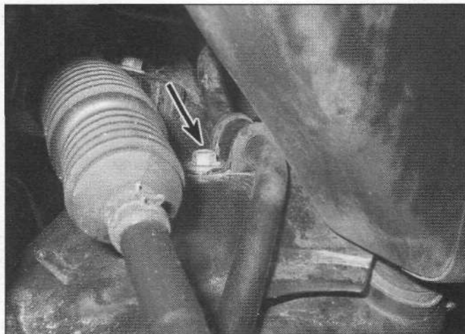
4.3 Stabilizer bar bracket bolt (other bolt not visible in photo)
