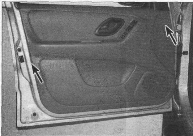
15.4b Location of the front door panel screws
