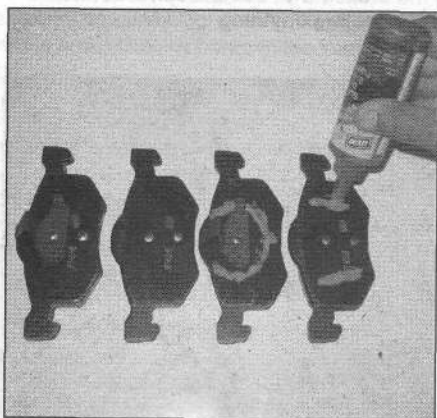
3.6j Apply anti-squeal compound to the back of the pads
