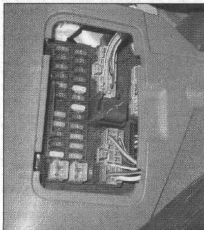
3.1c The passenger compartment fuse/relay box is located either in the left kick panel as shown, or on the right-hand side of the center console. It contains fuses and relays
