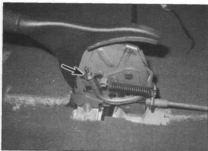
12.3 Turn the adjusting nut until the desired handle travel is obtained (center console removed for clarity)
