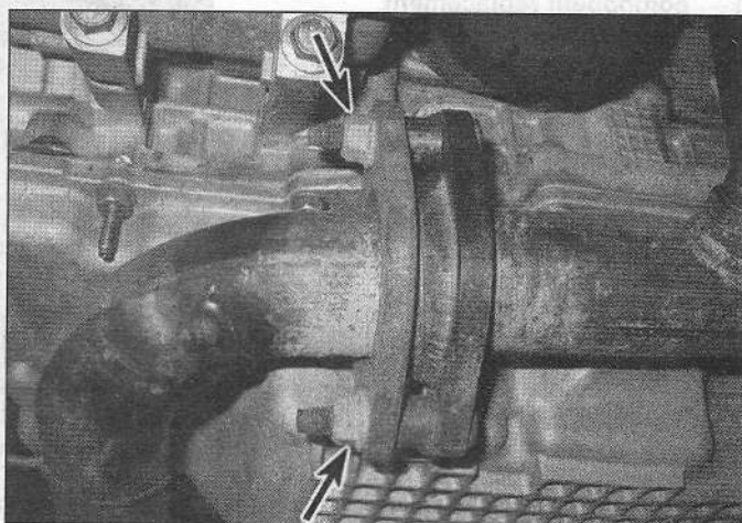
15.23 To disconnect the front flange of the crossover and flexible exhaust pipe from the exhaust manifold/catalytic converter for the front cylinder head, remove these two nuts
