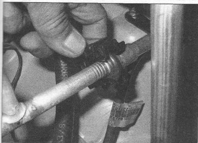
18.2a Remove the protective cover from the air conditioning line coupling
