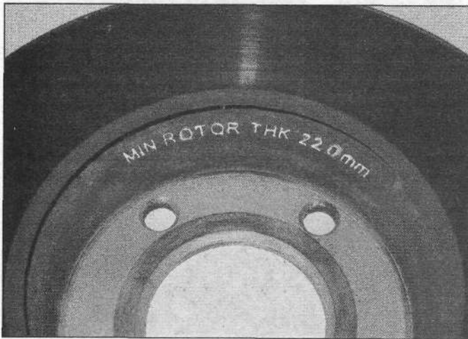
5.5a The minimum thickness dimension is cast into the back side of the disc
