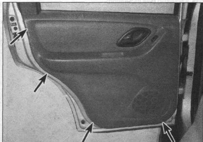
15.4c The rear door panel is not secured with mounting screws - carefully pry the door panel using a flat-bladed screwdriver or door panel tool until the door clips release
