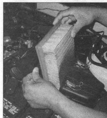
18.1b . . . pull the cover out of the way and lift the element out
