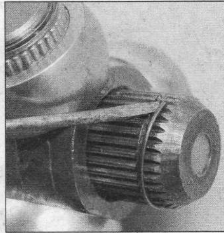
9.6b ... then slide the tri-pod assembly back and remove the retainer clip
