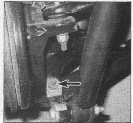
9.5 Remove the nut from the lower ballstud
