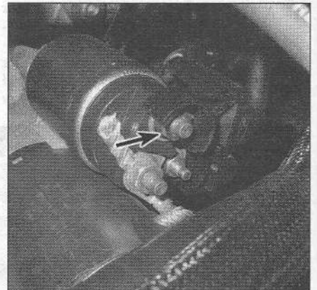
4.4c To disconnect the lower end of the positive battery cable from the starter solenoid, remove this nut (V6 model shown, other models similar)
