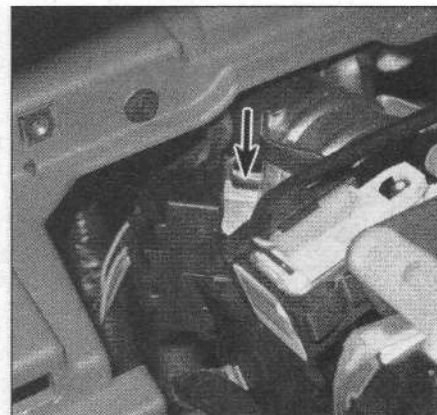
7.14a To remove the ignition switch from the steering column housing, release this button on top ...
