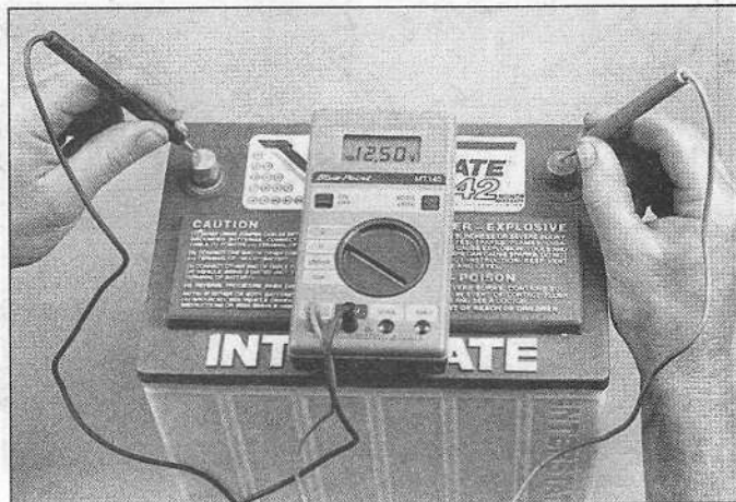
3.1b To test the open-circuit voltage of the battery, connect the black probe of a voltmeter to the negative terminal and the red probe to the positive terminal of the battery; if the battery is fully charged, the voltmeter should indicate about 12.5 volts (depending on the outside air temperature)
