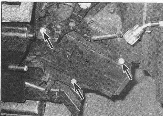
12.6 Remove the screws and detach the cover from the HVAC housing
