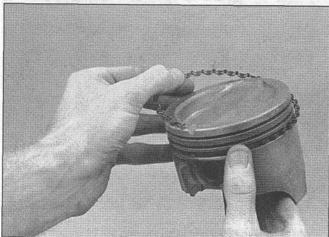
9.19a Installing the spacer/expander in the oil ring groove
