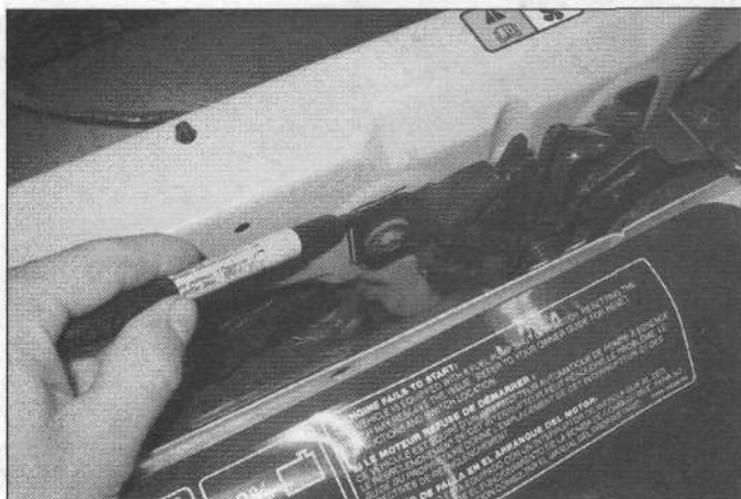
9.9 To adjust the hood latch horizontally or vertically, draw a reference mark and loosen the latch bolts
