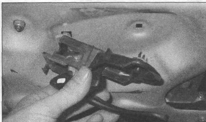
17.25b ... and separate the door handle from the door
