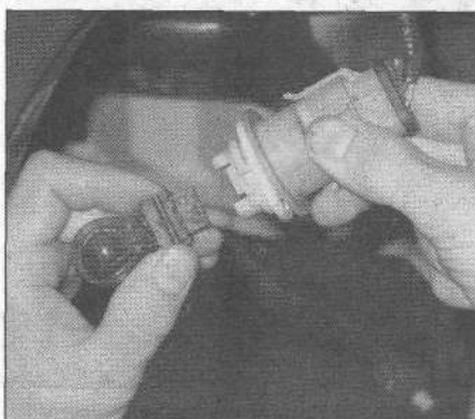
19.4 To remove the turn signal bulb from the bulb holder, pull it straight out of the holder
