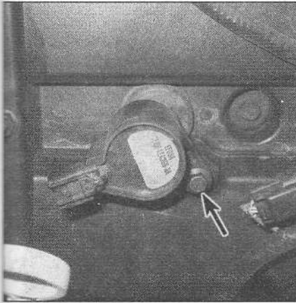
7.9 To detach an ignition coil from the valve cover, remove this bolt
