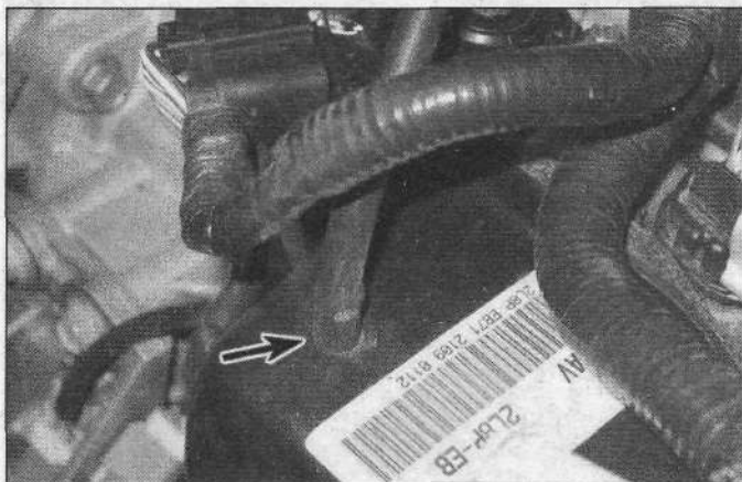
6.27 Remove the transaxle vent tube from the valve body cover
