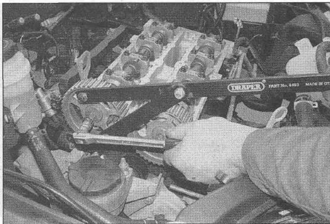
9.32 Use a sprocket holding tool while loosening the camshaft sprocket bolts
