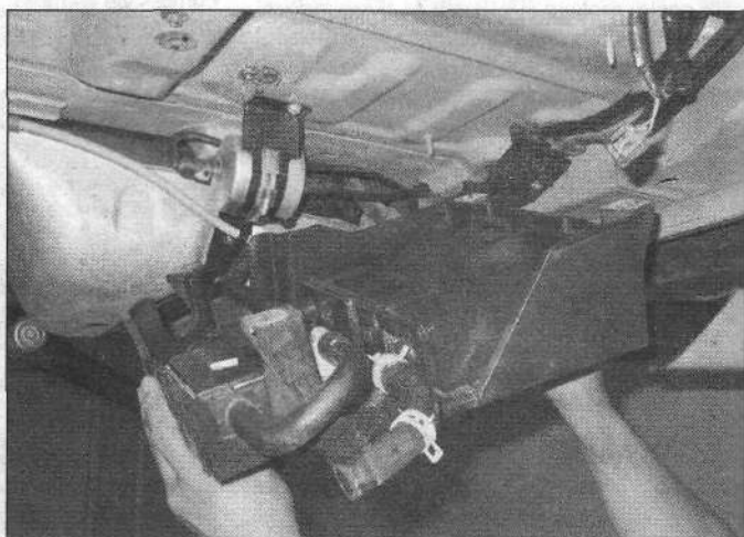
20.33c . . . and then lower the EVAP canister, the mounting bracket and the rest of the EVAP system components as a single assembly
