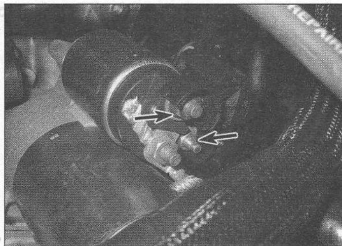
13.13 Disconnect the battery starter cable from the big terminal and the starter control cable from the smaller terminal (V6 models)
