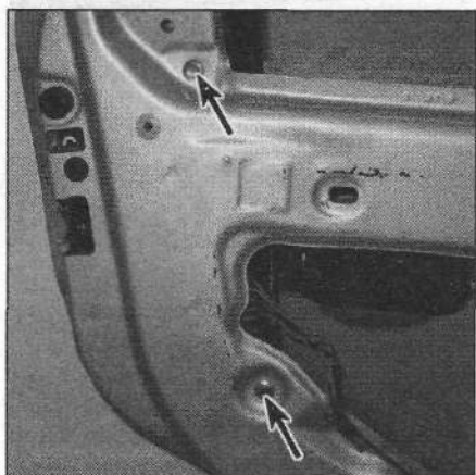
17.15 Remove the screws on the door glass top run
