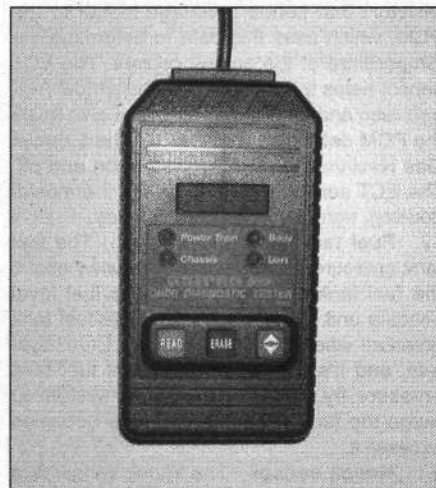
2.2 Trouble code readers like the Actron OBD-II diagnostic tester simplify the task of extracting the trouble codes
