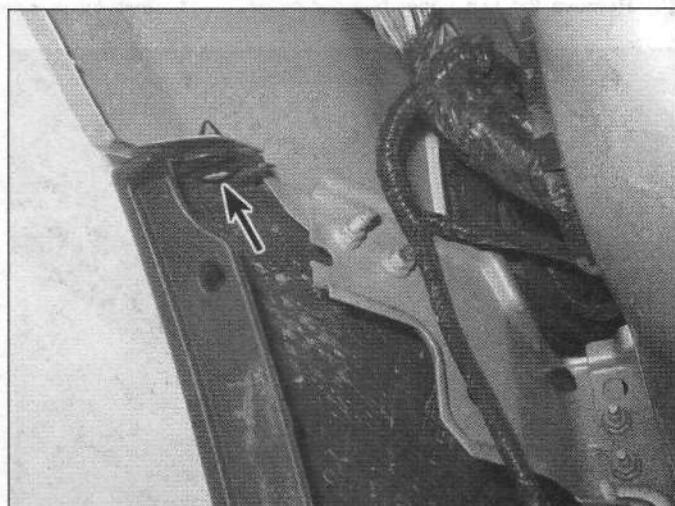
11.4 Remove the cover-to-fender retainers from each side of the vehicle
