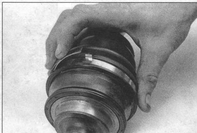
9.17a To install new fold-over type clamps, bend the tang down . . .
