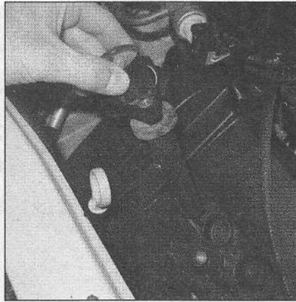
7.10 To remove an ignition coil from the valve cover, pull it straight up
