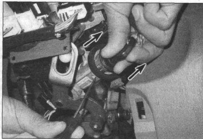
7.3b . . . through this hole in the steering column housing, then depress the release button on the lock cylinder and pull out the lock cylinder (steering column cover removed for clarity)
