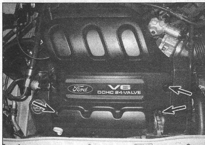
7.7 To detach the engine cover, remove these three nuts (V6 models)
