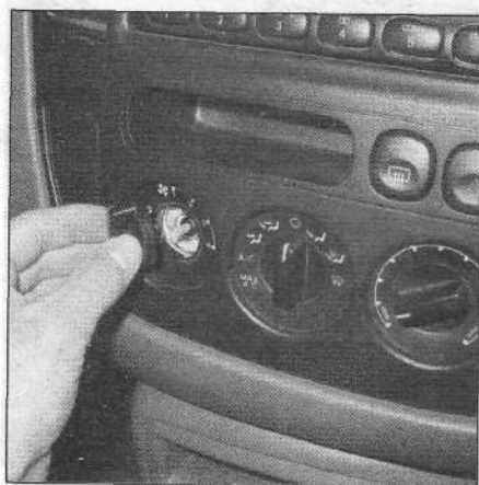
24.11 Remove the climate control knobs from the control assembly
