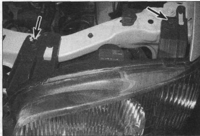
17.5 To detach the upper part of the headlight housing from the upper radiator crossmember, remove this bolt and nut
