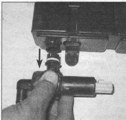
20.36a To separate the vent solenoid from the EVAP canister, simply pull the solenoid straight out
