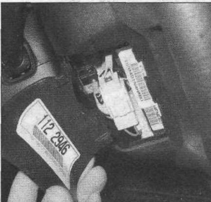
12.2 At the bottom of the steering wheel, open the cover to gain access to the airbag harness
