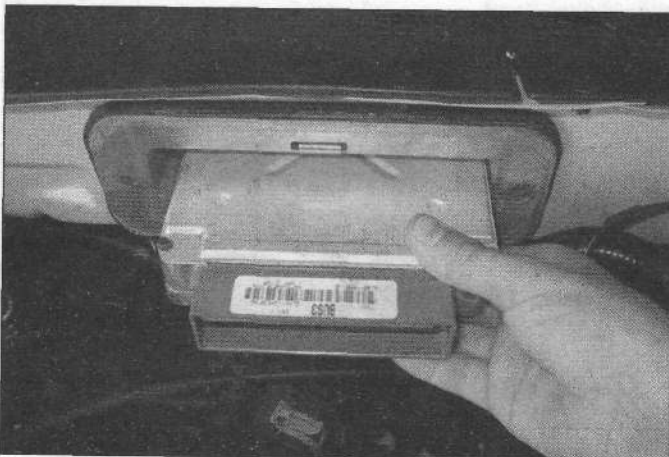
17.5 Carefully remove the PCM from its receptacle in the firewall
