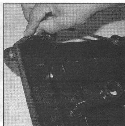
4.10 Press the new gasket into the groove in the valve cover, making sure it isn't twisted
