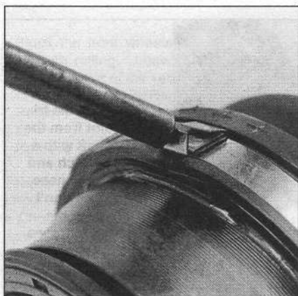
9.17b . . . and flatten the tabs to hold it in place
