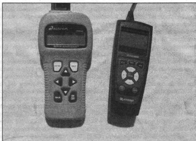
2.1 Scanners like these from Actron and AutoXray are powerful diagnostic aids - they can tell you just about anything you want to know about your engine management system
