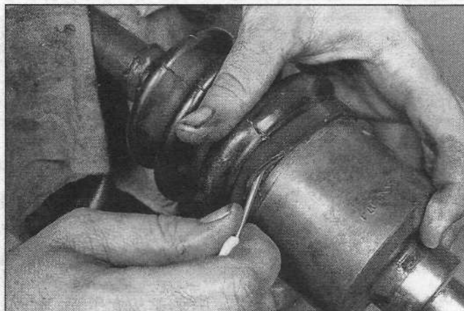
9.16 Equalize the pressure inside the boot by inserting a small, dull screwdriver between the boot and the outer race
