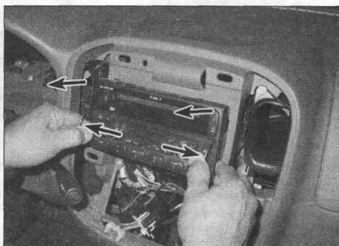
12.3 Push outward on both radio removal tools and simultaneously pull out the radio
