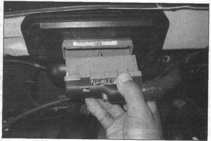
17.3b . . . then pull the connector straight out
