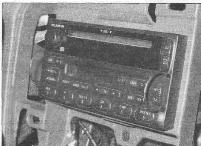
12.2b Insert the special radio removal tools into the holes at each end of the radio as shown, then push them in until you feel the internal clips release
