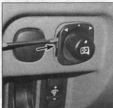
9.2 Carefully pry the left/right power mirror adjustment switch from the dash with a small screwdriver (the switch is secured to the dash by a small metal tab on each side)
