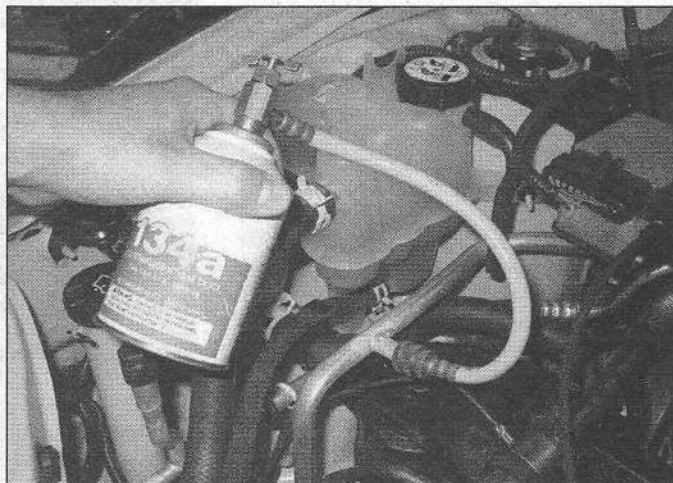
13.12 Cans of R-134A refrigerant (available at auto parts stores) can be added to the low side of the air conditioning system with a simple recharging kit (V6 engine shown)
