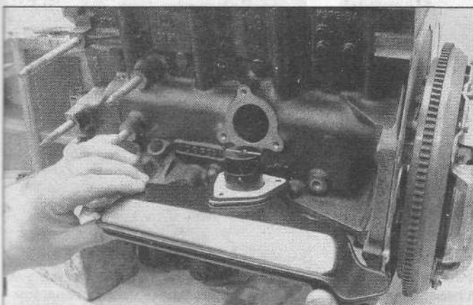
22.16b . . . and pull off the separator and the old gasket
