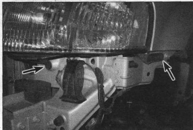
17.4 To detach the lower part of the headlight housing from the vehicle, remove these two bolts
