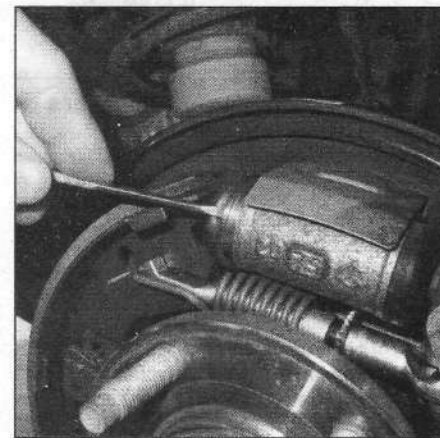
13.17 Carefully peel back the wheel cylinder boot and check for leaking fluid indicating that the cylinder must be replaced or rebuilt
