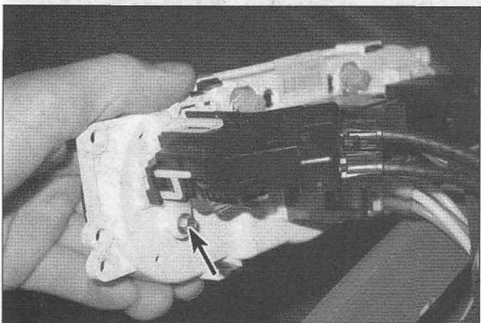
11.4a Remove the temperature blend door control cable mounting screw and separate the cable assembly from the control assembly
