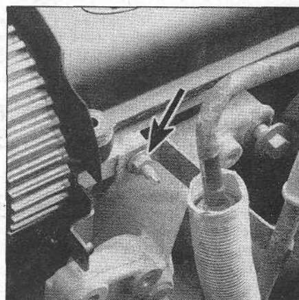
13.14 Remove the nut that secures the dipstick tube
