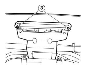
**NOTE** During reassembly, correctly set the protective screen in its housing.
