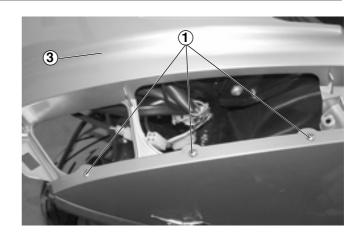
Unscrew and remove the three screws (2), taking care to recover the washers and ferrules.
