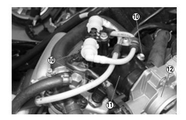
Unscrew and remove the three screws (13) fixing the throttle body (12) to the intake manifold (11).
