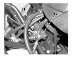
Operate the brake lever until the reservoir is completely free from air bubbles.
