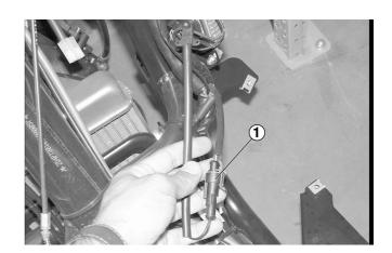
Measure the electrical resistance with an ohm meter (scale 0-20 kΩ) between the connector terminals (1).
