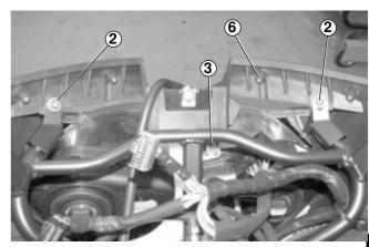
Disconnect the electrical connection (5). Remove the complete lighting assembly (6).
