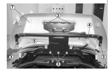
Disconnec the electrical connection from the bulbs (6) and the third stoplight.
