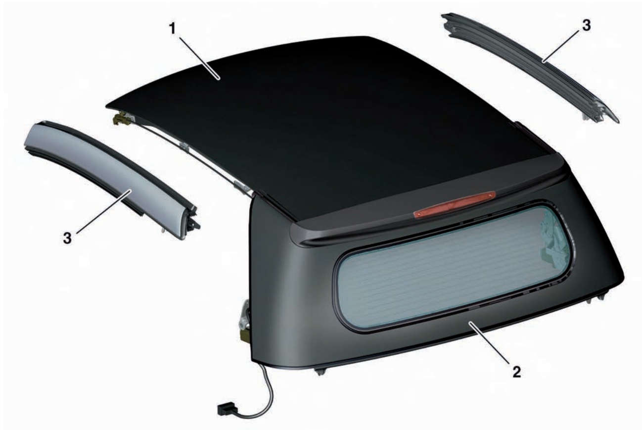
Components of Tritop textile soft top
