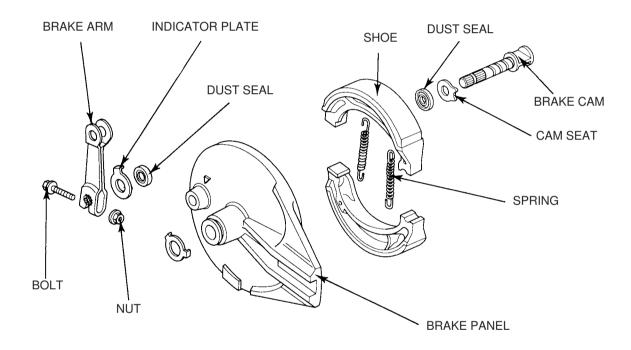
Apply grease to the lip of dust seals, then install them into the brake panel.
