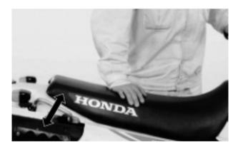
Support the motorcycle using a workstand. Move the rear wheel sideways with force to see wheel bearings are worn.
