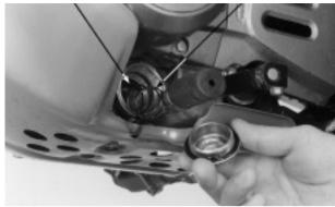
Install and tighten the oil filter screen cap to the specified torque.
