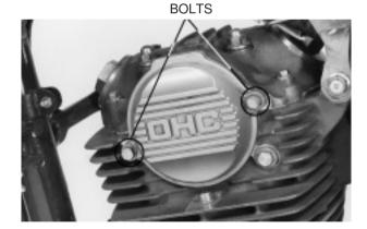
Install and tighten the timing hole cap and crankshaft hole cap.
