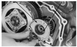
OIL FILTER ROTOR LOCK NUT
