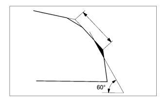
Install a 45 degree finish cutter and cut the seat to proper width. Make sure that all pitting and irregularities are removed. Refinish if necessary.
