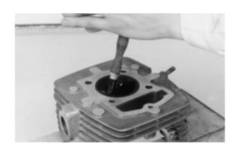
Remove the tool and inspect the width of each valve seat.
