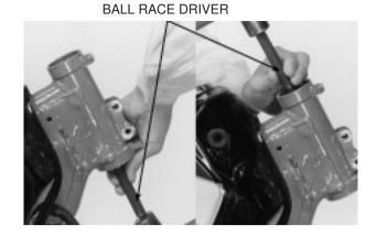
Install the new bearing races using the special tools.
