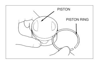
Temporarily install the piston rings in their proper positions with the marks facing up.
