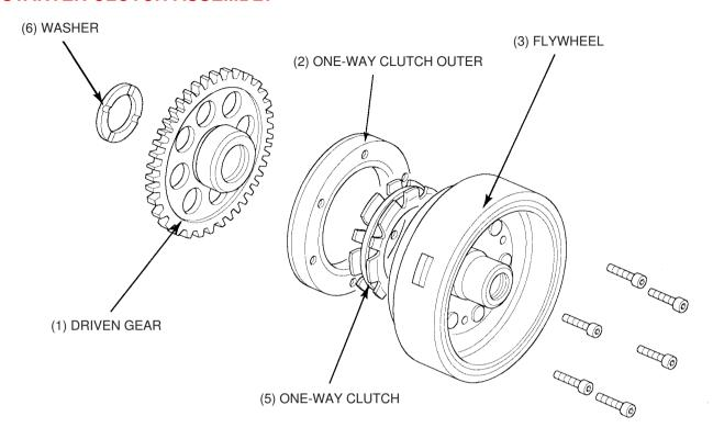
Apply clean engine oil to the one-way clutch rollers. Install the one-way clutch in the clutch outer facing its flange toward the flywheel.
