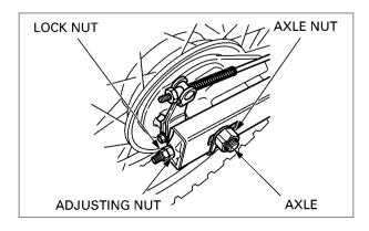
Install the brake rod spring, joint piece, brake rod and adjusting
