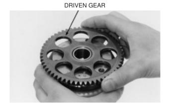
Inspect the starter driven gear teeth for damage or abnormal wear.
