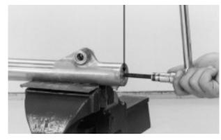
Remove the dust seal and stop ring.
