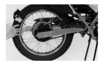
Move the swingarm side ways with force to see swingarm bushings are worn.
