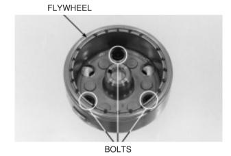
Check the one-way clutch rollers for wear or damage.
