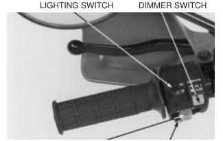
TURN SIGNAL SWITCH HORN SWITCH
