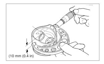
Measure the piston pin bore I.D. in two direction at right angle to each other.
