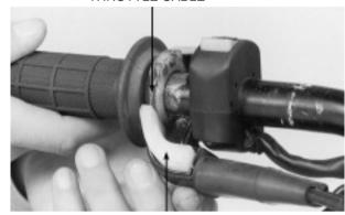
Install the screws and tighten the forward screw first, then the rear screw.
