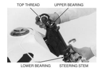
Tighten the top thread until it is sung against the top cone race.
