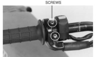
Place the front master cylinder on the handlebar and install the
