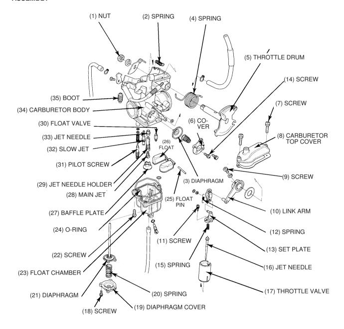
Install the diaphragm onto the carburetor body.
