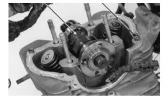
Remove the camshaft. Remove the dowel pins.
