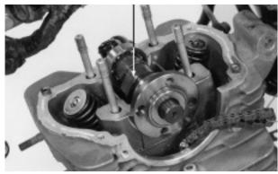
Apply sealant to the mating surface of the cylinder head cover.
