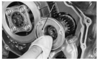
Clean the oil filter rotor. Check the oil through pipe operates freely, without binding. If necessary, remove the B-clip and replace faulty part. Install the oil filter rotor.
