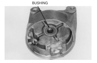
Check the dust seal and bushing of the front cover for wear or damage.
