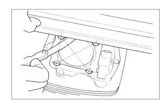
Inspect the cylinder bore for wear or damage.
