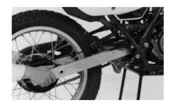
Check the shock absorber for leaks or damage. Tighten all rear suspension nuts/bolts to the specified torque values (page 1-5).
