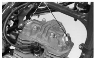
Remove the timing hole cap.
