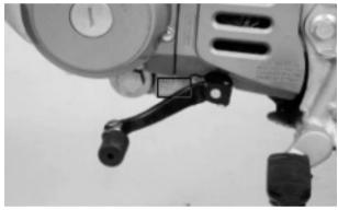
(2) The engine serial number is stamped on the lower left side of the crankcase.
