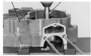
If the left crankshaft bearing remains on the crankshaft, remove it with universal bearing puller.
