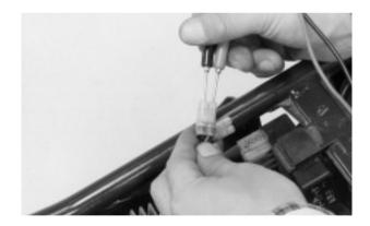
If the measurement is out of specifications, disconnet the exciter coil Black/Red connector and measure the resistance between the Black/Red and body ground.
