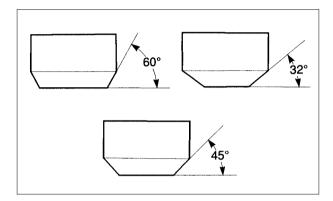
Use a 45 degree cutter to remove ant roughness or irregularities from the seat.
