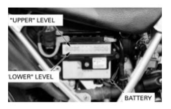
Measure the specific gravity of each cell with hidrometer.
