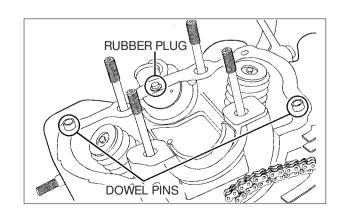
Apply oil to the cam lobes and camshaft bearings. Install the camshaft in the cylinder head, positioning the cam lobes down as shown.
