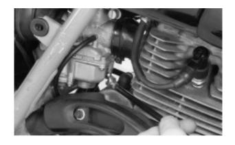
7. Adjust the idle speed with the throttle stop screw.
