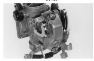
Install and tighten the cover screws.
