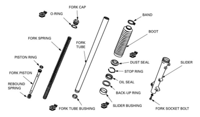
Before assembly, wash all parts with a high flash point or non-flammable solvent and wipe them off completely. Install the slider bushing, back-up ring and oil seal onto the fork tube.
