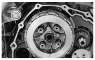
Install the clutch springs and lifter plate, and tighten the bolts in a crisscross pattern in 2-3 steps.
