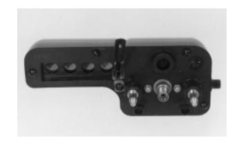
Remove the trip meter knob, then remove the speedometer.
