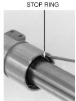
In quick successive back and forth strokes, pull the fork tube out from the slider.
