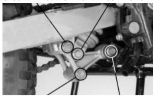
SHOCK LINK BOLT/NUT SHOCK ARM BOLT/NUT
