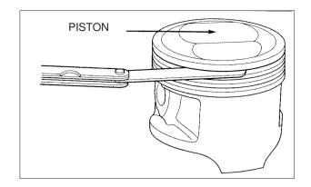
Insert each piston ring into the cylinder using the piston head and measure the ring end gap in the cylinder at a point 10 mm (0.4 in) from the bottom.
