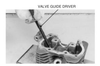
After driving in the valve guide, ream it with a valve guide reamer.
