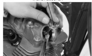
VALVE ADJUSTER WRENCH, 8 X 9 mm
