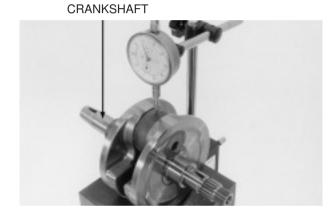
Set the crankshaft on a stand or V-blocks and read the runout using a dial indicator.
