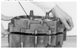
Remove the gasket and dowel pins.
