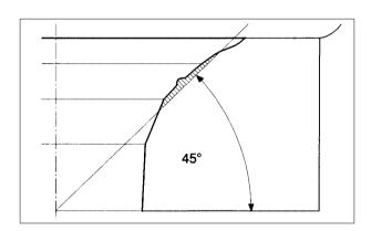
Using 32 degree cutter, remove 1/4 of the exiting valve seat material.
