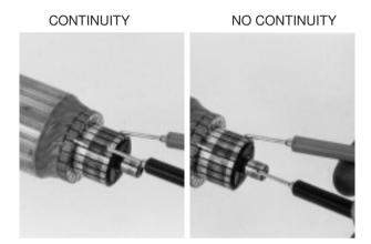
Check for continuity between cable terminal and the brush (the indigo covered wire or the insulated brush holder). There should be continuity.
