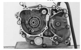
Place the left crankcase down and remove the right crankcase.
