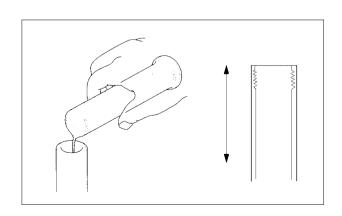
Install the fork spring B with the tapered end facing down. Install the fork spring B, spring seat and fork spring A into the fork tube.
