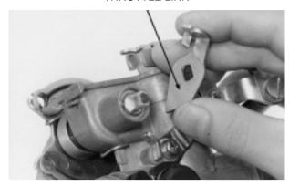
Install the washer and nut, then tighten the nut securely. Install and tighten the link arm screw.
