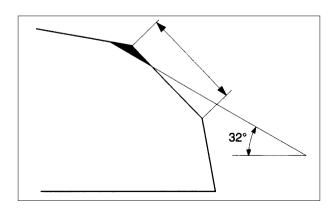
Using 60 degree cutter, remove the bottom 1/4 of the oil seat. Remove the cutter and inspect the area you have just removed.
