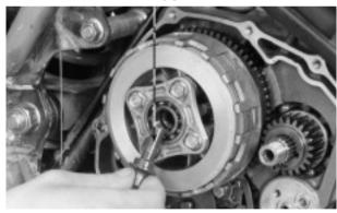
Install the clutch lifter guide.
