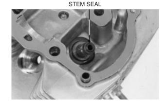
Lubricate each valve stem with engine oil. Insert the intake and exhaust valve into the valve guides. Install the valve spring seats, springs and retainers.
