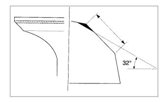
If the contact area is too low on the valve, the seat must be raised using a 60 degree inner cutter.
