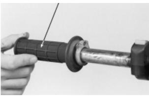
Connect the throttle cable end to the throttle pipe. Install the throttle cable guide.
