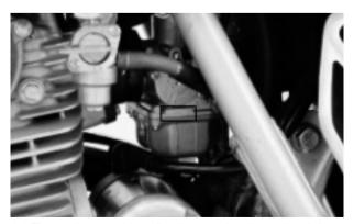
(3) The carburetor identification number is on the right side of the carburetor body.
