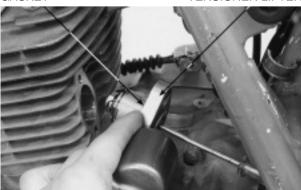
Tighten the cam chain tensioner lifter mounting bolts.
