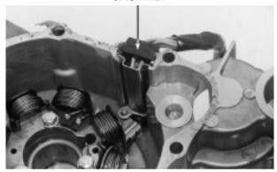
Insert the wire grommet into the groove in the left crankcase cover.
