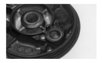
Install the brake cam seat, aligning its tabs with the projection of the brake panel.
