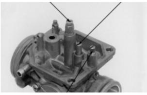
WASHER/O-RING/SPRING/PILOT SCREW **BAFFLE PLATE FLOAT**
