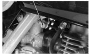
Adjust by loosening the lock nut and turning the adjusting screw until there is slight drag on the feeler gauge.
