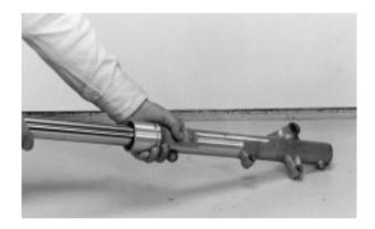
Remove the oil lock piece from the piston.
