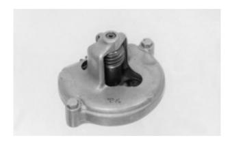
Install the outer and inner rotors. Install the gasket and pump cover.
