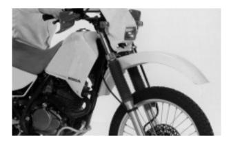
Tighten the upper axle holder nuts first, then the lower nuts.
