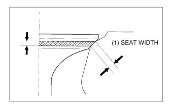
If the valve seat is too wide, too narrow or has low spots, the seat must be ground.
