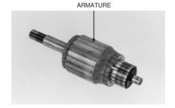
Check for continuity between individual commutator bars and the armature shaft; there should be no continuity.
