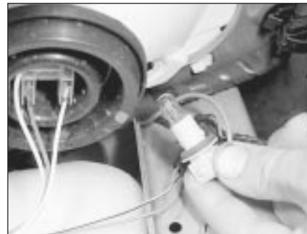
5.7 . . . and withdraw the sidelight bulbholder
