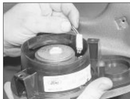
22.7B Detach the wiring from the speaker
