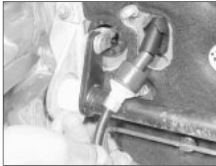
11.4 Withdrawing the speedometer cable through the bulkhead
