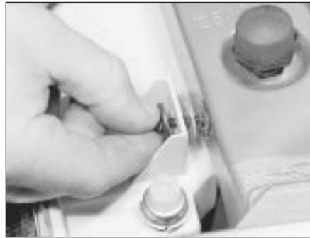
7.7B Headlight retaining screw showing washer arrangement
