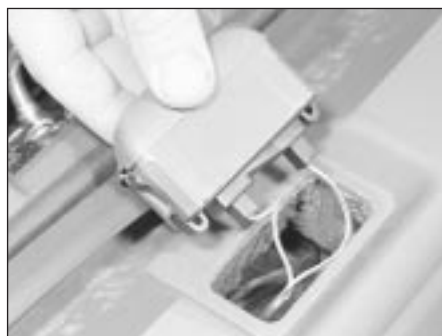
5.40 Number plate light removal from the bumper on Estate models
