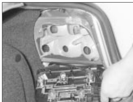
5.31A Rear bulbholder removal on pre-1993 Saloon and Hatchback models
