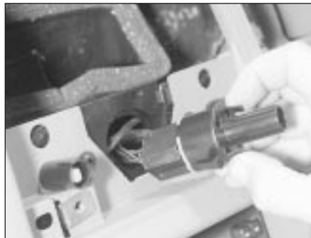
4.42 Heater blower motor switch removal
