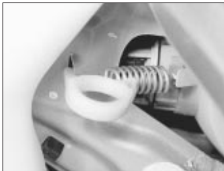
5.14 Front indicator unit retaining spring
