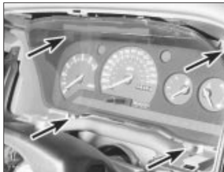
9.4A Instrument cluster retaining screws
