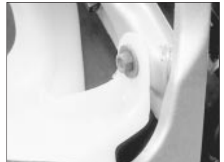
19.2 Washer reservoir retaining bolt in the engine compartment
