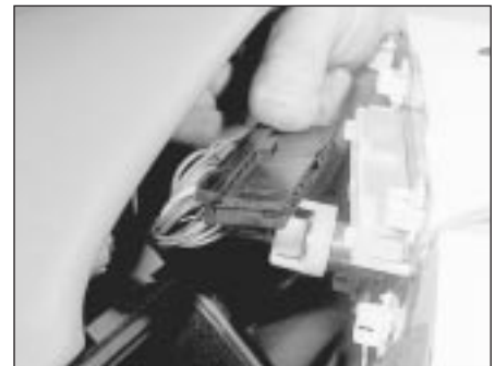
9.4B Detach the wiring multi-plugs from the instrument panel
