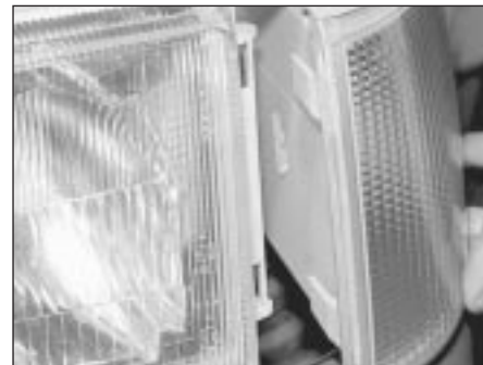
5.17 Engage the tags in their locating slots when refitting the front indicator unit
