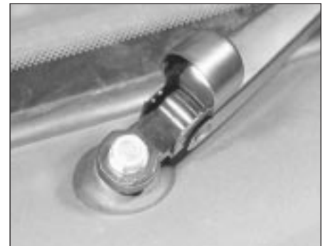
15.2 Windscreen wiper arm retaining nut
