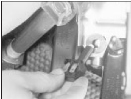
4.35 Brake stop-light switch removal
