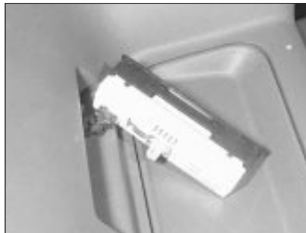
6.21B . . . for access to the bulbholder
