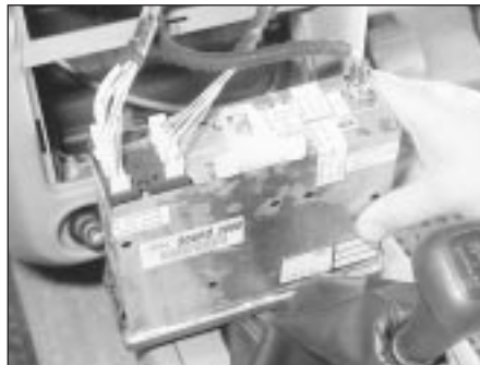
20.3 Wiring and aerial lead connections on the rear face of the radio/cassette
