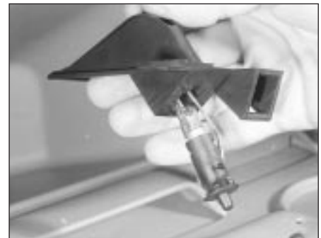
6.17 Glovebox light switch/bulbholder removal
