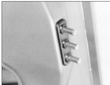
4.26 Contact switch unit in the tailgate
