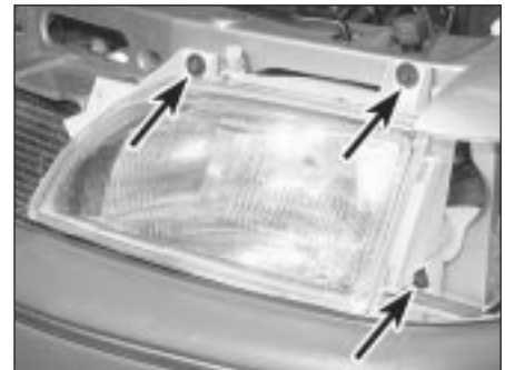
7.5 Headlight unit retaining screws (arrowed)
