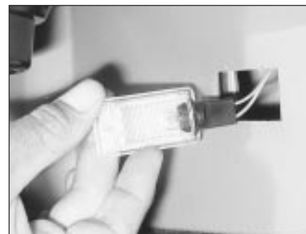
6.4 Luggage area light removed for bulb replacement
