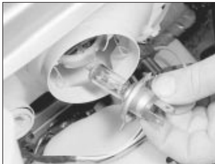
5.3 . . . and withdraw the headlight bulb
