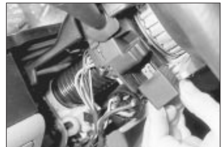
3.7 Direction indicator flasher relay removal
