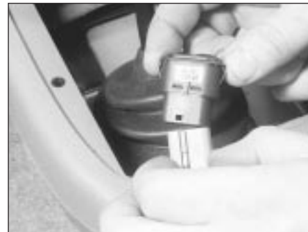
4.46 Electric window switch removal
