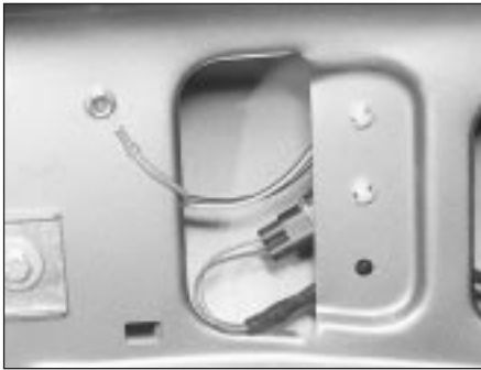
18.6 Tailgate wiper earth lead and in-line connector
