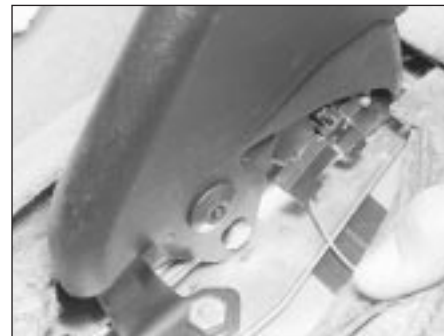
4.31 Handbrake warning light switch
