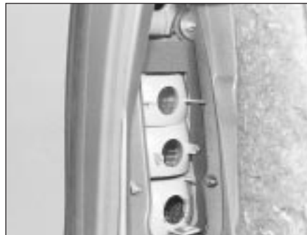
7.34 Rear light lens showing the retaining nuts
