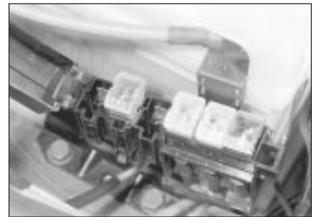
3.4 Additional "main" fuses at the front of the battery
