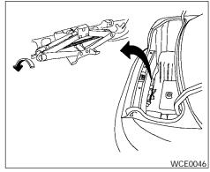
2. To remove the jack, turn the jack screw counterclockwise. Use the tapered end of the jack rod to loosen the jack from its storage position.
