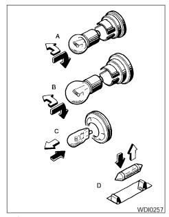
↑ Indicates bulb removal Indicates bulb replacement
