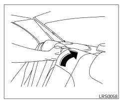
When using the fold down rear seatback, the rear center seat belt retractor may lock up and prevent folding down the seatback.
