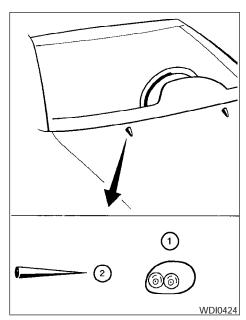
If you wax the surface of the hood, be careful not to let wax get into the washer nozzle 1. This may cause clogging or improper windshield washer operation. If wax gets into the nozzle, remove it with a needle or small pin (2).
