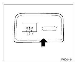
To defrost the rear window glass, start the engine and push the rear window defroster switch on. The rear window defroster indicator light on the switch comes on. Push the switch again to turn the defroster off.
