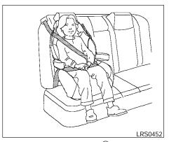
low back booster seat ① is chosen, the vehicle seat back must be at or above the center of the child's ears. If the seat back is lower than the center of the child's ears, a high back booster seat ② should be used.
