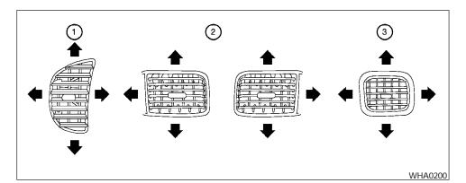
Adjust air flow direction for the driver's side (1), center (2), and passenger side (3) ventilators by moving the ventilator slide and/or ventilator assemblies.
