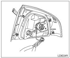
Rear combination light side maker bulb Use flat nose pliers to turn the bulb socket.
