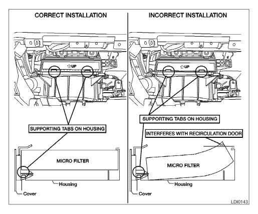
NOTE: Make sure the filter sits on top of the two supporting tabs on the housing.
