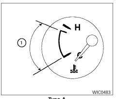
Type A **ENGINE COOLANT TEMPERATURE GAUGE**
