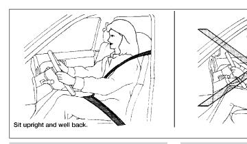
Keep hands on the outside of the steering wheel. Placing them inside the steering wheel rim could increase the risk that they are injured when the supplemental front air bag inflates.
