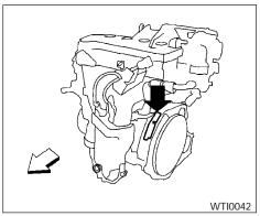
**QG18DE** engine **ENGINE SERIAL NUMBER**
