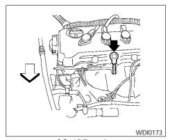
**QG18DE** engine CHECKING ENGINE OIL LEVEL
