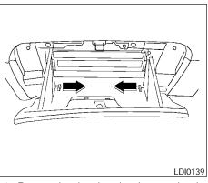
1. Remove the glove box door by removing the two lower hinge pins.
