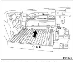
NOTE: The filter is marked "UP" with an arrow. The end of the filter with the arrow should face the rear of the vehicle.
