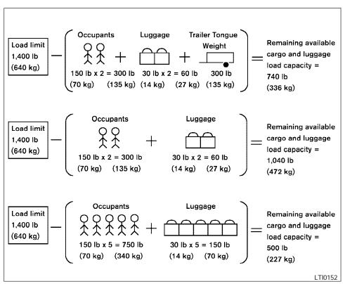
Steps for determining correct load limit
