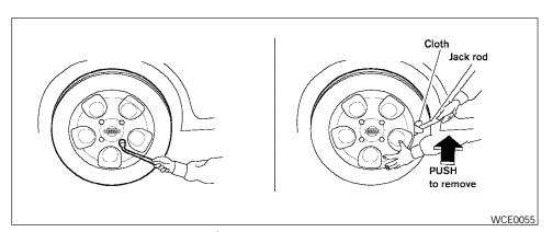
Removing bolt-on wheel cover (if so equipped)
