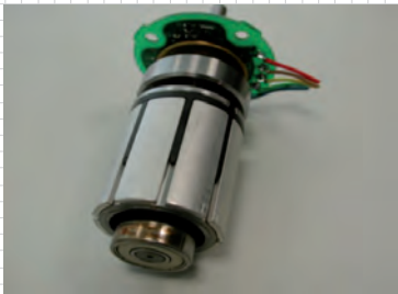
Rotor with four pairs of permanent magnets
