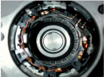
Stator with six solenoid pairs and three position sensors
