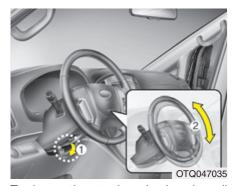
To change the steering wheel angle, pull down the lock-release lever (1), adjust the steering wheel to the desired angle (2), then pull up the lock-release lever to lock the steering wheel in place. Be sure to adjust the steering wheel to the desired position before driving.
