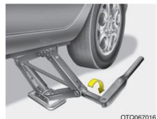
8. Insert the jack handle into the jack and turn it clockwise, raising the vehicle until the tire just clears the ground. This measurement is approximately 30 mm (1.2 in). Before removing the wheel lug nuts, make sure the vehicle is stable and that there is no chance for
