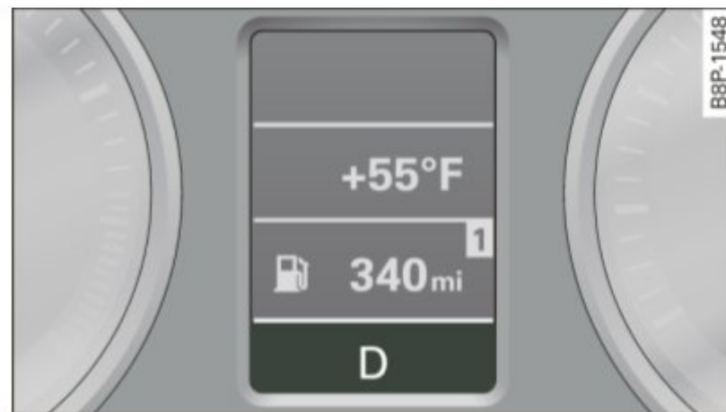
Fig. 114 Display: Selector lever positions
