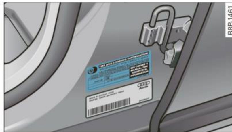
Fig. 171 Tire pressure label: located either on driver's side B-pillar or inside the fuel filler flap
