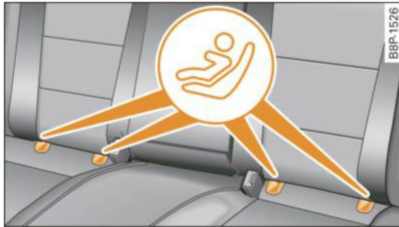
Fig. 149 Rear seat-backs: locator buttons for lower anchorages
