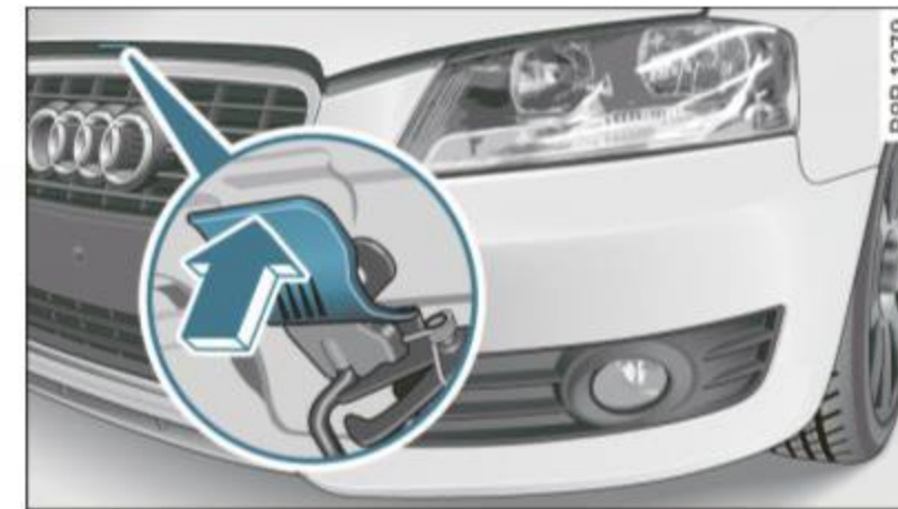
Fig. 160 Engine hood release lever
