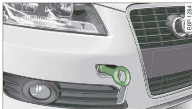
Fig. 199 Front bumper: screwing in the towing loop
