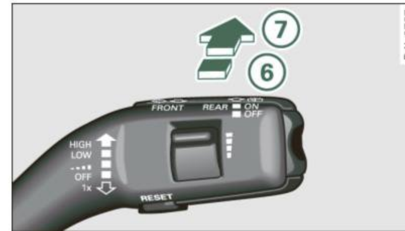
Fig. 63 Wiper lever: activating the rear window wiper and washer
