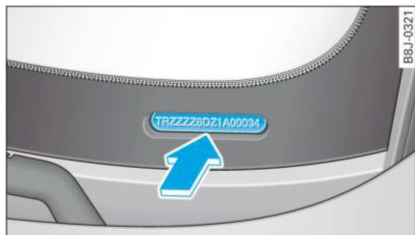
Fig. 205 Vehicle Identification Number (VIN) plate: location on driver's side dash panel
