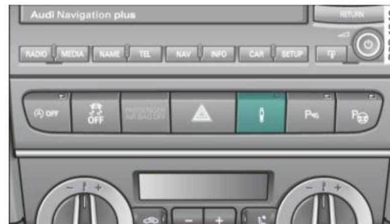
Fig. 112 Center console: Switch for Audi magnetic ride
