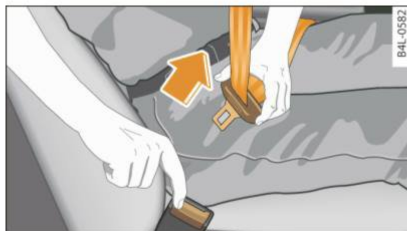
Fig. 134 Releasing the tongue from the buckle
