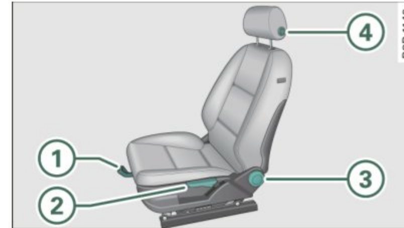
Fig. 69 Adjustment controls: locations on driver's seat
