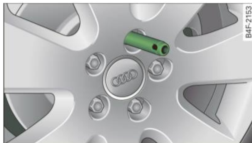
Fig. 192 Wheel change: alignment pin inside the top hole
