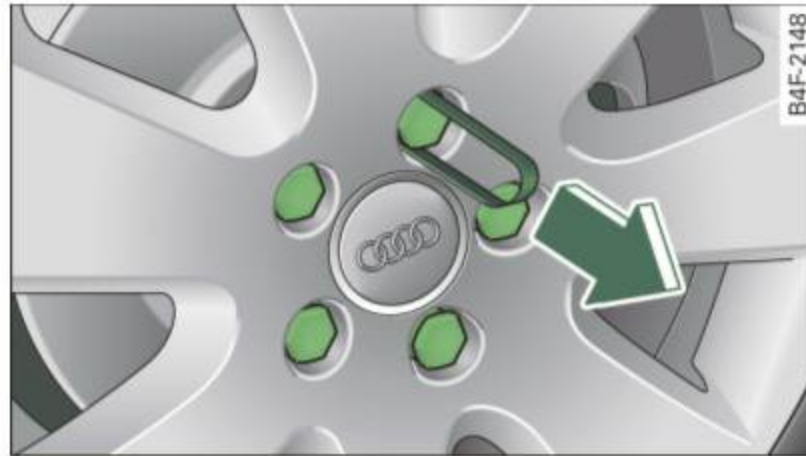
Fig. 186 Wheel change: removing the wheel bolt caps
