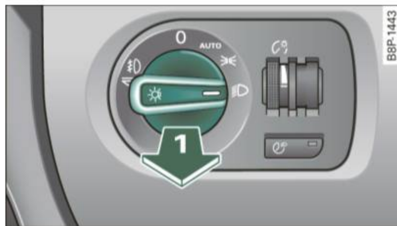
Fig. 51 Fog light activation: light switch position on vehicles WITHOUT sensor light
