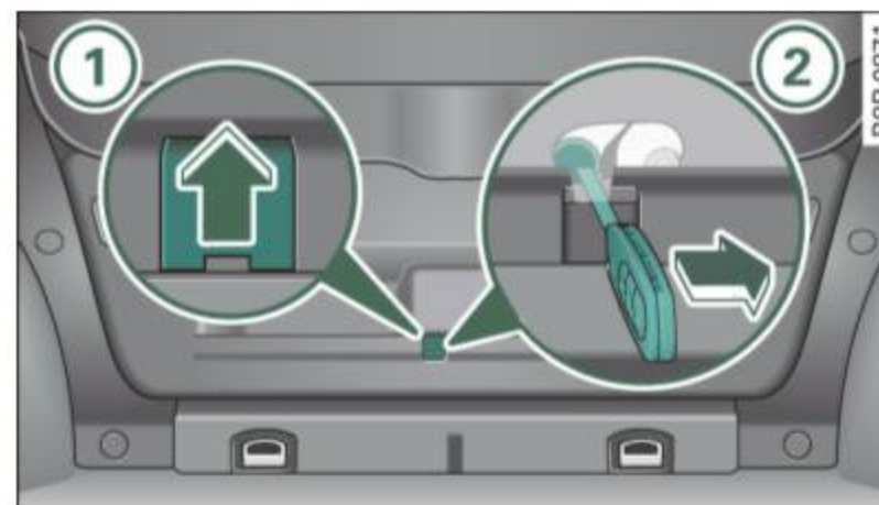
Fig. 36 Rear lid interior section: Emergency release
