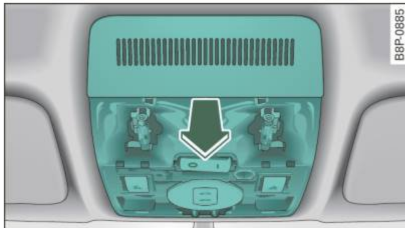
Fig. 46 Removing the light unit
