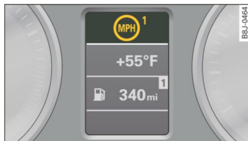
Fig. 21 Display: speed warning system
