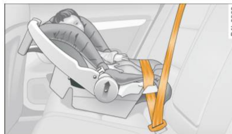
Fig. 144 Schematic overview: rearward-facing infant seat, properly installed on the rear seat
