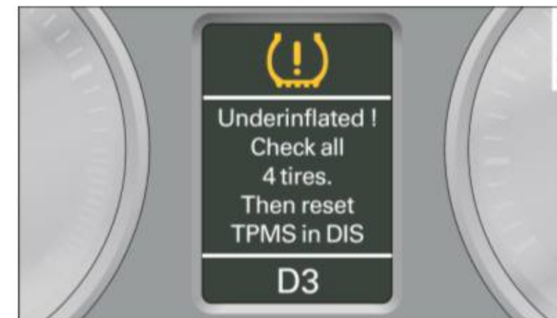
Fig. 176 Display: underinflation warning
