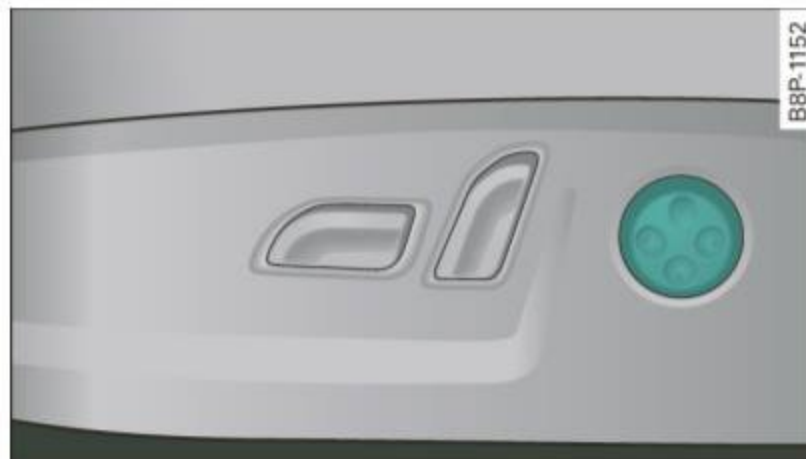
Fig. 73 Driver seat: switch for lumbar adjustment
