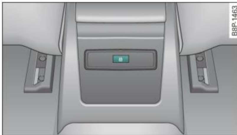
Fig. 32 Rear power locking switch
