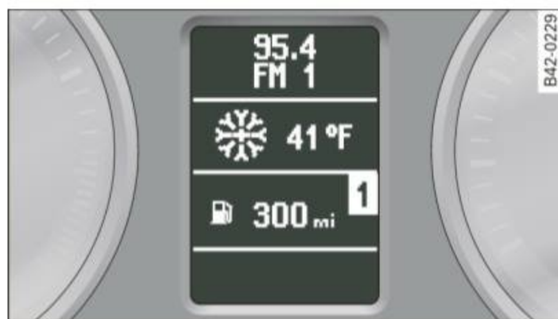
Fig. 6 Instrument cluster: center display
