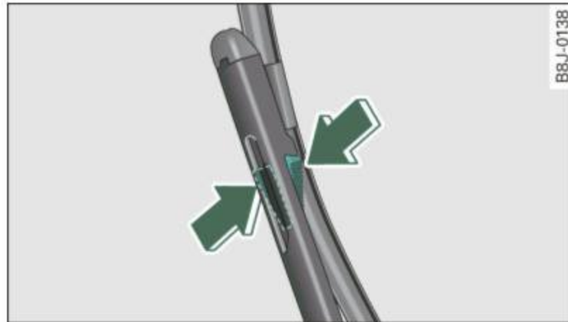
Fig. 64 Unlatching wiper blades
