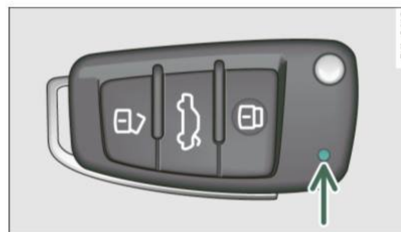
Fig. 27 Check light in the master key
