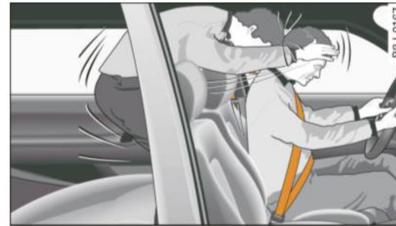
Fig. 129 A rear passenger not wearing a safety belt will fly forward and strike the driver
