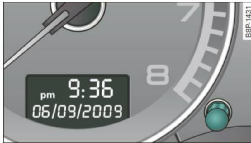
Fig. 22 Section of instrument cluster: Set/Check button
