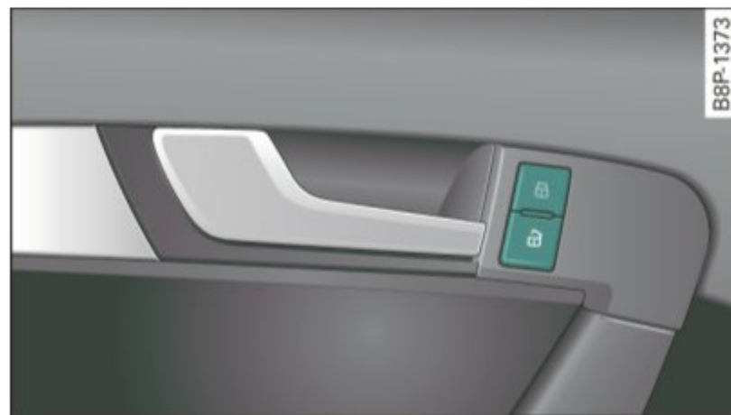
Fig. 31 Driver's door: power locking switch
