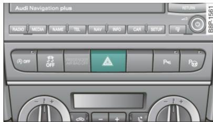
Fig. 53 Center console: emergency flasher switch
