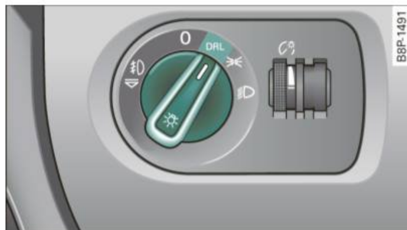
Fig. 50 Instrument panel: Light switch with daytime running lights (DRL)
