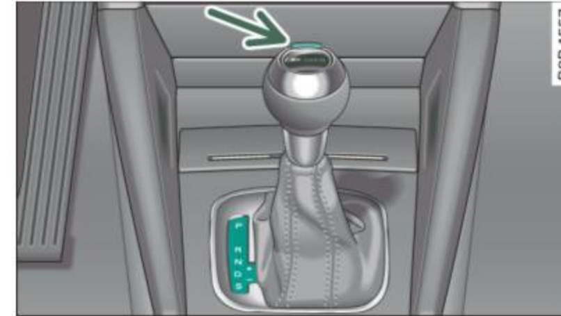
Fig. 116 Section from center console: Selector lever with release button
