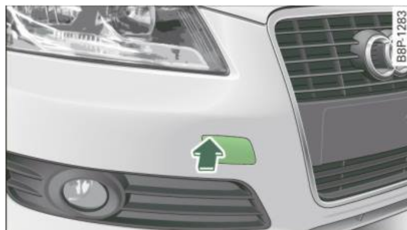
Fig. 198 Front bumper: removing the cover cap
