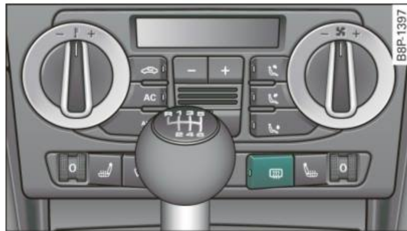
Fig. 103 Switch for rear window defogger with air-conditioning
