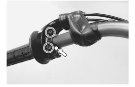
• Remove the handlebar holder bolts and remove the handlebars.
