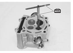
Cool down the new valve guides in a freezer for about one hour and heat the cylinder head to 100 – 150 °C (212 – 302 °F) with a hot plate.
