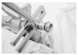
• Tighten the center bolt to the specified torque.
