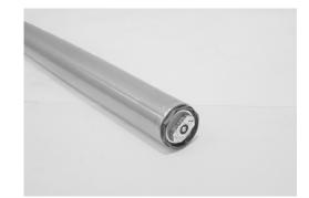
• Temporarily tighten the fork cap bolt (sub-tank).
