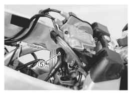
• Loosen the carburetor clamp screws and take out the carburetor from between the carburetor holder and air cleaner duct.
