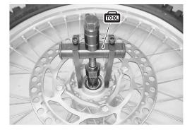
• Reassemble the bearings with the special tools, using the suitable spacer (A) match for the outside dimension of bearings.
