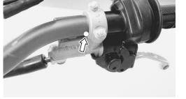
• Remove the throttle housing cover screws.
