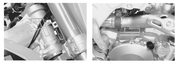
The frame number 1 is stamped on the steering head as shown in the photograph. The engine serial number 2 is stamped on the right side of the crankcase assembly. Write down the serial numbers here for your future reference.
