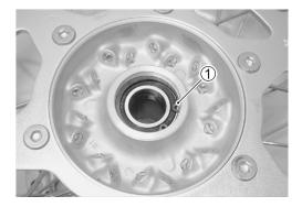
• Remove the dust seals with the special tool.
