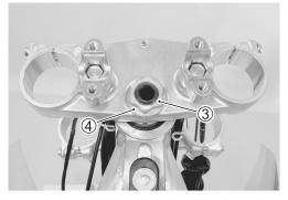
• Remove the handlebar holder set bolts and nuts.
