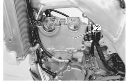
• Install the seal washers to the cylinder head bolts as shown.
