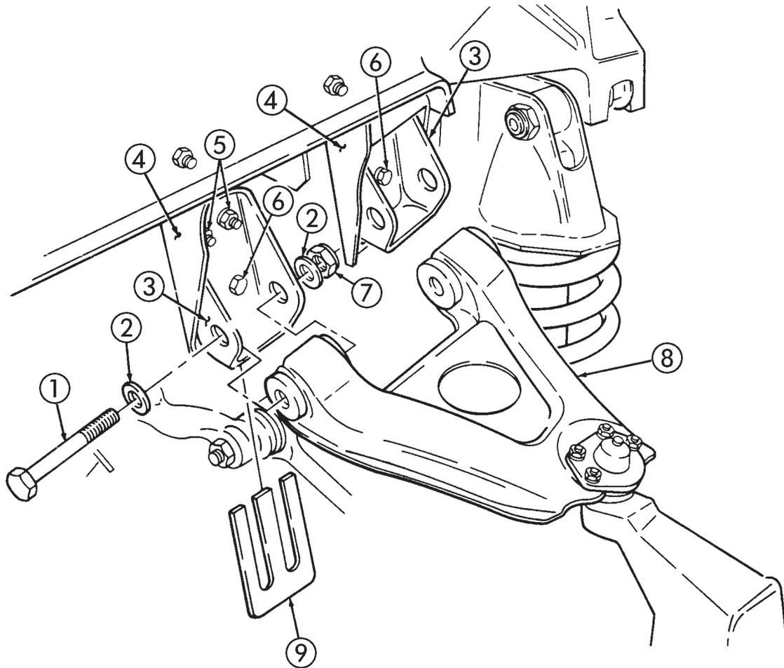
Figure 7-14 (Repeat). Caster and Camber Adjustment.
