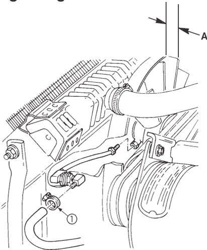
Figure 1-11. Fan Shroud Adjustment.
