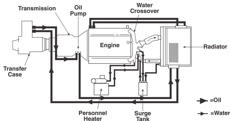
Figure 1-12. Cooling System Schematic.
