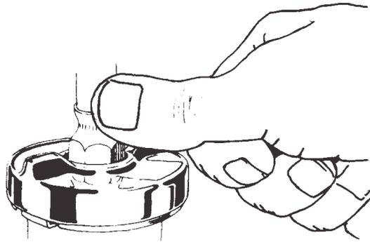
Figure 1-6. Releasing Cooling System Pressure Tester.
