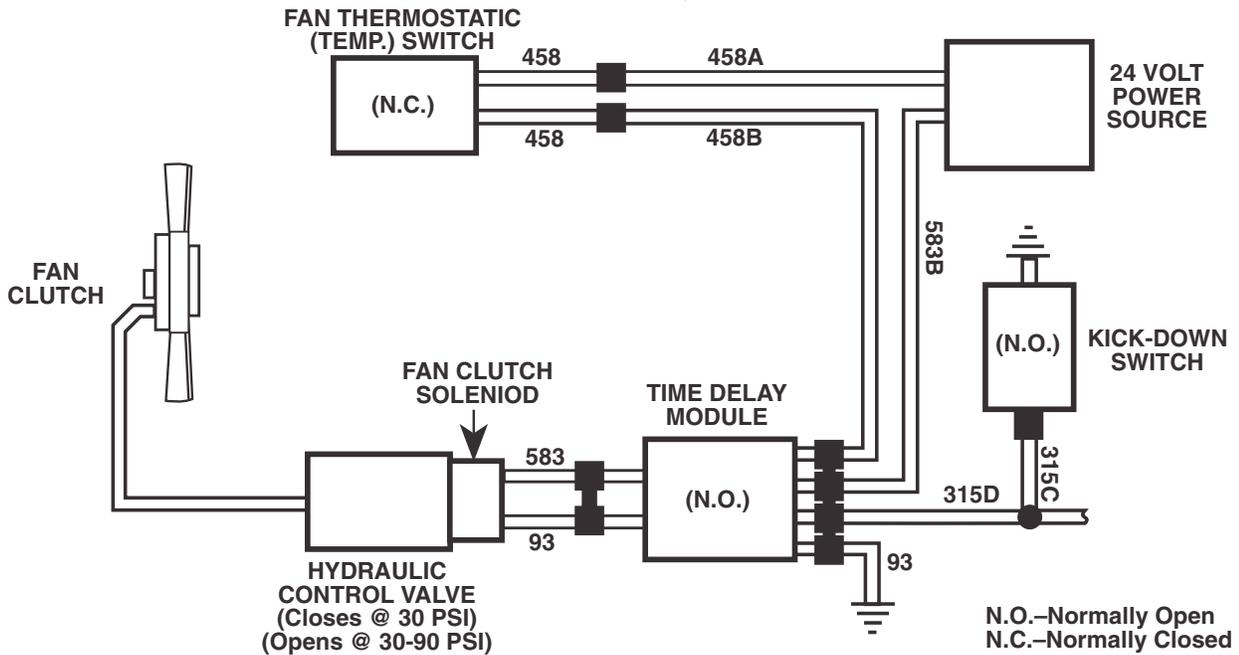
Figure 1-2. Fan Clutch Solenoid Resistance Test Hookup.
