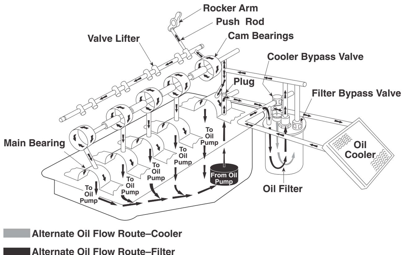
Figure 1-13. Engine Lubrication System Schematic.
