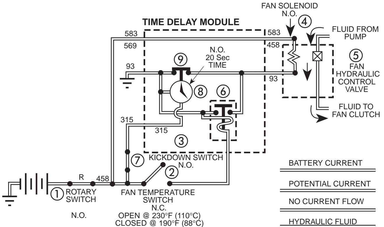
Figure 13-4. Fan Temperature Switch Open
