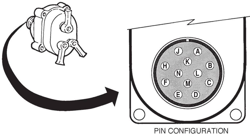
Figure 12-12. Master Lightswitch Pin Configuration.
