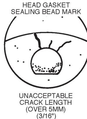
Figure 4-14. Pre-chamber Cracks.
