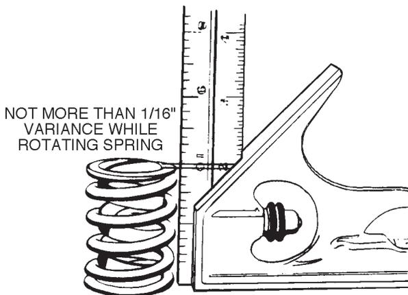
Figure 4-15. Valve Spring Check.
