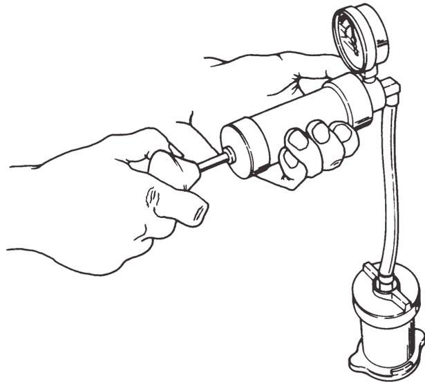
Figure 1-9. Pressure Cap Test.
