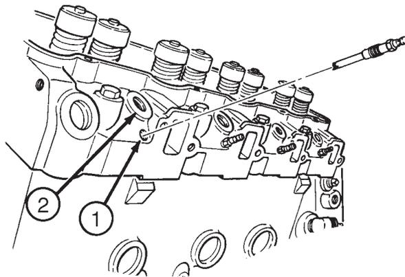
Figure 4-2. Damaged Glow Plug Removal
