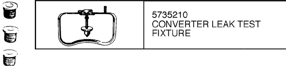
Figure 6-12. Converter Leak Tst Fixture.
