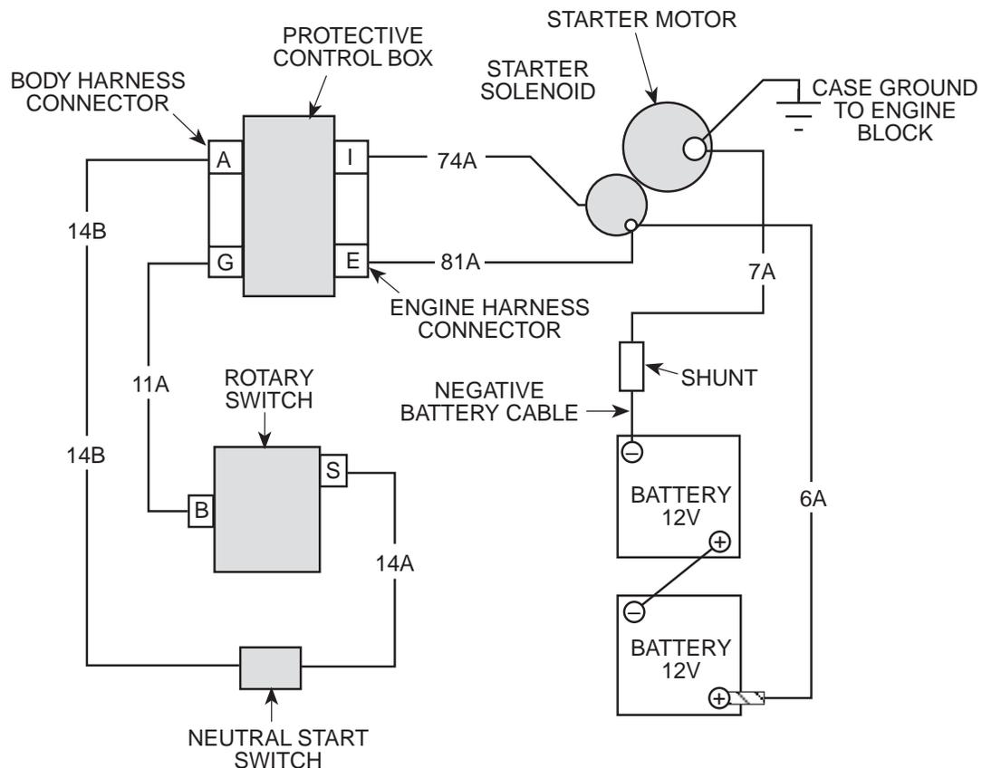
Figure 12-10. Starting System Schematic—Protective Control Box Testing.
