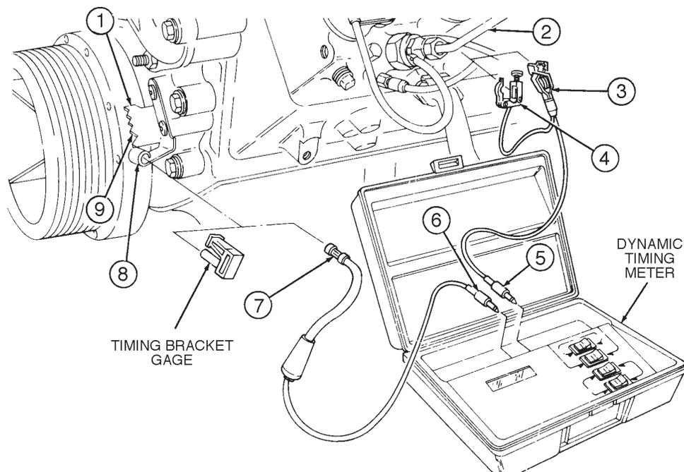
Figure 4-3. Engine Injection Pump Timing Meter Hook-up.
