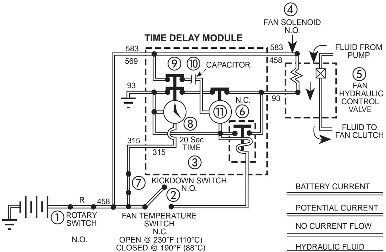
Figure 13-5. Fan Temperature Switch Open
