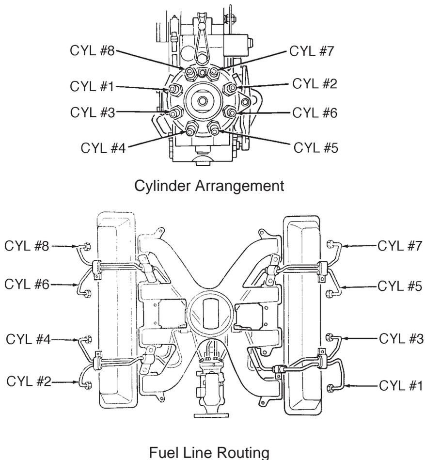
Figure 3-1. Cylinder Arrangement and Fuel Line Routing.
