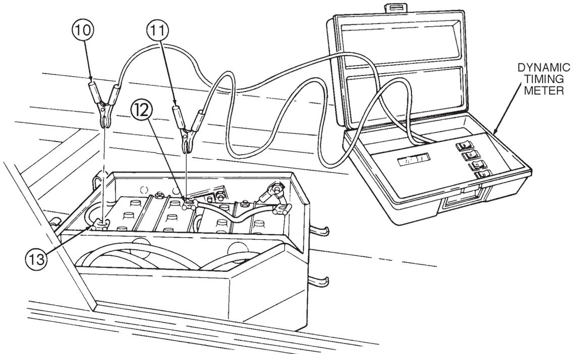
Figure 4-4. Timing Meter Power Hook-up
