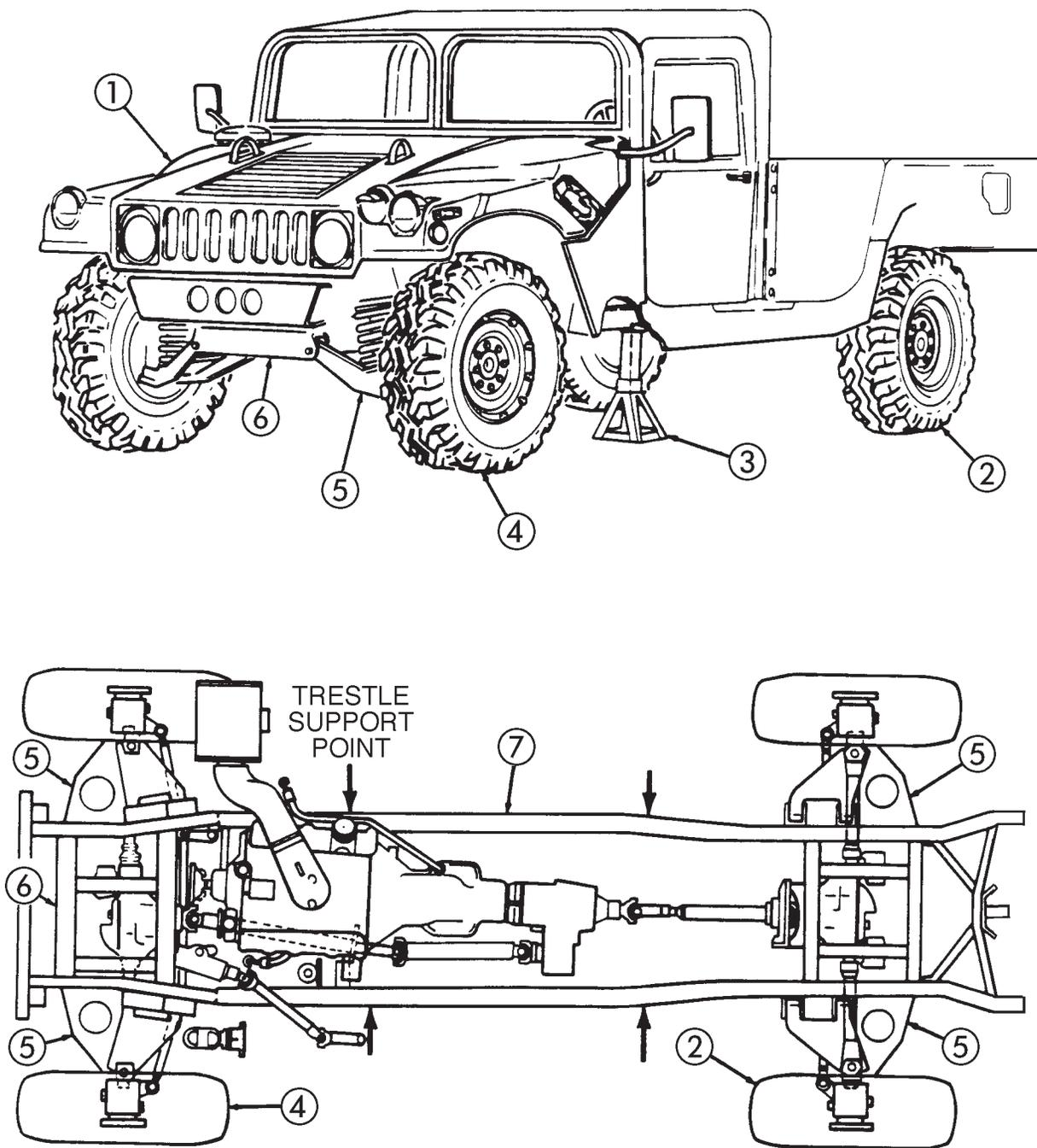
Figure 8-1. Front and Corner Jacking Procedures.
