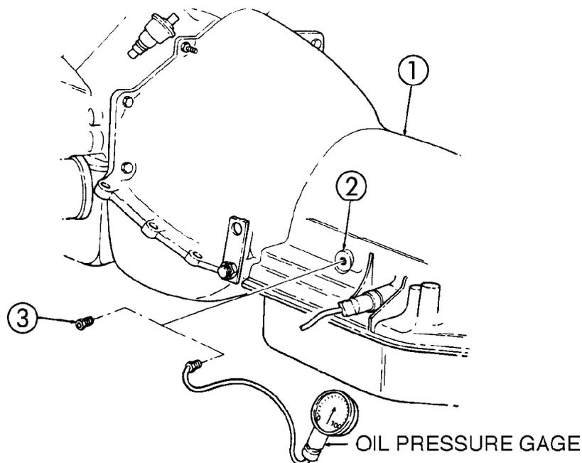
Figure 6-6. Transmission Oil Pressure Test Hook-up.
