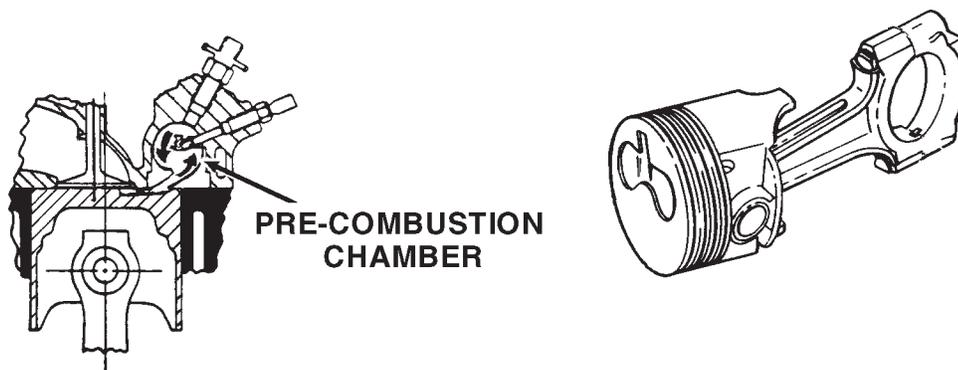
Figure 4-1. Pre-combustion Chamber and Piston Crown Shape.
