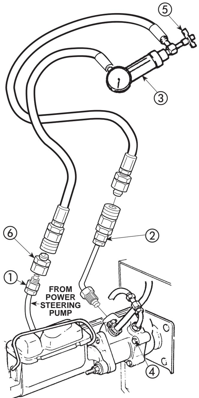
Figure 9-1. Power Steering Test Hook-up
