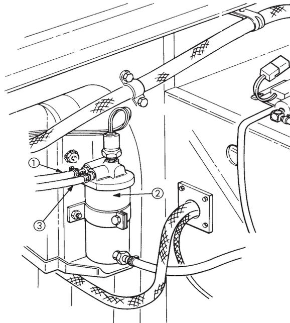
Figure 3-4. Fuel Filter Pressure Test Hook-up
