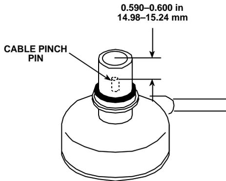
Figure 6-2. Modulator Pinch Pin Depth.
