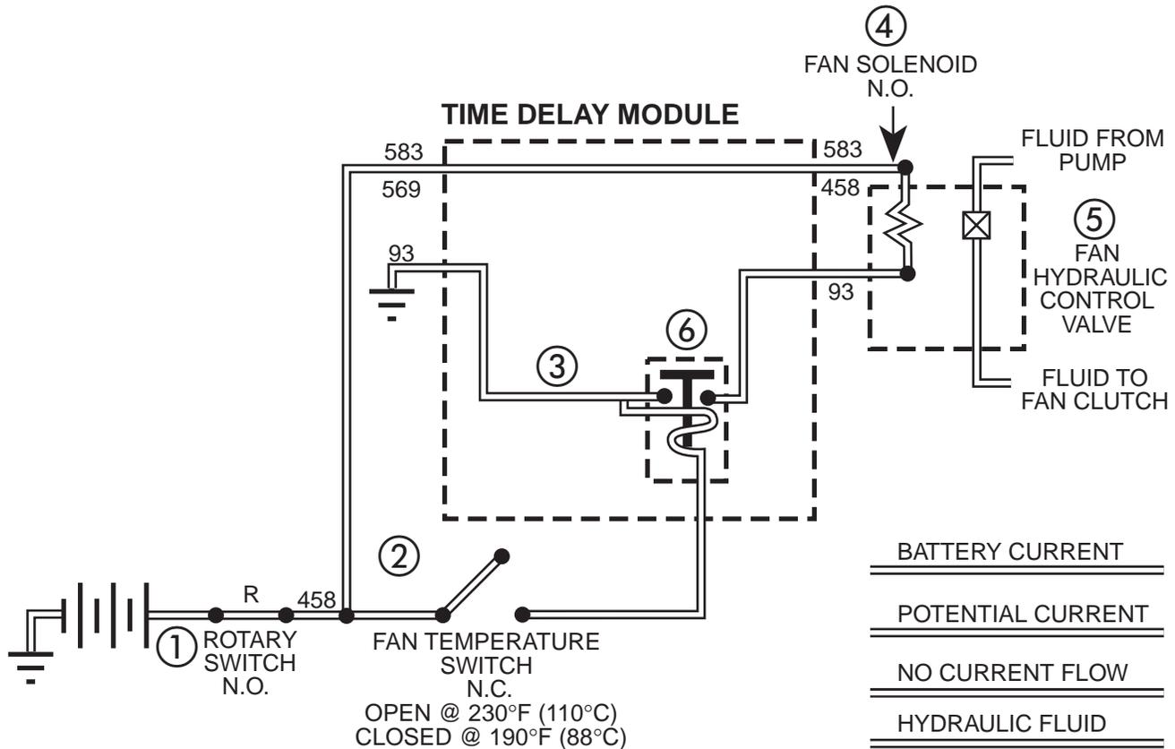
Figure 13-3. Fan Temperature Switch Closed
