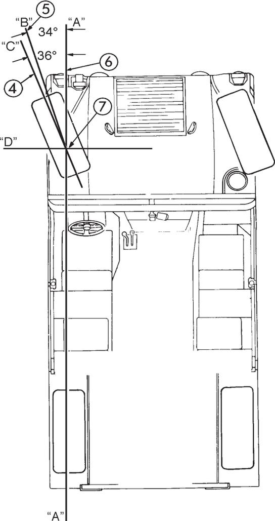
Figure 7-11. Steering Stop Reference line
