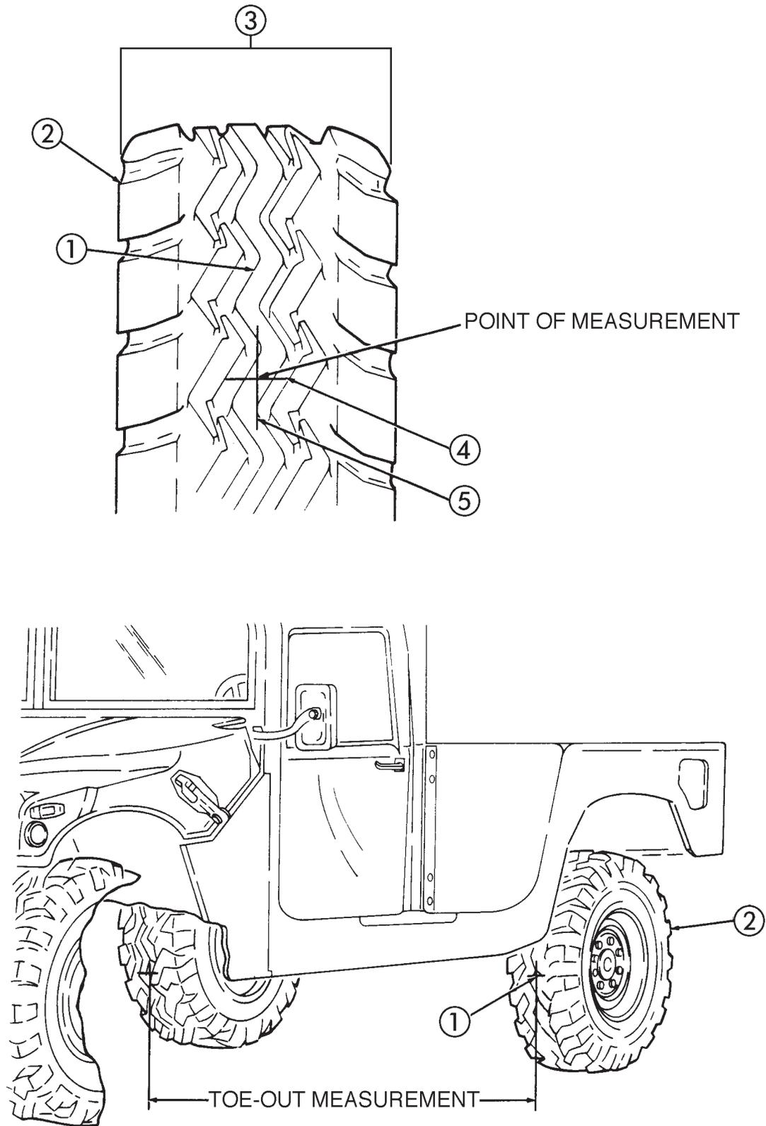
Figure 7-8. Toe-Out Points of Measurement.
