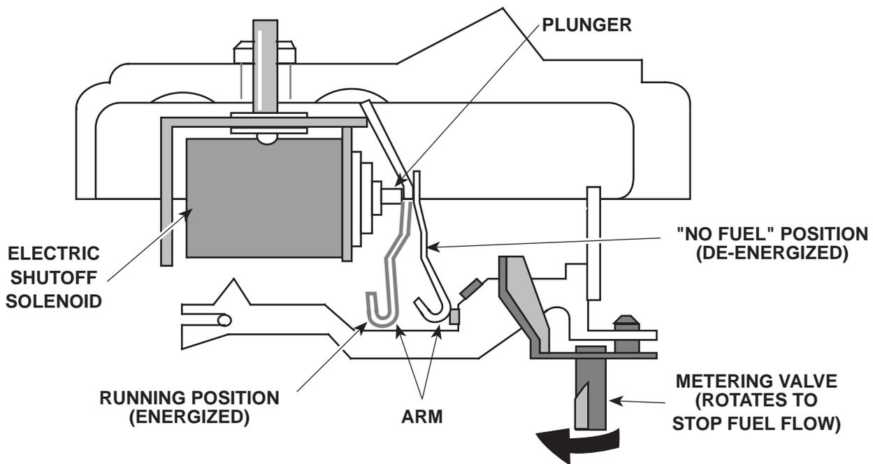
Figure 3-9. Electrical Shutoff Solenoid.
