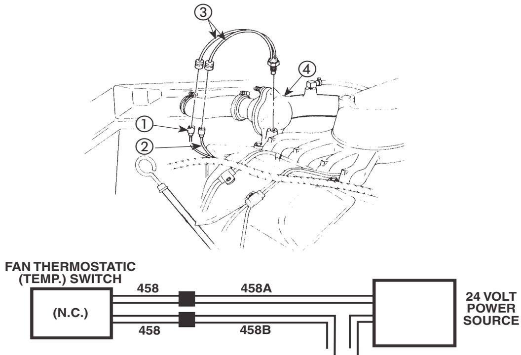
Figure 1-1. Fan Thermostatic Switch Testing Hookup.
