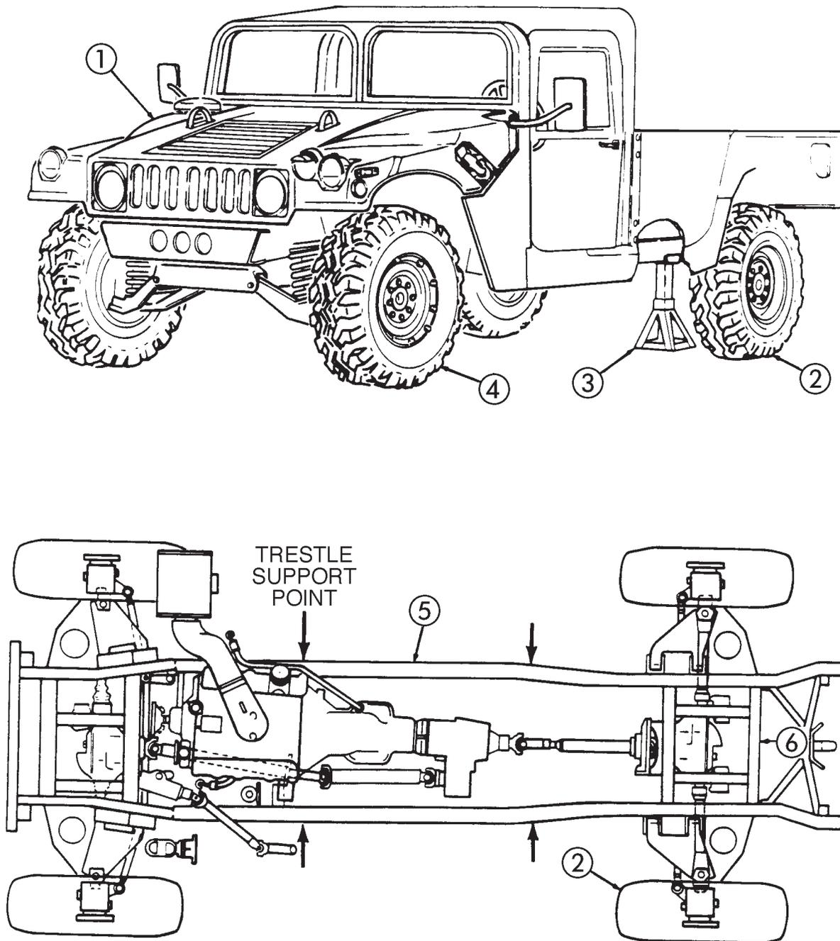
Figure 8-2. Rear and Entire Vehicle Jacking Procedures.
