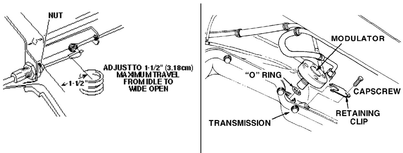
Figure 6.3. Modulator Maintenance and Adjustment.
