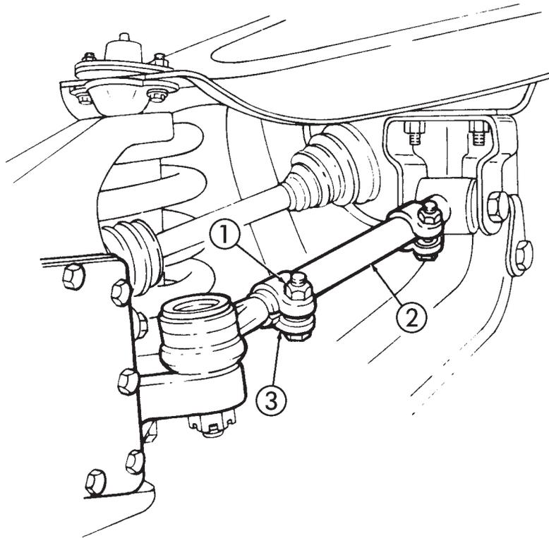
Figure 7-9. Toe -out Adjustment.
