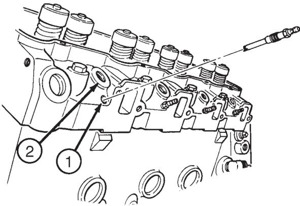
Figure 4-13. Glow Plug Removal
