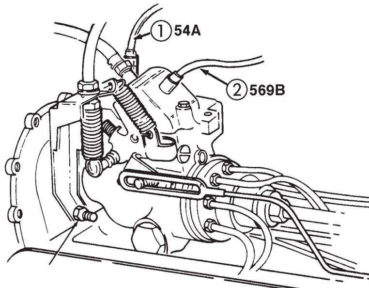
Figure 3-7. Fuel Solenoid Test Hook-up.
