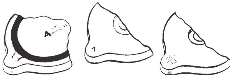
Figure 1-7. Pressure Cap Markings
