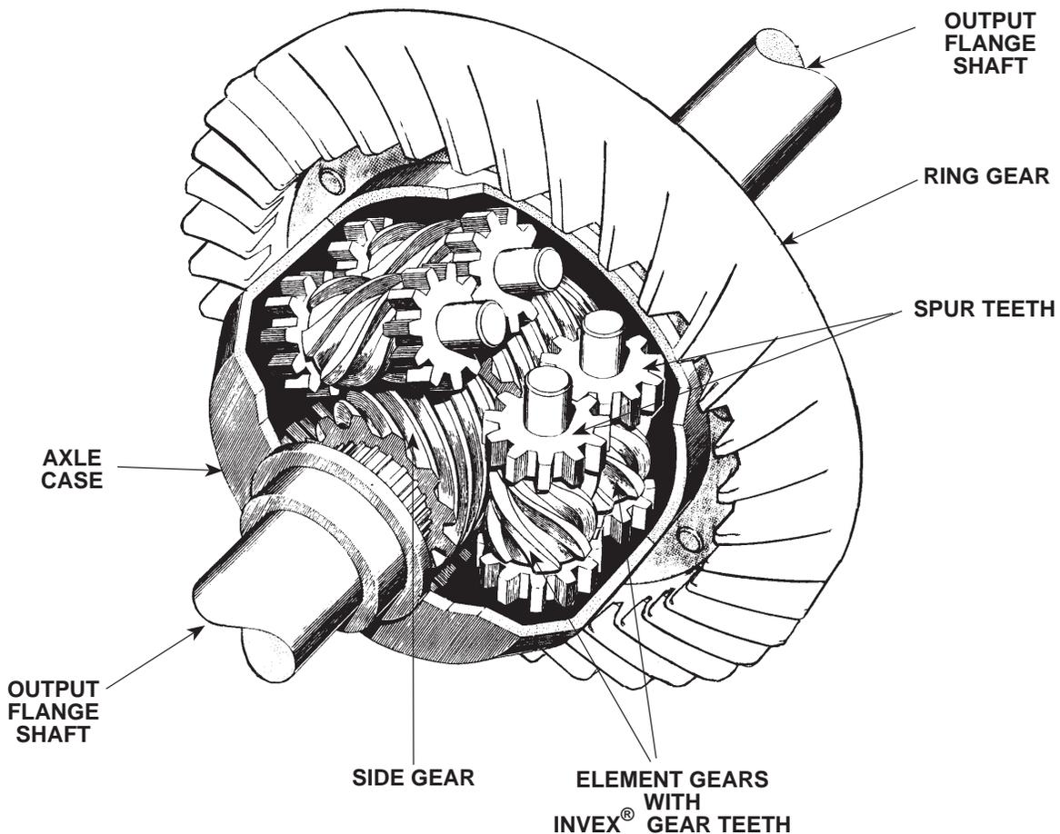
Figure 11-1 Repeat. Torsen Differential.
