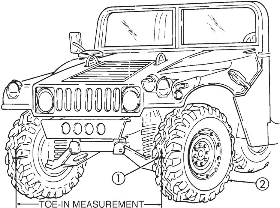
Figure 7-5. Toe-in Measurement Check.
