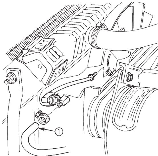
Figure 1-3. Fan Clutch Valve Pressure Test Hookup.
