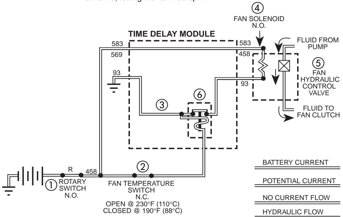
Figure 13-2. Fan Temperature Switch Closed,
