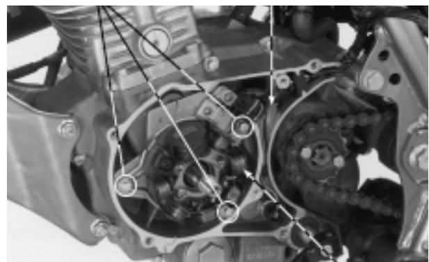
ESTATOR CONEXION 6P CONEXION NEGRA/ROJA
