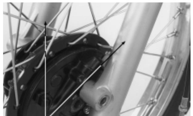
**AMORTIGUADORES DELANTEROS****CABLE DEL VELOCIMETRO**
