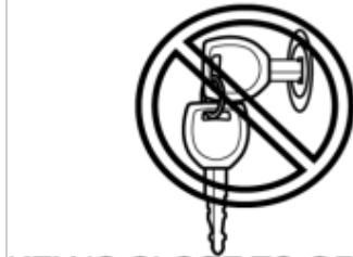
KEY IS CLOSE TO OR TOUCHING ANOTHER IMMOBILIZER SYSTEM KEY
