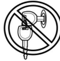
KEY IS CLOSE TO OR TOUCHING ANOTHER IMMOBILIZER SYSTEM KEY
