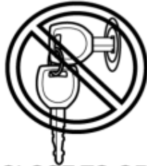
KEY IS CLOSE TO OR TOUCHING ANOTHER IMMOBILIZER SYSTEM KEY
